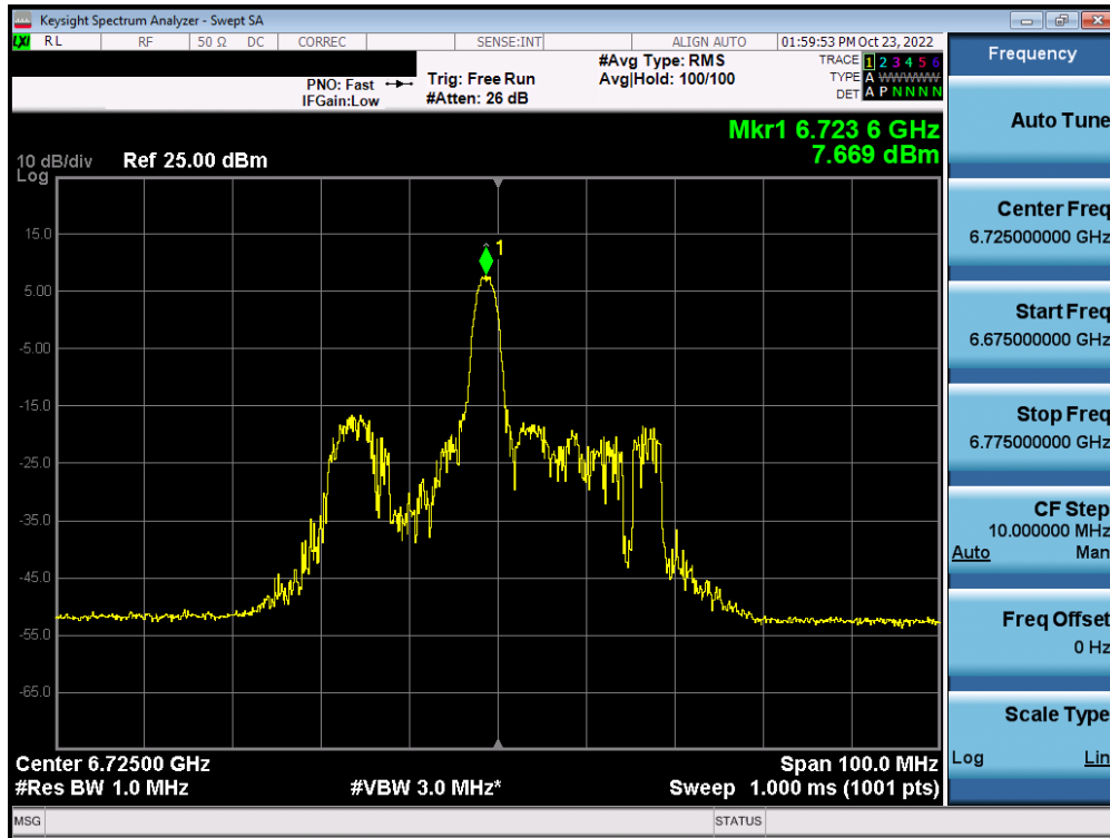
Plot 7-275. Power Spectral Density Plot MIMO ANT1 (40MHz BW 802.11ax (26 Tones) (UNII Band 7) – Ch. 155) – SP
