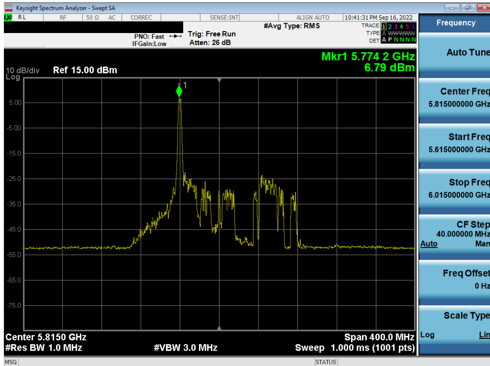
Plot 7-263. Power Spectral Density Plot MIMO ANT2 (160MHz BW (L) 802.11ax – 26 Tones (UNII Band 3/4) – Ch. 163)
