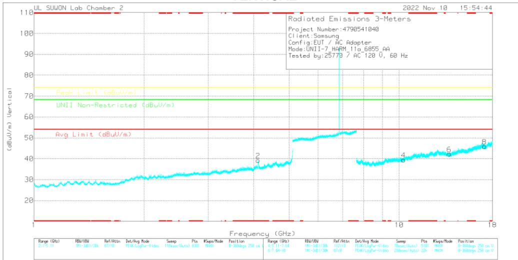
Note. Emission was scanned up to 40GHz; No emissions were detected above the noise floor which was at least 20dB below the specification limit.
