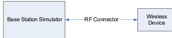
Figure 9-3 Power Measurement Setup – NR FDD
