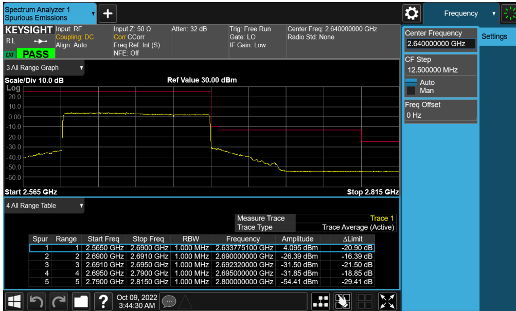
Plot 7-491. Upper ACP Plot (NR Band n41 - 100MHz CP-OFDM-QPSK – Full RB - Ant F)
