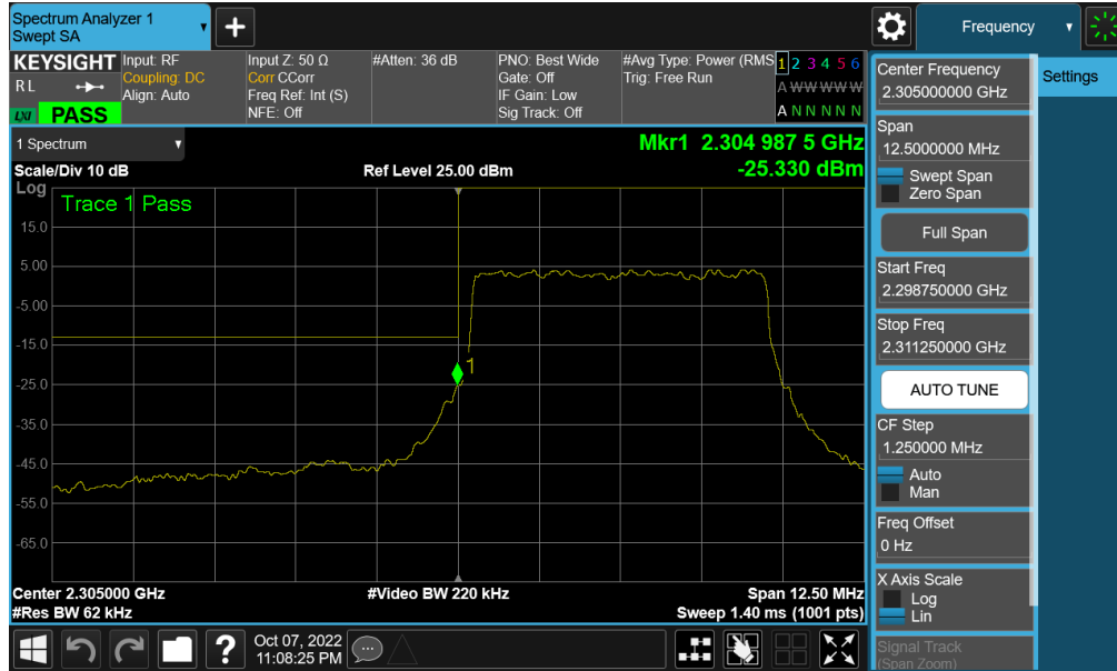
Plot 7-457. Lower Band Edge Plot (NR Band n30 - 5MHz CP-OFDM-QPSK – Full RB - Ant F)
