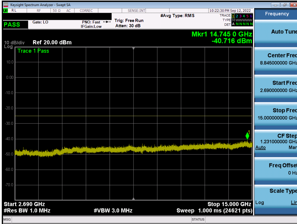
Plot 7-363. Conducted Spurious Plot (ULCA LTE B41(PC3) - 20MHz QPSK - RB Size 1, RB Offset 0 - Mid Channel - Ant B)
