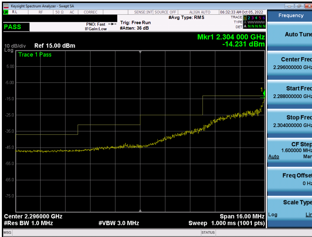
Plot 7-386. Extended Lower Band Edge Plot (LTE Band 30 - 5MHz QPSK – Full RB - Ant A)
