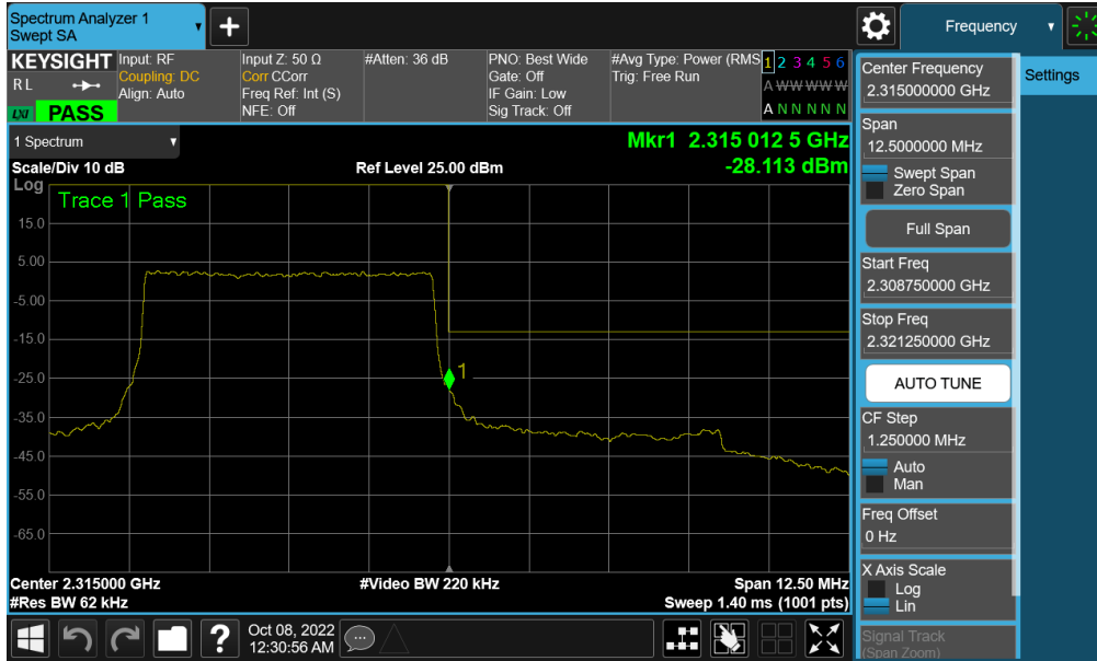
Plot 7-395. Upper Band Edge Plot (LTE Band 30 - 5MHz QPSK – Full RB - Ant F)
