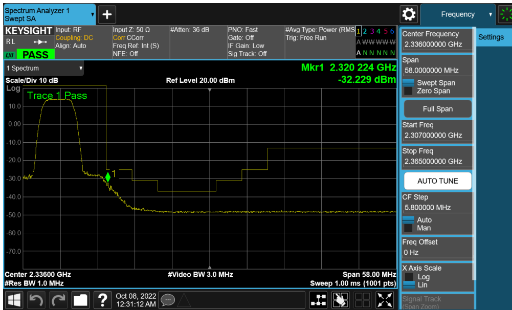
Plot 7-396. Extended Upper Band Edge Plot (LTE Band 30 - 5MHz QPSK – Full RB - Ant F)
