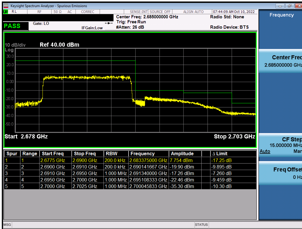
Plot 7-418. Upper ACP Plot (LTE Band 41(PC2) - 10MHz QPSK - Full RB - Ant B)
