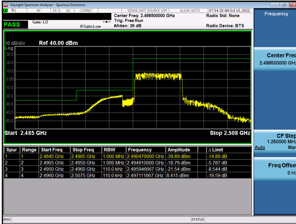
Plot 7-419. Lower ACP Plot (LTE Band 41(PC2) - 5MHz QPSK - Full RB - Ant B)
