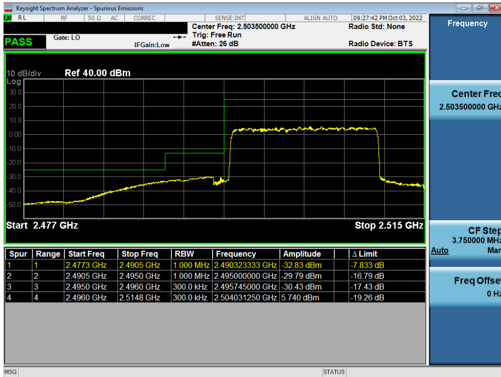
Plot 7-439. Lower ACP Plot (LTE Band 41(PC3) - 15MHz QPSK - Full RB - Ant F)
