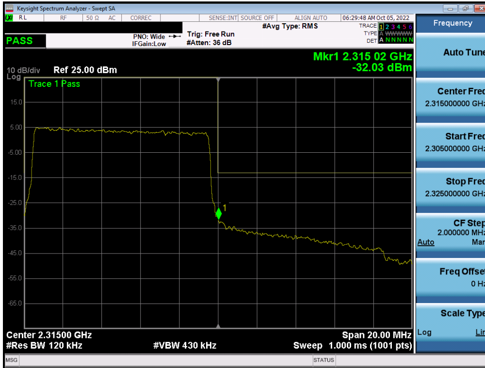
Plot 7-383. Upper Band Edge Plot (LTE Band 30 - 10MHz QPSK – Full RB - Ant A)
