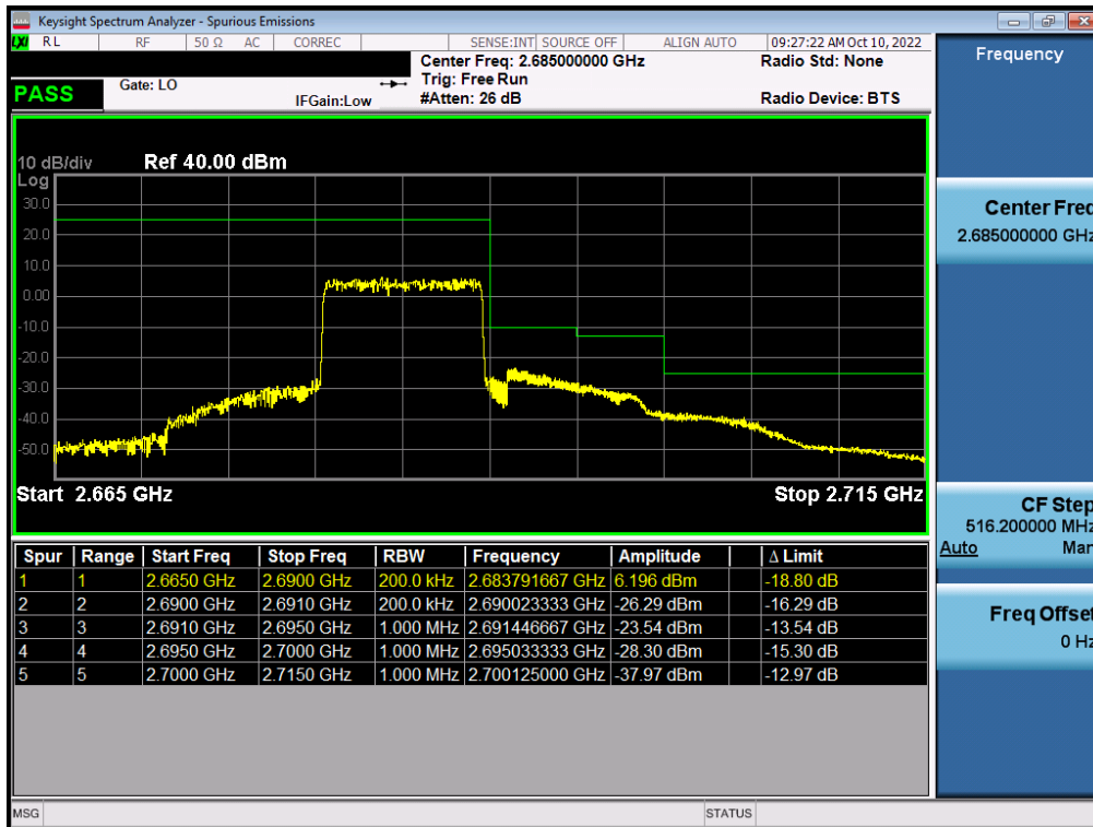
Plot 7-434. Upper ACP Plot (LTE Band 41(PC3) - 10MHz QPSK - Full RB - Ant B)
