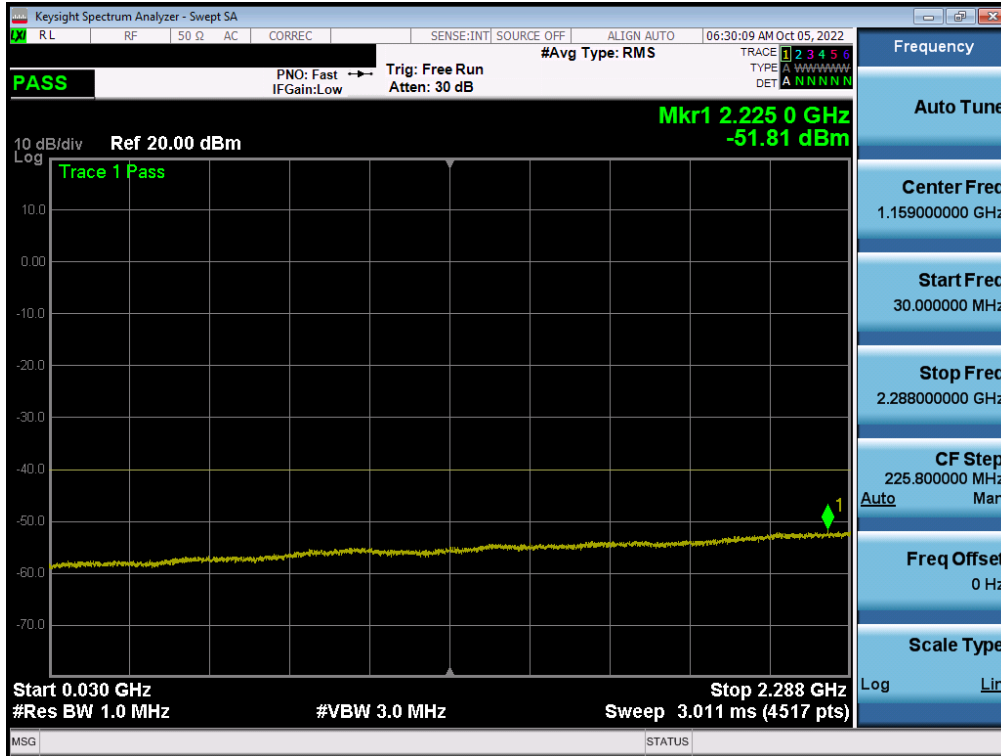
Plot 7-177. Conducted Spurious Plot (LTE Band 30 - 10MHz QPSK - RB Size 1, RB Offset 0 - Ant A)
