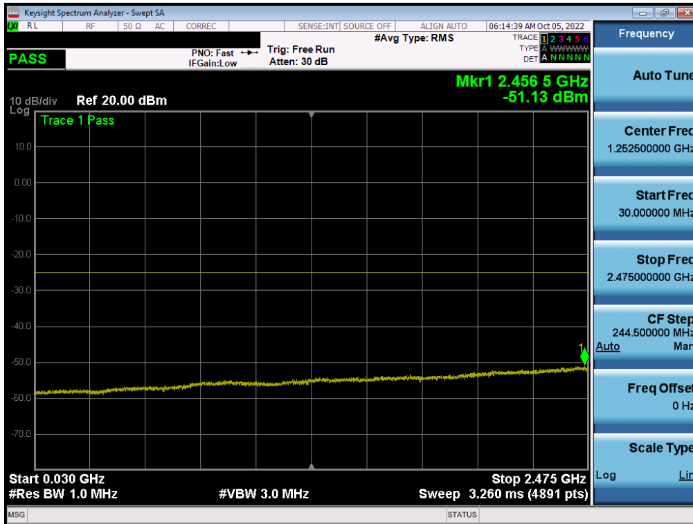
Plot 7-183. Conducted Spurious Plot (LTE Band 7 - 20MHz QPSK - RB Size 1, RB Offset 0 - Low Channel - Ant B)
