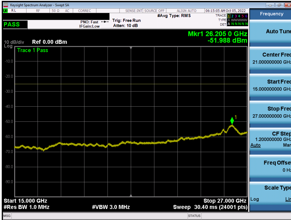
Plot 7-185. Conducted Spurious Plot (LTE Band 7 - 20MHz QPSK - RB Size 1, RB Offset 0 - Low Channel - Ant B)
