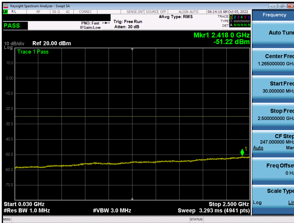
Plot 7-186. Conducted Spurious Plot (LTE Band 7 - 20MHz QPSK - RB Size 1, RB Offset 0 - Mid Channel - Ant B)
