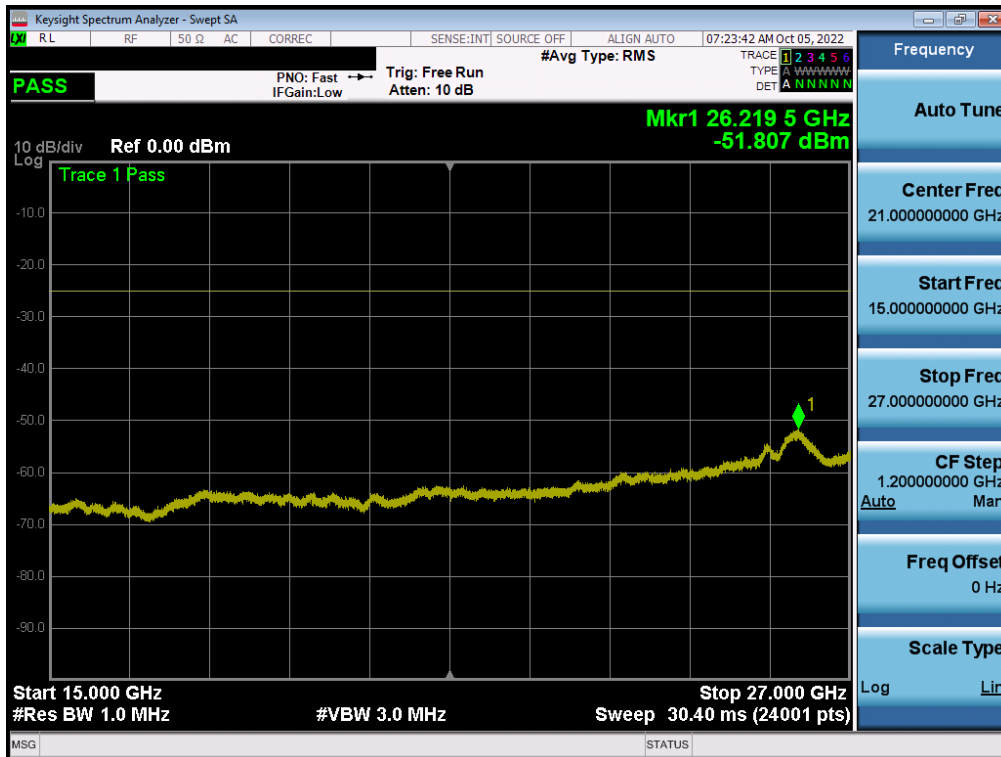
Plot 7-197. Conducted Spurious Plot (LTE Band 7 - 20MHz QPSK - RB Size 1, RB Offset 0 - Mid Channel - Ant F)
