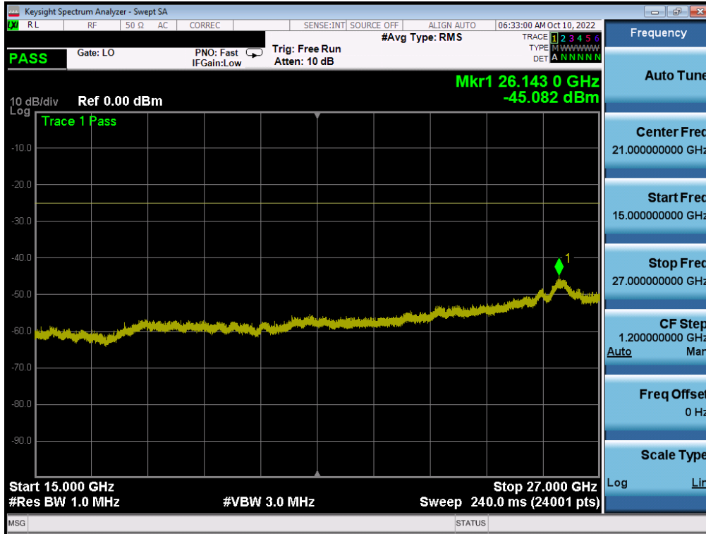
Plot 7-209. Conducted Spurious Plot (LTE Band 41(PC2) - 20MHz QPSK - RB Size 1, RB Offset 0 - High Channel - Ant B)
