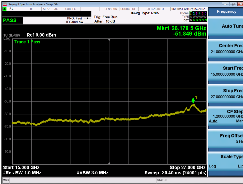
Plot 7-179. Conducted Spurious Plot (LTE Band 30 - 10MHz QPSK - RB Size 1, RB Offset 0 - Ant A)
