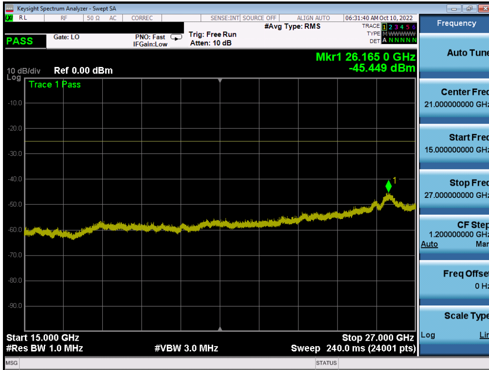
Plot 7-203. Conducted Spurious Plot (LTE Band 41(PC2) - 20MHz QPSK - RB Size 1, RB Offset 0 - Low Channel - Ant B)
