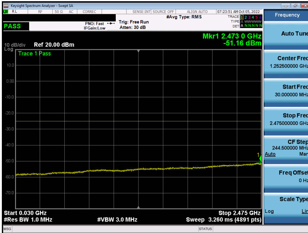
Plot 7-192. Conducted Spurious Plot (LTE Band 7 - 20MHz QPSK - RB Size 1, RB Offset 0 - Low Channel - Ant F)
