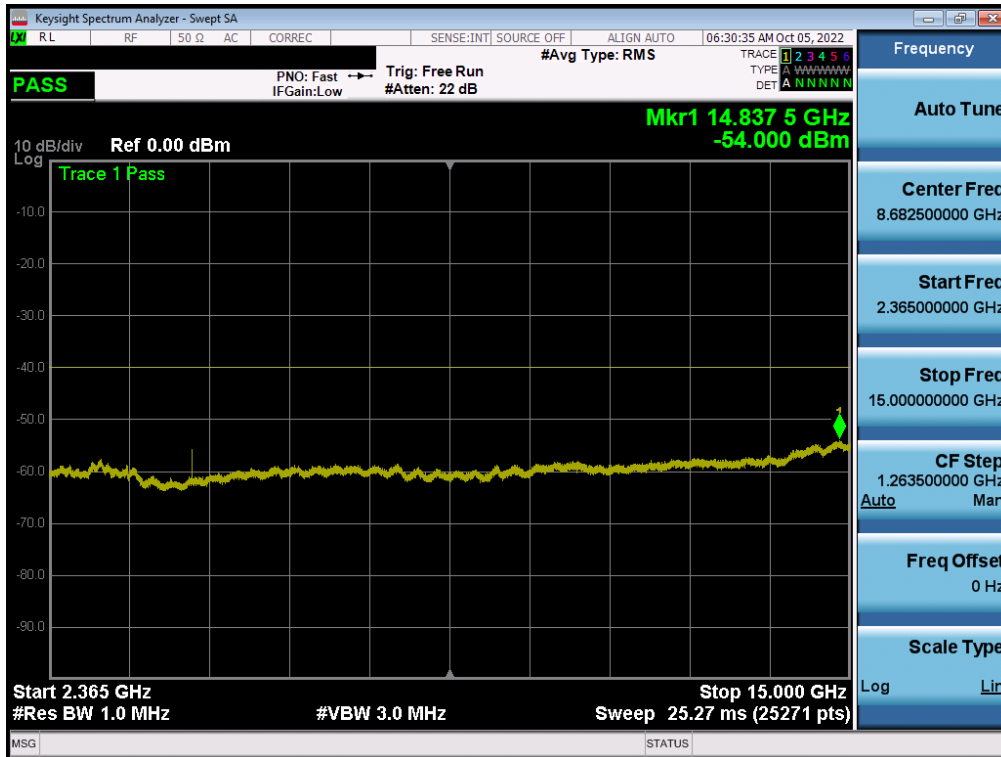
Plot 7-178. Conducted Spurious Plot (LTE Band 30 - 10MHz QPSK - RB Size 1, RB Offset 0 - Ant A)
