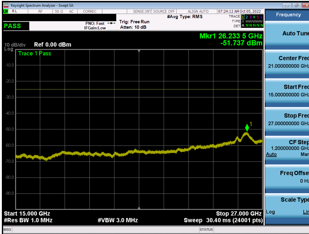
Plot 7-194. Conducted Spurious Plot (LTE Band 7 - 20MHz QPSK - RB Size 1, RB Offset 0 - Low Channel - Ant F)
