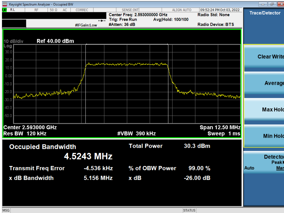
Plot 7-56. Occupied Bandwidth Plot (LTE Band 41(PC3)/38 - 5MHz 16-QAM - Full RB - Ant F)
