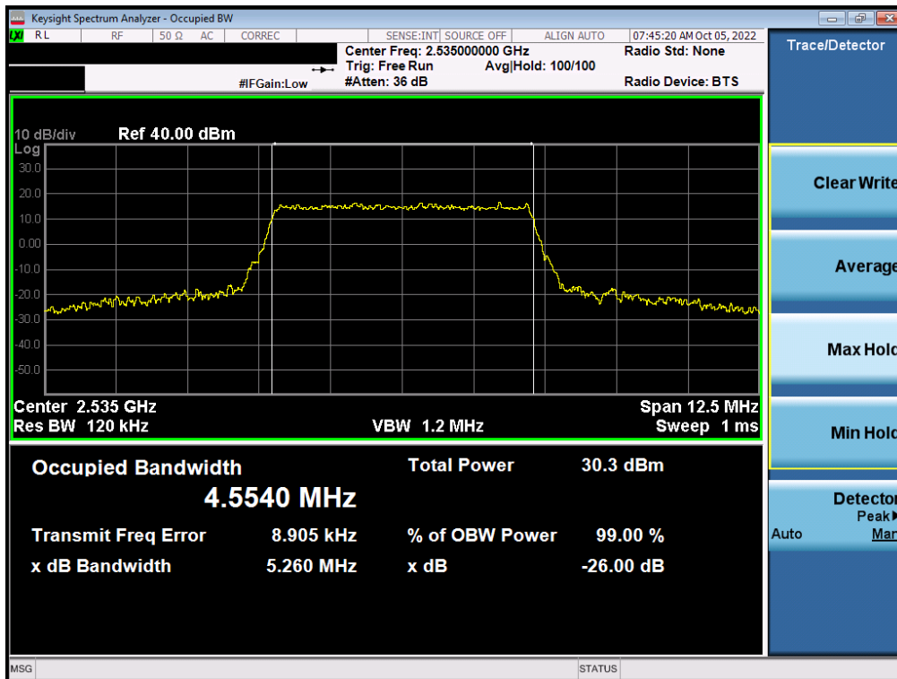
Plot 7-24. Occupied Bandwidth Plot (LTE Band 7 - 5MHz 16-QAM - Full RB - Ant F)
