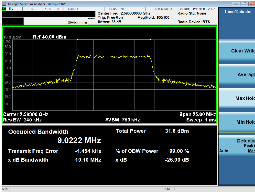
Plot 7-38. Occupied Bandwidth Plot (LTE Band 41(PC2) - 10MHz 16-QAM - Full RB - Ant F)
