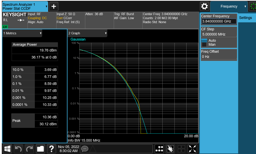
Plot 7-249. PAR Plot (NR Band n77 - C-Band – 15MHz CP-OFDM 256-QAM - Full RB)
