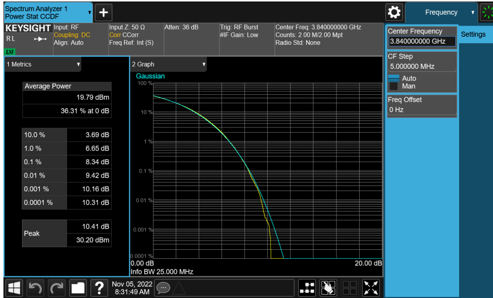
Plot 7-243. PAR Plot (NR Band n77 - C-Band – 25MHz CP-OFDM 256-QAM - Full RB)
