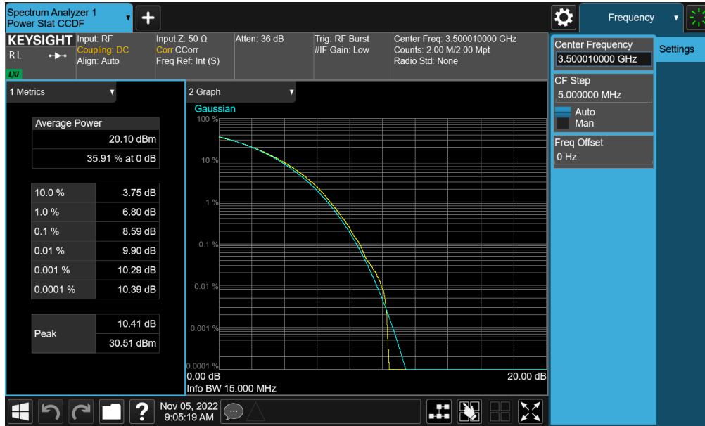
Plot 7-213. PAR Plot (NR Band n77 - DoD Band – 15MHz CP-OFDM 256-QAM - Full RB)
