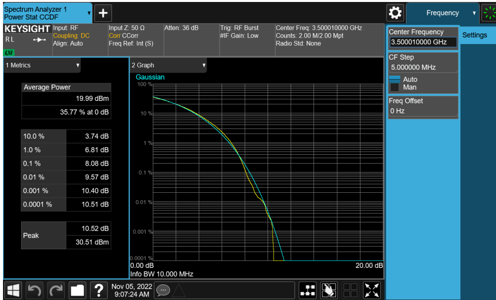
Plot 7-216. PAR Plot (NR Band n77 - DoD Band – 10MHz CP-OFDM 256-QAM - Full RB)
