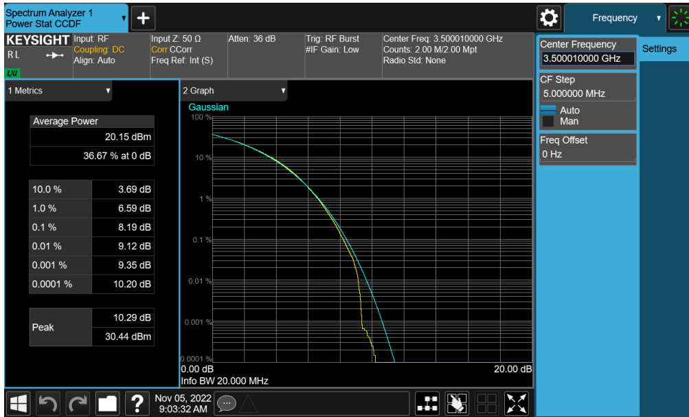
Plot 7-210. PAR Plot (NR Band n77 - DoD Band – 20MHz CP-OFDM 256-QAM - Full RB)
