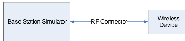
Figure 9-3 Power Measurement Setup
