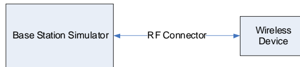
Figure 9-4 Power Measurement Setup – NR FDD
