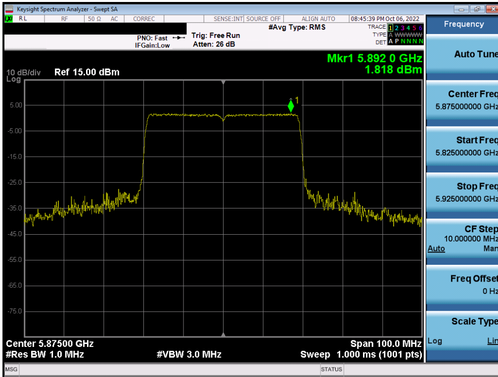
Plot 7-223. Power Spectral Density Plot MIMO ANT1 (40MHz BW 802.11ax – Full Tones (UNII Band 3) – Ch. 175)
