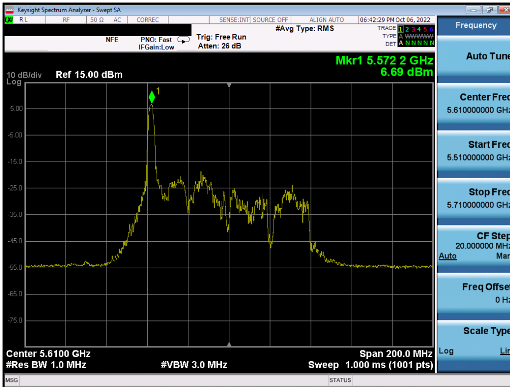
Plot 7-172. Power Spectral Density Plot MIMO ANT1 (80MHz BW 802.11ax – 26 Tones (UNII Band 2C) – Ch. 122)
