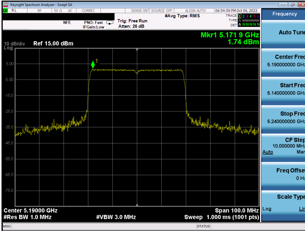
Plot 7-193. Power Spectral Density Plot MIMO ANT1 (40MHz BW 802.11ax – Full Tones (UNII Band 1) – Ch. 38)
