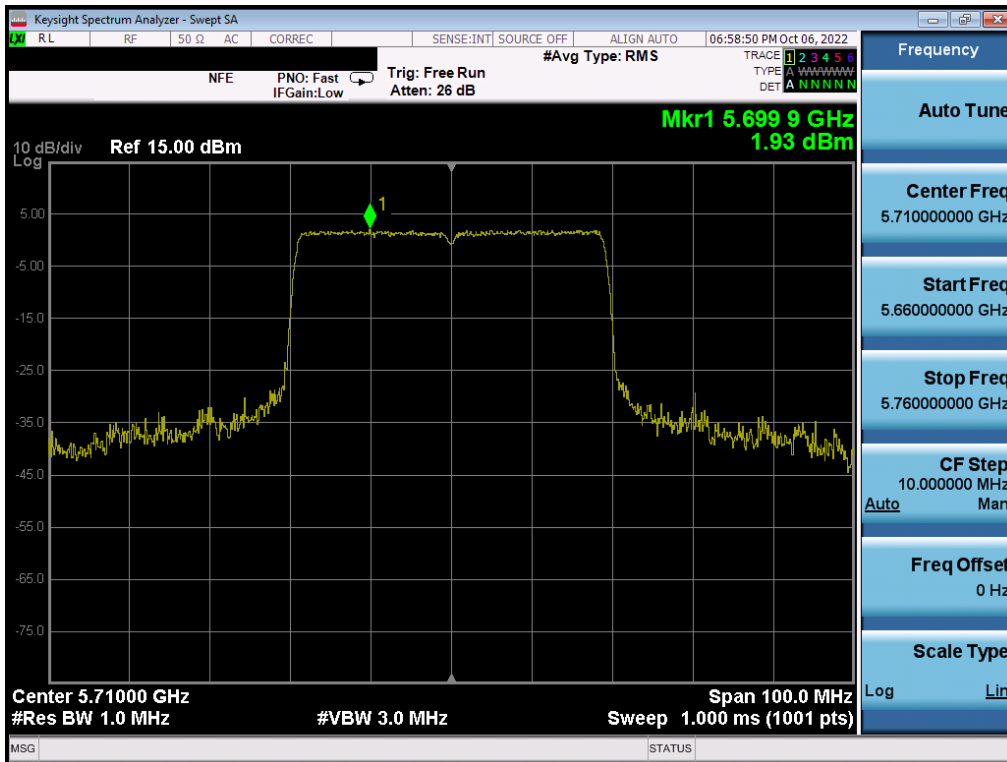
Plot 7-208. Power Spectral Density Plot MIMO ANT1 (40MHz BW 802.11ax – Full Tones (UNII Band 2C) – Ch. 142)
