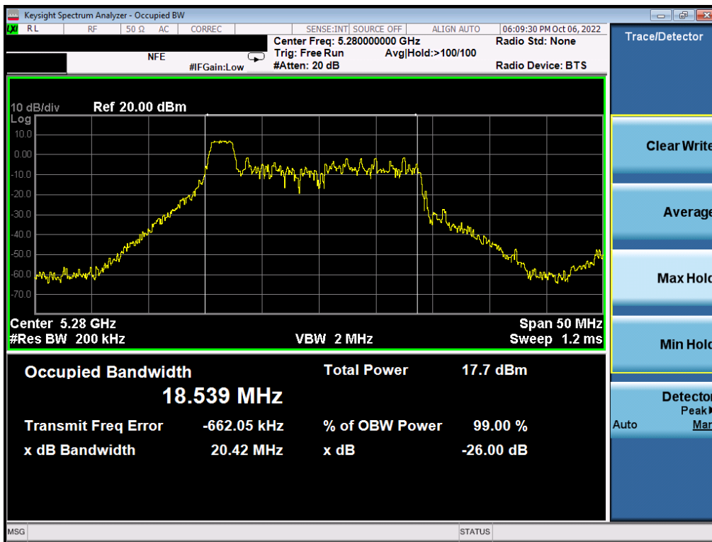
Plot 7-10. 26dB Bandwidth Plot MIMO ANT1 (20MHz BW 802.11ax – 26 Tones (UNII Band 2A) – Ch. 56)
