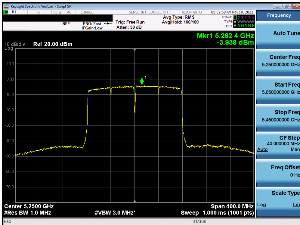
Plot 7-276. Power Spectral Density Plot MIMO ANT2 (160MHz BW 802.11ac (UNII Band 1/2A) – Ch. 50)
