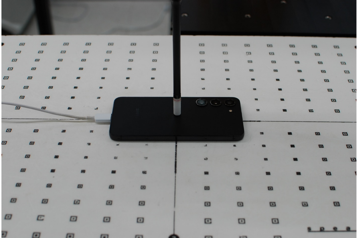
Figure F-14 Near Field Power Density Test Setup Photo – Back Side at 2 mm
