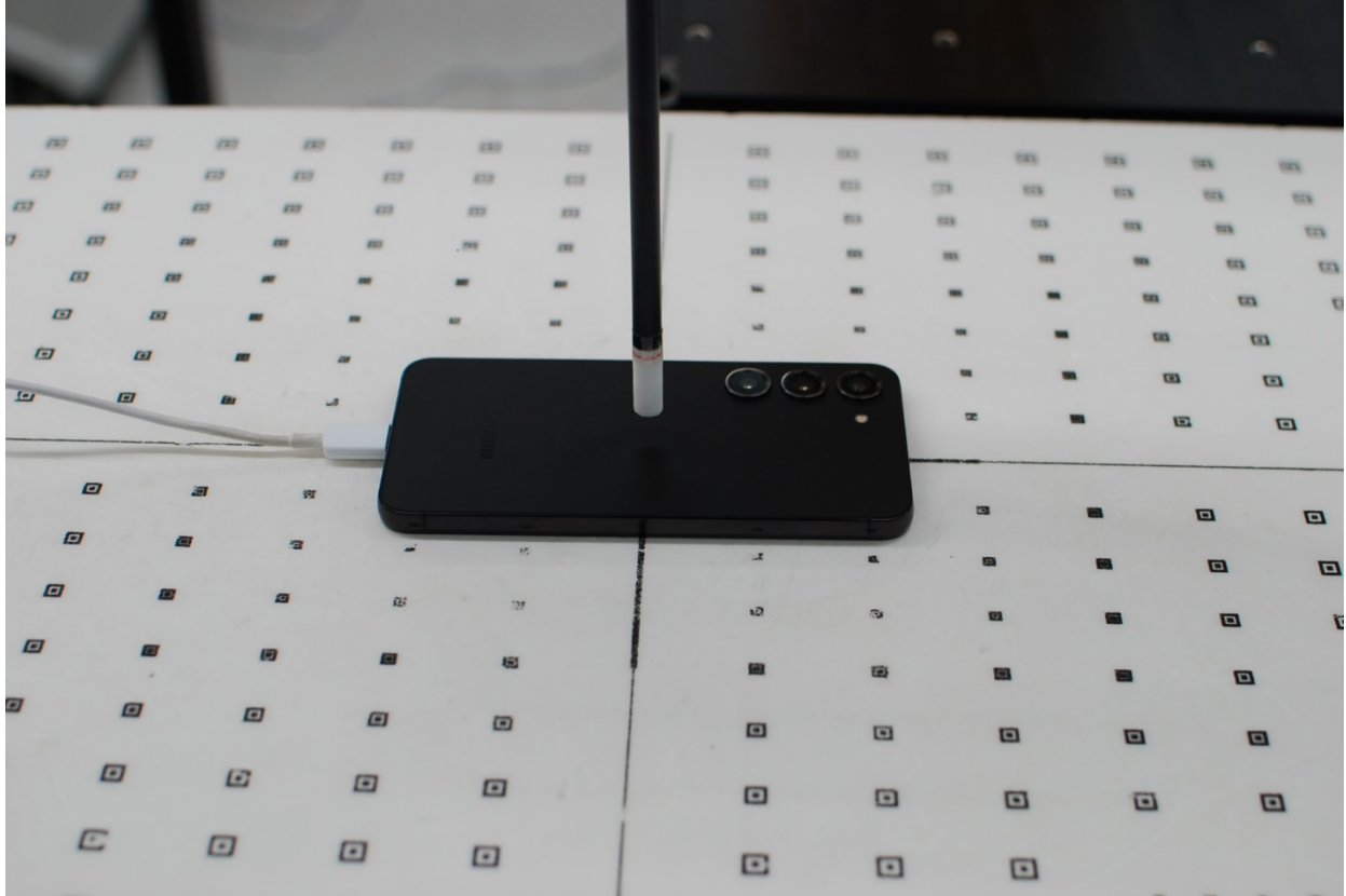
Figure F-15 Near Field Power Density Test Setup Photo – Back Side at 9.51 mm
