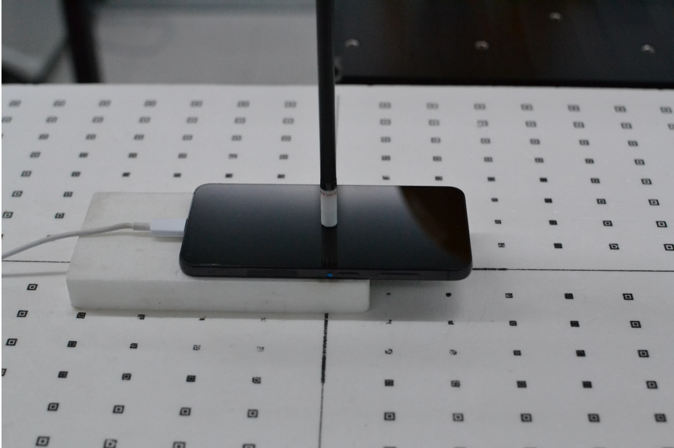
Figure F-16 Near Field Power Density Test Setup Photo – Front Side at 2 mm
