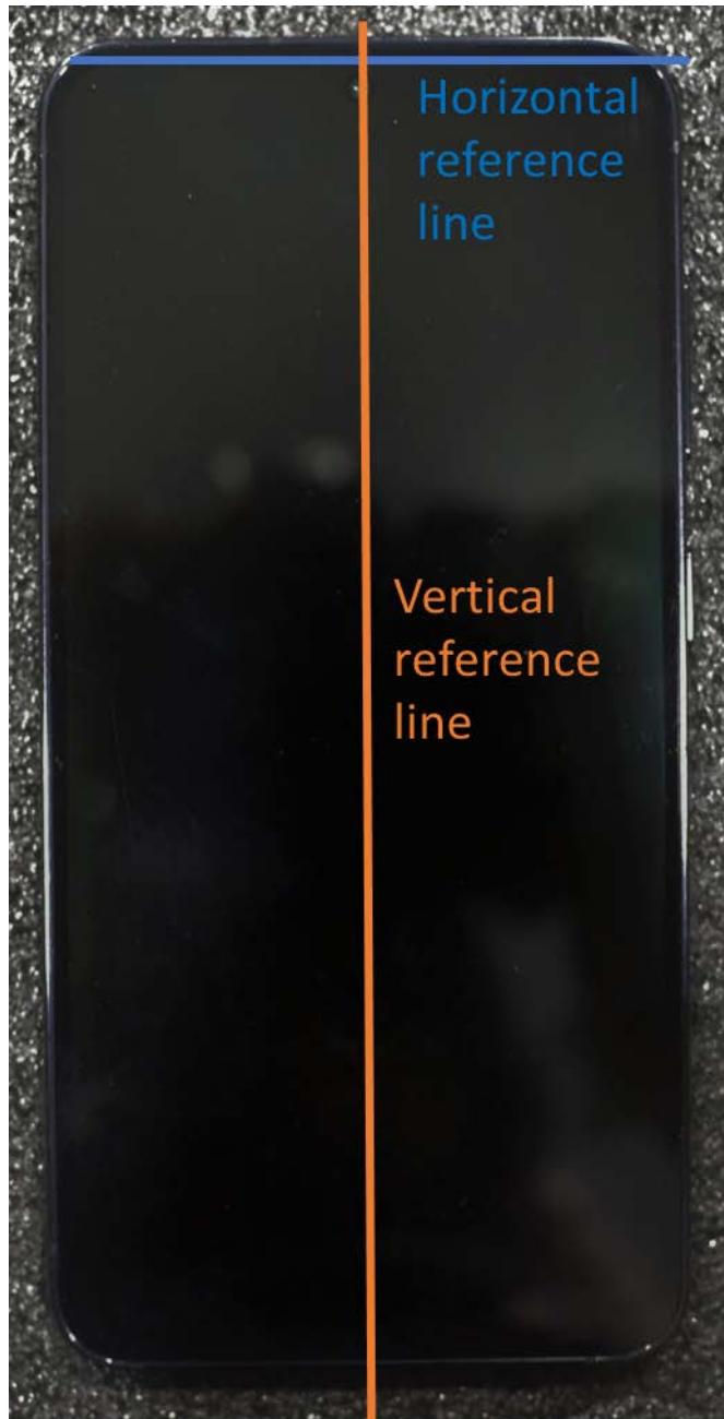
Figure F-13 SAR Test Setup Photo–Horizontal and Vertical Reference Lines
