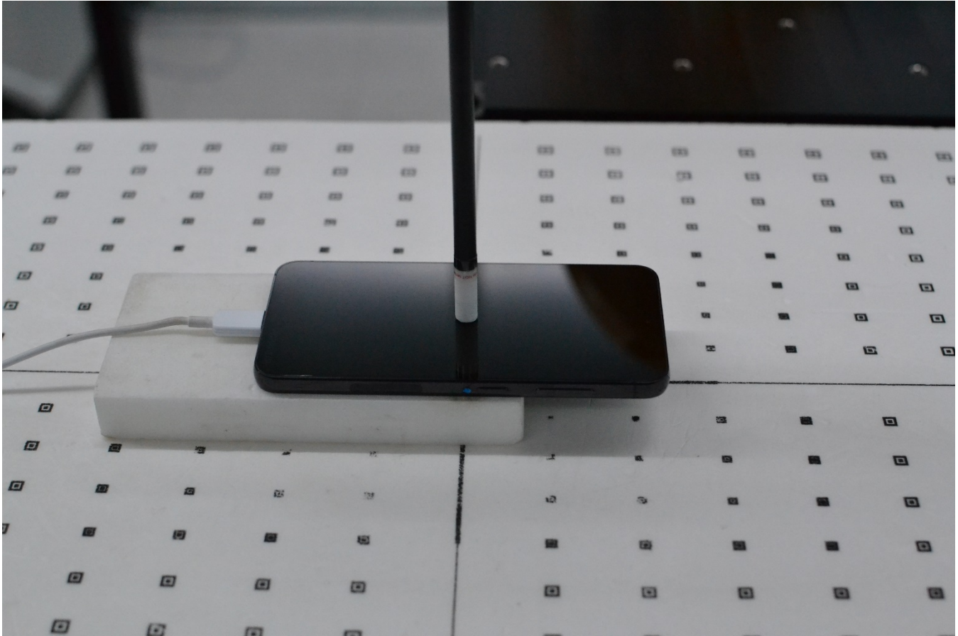
Figure E-6 Near Field Power Density Test Setup Photo – Front Side at 2 mm
