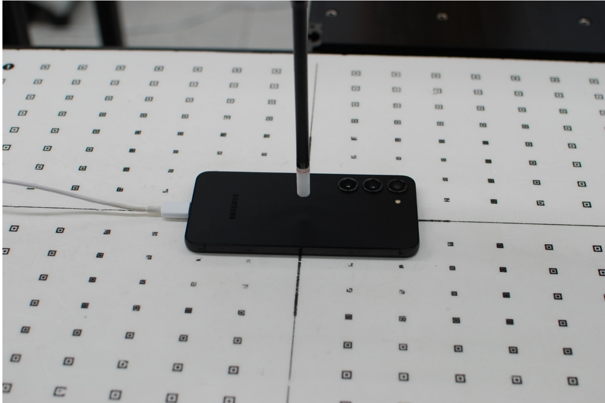
Figure E-5 Near Field Power Density Test Setup Photo – Back Side at 10 mm
