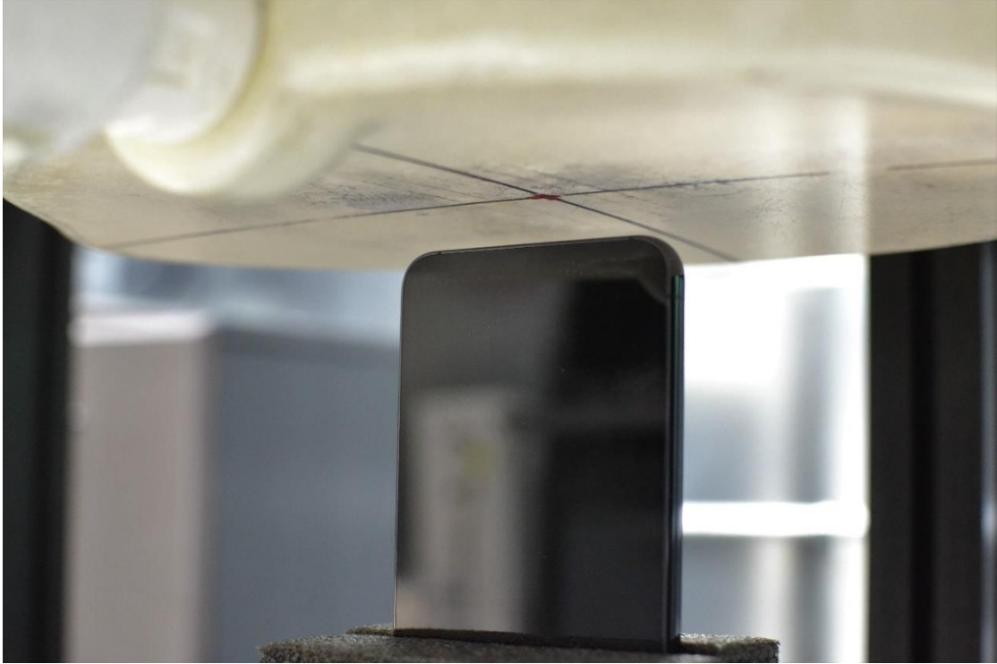
SAR Test Setup Photo 13 – Hotspot, Bottom Edge at 10mm
