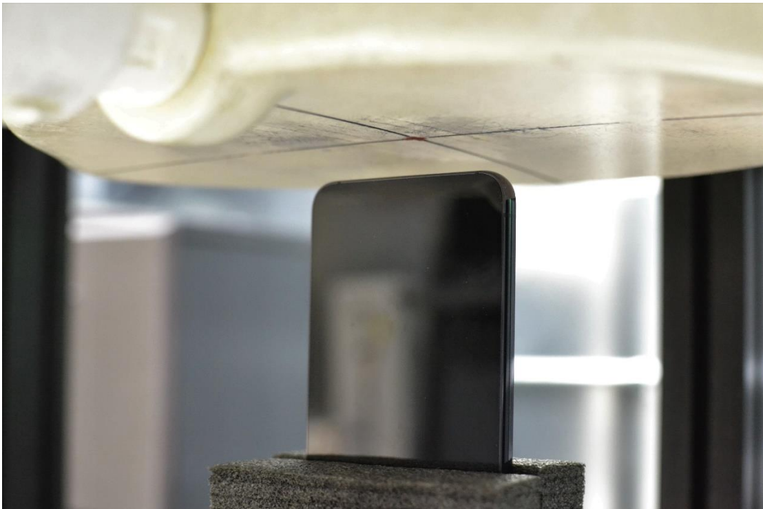
SAR Test Setup Photo 12 – Phablet, Bottom Edge at 11mm
