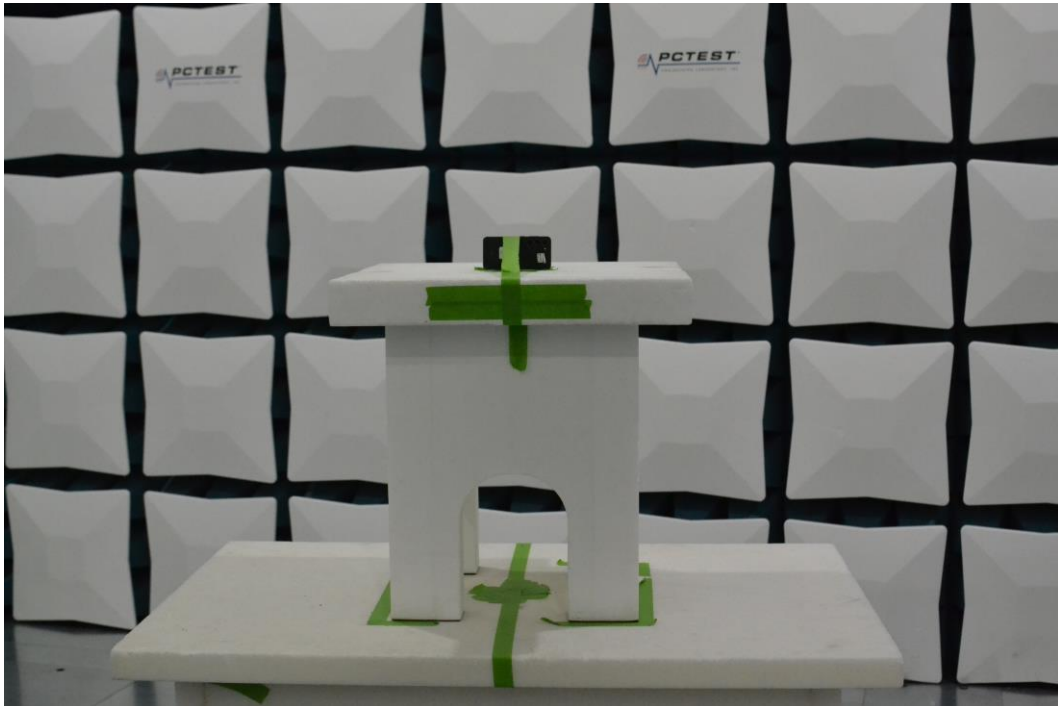
Figure 4. Test Setup – Y Position – 1GHz-18GHz
