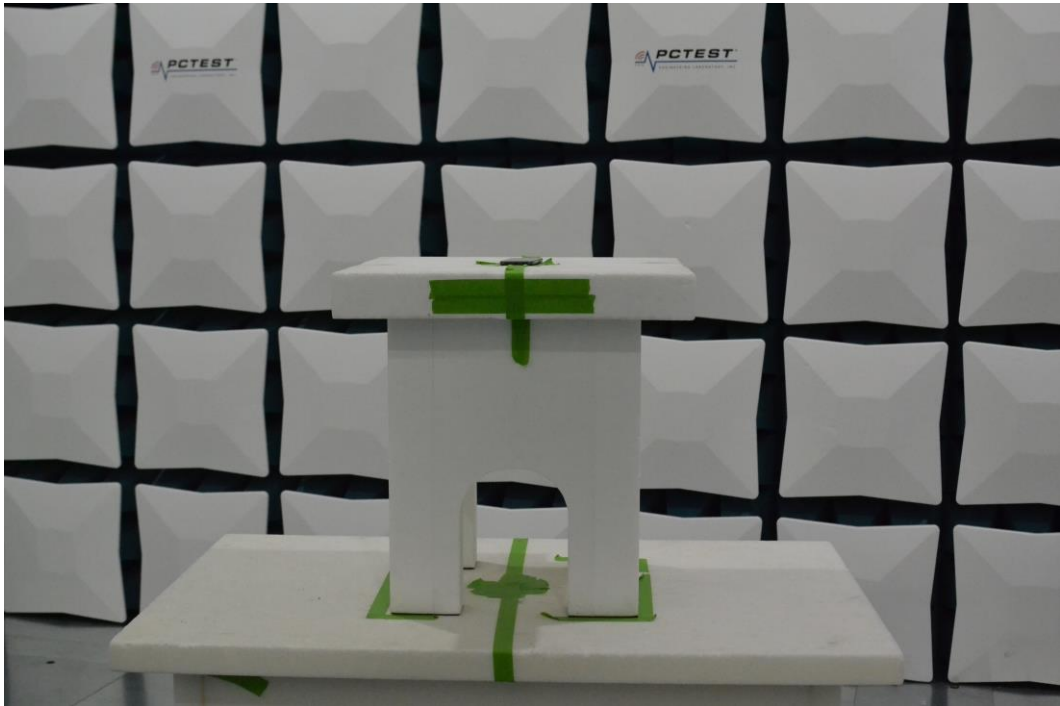
Figure 2. Test Setup – X Position – 1GHz-18GHz
