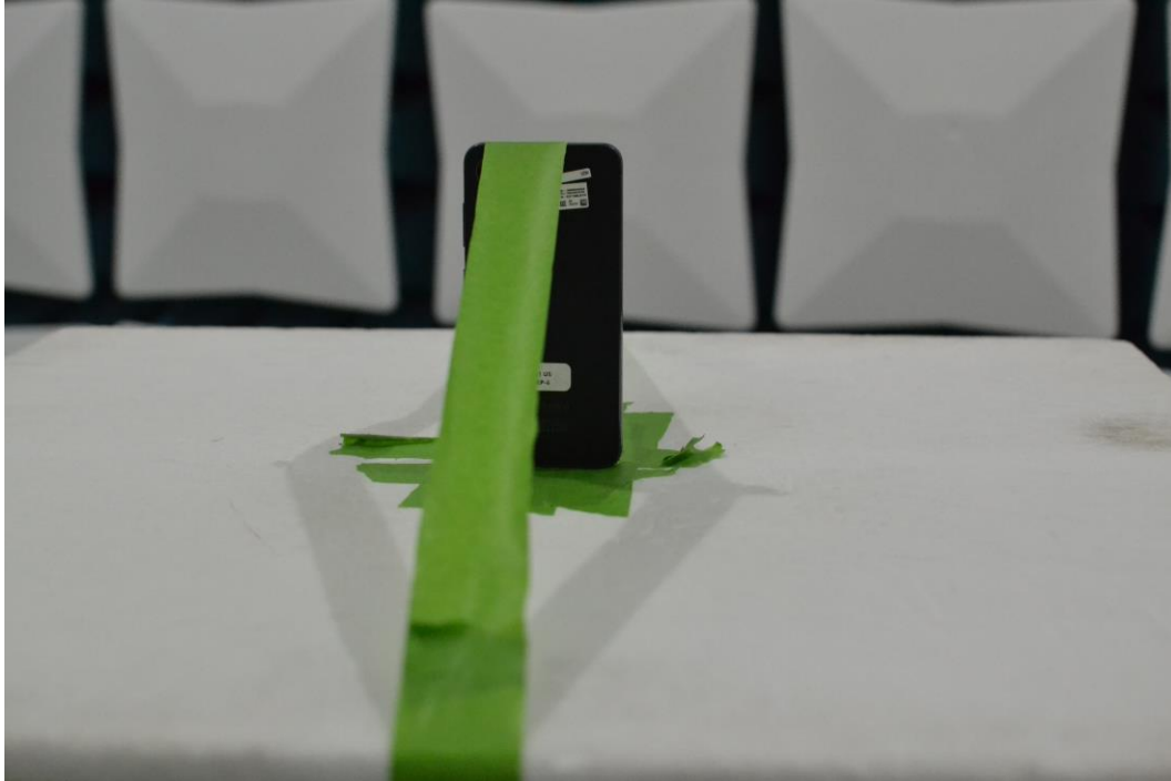
Figure 5. Test Setup – Z Position – 1GHz-18GHz
