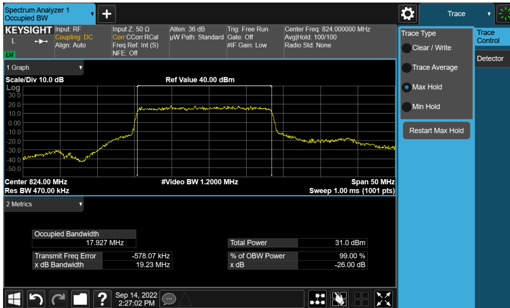
Plot 7-15. Occupied Bandwidth Plot (NR Band n26- 20MHz \pi/2 BPSK - Full RB)
