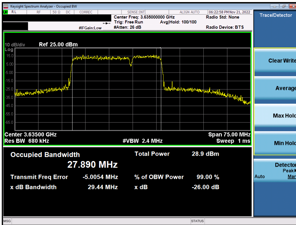
Plot 7-14. Occupied Bandwidth Plot (ULCA LB48 - 20+10MHz 16-QAM - Full RB Configuration)
