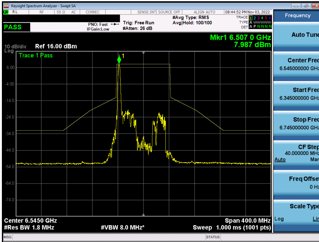
Plot 7-583. In-Band Emission Plot MIMO ANT2 (80MHz BW 802.11ax (26 Tones) (UNII Band 7) – Ch. 119) – SP
