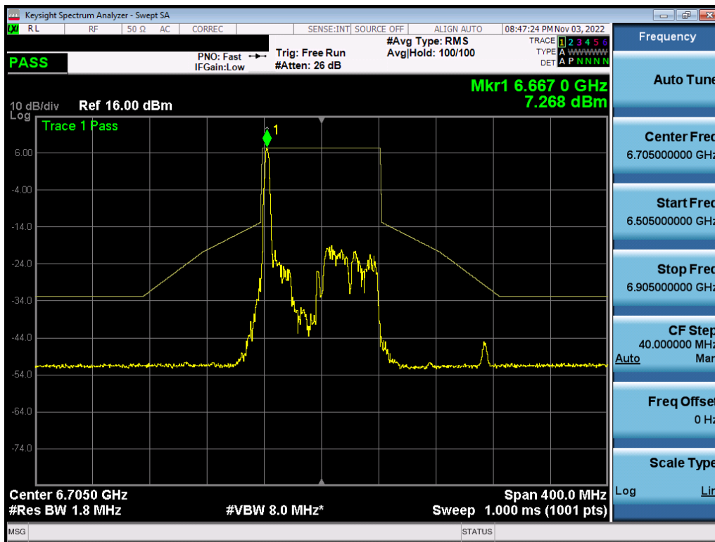
Plot 7-584. In-Band Emission Plot MIMO ANT2 (80MHz BW 802.11ax (26 Tones) (UNII Band 7) – Ch. 151) – SP
