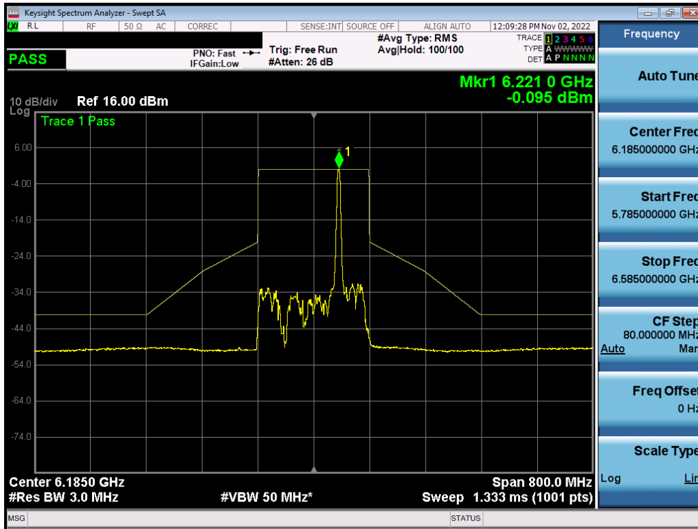
Plot 7-535. In-Band Emission Plot MIMO ANT2 (160MHz BW 802.11ax (26 Tones) (UNII Band 5) – Ch. 47) – LPI
