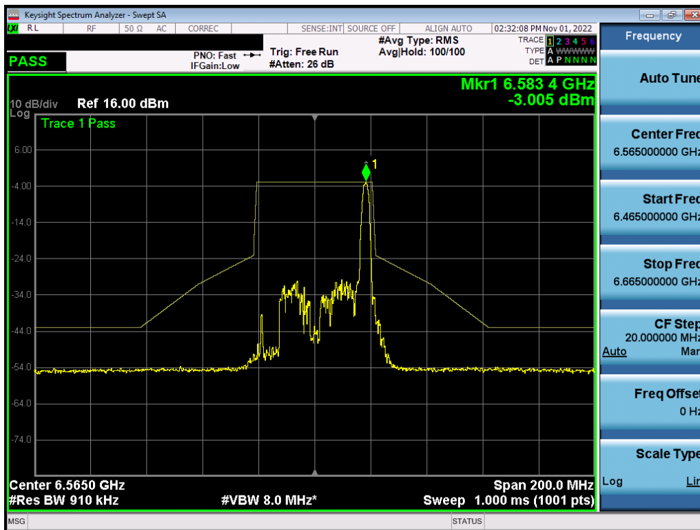
Plot 7-548. In-Band Emission Plot MIMO ANT2 (40MHz BW 802.11ax (26 Tones) (UNII Band 7) – Ch. 123) – LPI
