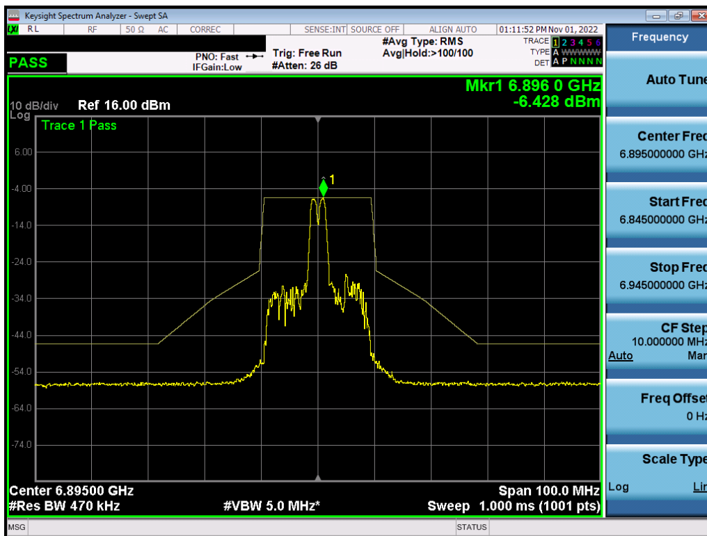
Plot 7-556. In-Band Emission Plot MIMO ANT2 (20MHz BW 802.11ax (26 Tones) (UNII Band 8) – Ch. 189) – LPI
