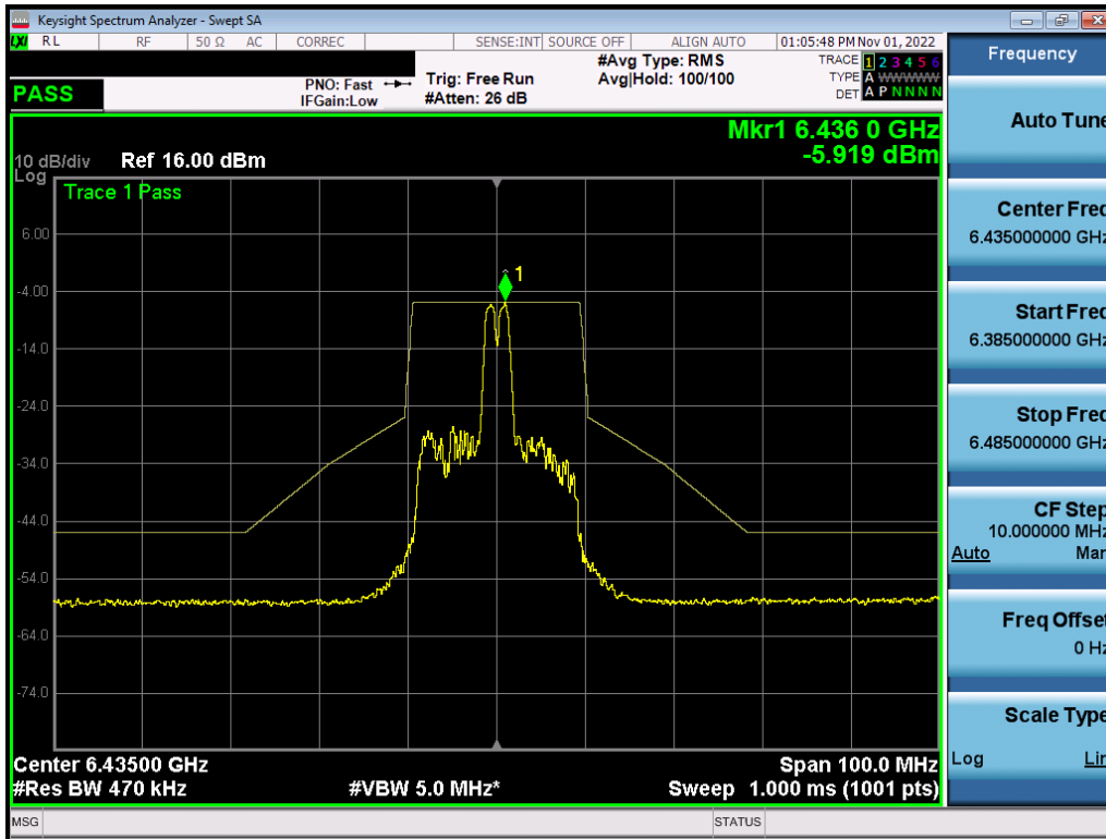
Plot 7-537. In-Band Emission Plot MIMO ANT2 (20MHz BW 802.11ax (26 Tones) (UNII Band 6) – Ch. 97) – LPI
