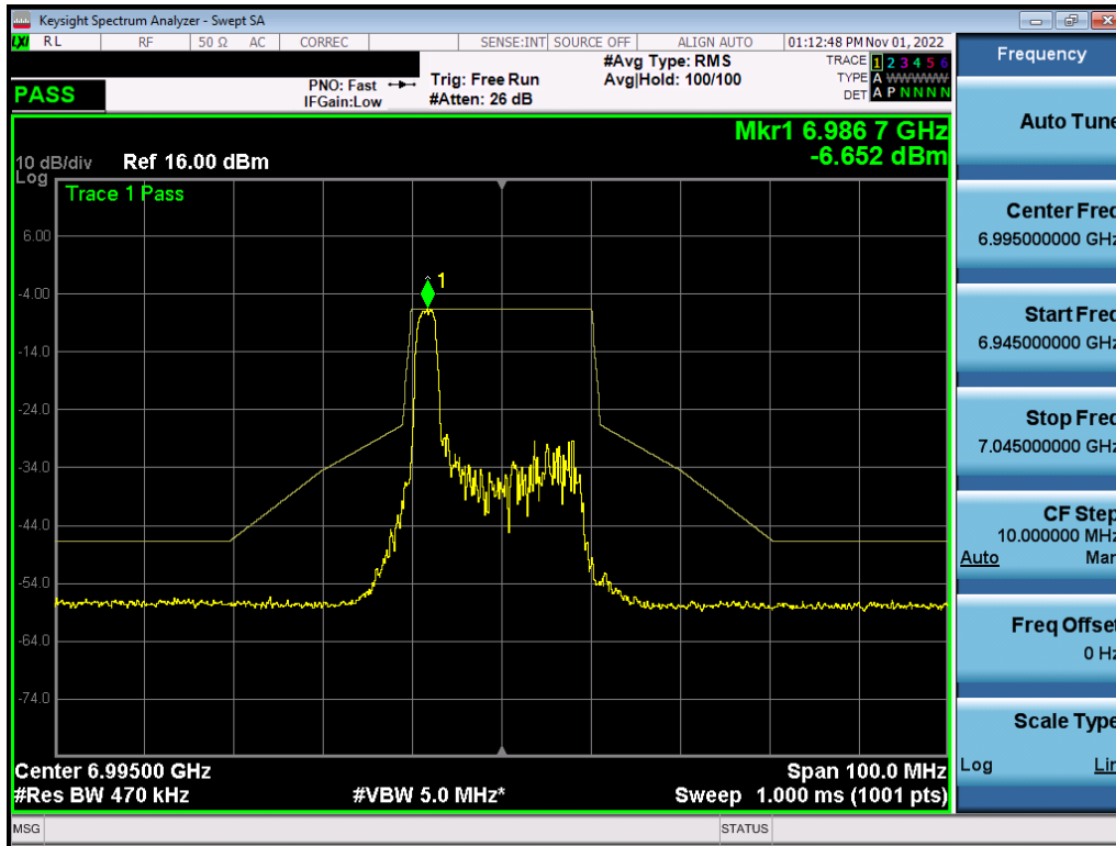
Plot 7-557. In-Band Emission Plot MIMO ANT2 (20MHz BW 802.11ax (26 Tones) (UNII Band 8) – Ch. 209) – LPI
