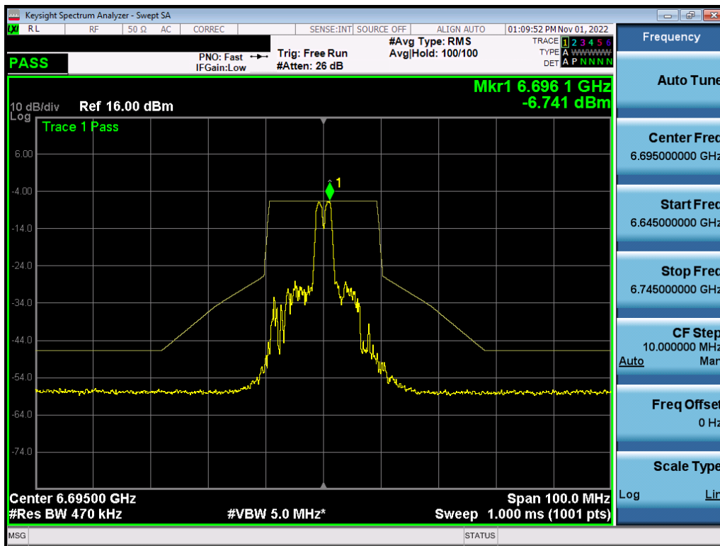
Plot 7-546. In-Band Emission Plot MIMO ANT2 (20MHz BW 802.11ax (26 Tones) (UNII Band 7) – Ch. 149) – LPI
