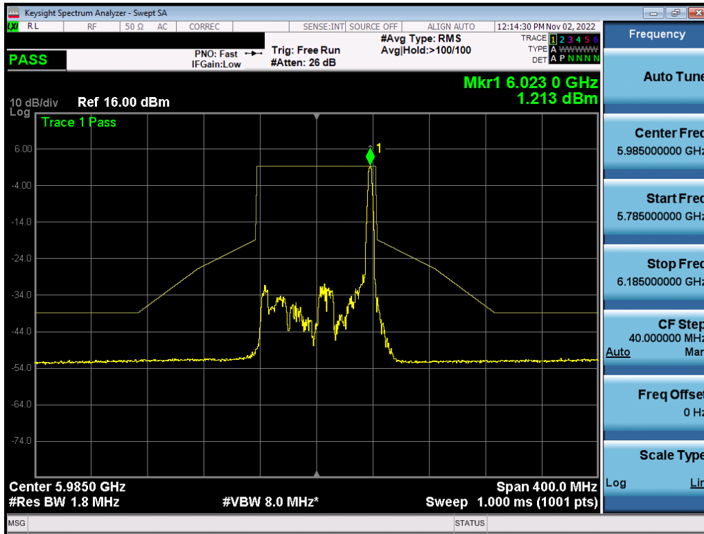
Plot 7-531. In-Band Emission Plot MIMO ANT2 (80MHz BW 802.11ax (26 Tones) (UNII Band 5) – Ch. 7) – LPI
