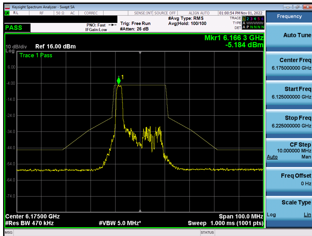
Plot 7-526. In-Band Emission Plot MIMO ANT2 (20MHz BW 802.11ax (26 Tones) (UNII Band 5) – Ch. 45) – LPI
