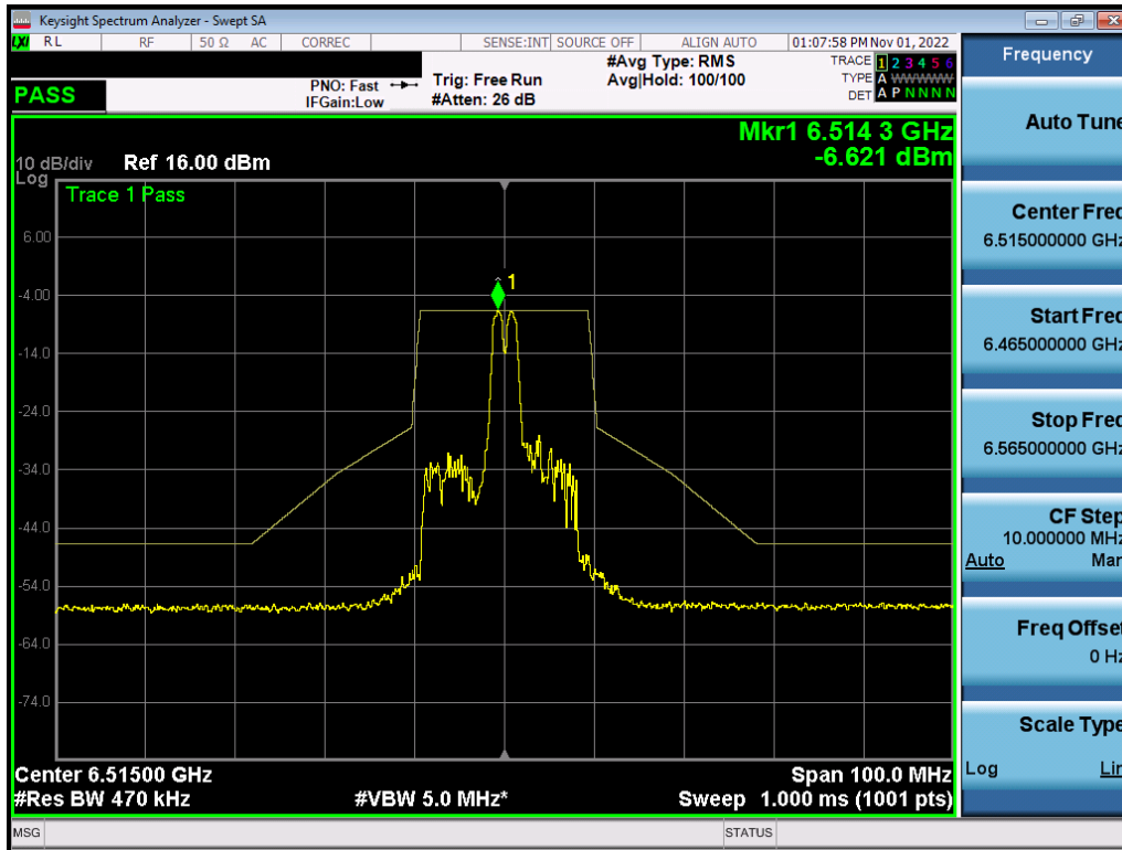
Plot 7-539. In-Band Emission Plot MIMO ANT2 (20MHz BW 802.11ax (26 Tones) (UNII Band 6) – Ch. 113) – LPI
