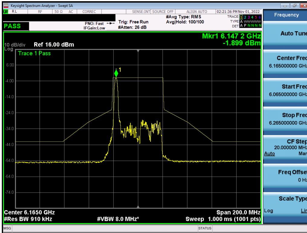
Plot 7-529. In-Band Emission Plot MIMO ANT2 (40MHz BW 802.11ax (26 Tones) (UNII Band 5) – Ch. 43) – LPI
