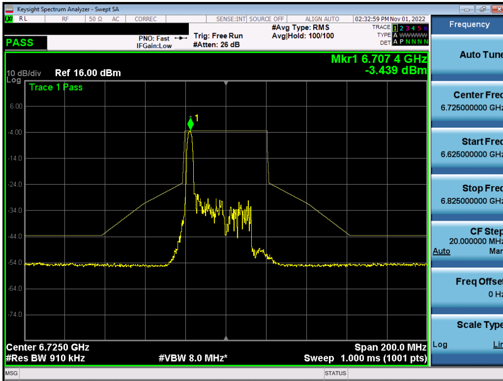
Plot 7-549. In-Band Emission Plot MIMO ANT2 (40MHz BW 802.11ax (26 Tones) (UNII Band 7) – Ch. 155) – LPI
