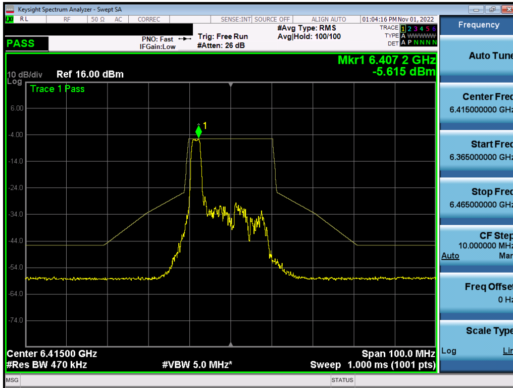
Plot 7-527. In-Band Emission Plot MIMO ANT2 (20MHz BW 802.11ax (26 Tones) UNII Band 5) – Ch. 93) – LPI
