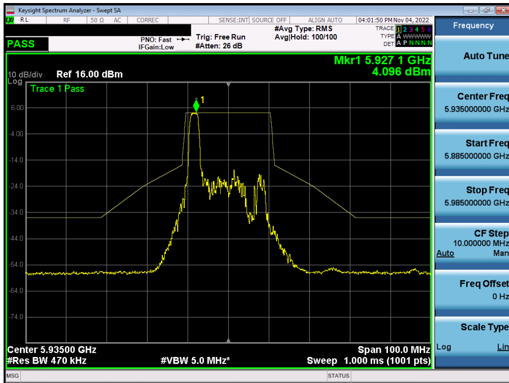
Plot 7-459. In-Band Emission Plot MIMO ANT1 (20MHz BW 802.11ax (26 Tones) UNII Band 5) – Ch. 2 - SP
