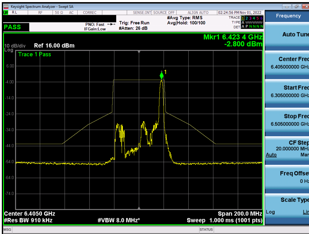
Plot 7-530. In-Band Emission Plot MIMO ANT2 (40MHz BW 802.11ax (26 Tones) (UNII Band 5) – Ch. 91) – LPI
