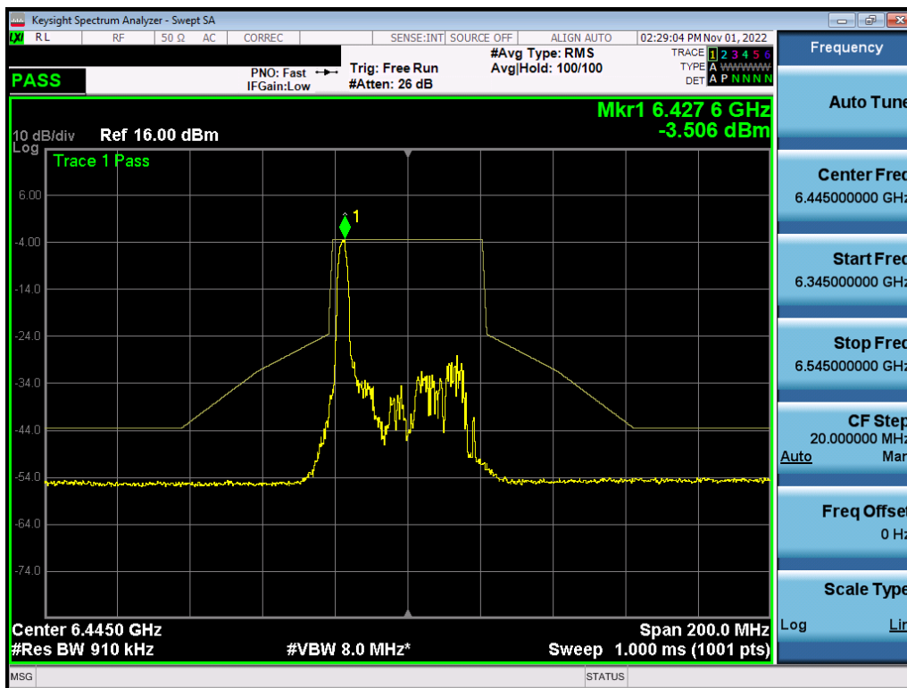
Plot 7-540. In-Band Emission Plot MIMO ANT2 (40MHz BW 802.11ax (26 Tones) (UNII Band 6) – Ch. 99) – LPI
