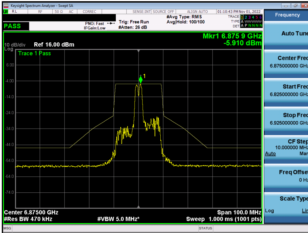
Plot 7-547. In-Band Emission Plot MIMO ANT2 (20MHz BW 802.11ax (26 Tones) (UNII Band 7) – Ch. 185) – LPI
