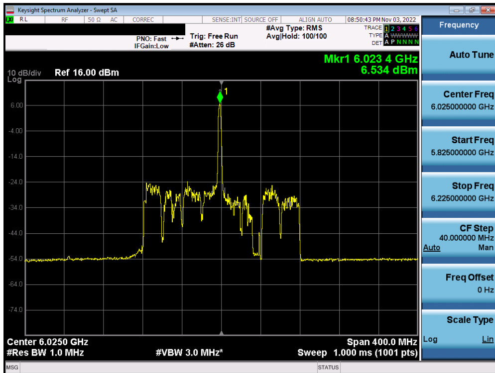
Plot 7-362. Power Spectral Density Plot MIMO ANT2 (160MHz BW 802.11ax (26 Tones) (UNII Band 5) – Ch. 15) – SP
