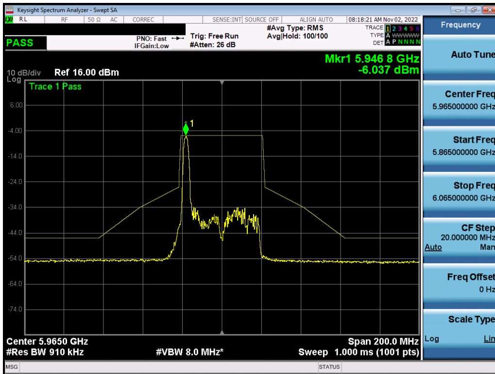
Plot 7-422. In-Band Emission Plot MIMO ANT1 (40MHz BW 802.11ax (26 Tones) (UNII Band 5) – Ch. 3) – LPI
