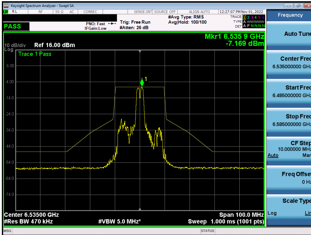
Plot 7-439. In-Band Emission Plot MIMO ANT1 (20MHz BW 802.11ax (26 Tones) (UNII Band 7) – Ch. 117) – LPI
