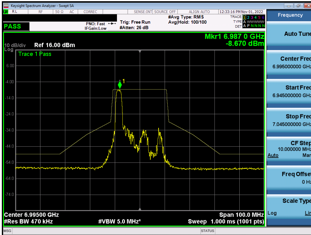
Plot 7-451. In-Band Emission Plot MIMO ANT1 (20MHz BW 802.11ax (26 Tones) (UNII Band 8) – Ch. 209) – LPI
