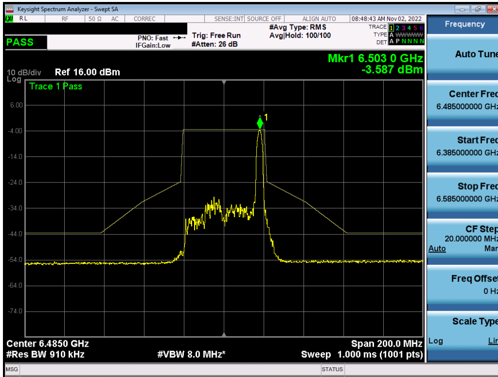
Plot 7-435. In-Band Emission Plot MIMO ANT1 (40MHz BW 802.11ax (26 Tones) (UNII Band 6) – Ch. 107) – LPI
