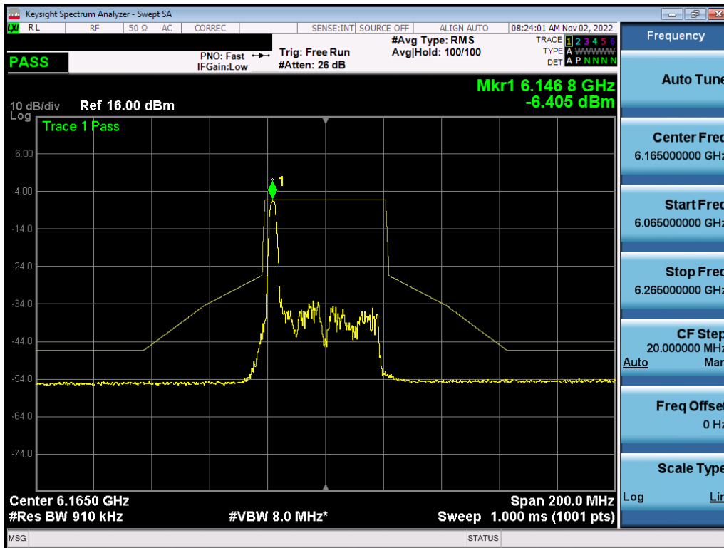
Plot 7-423. In-Band Emission Plot MIMO ANT1 (40MHz BW 802.11ax (26 Tones) (UNII Band 5) – Ch. 43) – LPI
