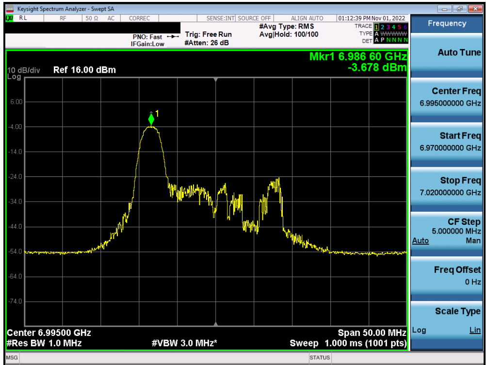
Plot 7-345. Power Spectral Density Plot MIMO ANT2 (20MHz BW 802.11ax (26 Tones) (UNII Band 8) – Ch. 209) – LPI
