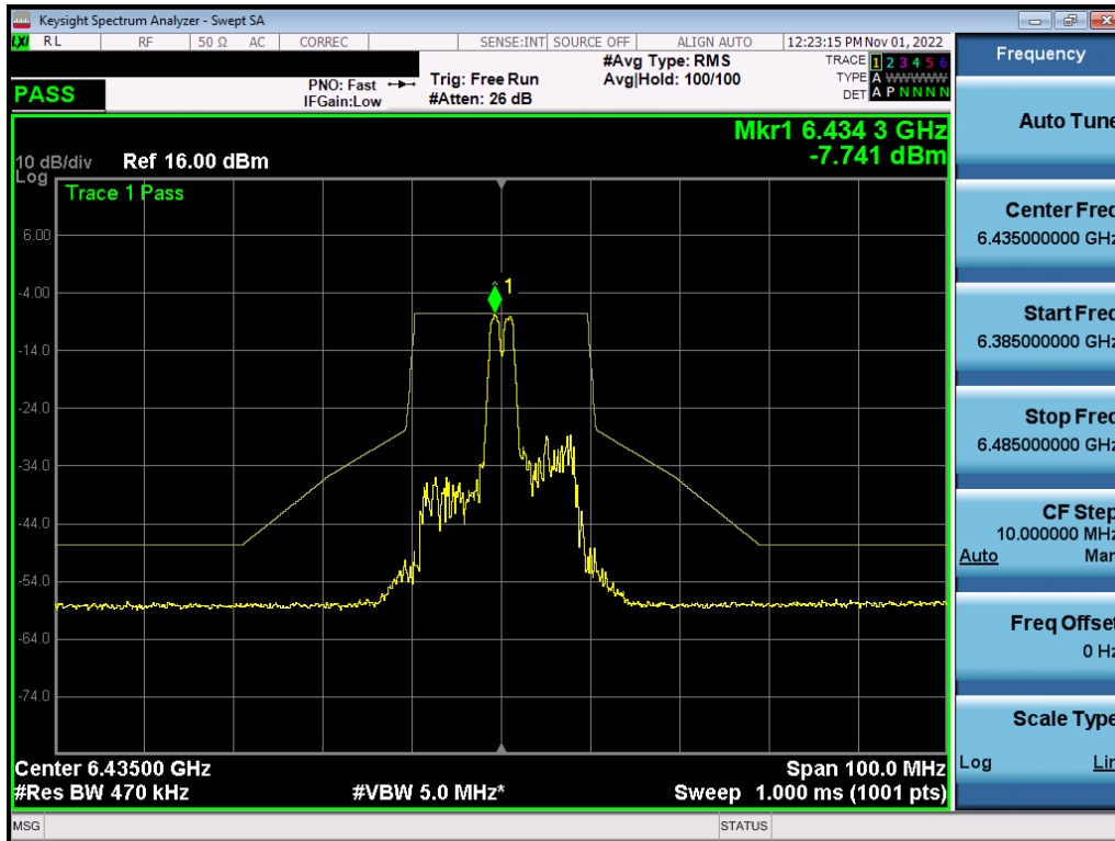
Plot 7-431. In-Band Emission Plot MIMO ANT1 (20MHz BW 802.11ax (26 Tones) (UNII Band 6) – Ch. 97) – LPI
