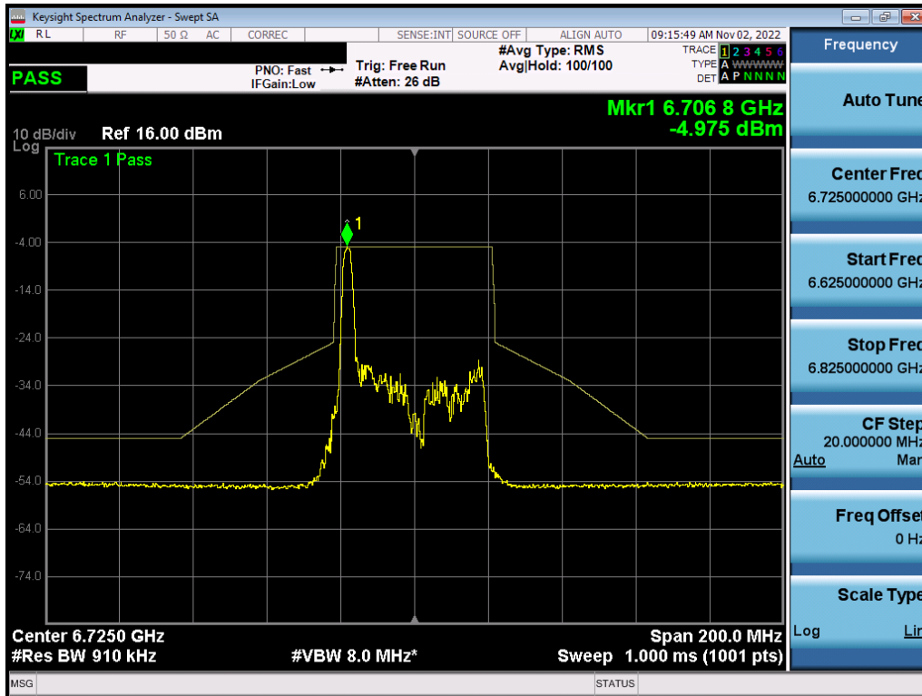
Plot 7-443. In-Band Emission Plot MIMO ANT1 (40MHz BW 802.11ax (26 Tones) (UNII Band 7) – Ch. 155) – LPI
