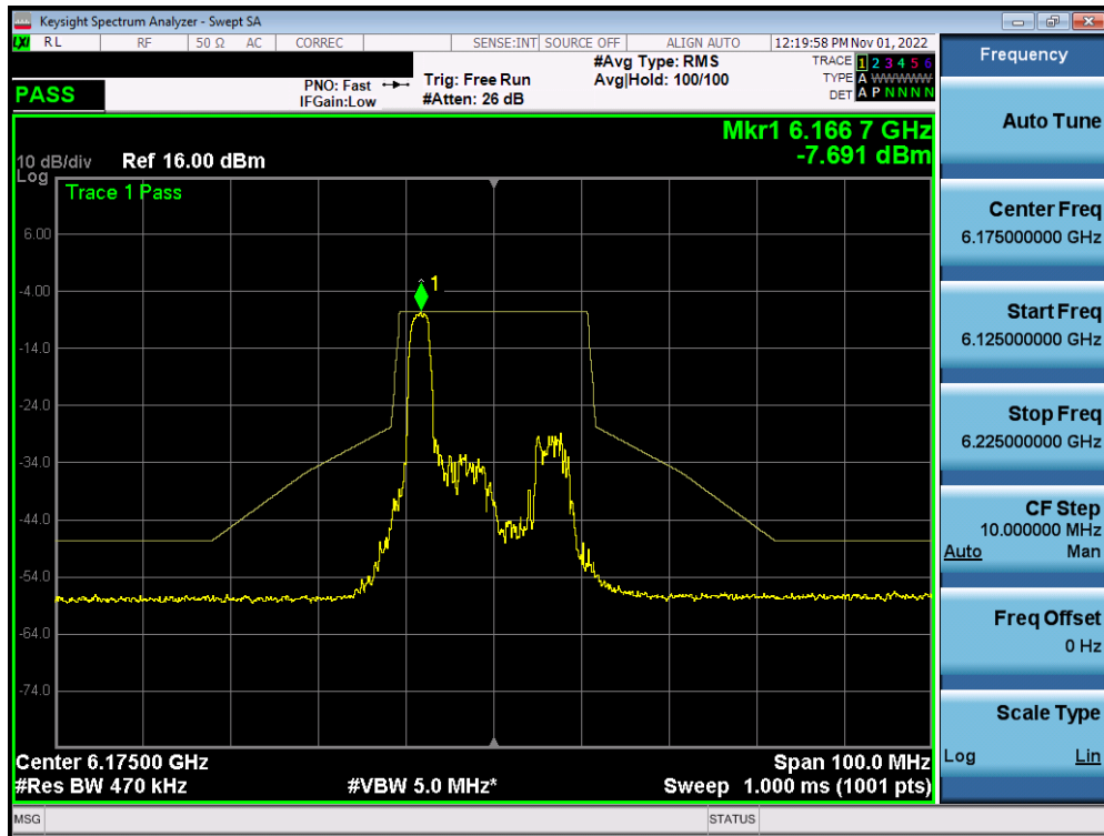
Plot 7-420. In-Band Emission Plot MIMO ANT1 (20MHz BW 802.11ax (26 Tones) (UNII Band 5) – Ch. 45) – LPI
