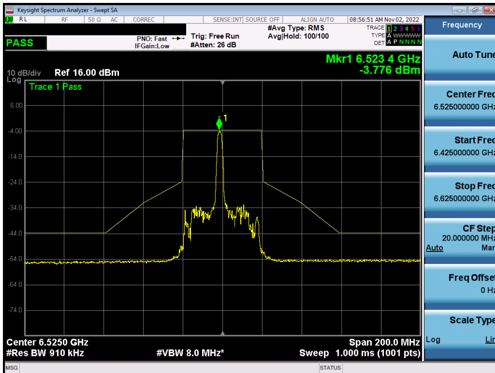
Plot 7-436. In-Band Emission Plot MIMO ANT1 (40MHz BW 802.11ax (26 Tones) (UNII Band 6) – Ch. 115) – LPI
