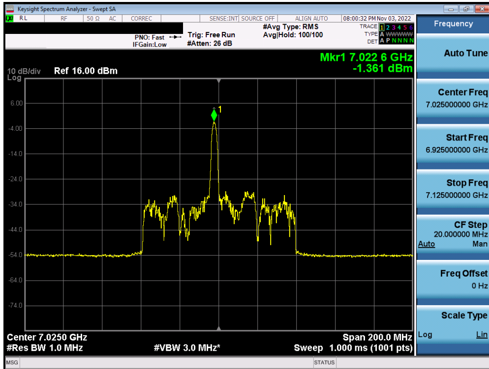
Plot 7-351. Power Spectral Density Plot MIMO ANT2 (80MHz BW 802.11ax (26 Tones) (UNII Band 8) – Ch. 215) – LPI
