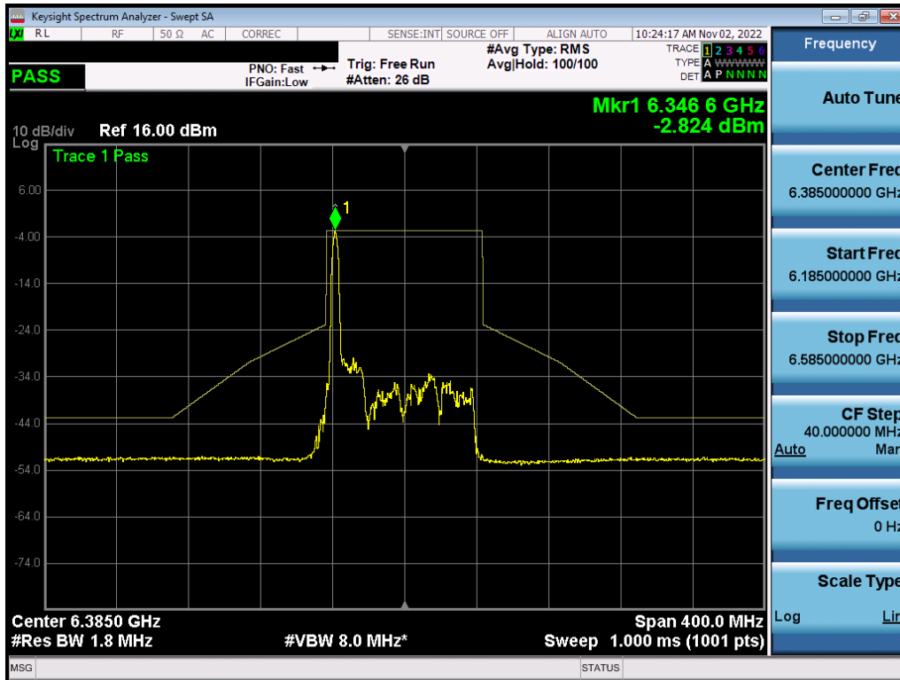
Plot 7-427. In-Band Emission Plot MIMO ANT1 (80MHz BW 802.11ax (26 Tones) (UNII Band 5) – Ch. 87) – LPI
