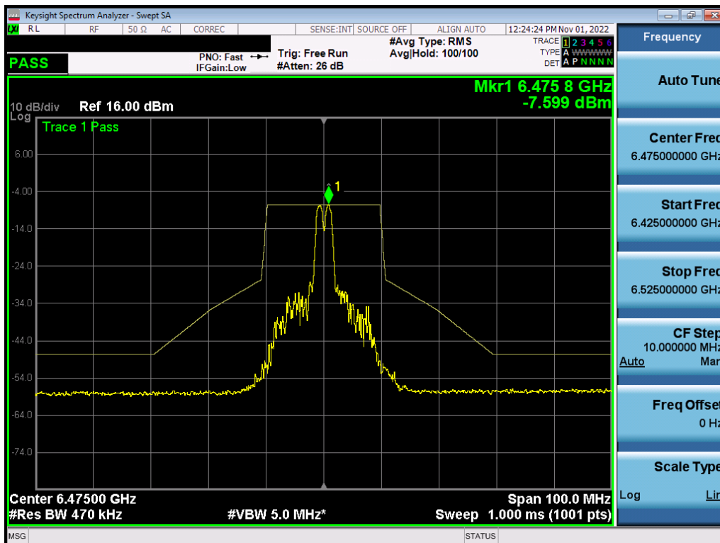
Plot 7-432. In-Band Emission Plot MIMO ANT1 (20MHz BW 802.11ax (26 Tones) (UNII Band 6) – Ch. 105) – LPI
