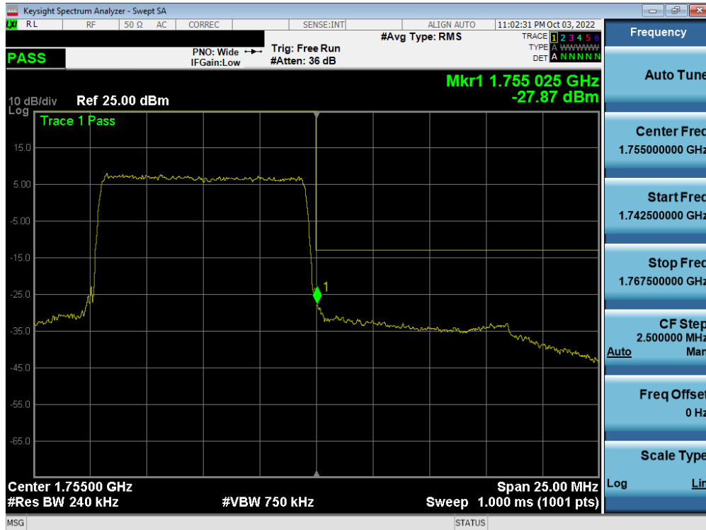
Plot 7-341. Upper Band Edge Plot (LTE Band 4 - 10MHz QPSK – Full RB - Ant F)
