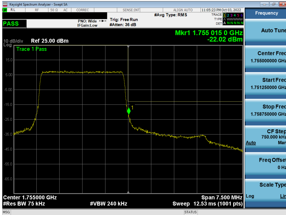
Plot 7-353. Upper Band Edge Plot (LTE Band 4 - 3MHz QPSK – Full RB - Ant F)
