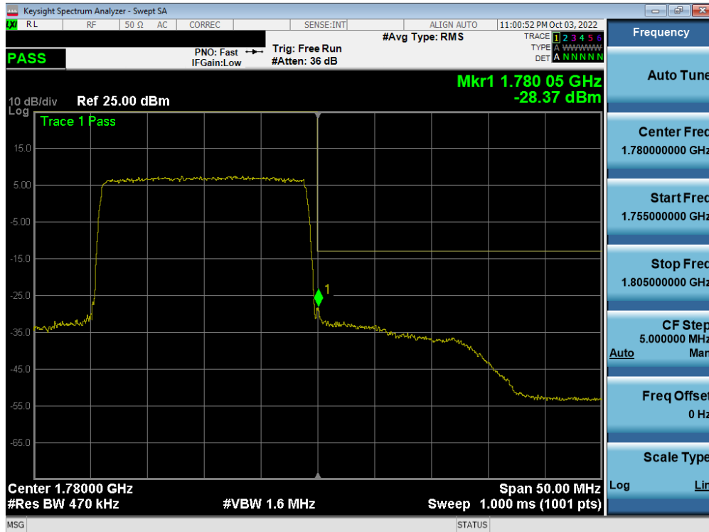
Plot 7-331. Upper Band Edge Plot (LTE Band 66 - 20MHz QPSK – Full RB - Ant F)
