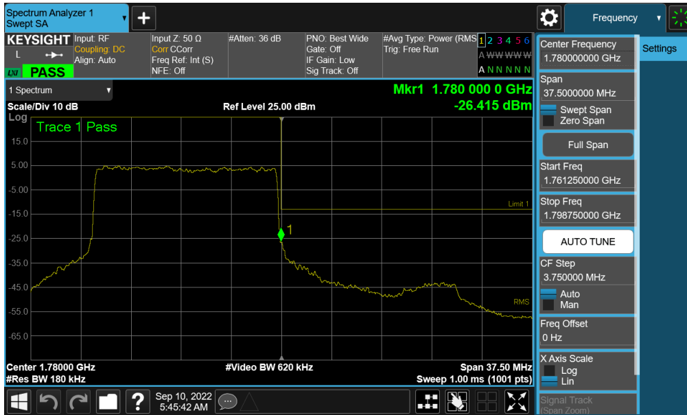
Plot 7-313. Upper Band Edge Plot (NR Band n66 – 15.0MHz - Full RB - Ant A)
