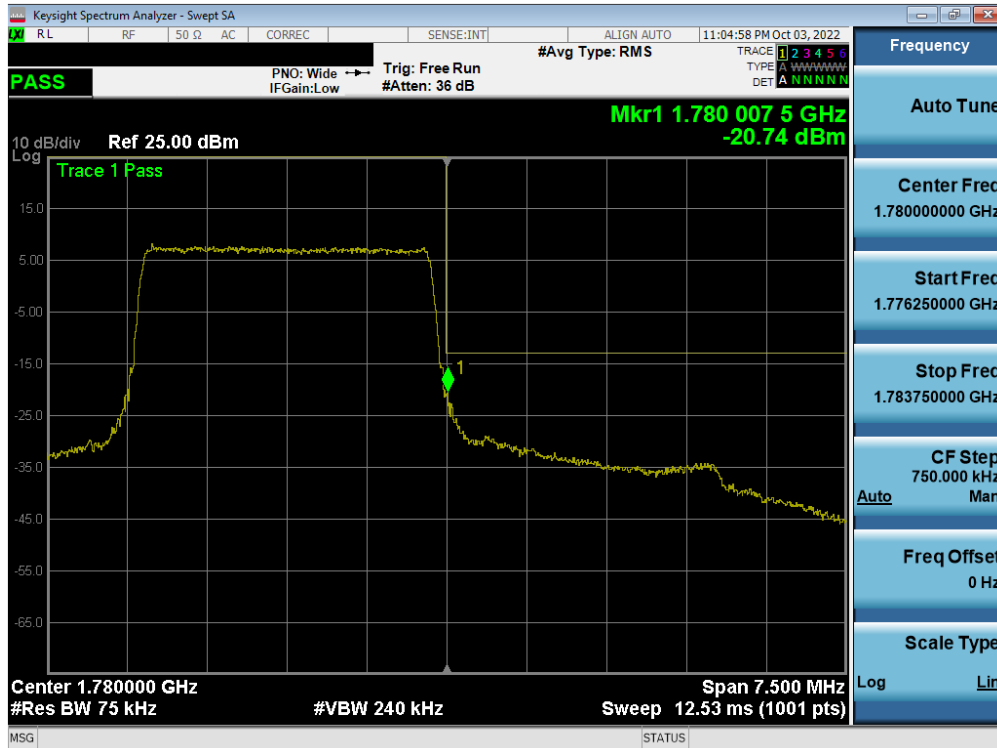
Plot 7-355. Upper Band Edge Plot (LTE Band 66 - 3MHz QPSK – Full RB - Ant F)
