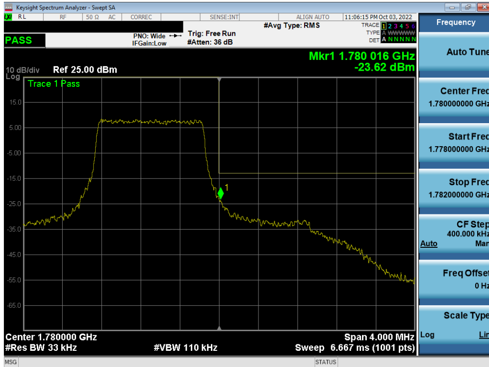
Plot 7-361. Upper Band Edge Plot (LTE Band 66 – 1.4MHz QPSK – Full RB - Ant F)
