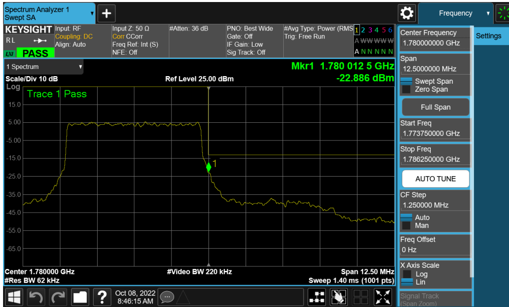
Plot 7-389. Upper Band Edge Plot (NR Band n66 – 5.0MHz - Full RB - Ant F)
