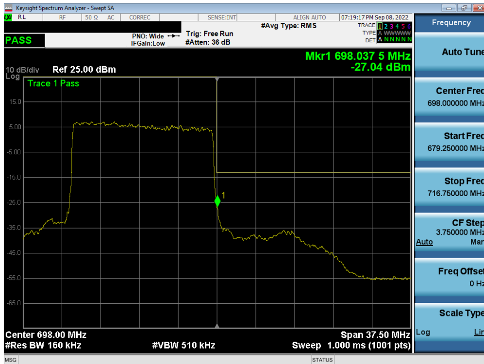
Plot 7-244. Upper Band Edge Plot (NR Band n71 – 15.0MHz - Full RB - Ant A)
