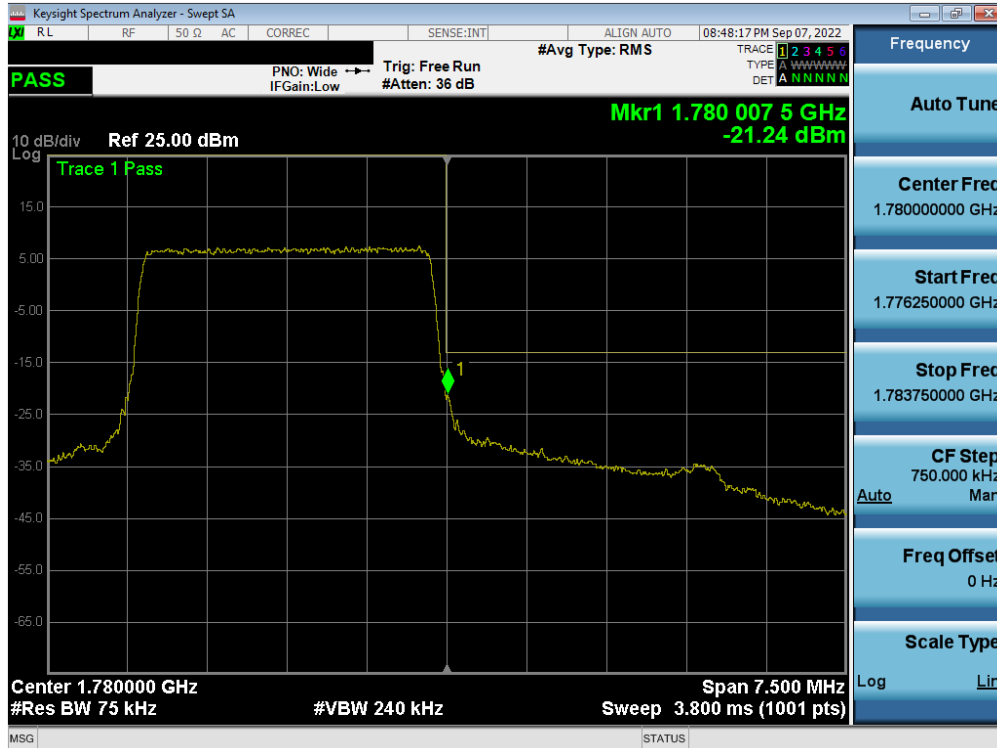
Plot 7-287. Upper Band Edge Plot (LTE Band 66 - 3MHz QPSK – Full RB - Ant A)
