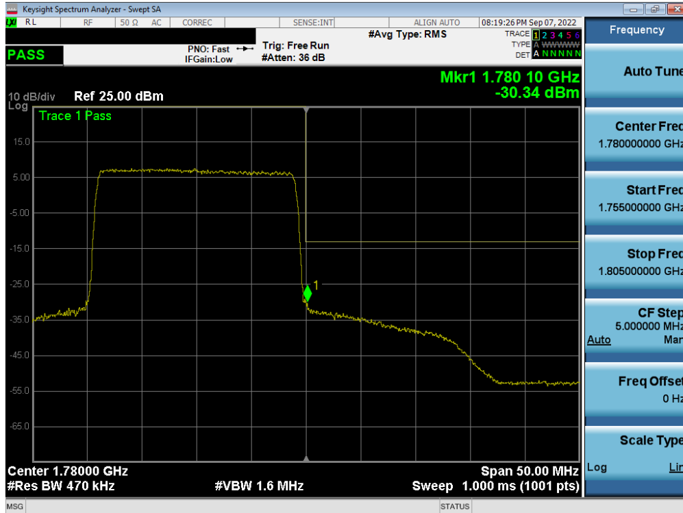
Plot 7-263. Upper Band Edge Plot (LTE Band 66 - 20MHz QPSK - Full RB - Ant A)
