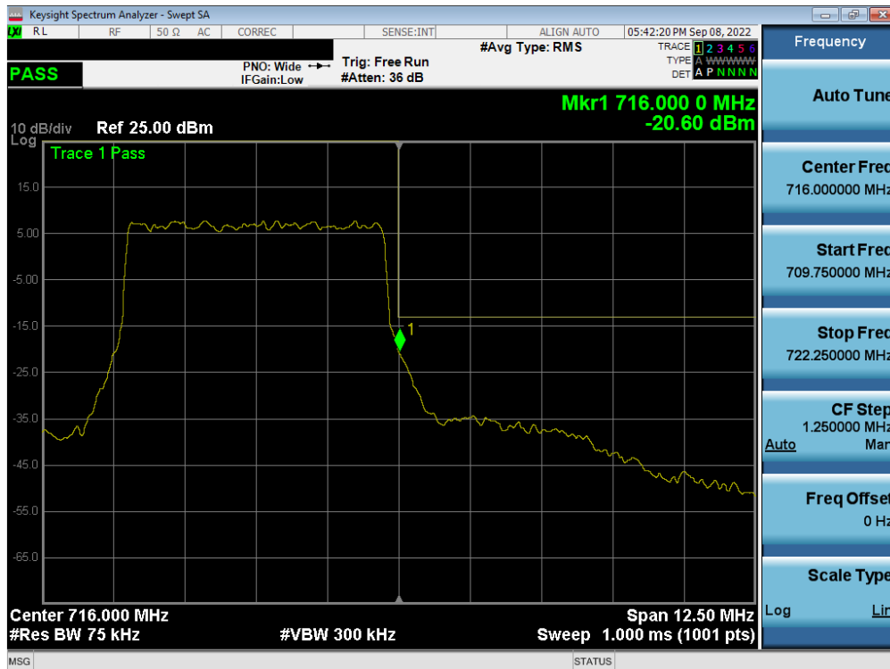
Plot 7-254. Upper Band Edge Plot (NR Band n12 – 5.0MHz - Full RB - Ant A)
