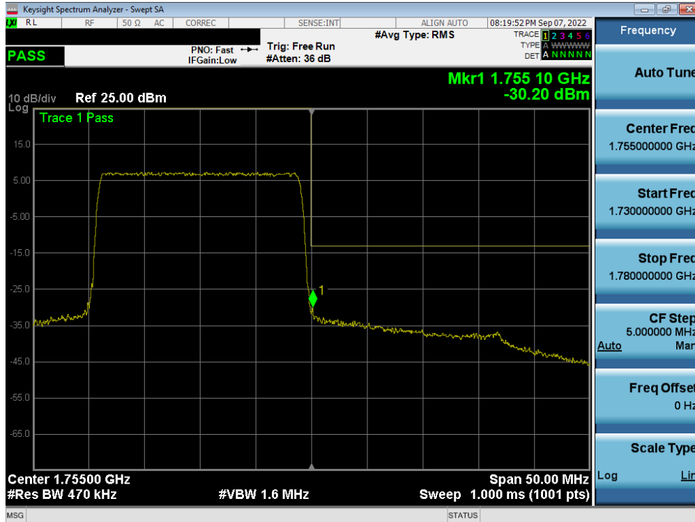
Plot 7-261. Upper Band Edge Plot (LTE Band 4 - 20MHz QPSK – Full RB - Ant A)
