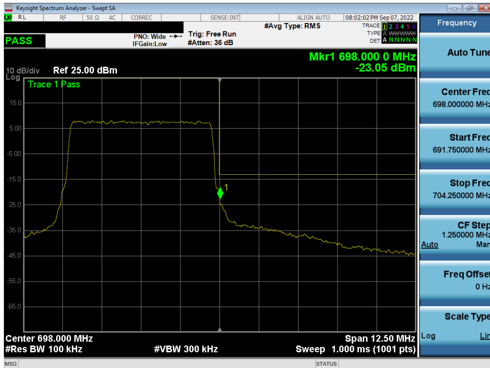
Plot 7-224. Upper Band Edge Plot (LTE Band 71 - 5MHz QPSK – Full RB - Ant A)
