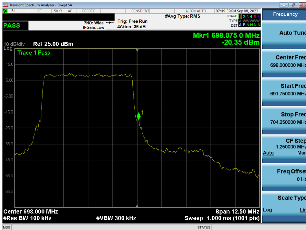
Plot 7-248. Upper Band Edge Plot (NR Band n71 – 5.0MHz - Full RB - Ant A)
