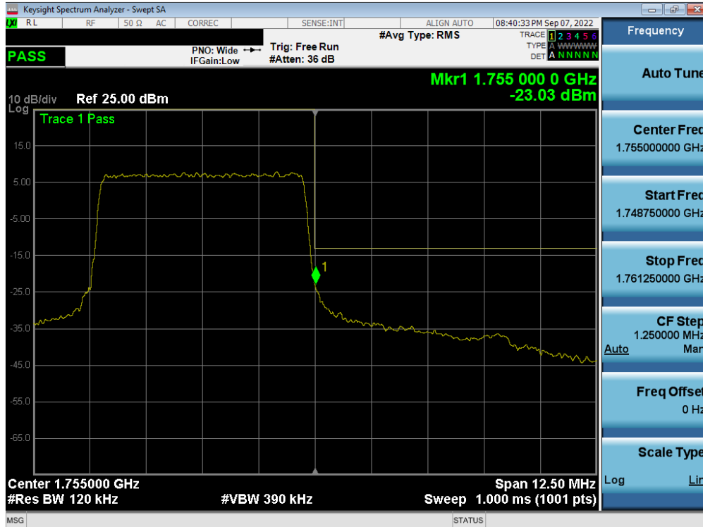
Plot 7-279. Upper Band Edge Plot (LTE Band 4 - 5MHz QPSK – Full RB - Ant A)
