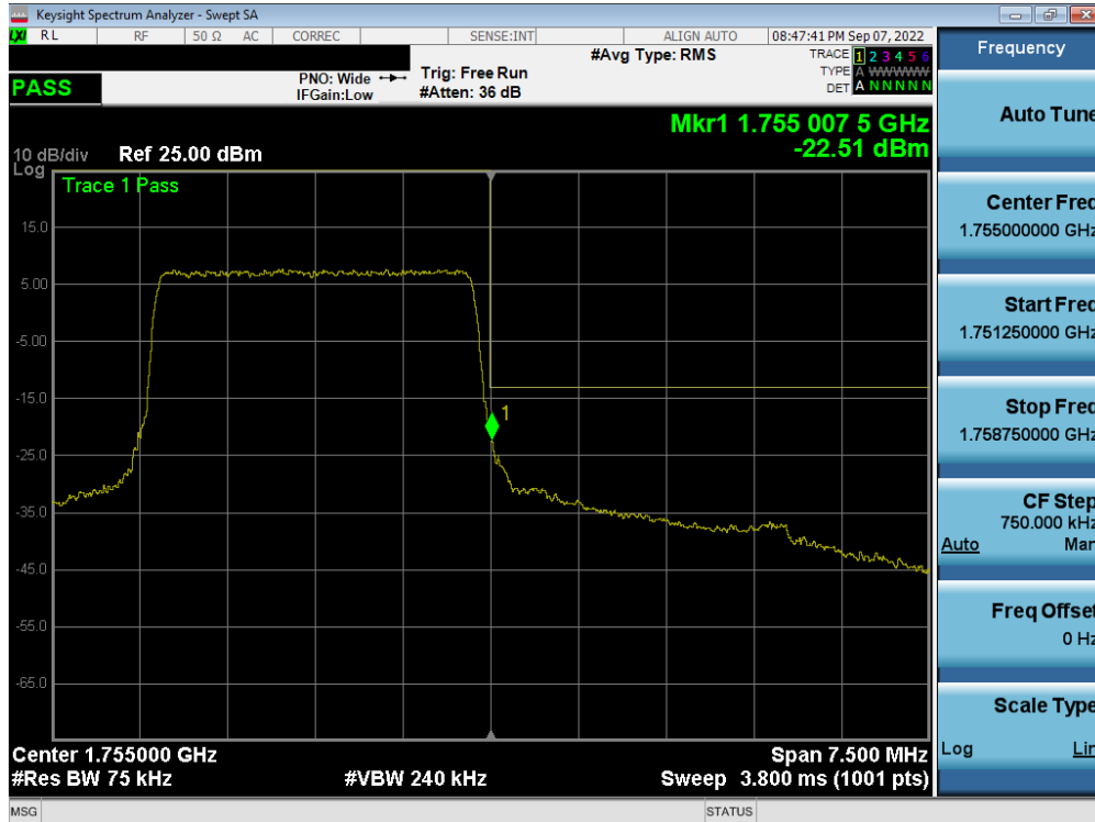
Plot 7-285. Upper Band Edge Plot (LTE Band 4 - 3MHz QPSK – Full RB - Ant A)
