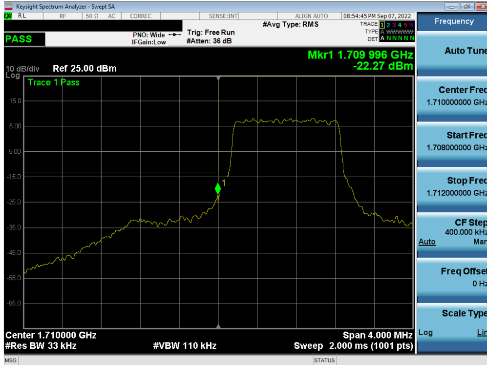
Plot 7-289. Lower Band Edge Plot (LTE Band 66/4 – 1.4MHz QPSK – Full RB - Ant A)
