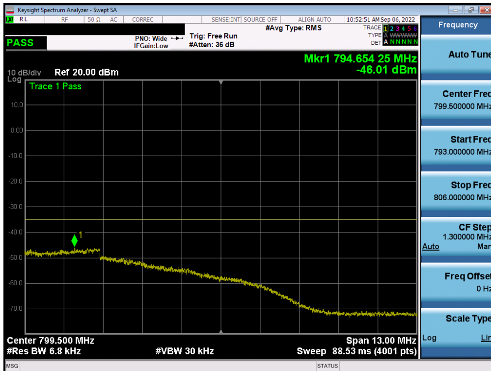
Plot 7-236. Upper Emission Mask Plot (LTE Band 13 - 10MHz QPSK – Full RB - Ant A)
