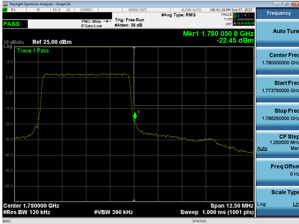
Plot 7-281. Upper Band Edge Plot (LTE Band 66 - 5MHz QPSK – Full RB - Ant A)
