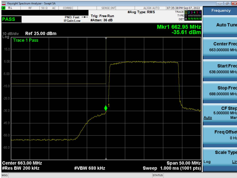
Plot 7-217. Lower Band Edge Plot (LTE Band 71 - 20MHz QPSK – Full RB - Ant A)
