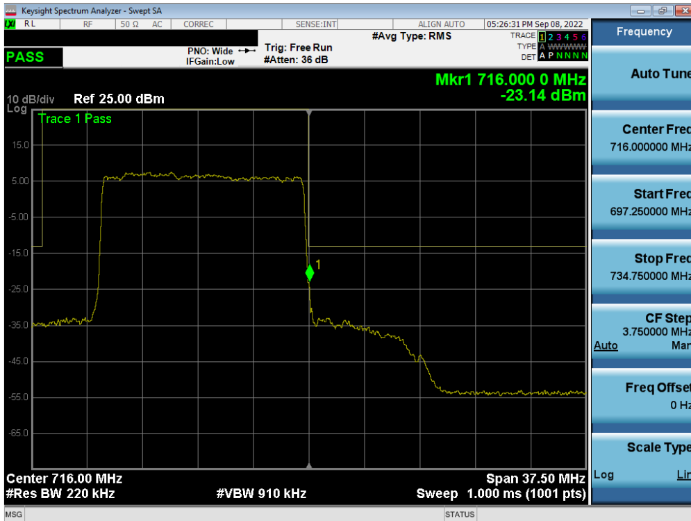
Plot 7-250. Upper Band Edge Plot (NR Band n12 – 15.0MHz - Full RB - Ant A)
