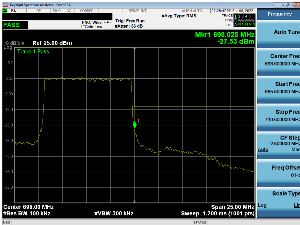
Plot 7-246. Upper Band Edge Plot (NR Band n71 – 10.0MHz - Full RB - Ant A)
