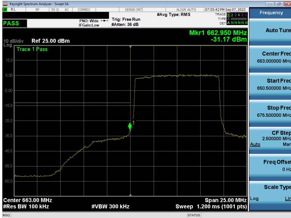
Plot 7-221. Lower Band Edge Plot (LTE Band 71 - 10MHz QPSK – Full RB - Ant A)
