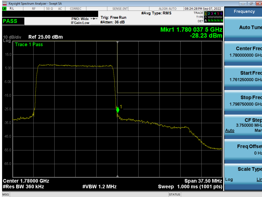
Plot 7-269. Upper Band Edge Plot (LTE Band 66 - 15MHz QPSK - Full RB - Ant A)
