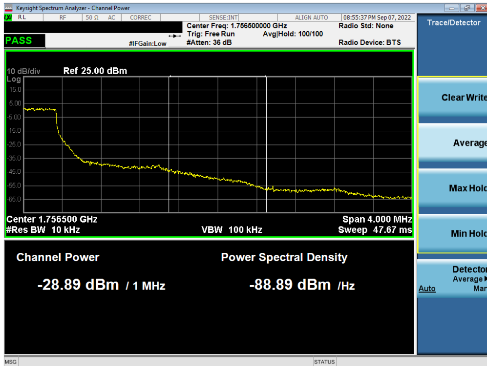
Plot 7-292. Upper Extended Band Edge Plot (LTE Band 4 – 1.4MHz QPSK – Full RB - Ant A)
