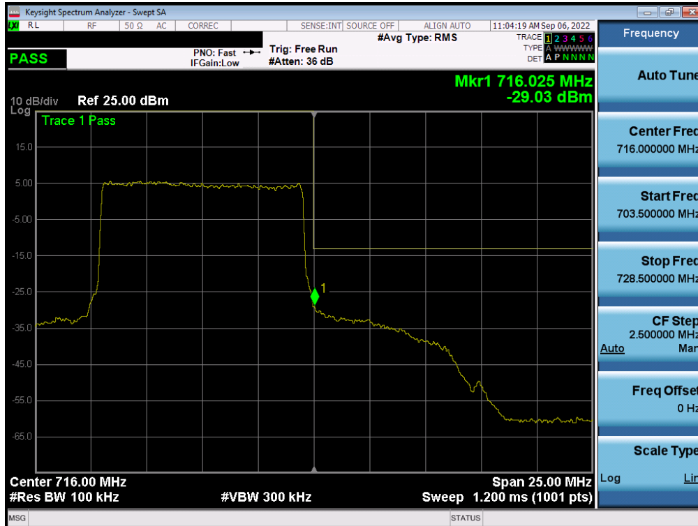
Plot 7-226. Upper Band Edge Plot (LTE Band 12 - 10MHz QPSK – Full RB - Ant A)
