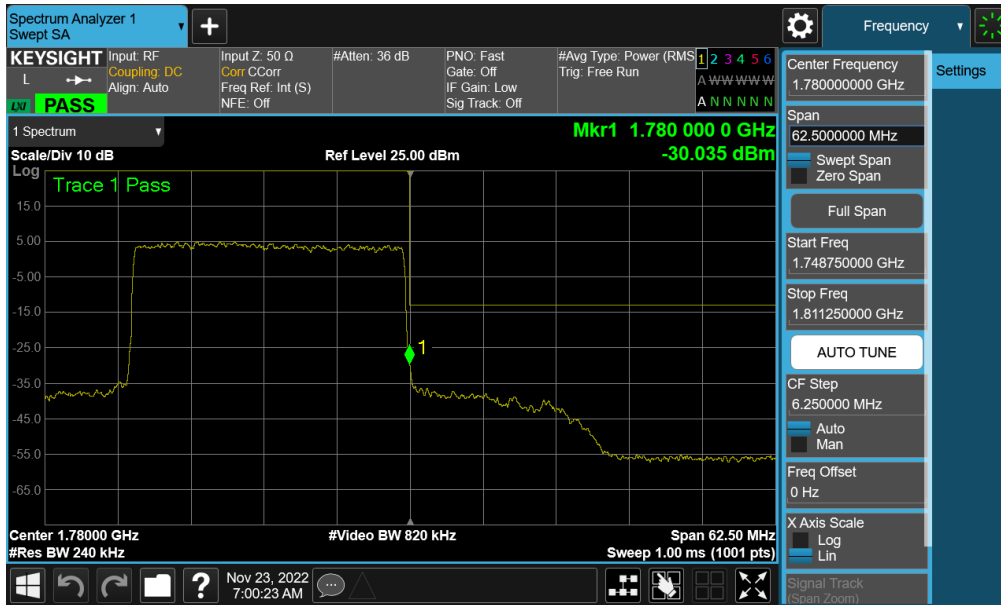
Plot 7-305. Upper Band Edge Plot (NR Band n66 – 25.0MHz - Full RB - Ant A)
