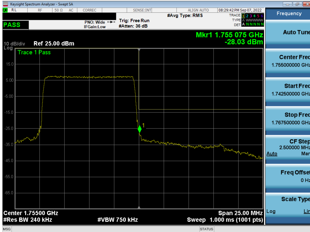
Plot 7-273. Upper Band Edge Plot (LTE Band 4 - 10MHz QPSK – Full RB - Ant A)
