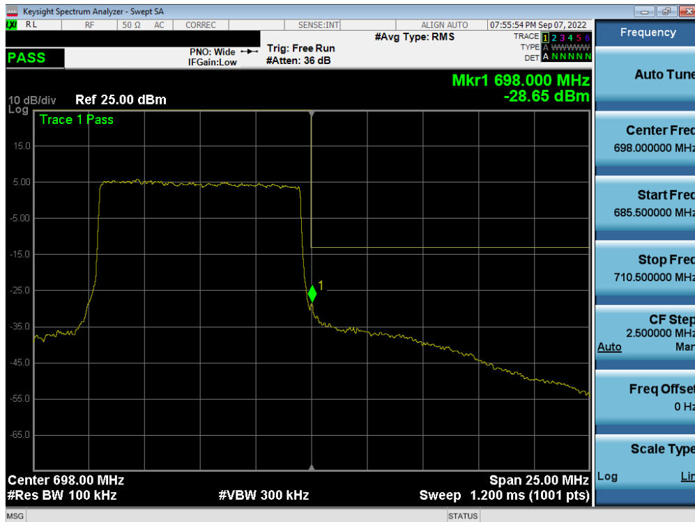
Plot 7-222. Upper Band Edge Plot (LTE Band 71 - 10MHz QPSK – Full RB - Ant A)
