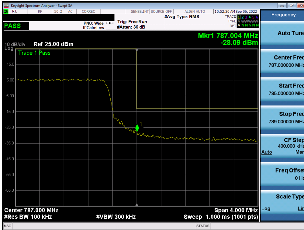
Plot 7-235. Upper Band Edge Plot (LTE Band 13 - 10MHz QPSK – Full RB - Ant A)
