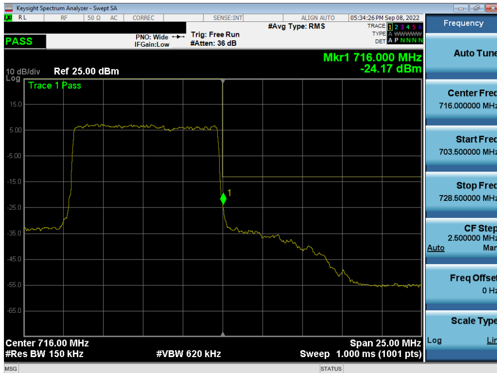
Plot 7-252. Upper Band Edge Plot (NR Band n12 – 10.0MHz - Full RB - Ant A)
