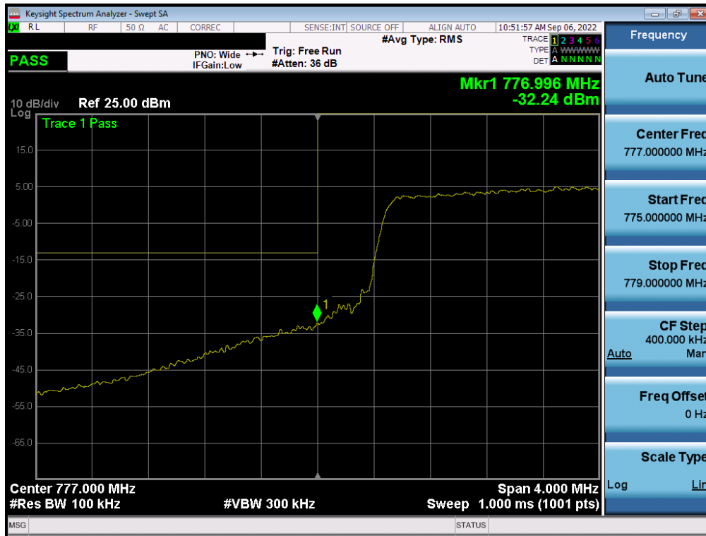
Plot 7-233. Lower Band Edge Plot (LTE Band 13 - 10MHz QPSK – Full RB - Ant A)
