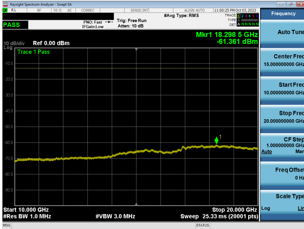
Plot 7-195. Conducted Spurious Plot (LTE Band 66/4 - 20MHz QPSK - 1 RB - High Channel – Ant F)
