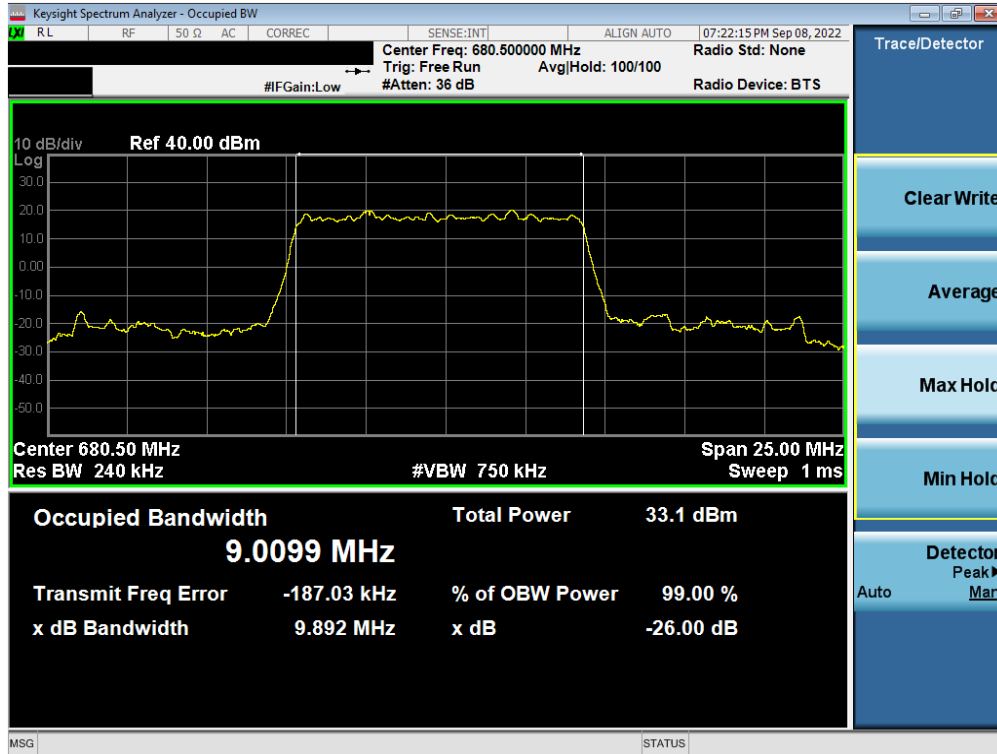
Plot 7-27. Occupied Bandwidth Plot (NR Band n71 - 10MHz DFT's BPSK - Full RB – Ant A)
