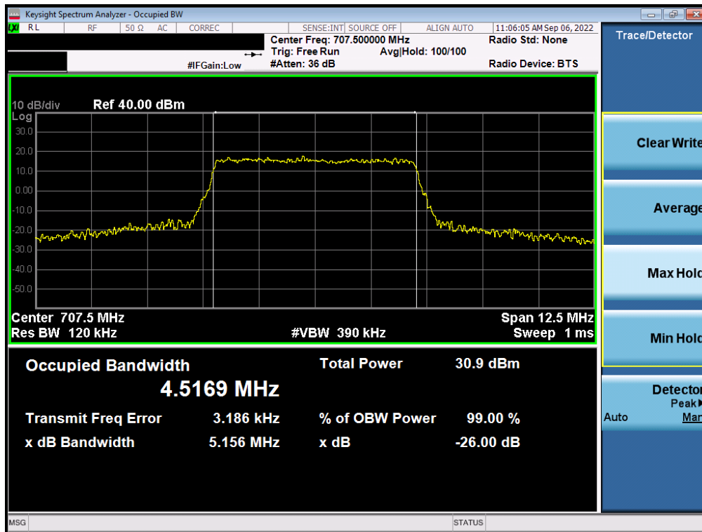
Plot 7-12. Occupied Bandwidth Plot (LTE Band 12 - 5MHz 16-QAM - Full RB – Ant A)
