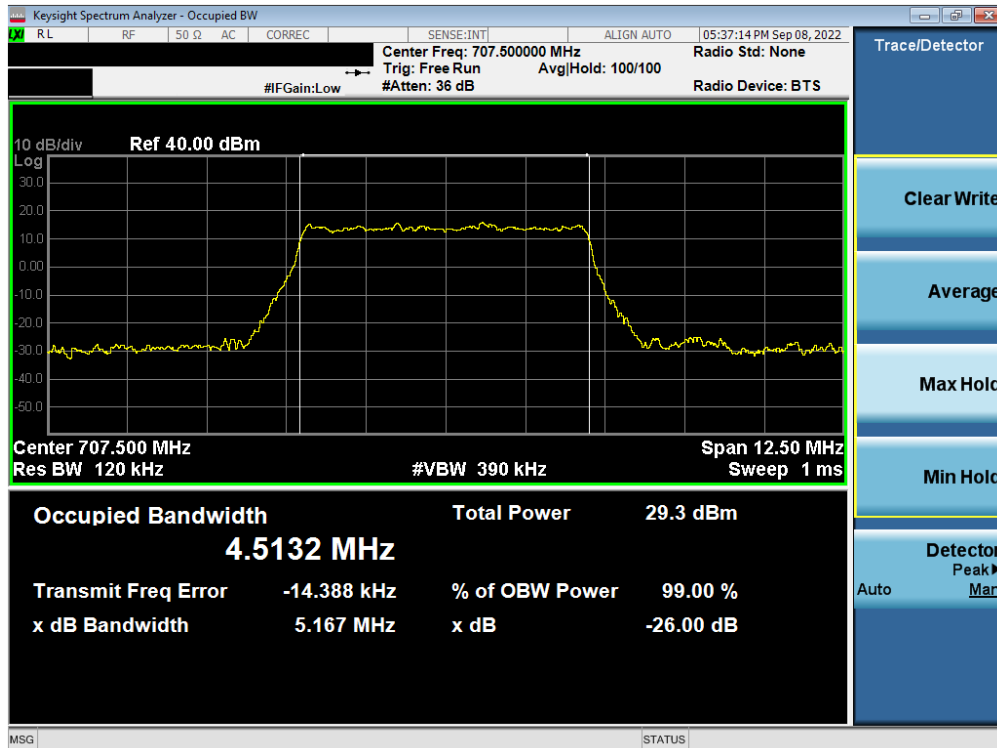
Plot 7-40. Occupied Bandwidth Plot (NR Band n12 - 5MHz CP-OFDM QPSK - Full RB – Ant A)
