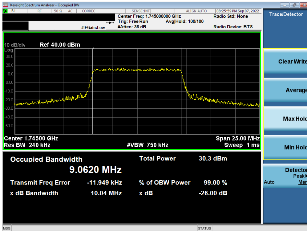
Plot 7-48. Occupied Bandwidth Plot (LTE Band 66/4 - 10MHz 16-QAM - Full RB - Ant A)
