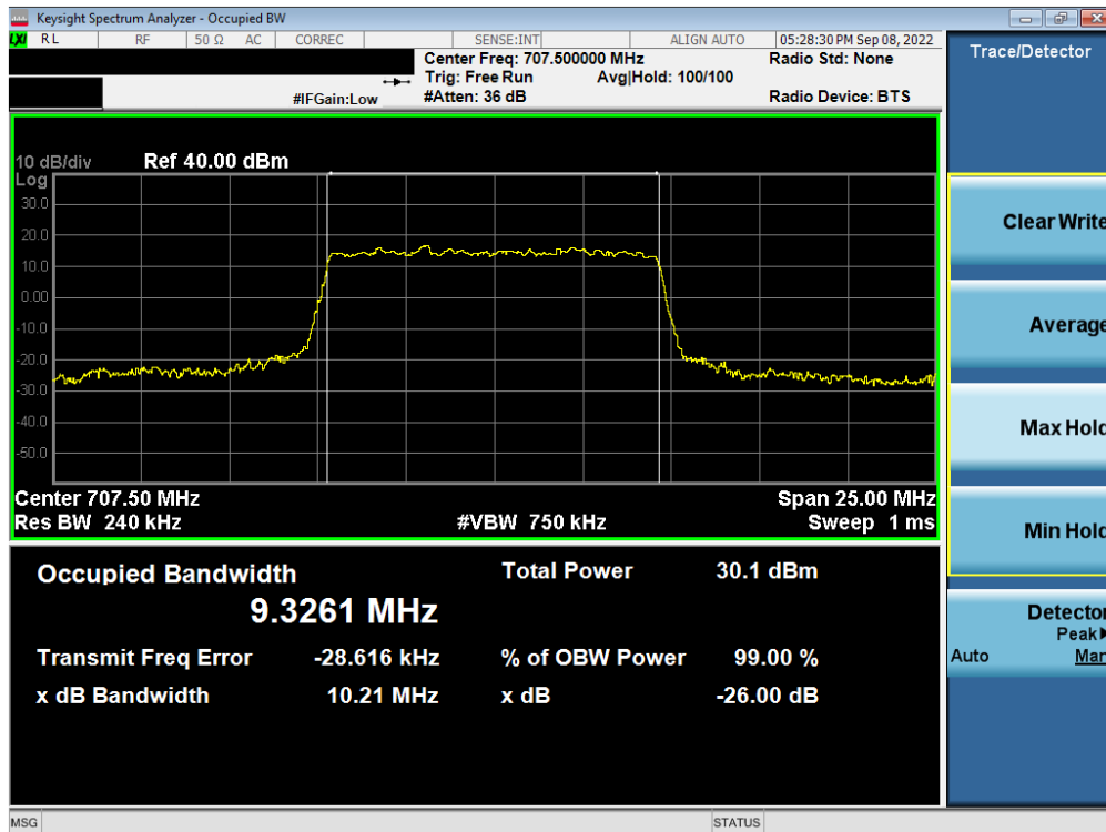
Plot 7-38. Occupied Bandwidth Plot (NR Band n12 - 10MHz CP-OFDM 16-QAM - Full RB – Ant A)
