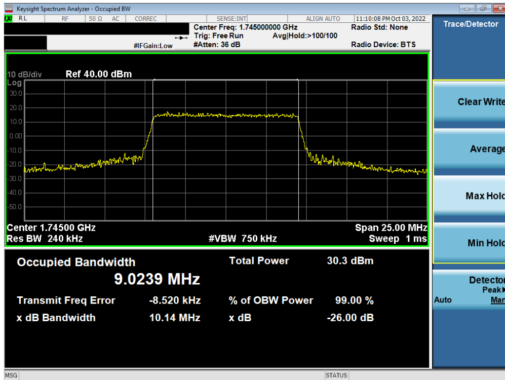
Plot 7-81. Occupied Bandwidth Plot (LTE Band 66/4 - 10MHz 16-QAM - Full RB - Ant F)
