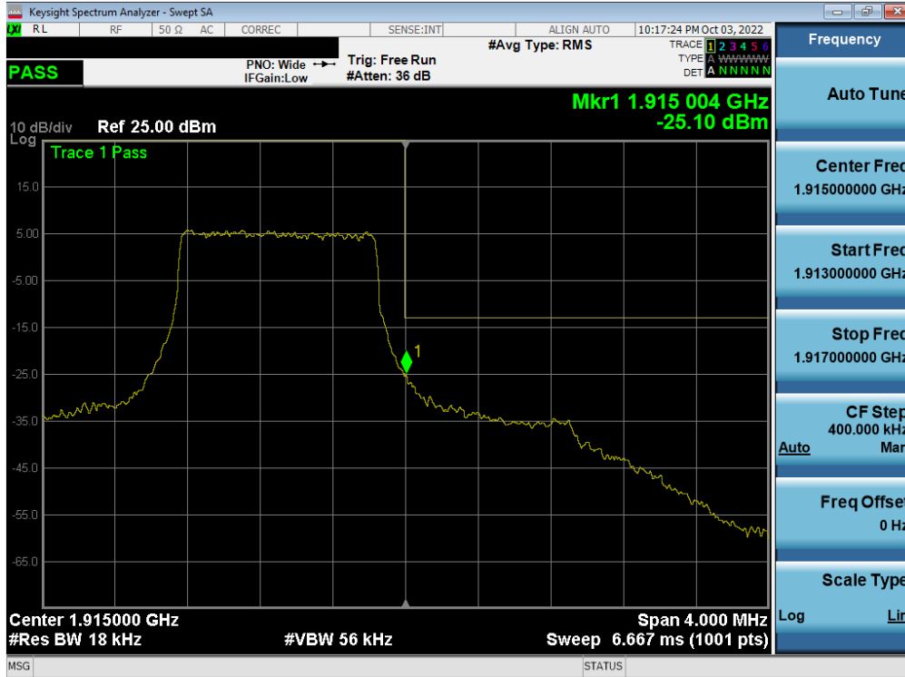
Plot 7-194. Upper Band Edge Plot (LTE Band 25 – 1.4MHz QPSK – Full RB - Ant F)
