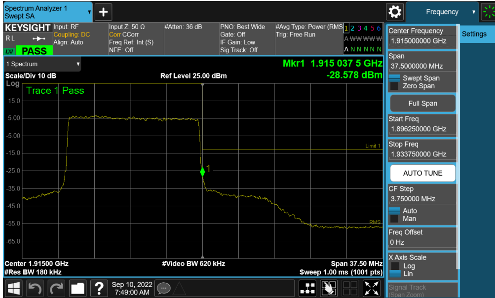
Plot 7-218. Upper Band Edge Plot (NR Band n25 - 15MHz QPSK – Full RB - Ant A)
