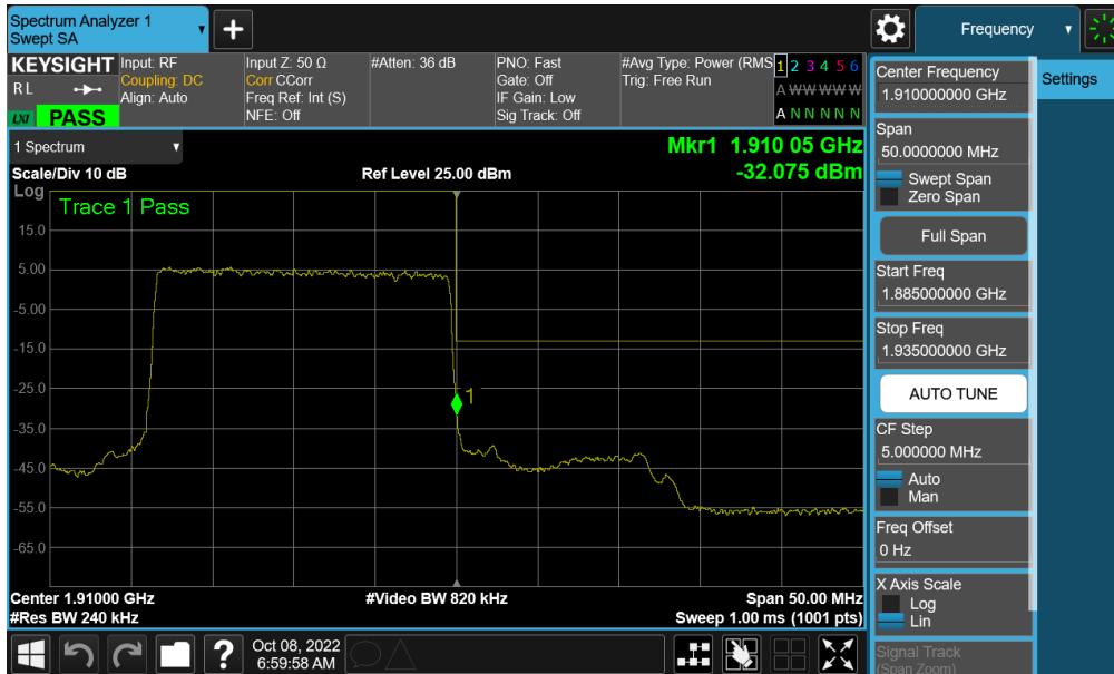
Plot 7-246. Upper Band Edge Plot (NR Band n2 - 20MHz QPSK – Full RB - Ant F)
