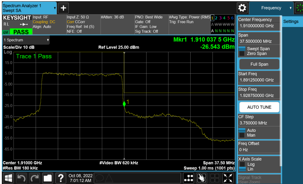
Plot 7-252. Upper Band Edge Plot (NR Band n2 - 15MHz QPSK – Full RB - Ant F)
