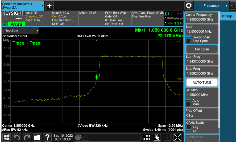
Plot 7-226. Lower Band Edge Plot (NR Band n25/2 – 5MHz QPSK – Full RB - Ant A)
