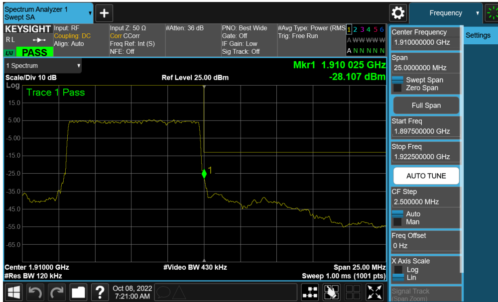
Plot 7-258. Upper Band Edge Plot (NR Band n2 - 10MHz QPSK – Full RB - Ant F)
