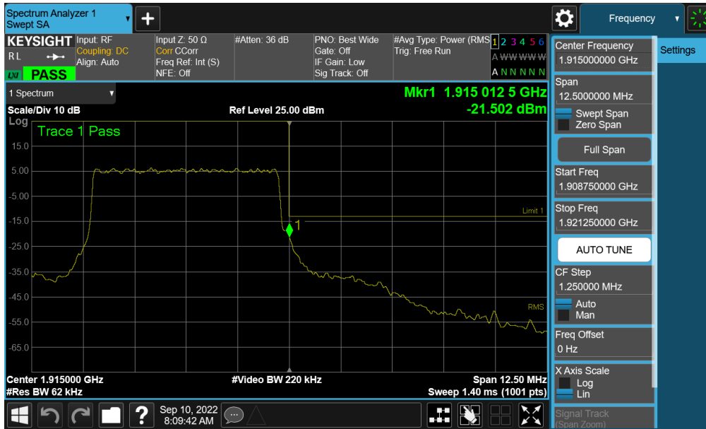
Plot 7-230. Upper Band Edge Plot (NR Band n25 – 5MHz QPSK – Full RB - Ant A)
