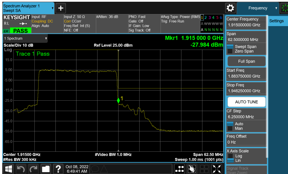
Plot 7-242. Upper Band Edge Plot (NR Band n25 - 25MHz QPSK – Full RB - Ant F)
