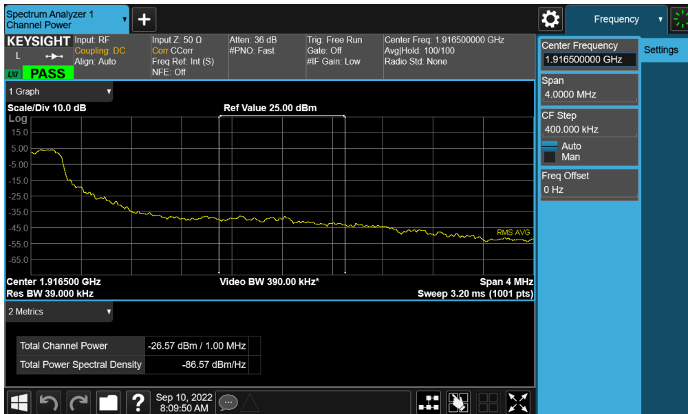
Plot 7-231. Extended Upper Band Edge Plot (NR Band n25 – 5MHz QPSK – Full RB - Ant A)
