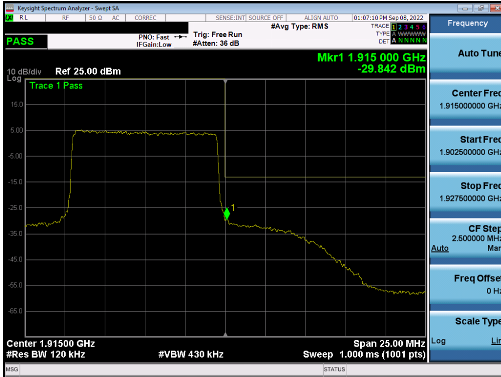
Plot 7-140. Upper Band Edge Plot (LTE Band 25 - 10MHz QPSK – Full RB - Ant A)
