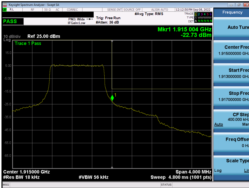
Plot 7-158. Upper Band Edge Plot (LTE Band 25 – 1.4MHz QPSK – Full RB - Ant1)
