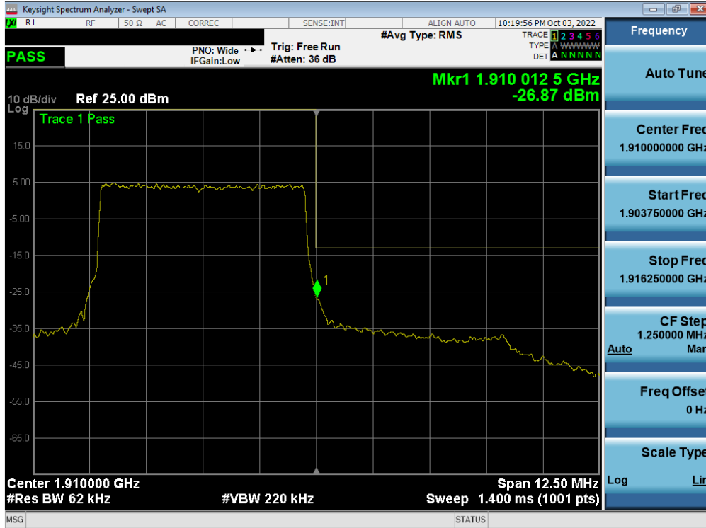
Plot 7-180. Upper Band Edge Plot (LTE Band 2 - 5MHz QPSK – Full RB - Ant F)
