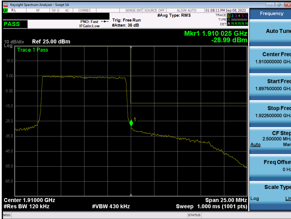
Plot 7-138. Upper Band Edge Plot (LTE Band 2 - 10MHz QPSK – Full RB - Ant A)
