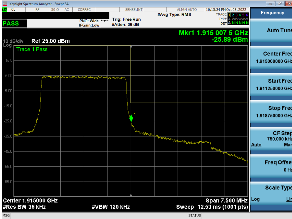
Plot 7-188. Upper Band Edge Plot (LTE Band 25 - 3MHz QPSK – Full RB - Ant F)
