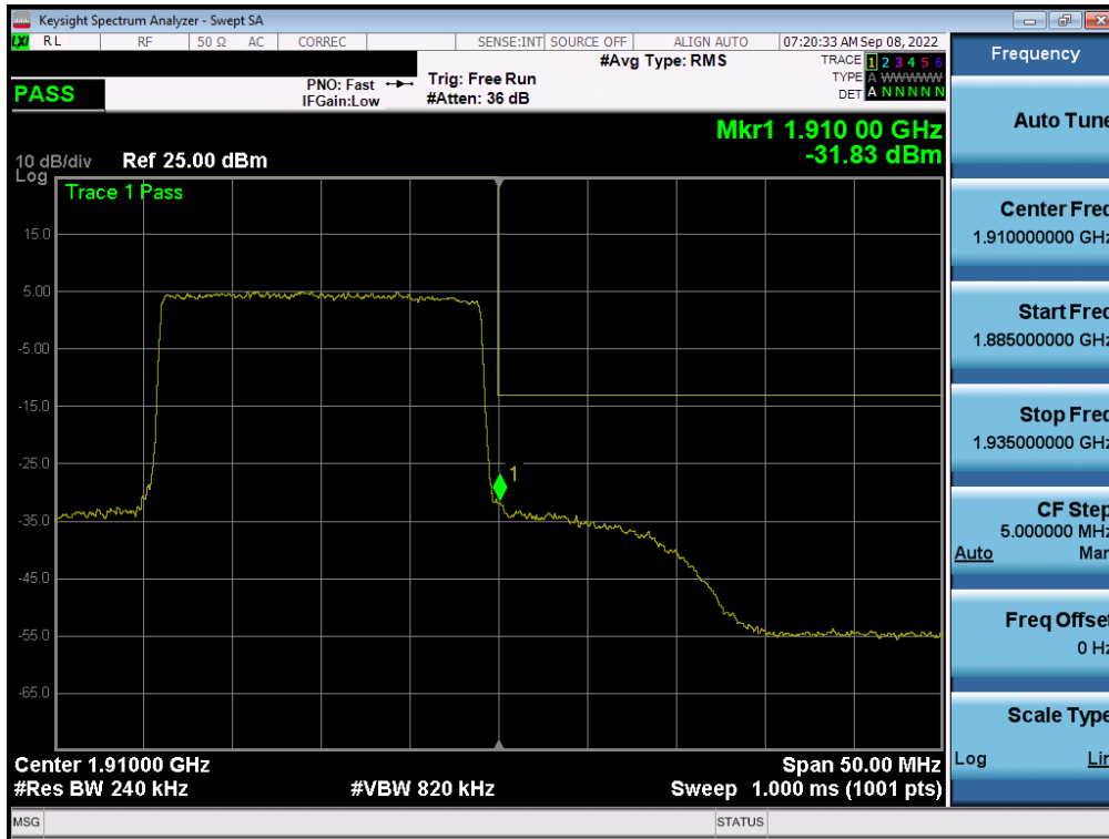
Plot 7-126. Upper Band Edge Plot (LTE Band 2 - 20MHz QPSK – Full RB - Ant A)
