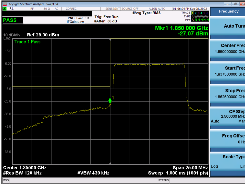
Plot 7-136. Lower Band Edge Plot (LTE Band 25/2 - 10MHz QPSK – Full RB - Ant A)
