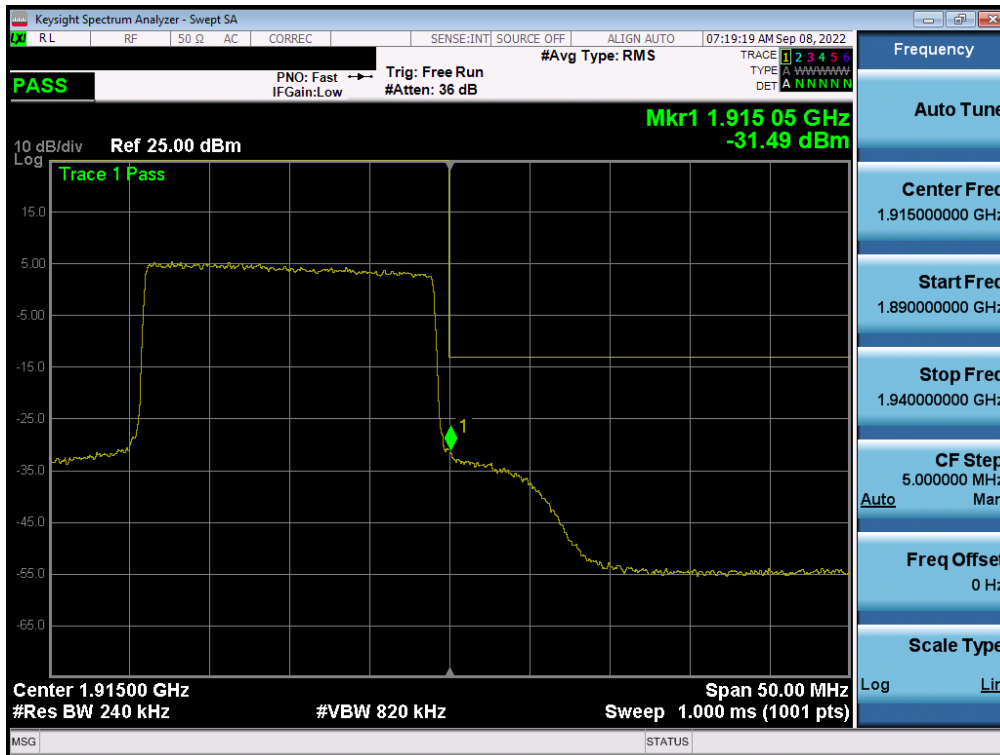
Plot 7-128. Upper Band Edge Plot (LTE Band 25 - 20MHz QPSK – Full RB - Ant A)
