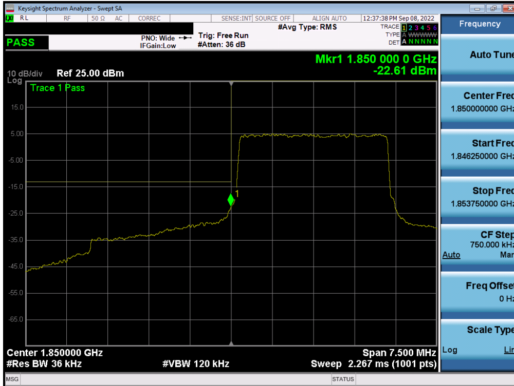
Plot 7-148. Lower Band Edge Plot (LTE Band 25/2 - 3MHz QPSK – Full RB - Ant A)
