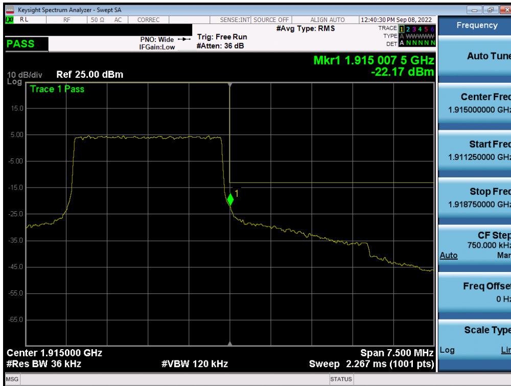
Plot 7-152. Upper Band Edge Plot (LTE Band 25 - 3MHz QPSK – Full RB - Ant1)
