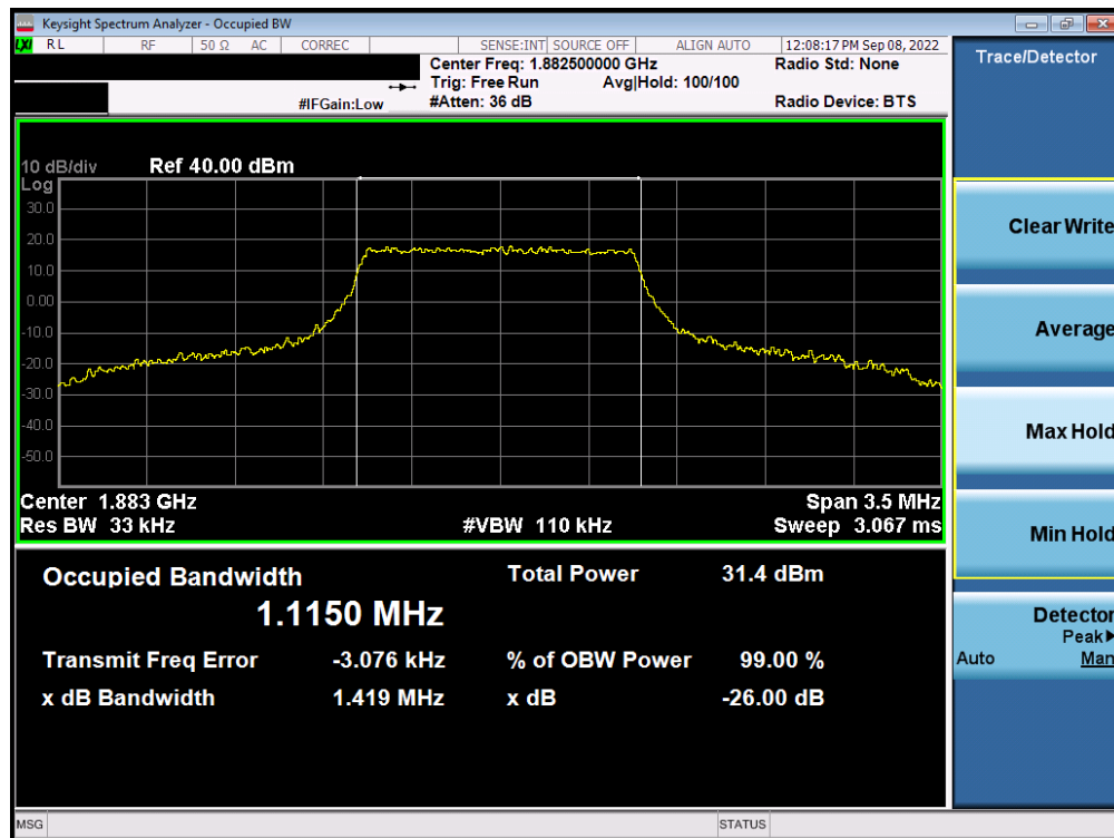
Plot 7-12. Occupied Bandwidth Plot (LTE Band 25/2 - 1.4MHz 16-QAM - Full RB - Ant A)
