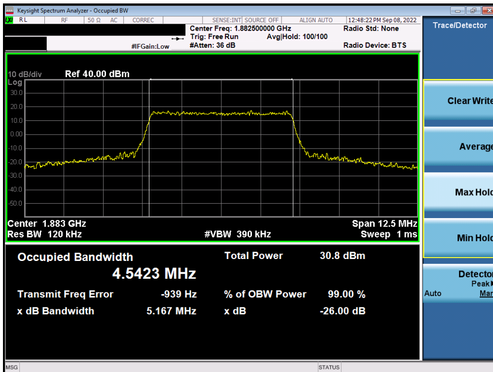
Plot 7-8. Occupied Bandwidth Plot (LTE Band 25/2 - 5MHz 16-QAM - Full RB - Ant A)
