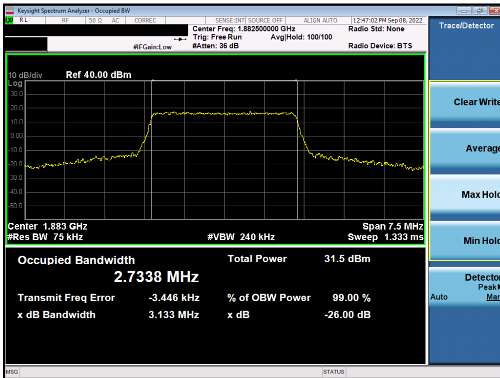
Plot 7-10. Occupied Bandwidth Plot (LTE Band 25/2 - 3MHz 16-QAM - Full RB - Ant A)
