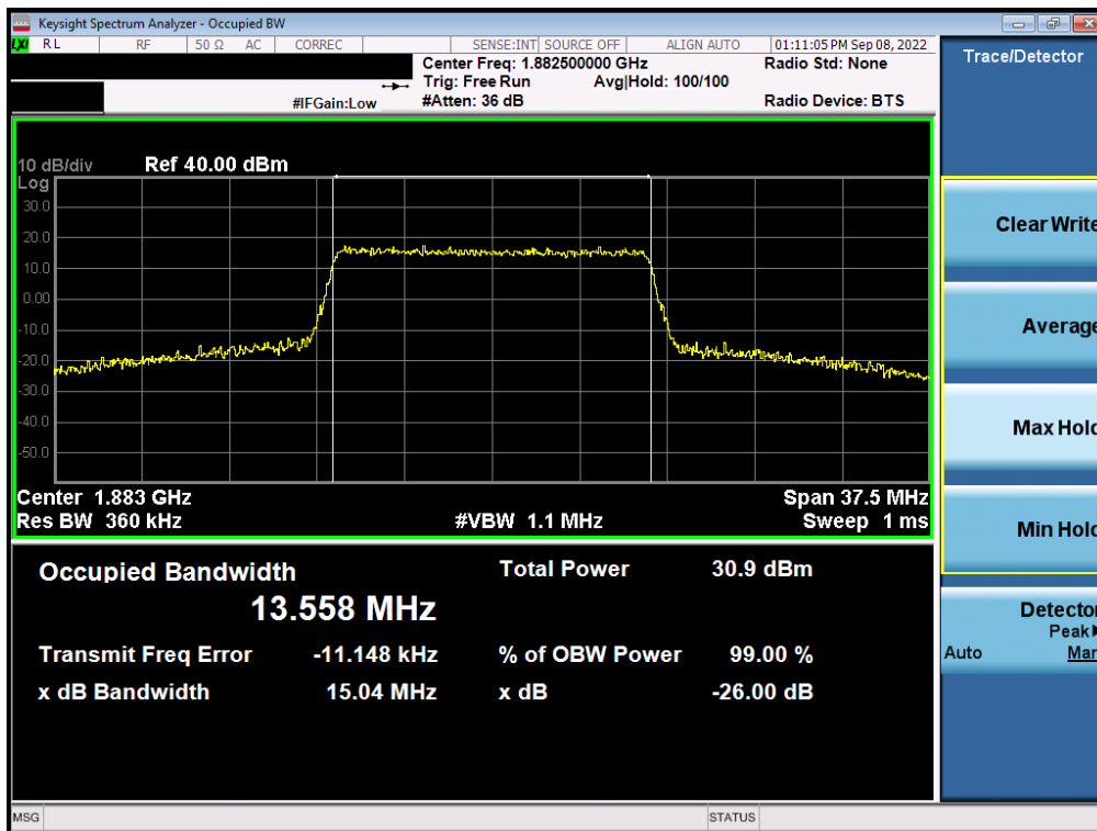
Plot 7-4. Occupied Bandwidth Plot (LTE Band 25/2 - 15MHz 16-QAM - Full RB - Ant A)
