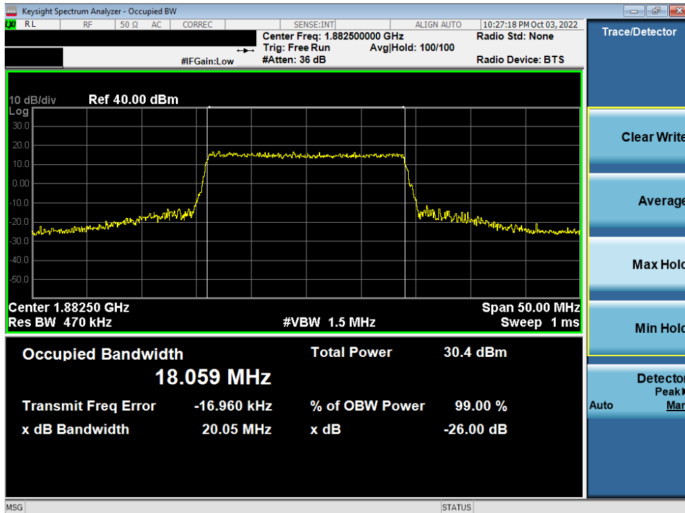
Plot 7-14. Occupied Bandwidth Plot (LTE Band 25/2 - 20MHz 16-QAM - Full RB - Ant F)
