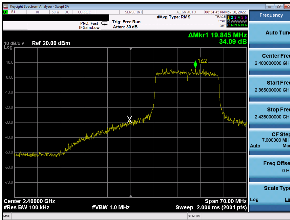
Plot 7-82. Band Edge Plot (802.11ax (2.4GHz) – Ch. 2) SISO ANT 2
