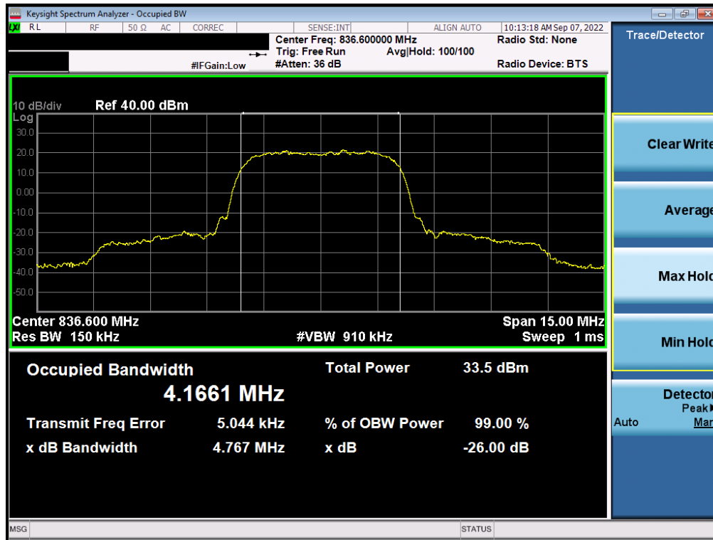
Plot 7-25. Occupied Bandwidth Plot (WCDMA, Ch. 4183)
