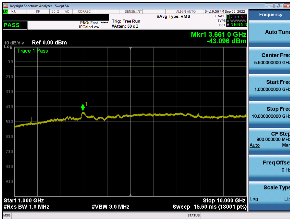
Plot 7-49. Conducted Spurious Plot (NR Band n26/5 - 20.0MHz - 1 RB - Mid Channel)
