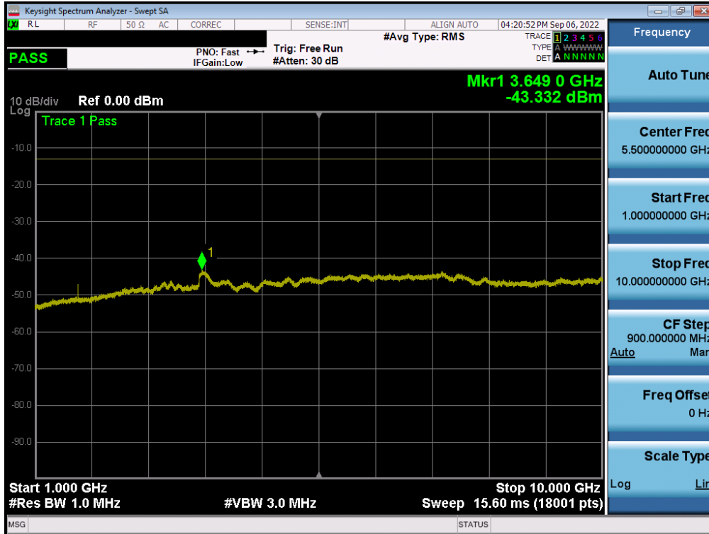
Plot 7-52. Conducted Spurious Plot (NR Band n26/5 - 20.0MHz - 1 RB - High Channel)
