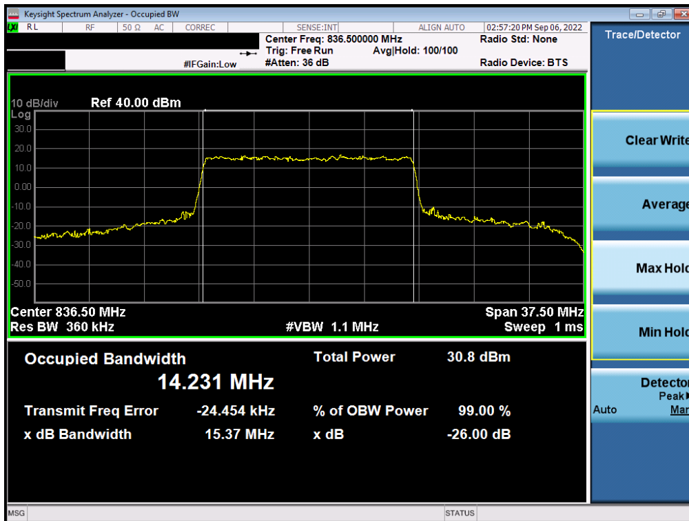
Plot 7-16. Occupied Bandwidth Plot (NR Band n26/5 - 15MHz 16-QAM - Full RB)
