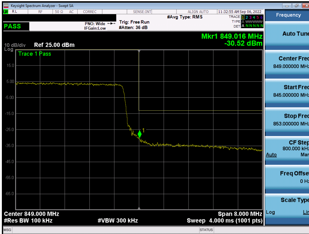
Plot 7-74. Upper Band Edge Plot (LTE Band 26/5 - 10MHz QPSK – Full RB)
