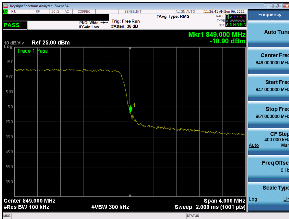
Plot 7-78. Upper Band Edge Plot (LTE Band 26/5 - 3MHz QPSK – Full RB)
