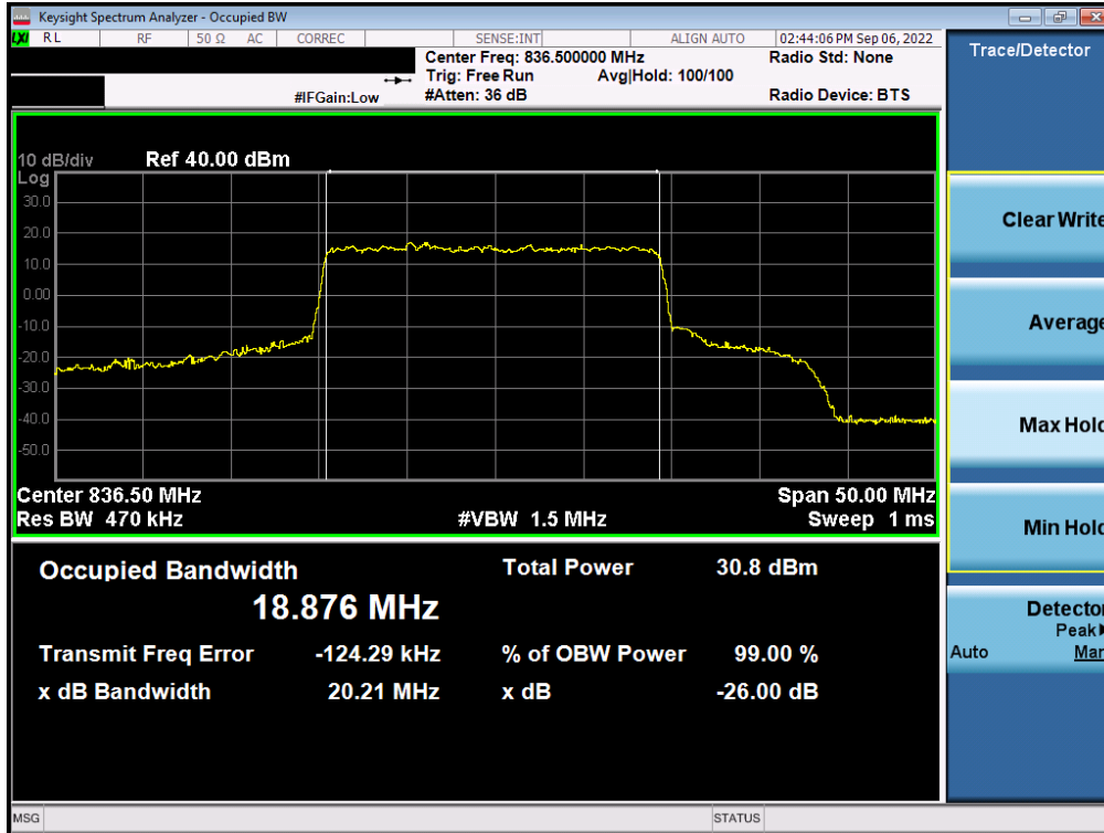
Plot 7-13. Occupied Bandwidth Plot (NR Band n26/5 - 20MHz 16-QAM - Full RB)
