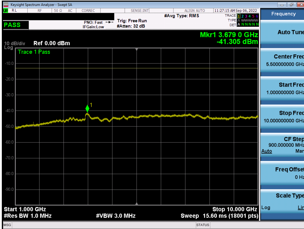
Plot 7-34. Conducted Spurious Plot (LTE Band 26/5 - 10MHz QPSK - 1 RB - High Channel)
