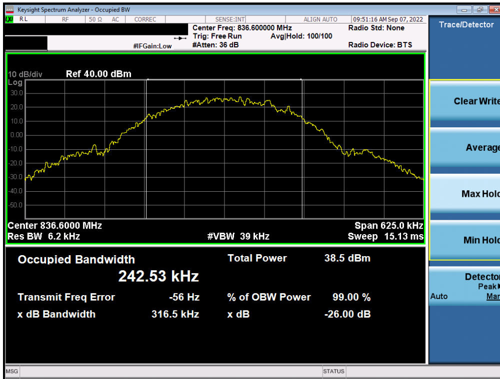
Plot 7-23. Occupied Bandwidth Plot (GPRS, Ch. 190)
