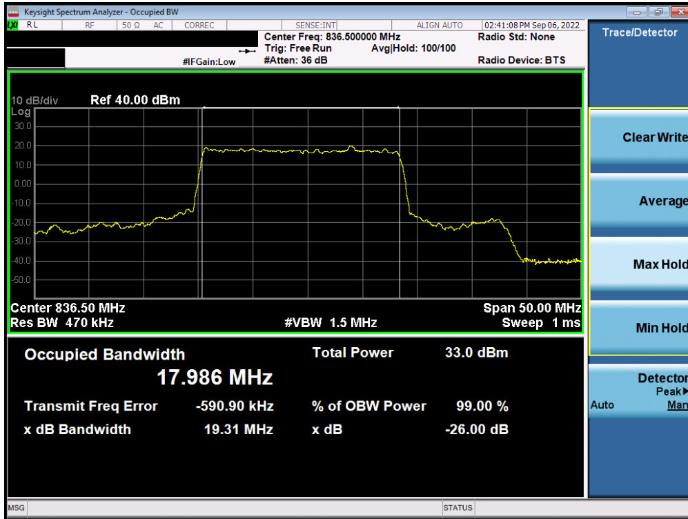
Plot 7-11. Occupied Bandwidth Plot (NR Band n26/5 - 20MHz \pi/2 BPSK - Full RB)
