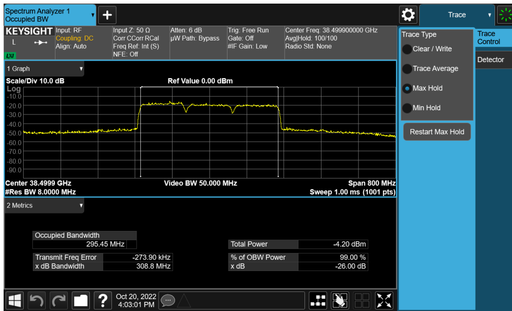
Plot 7-61. M patch Occupied Bandwidth Plot (100MHz-3CC – DFT-s-OFDM QPSK – Mid Channel)
