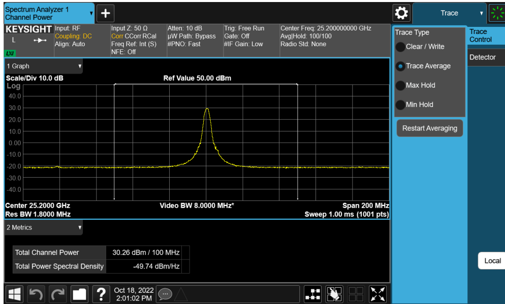
Plot 7-76. M patch EIRP Plot (Band n258-R2 – 100MHz-1CC High Channel DFT-s-OFDM \pi/2 BPSK)
