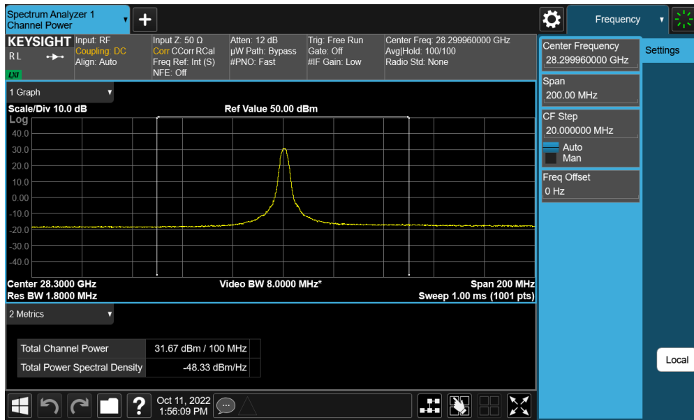
Plot 7-89. N patch EIRP Plot (Band n261 – 100MHz-1CC High Channel DFT-s-OFDM \pi/2 BPSK)
