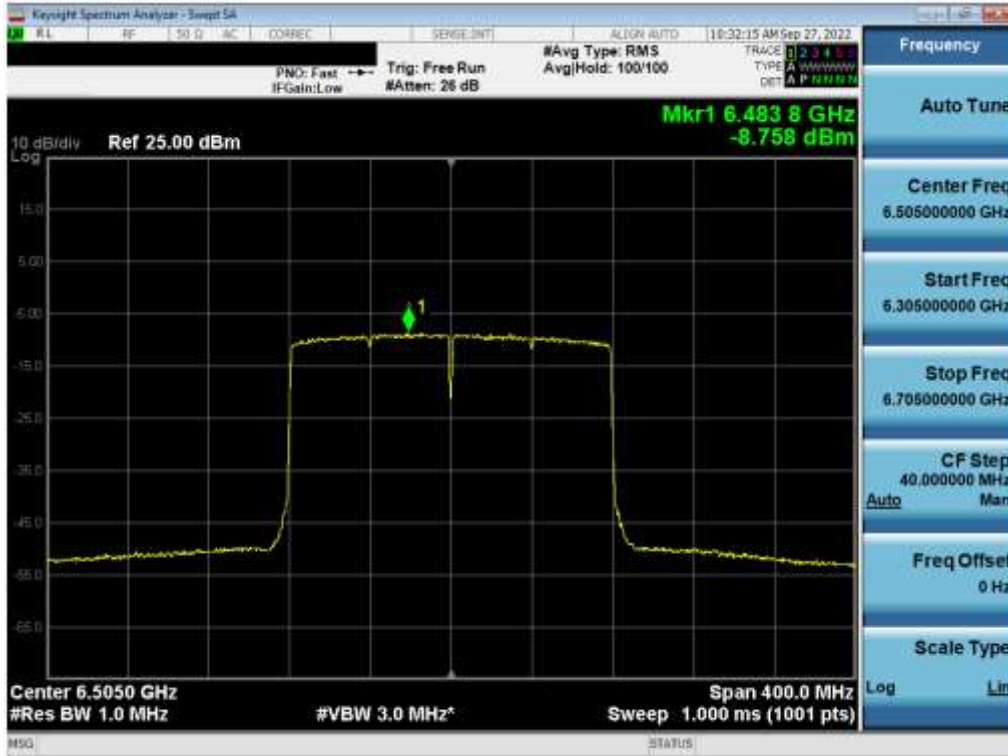
Plot 7-182. Power Spectral Density Measurement MIMO ANT2 (160MHz 802.11ax (UNII Band 6) – Ch. 111)
