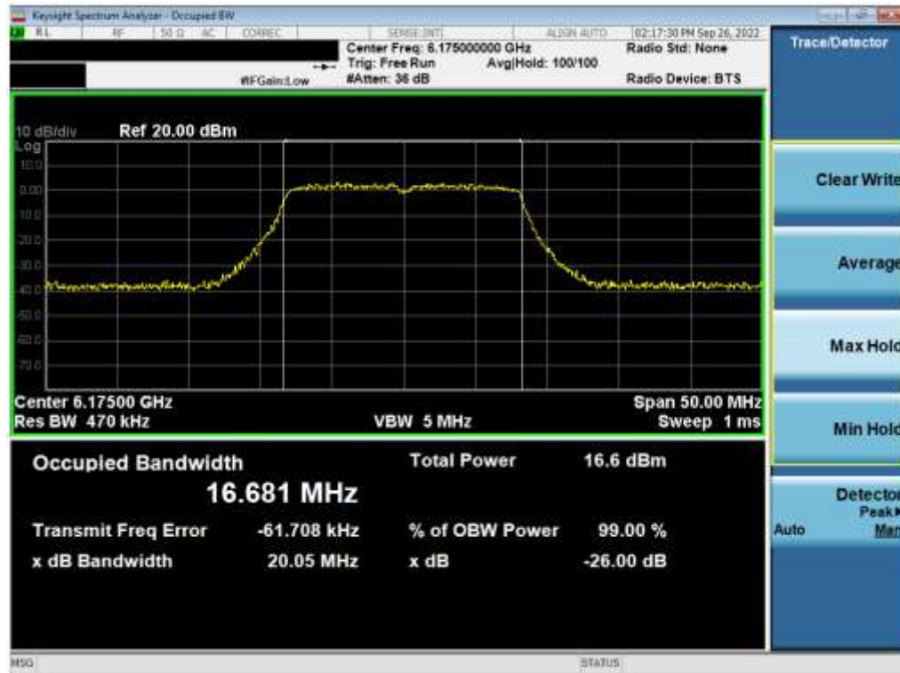
Plot 7-54. 26dB Bandwidth Plot MIMO ANT2 (20MHz 802.11a (UNII Band 5) – Ch. 45)
