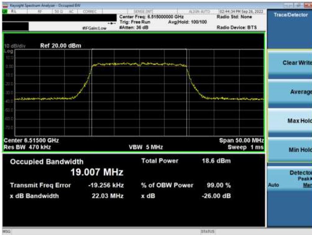
Plot 7-73. 26dB Bandwidth Plot MIMO ANT2 (20MHz 802.11ax (UNII Band 6) – Ch. 113)
