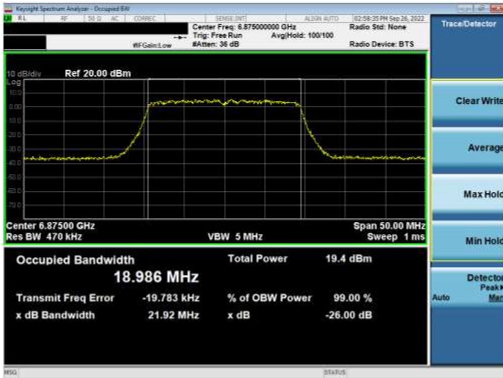
Plot 7-84. 26dB Bandwidth Plot MIMO ANT2 (20MHz 802.11ax (UNII Band 7) – Ch. 185)
