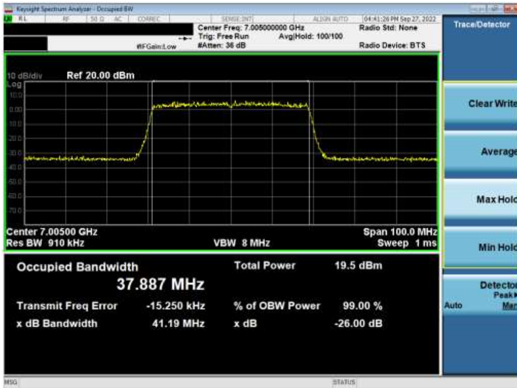
Plot 7-48. 26dB Bandwidth Plot MIMO ANT1 (40MHz 802.11ax (UNII Band 8) – Ch. 211)
