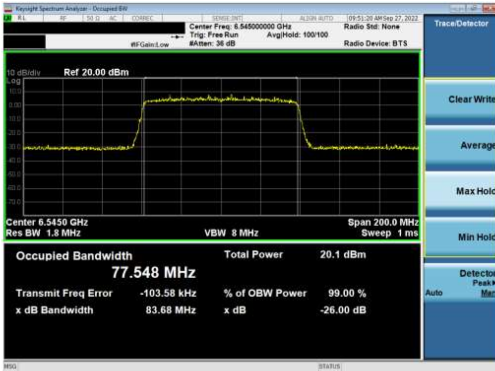
Plot 7-88. 26dB Bandwidth Plot MIMO ANT2 (80MHz 802.11ax (UNII Band 7) – Ch. 119)
