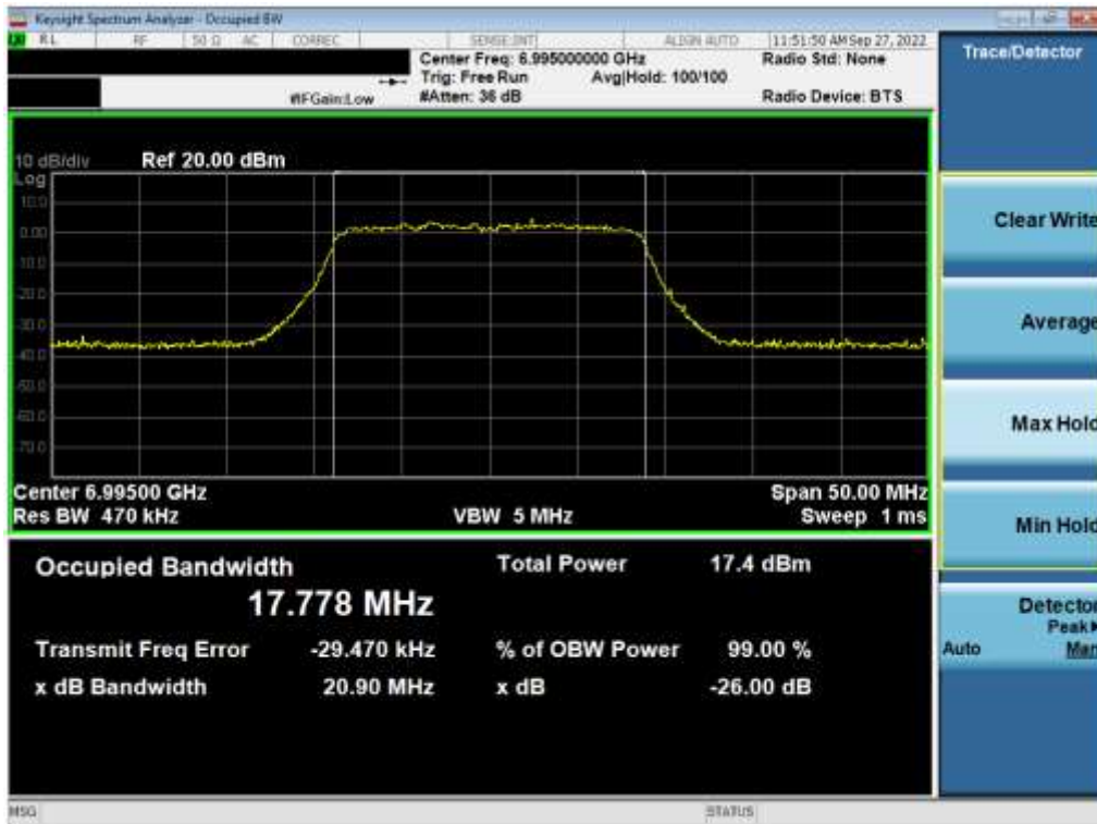
Plot 7-42. 26dB Bandwidth Plot MIMO ANT1 (20MHz 802.11a (UNII Band 8) – Ch. 209)
