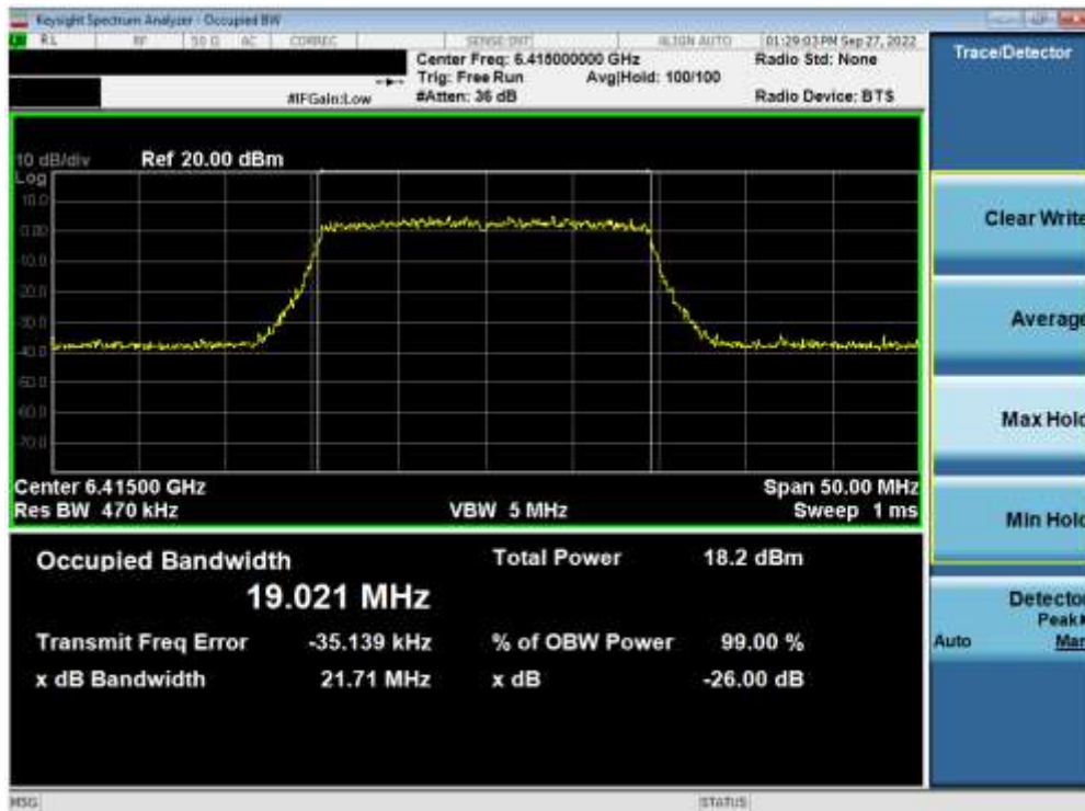
Plot 7-6. 26dB Bandwidth Plot MIMO ANT1 (20MHz 802.11ax (UNII Band 5) – Ch. 93)
