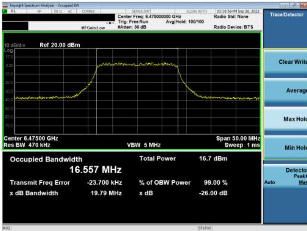
Plot 7-69. 26dB Bandwidth Plot MIMO ANT2 (20MHz 802.11a (UNII Band 6) – Ch. 105)
