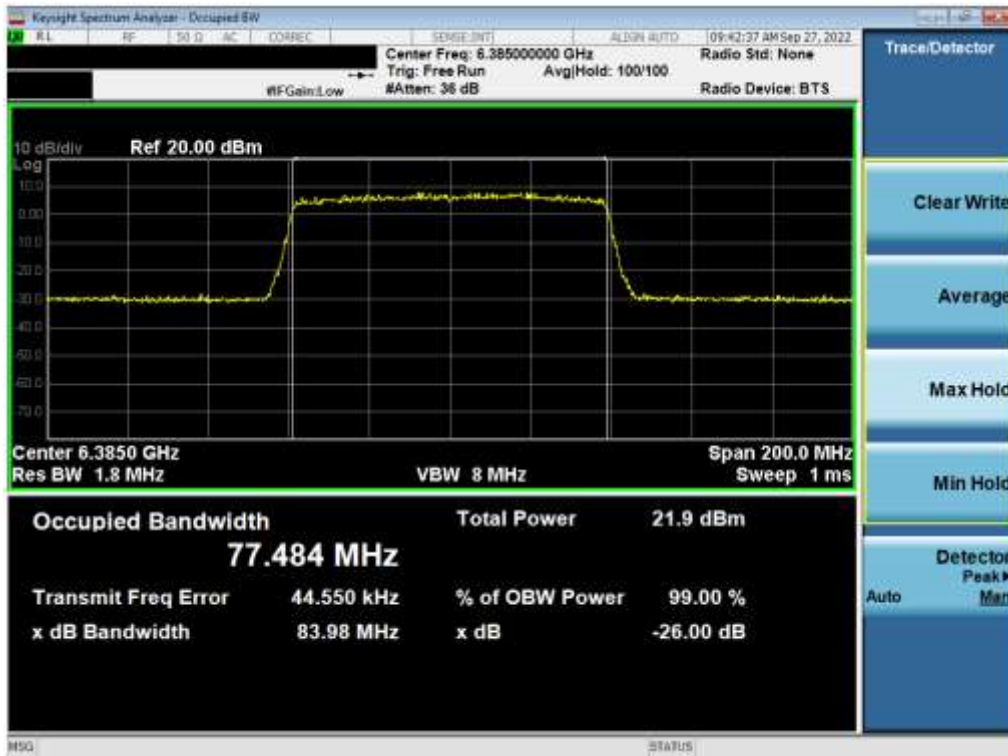
Plot 7-64. 26dB Bandwidth Plot MIMO ANT2 (80MHz 802.11ax (UNII Band 5) – Ch. 87)
