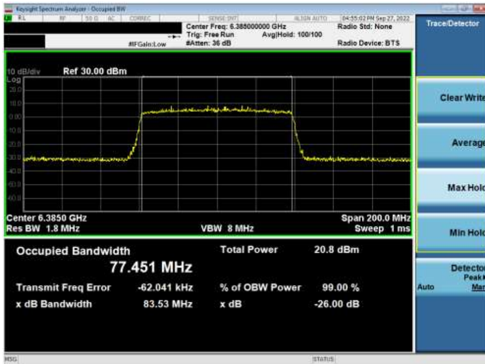
Plot 7-12. 26dB Bandwidth Plot MIMO ANT1 (80MHz 802.11ax (UNII Band 5) – Ch. 87)
