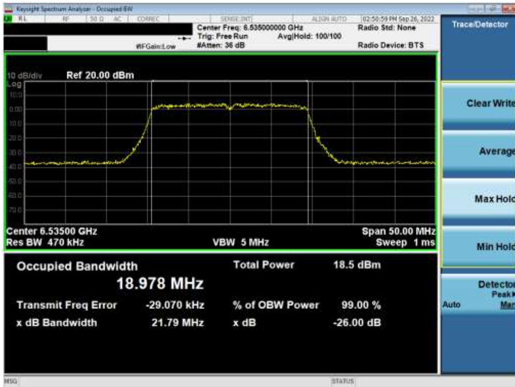
Plot 7-82. 26dB Bandwidth Plot MIMO ANT2 (20MHz 802.11ax (UNII Band 7) – Ch. 117)
