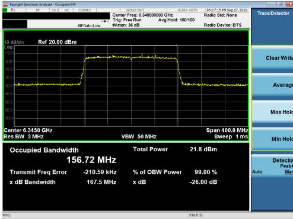
Plot 7-15. 26dB Bandwidth Plot MIMO ANT1 (160MHz 802.11ax (UNII Band 5) – Ch. 79)
