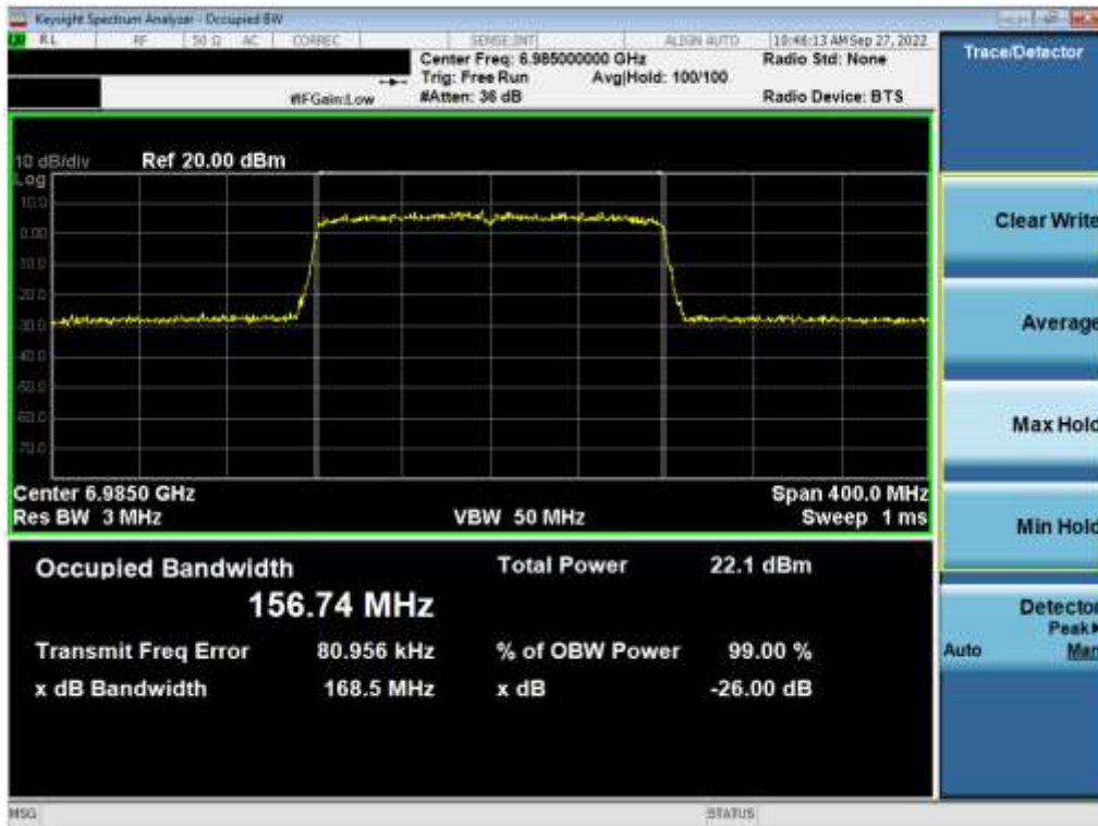
Plot 7-104. 26dB Bandwidth Plot MIMO ANT2 (160MHz 802.11ax (UNII Band 8) – Ch. 207)
