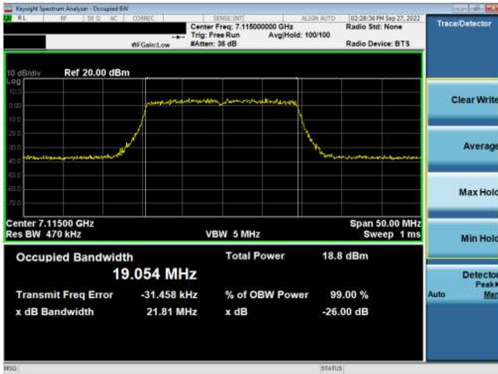
Plot 7-46. 26dB Bandwidth Plot MIMO ANT1 (20MHz 802.11ax (UNII Band 8) – Ch. 233)
