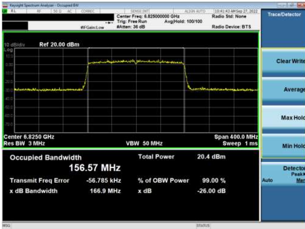
Plot 7-92. 26dB Bandwidth Plot MIMO ANT2 (160MHz 802.11ax (UNII Band 7) – Ch. 175)
