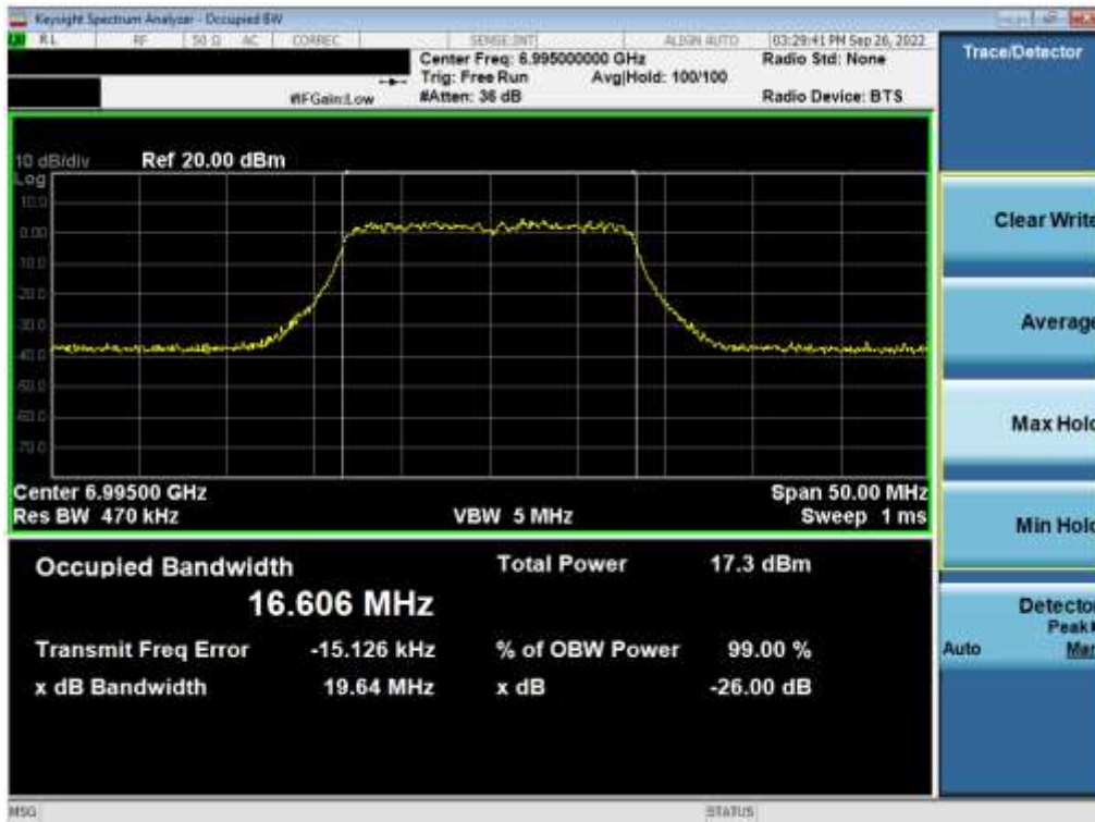
Plot 7-94. 26dB Bandwidth Plot MIMO ANT2 (20MHz 802.11a (UNII Band 8) – Ch. 209)
