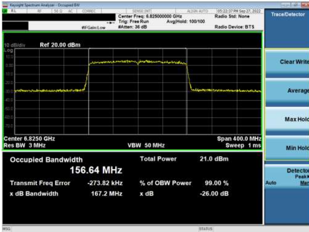
Plot 7-40. 26dB Bandwidth Plot MIMO ANT1 (160MHz 802.11 ax (UNII Band 7) – Ch. 175)
