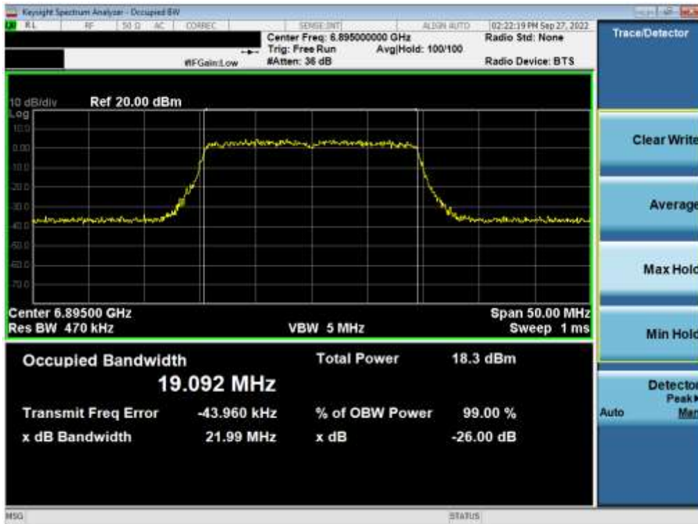
Plot 7-44. 26dB Bandwidth Plot MIMO ANT1 (20MHz 802.11ax (UNII Band 8) – Ch. 189)
