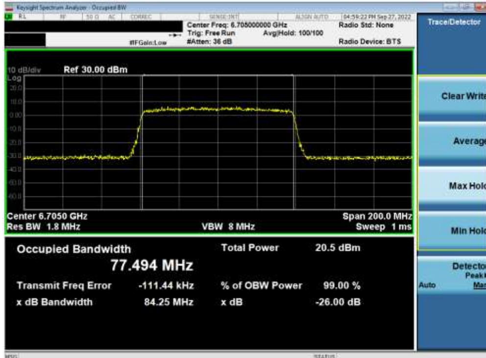
Plot 7-37. 26dB Bandwidth Plot MIMO ANT1 (80MHz 802.11ax (UNII Band 7) – Ch. 151)
