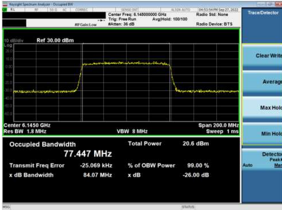
Plot 7-11. 26dB Bandwidth Plot MIMO ANT1 (80MHz 802.11ax (UNII Band 5) – Ch. 39)
