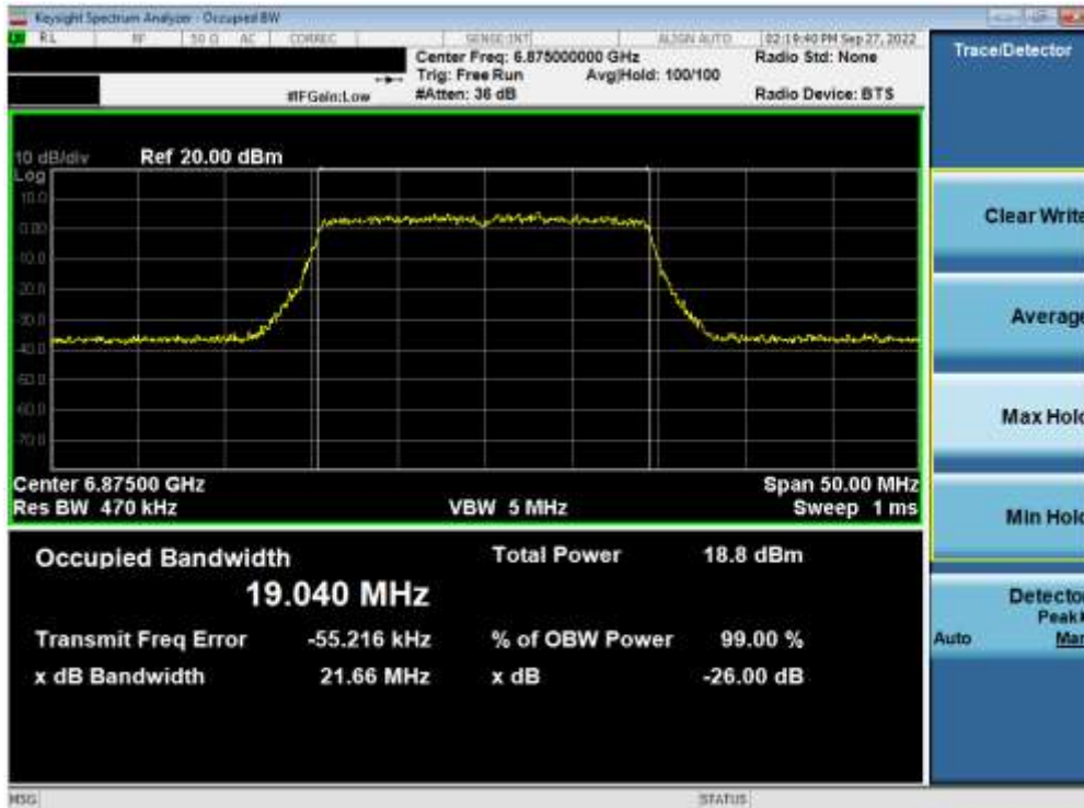
Plot 7-32. 26dB Bandwidth Plot MIMO ANT1 (20MHz 802.11ax (UNII Band 7) – Ch. 185)
