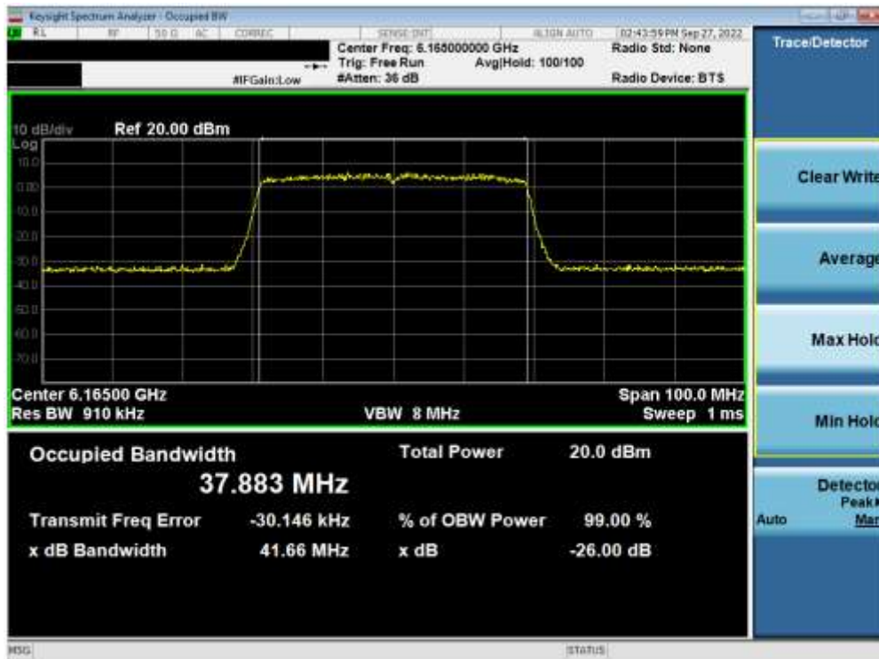
Plot 7-8. 26dB Bandwidth Plot MIMO ANT1 (40MHz 802.11ax (UNII Band 5) – Ch. 43)
