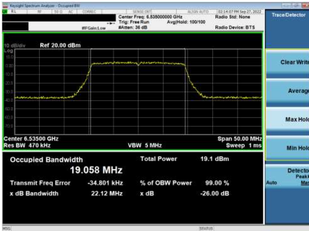
Plot 7-30. 26dB Bandwidth Plot MIMO ANT1 (20MHz 802.11ax (UNII Band 7) – Ch. 117)
