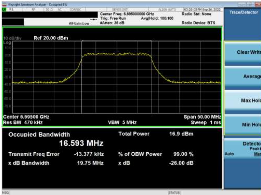
Plot 7-80. 26dB Bandwidth Plot MIMO ANT2 (20MHz 802.11a (UNII Band 7) – Ch. 149)
