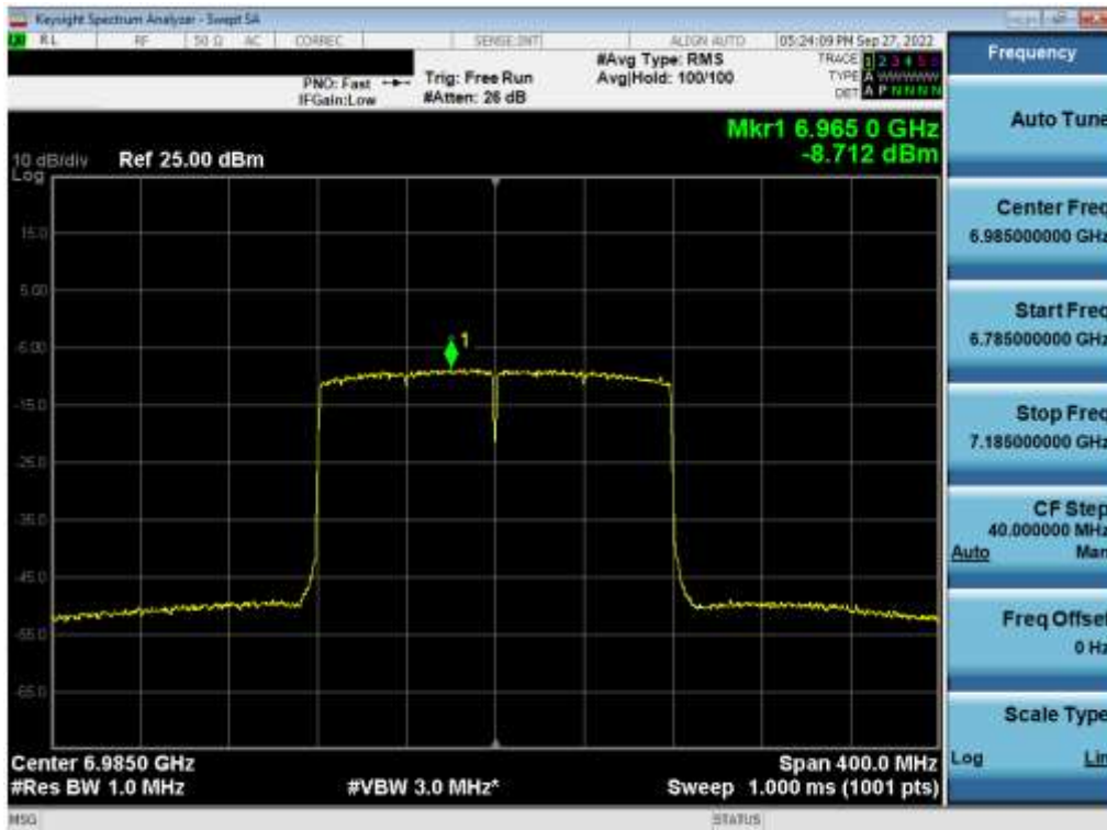
Plot 7-156. Power Spectral Density Measurement MIMO ANT1 (160MHz 802.11ax (UNII Band 8) – Ch. 207)
