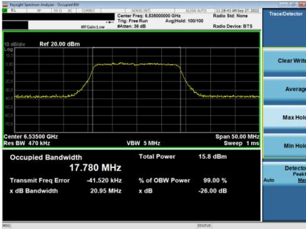
Plot 7-27. 26dB Bandwidth Plot MIMO ANT1 (20MHz 802.11a (UNII Band 7) – Ch. 117)
