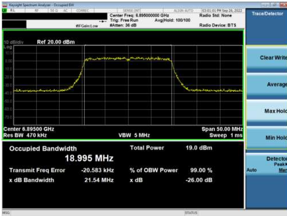
Plot 7-96. 26dB Bandwidth Plot MIMO ANT2 (20MHz 802.11ax (UNII Band 8) – Ch. 189)
