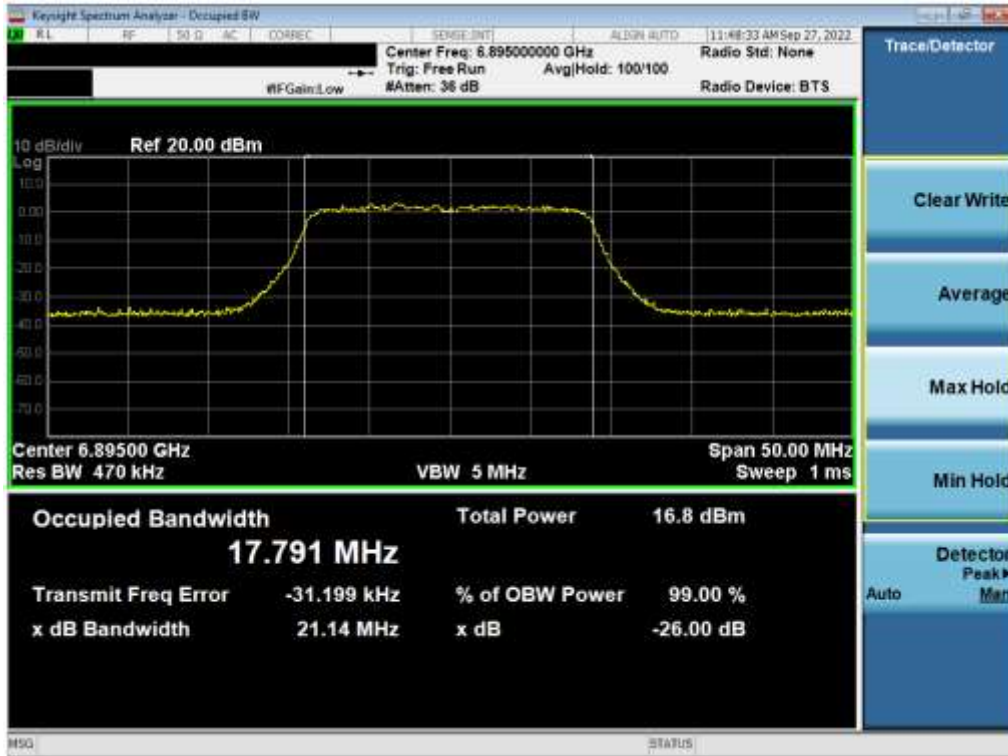
Plot 7-41. 26dB Bandwidth Plot MIMO ANT1 (20MHz 802.11a (UNII Band 8) – Ch. 189)
