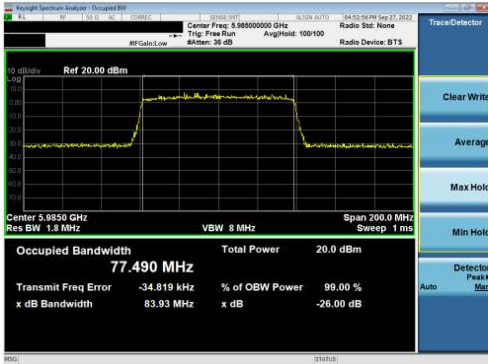
Plot 7-10. 26dB Bandwidth Plot MIMO ANT1 (80MHz 802.11ax (UNII Band 5) – Ch. 7)
