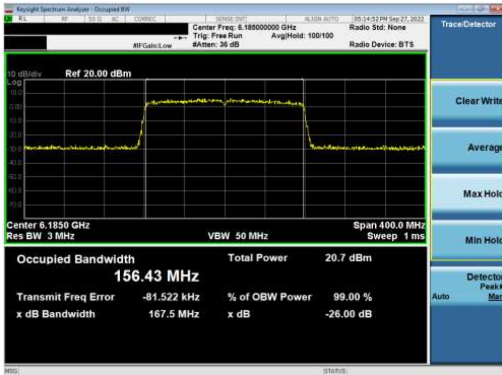
Plot 7-14. 26dB Bandwidth Plot MIMO ANT1 (160MHz 802.11ax (UNII Band 5) – Ch. 47)
