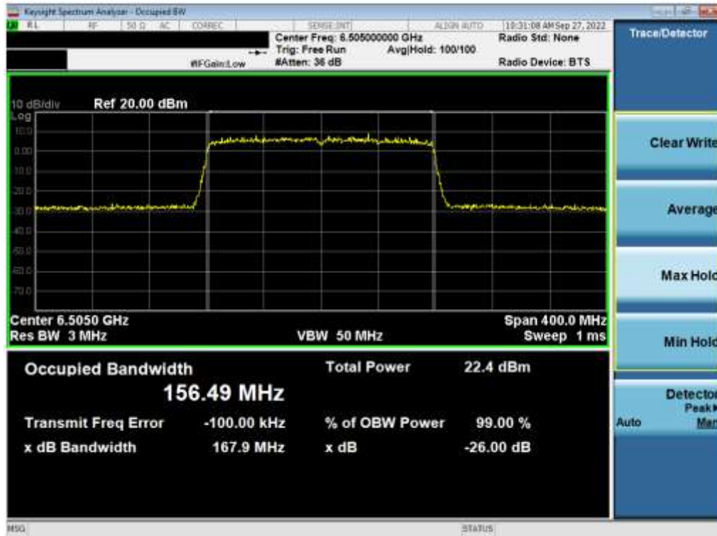
Plot 7-78. 26dB Bandwidth Plot MIMO ANT2 (160MHz 802.11ax (UNII Band 6) – Ch. 111)
