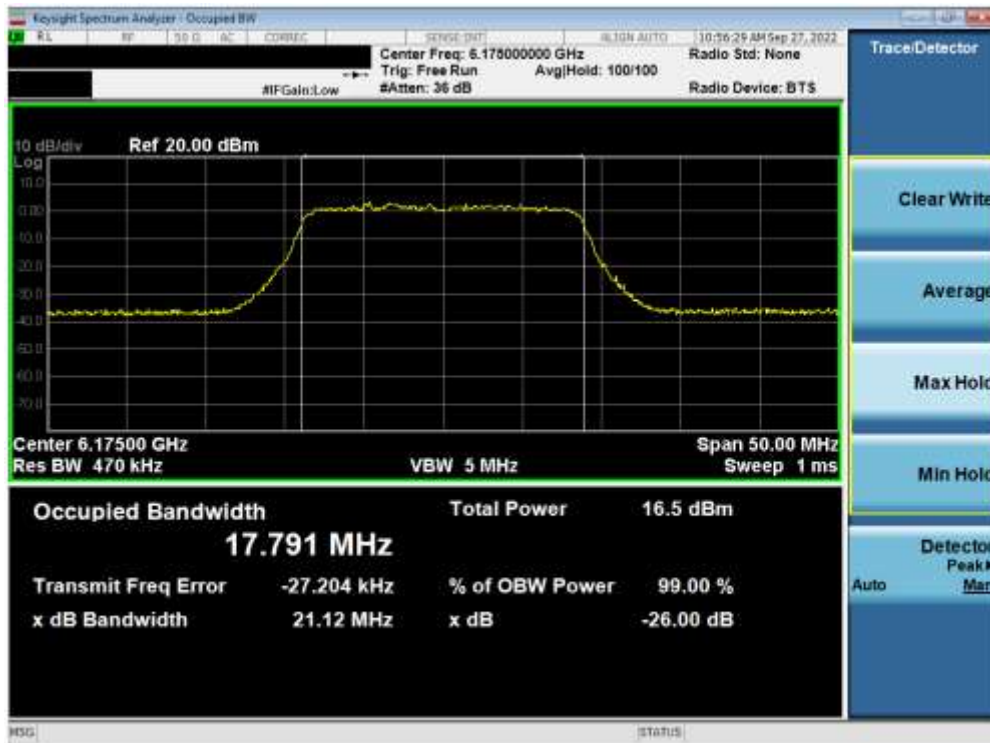
Plot 7-2. 26dB Bandwidth Plot MIMO ANT1 (20MHz 802.11a (UNII Band 5) – Ch. 45)
