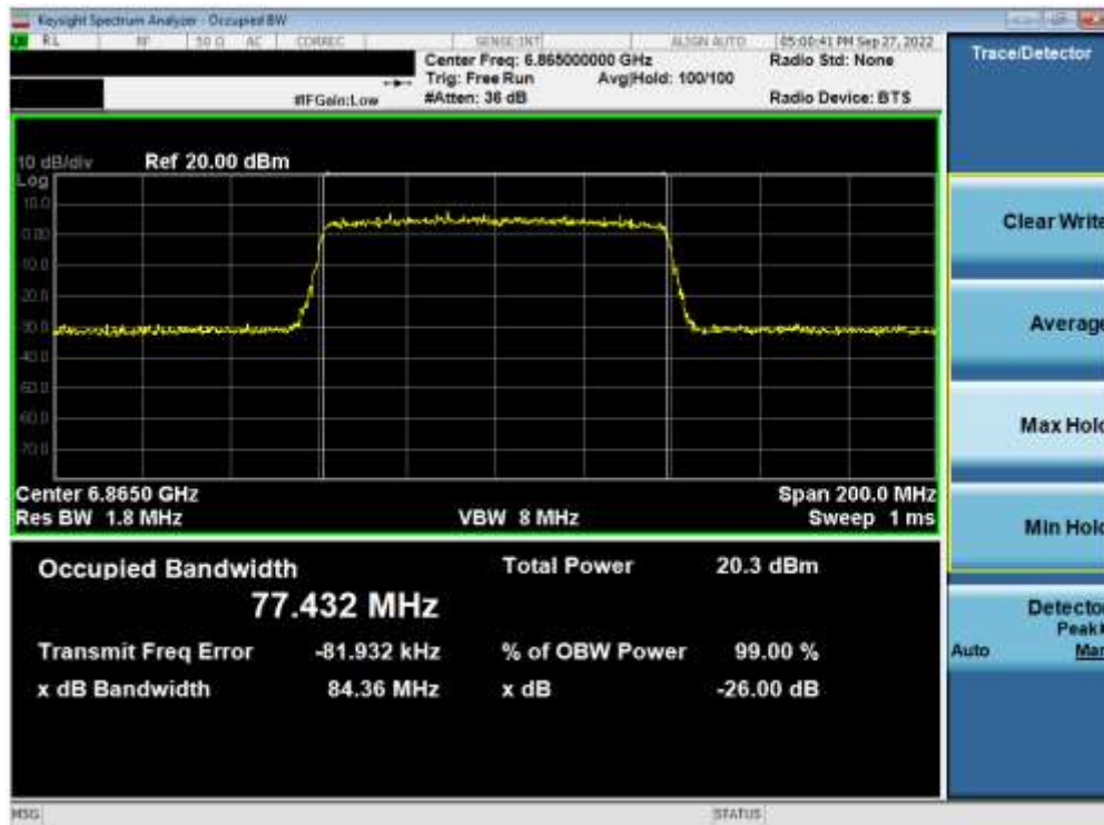
Plot 7-38. 26dB Bandwidth Plot MIMO ANT1 (80MHz 802.11ax (UNII Band 7) – Ch. 183)
