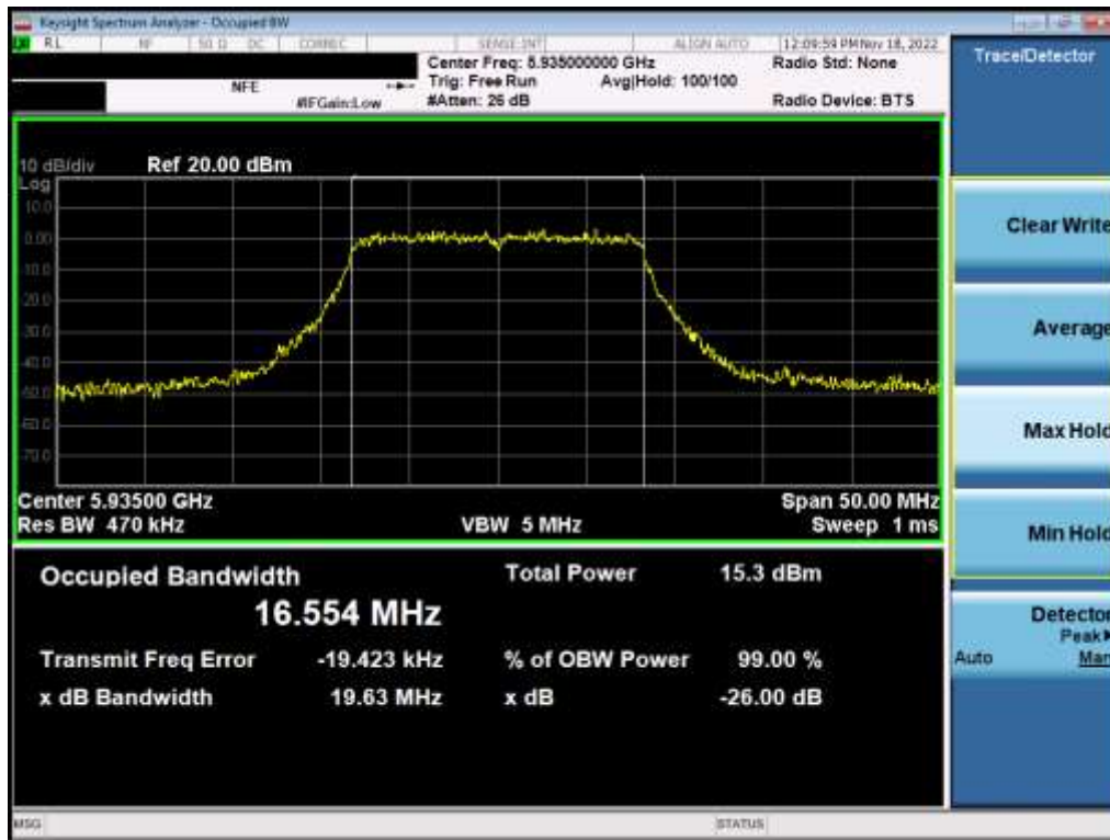
Plot 7-56. 26dB Bandwidth Plot MIMO ANT2 (20MHz 802.11ax (UNII Band 5) – Ch. 2)
