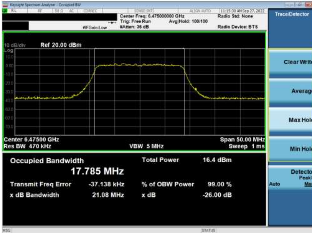
Plot 7-17. 26dB Bandwidth Plot MIMO ANT1 (20MHz 802.11a (UNII Band 6) – Ch. 105)
