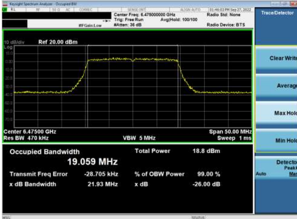
Plot 7-20. 26dB Bandwidth Plot MIMO ANT1 (20MHz 802.11ax (UNII Band 6) – Ch. 105)
