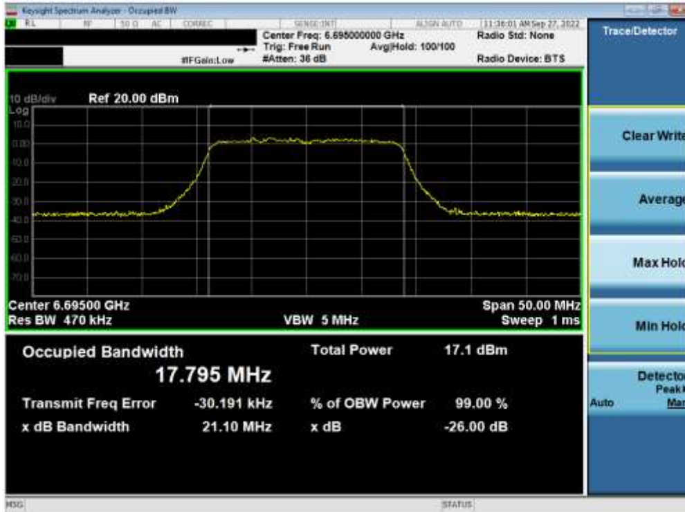
Plot 7-28. 26dB Bandwidth Plot MIMO ANT1 (20MHz 802.11a (UNII Band 7) – Ch. 149)
