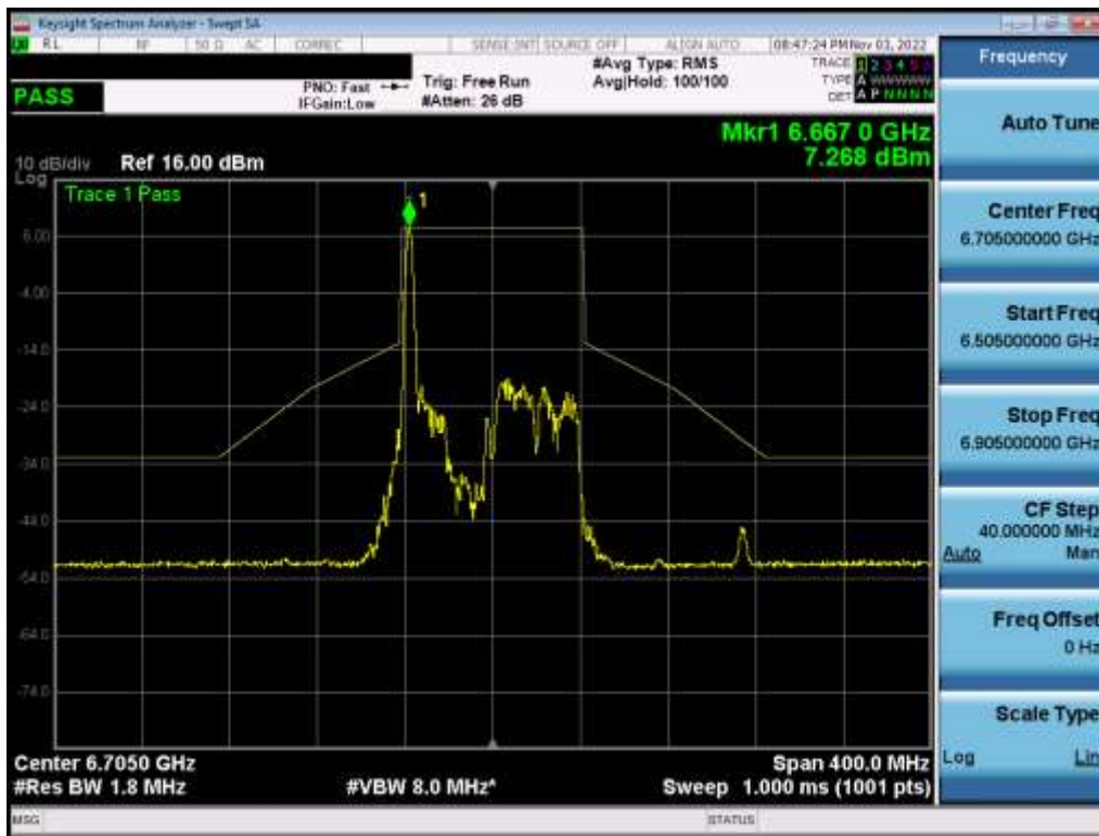
Plot 7-584. In-Band Emission Plot MIMO ANT2 (80MHz BW 802.11ax (26 Tones) (UNII Band 7) – Ch. 151) – SP
