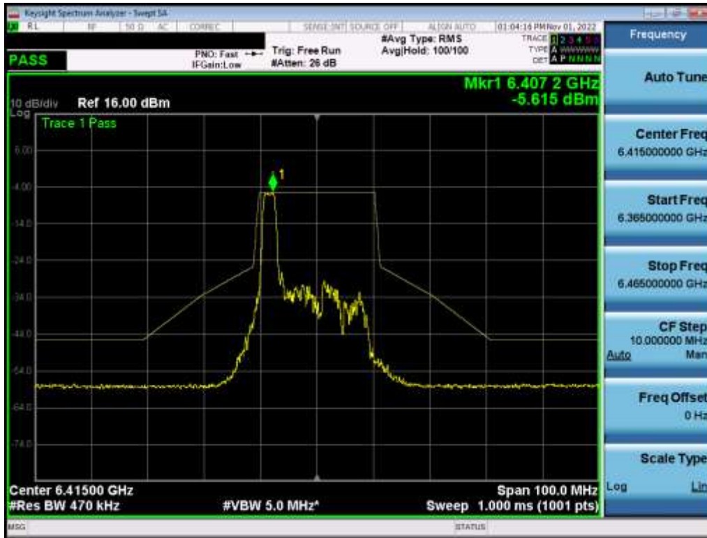
Plot 7-527. In-Band Emission Plot MIMO ANT2 (20MHz BW 802.11ax (26 Tones) UNII Band 5) – Ch. 93) – LPI
