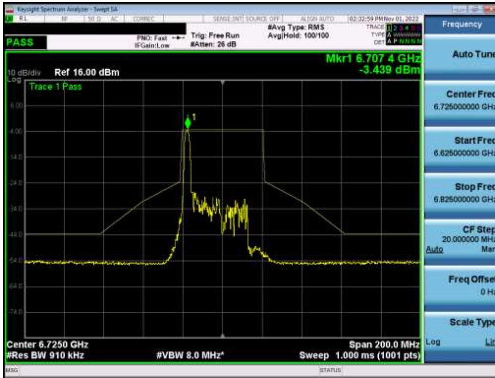
Plot 7-549. In-Band Emission Plot MIMO ANT2 (40MHz BW 802.11ax (26 Tones) (UNII Band 7) – Ch. 155) – LPI
