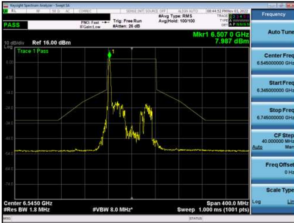
Plot 7-583. In-Band Emission Plot MIMO ANT2 (80MHz BW 802.11ax (26 Tones) (UNII Band 7) – Ch. 119) – SP
