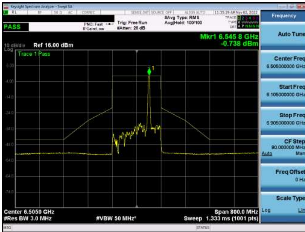
Plot 7-544. In-Band Emission Plot MIMO ANT2 (160MHz BW 802.11ax (26 Tones) (UNII Band 6) – Ch. 111) – LPI
