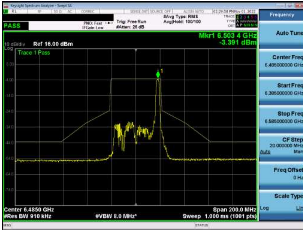
Plot 7-541. In-Band Emission Plot MIMO ANT2 (40MHz BW 802.11ax (26 Tones) (UNII Band 6) – Ch. 107) – LPI
