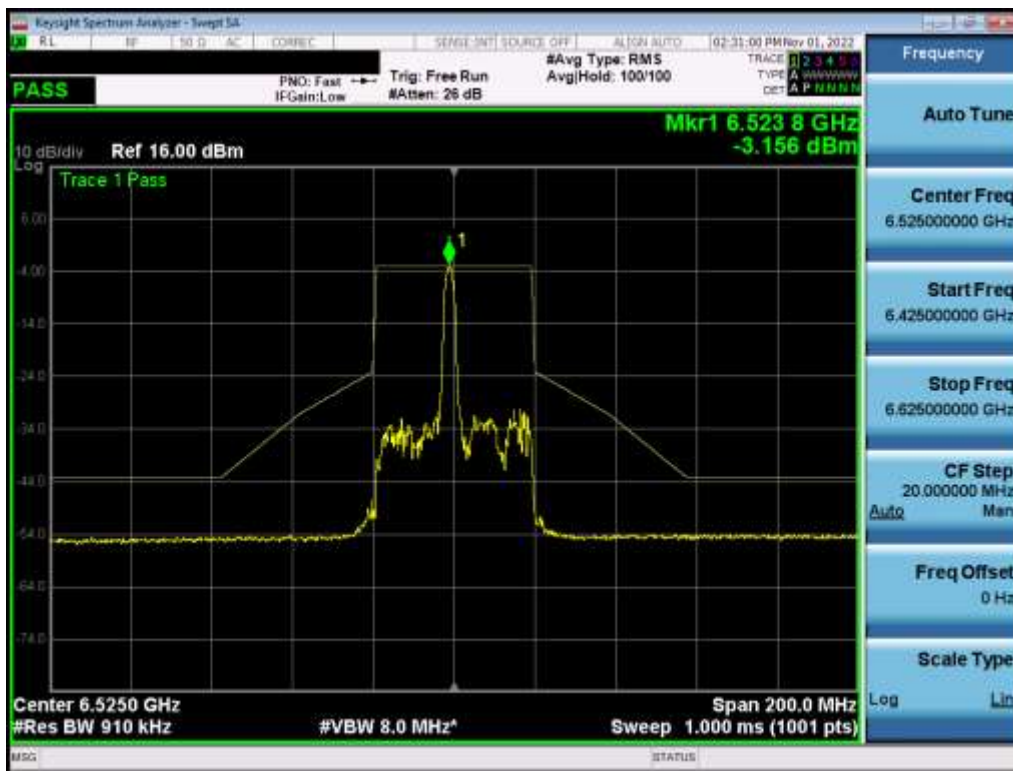
Plot 7-542. In-Band Emission Plot MIMO ANT2 (40MHz BW 802.11ax (26 Tones) (UNII Band 6) – Ch. 115) – LPI
