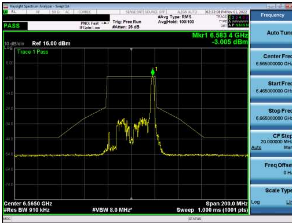
Plot 7-548. In-Band Emission Plot MIMO ANT2 (40MHz BW 802.11ax (26 Tones) (UNII Band 7) – Ch. 123) – LPI
