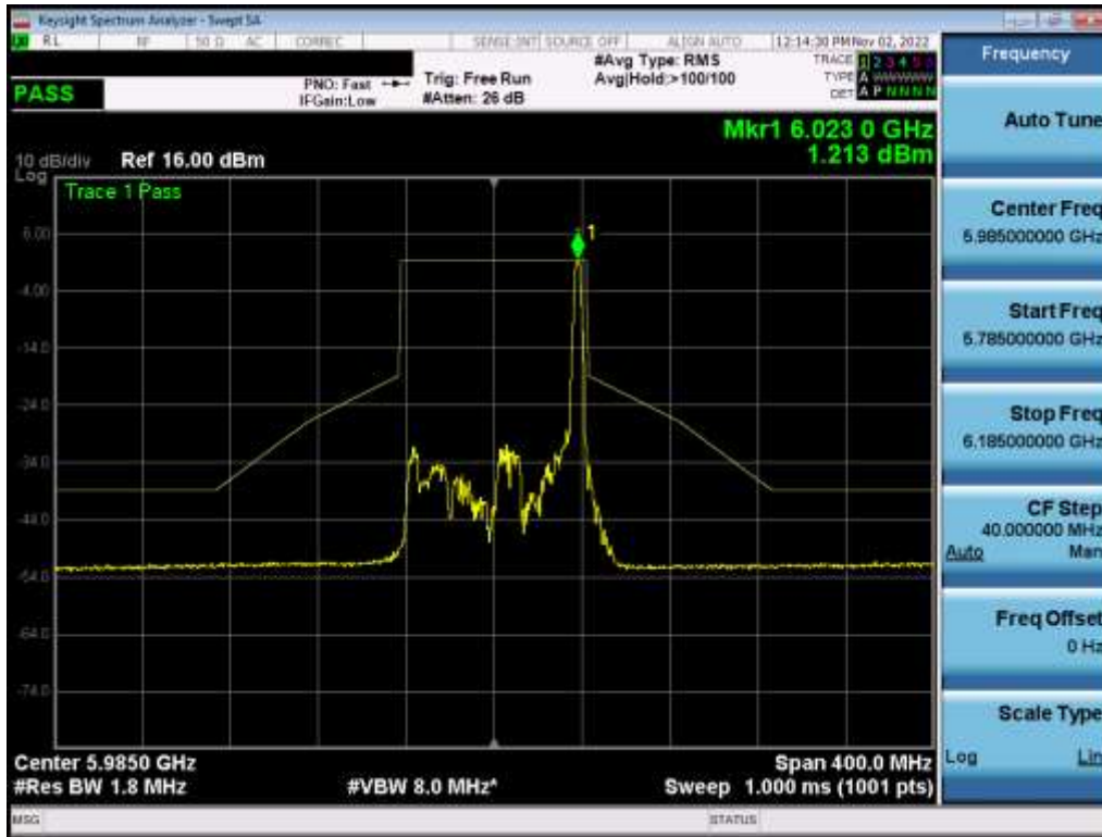
Plot 7-531. In-Band Emission Plot MIMO ANT2 (80MHz BW 802.11ax (26 Tones) (UNII Band 5) – Ch. 7) – LPI
