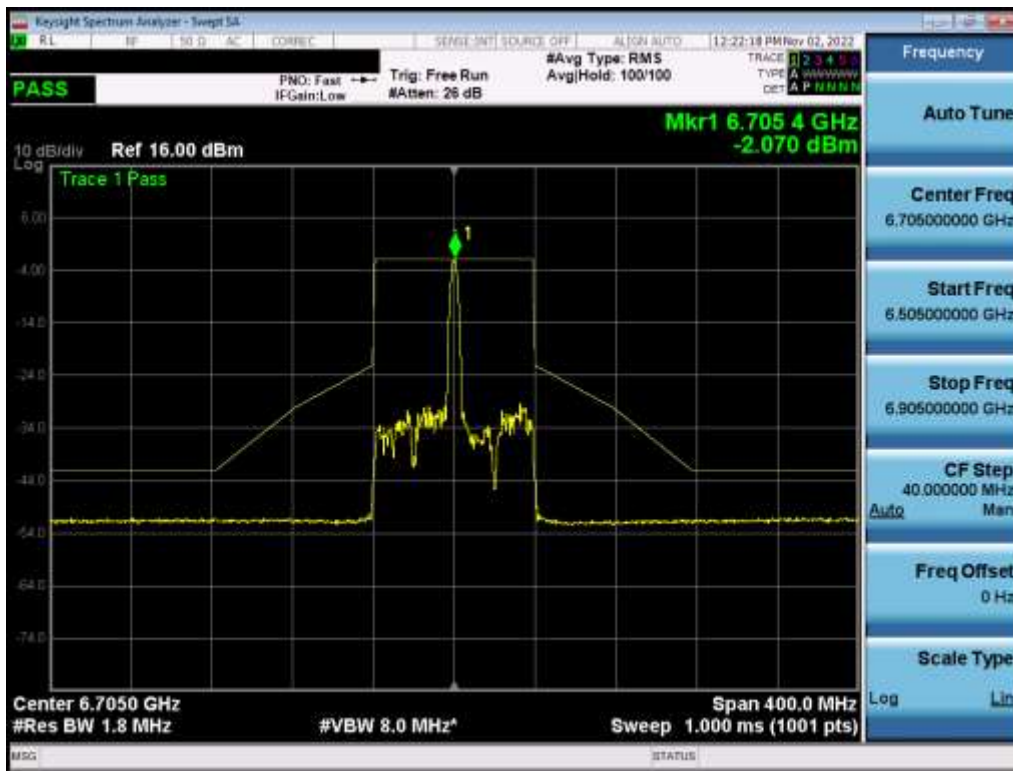
Plot 7-552. In-Band Emission Plot MIMO ANT2 (80MHz BW 802.11ax (26 Tones) (UNII Band 7) – Ch. 151) – LPI
