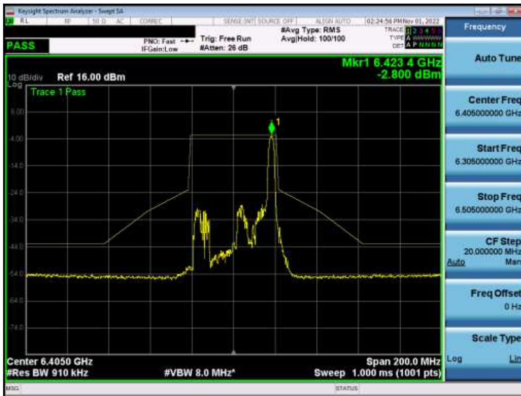
Plot 7-530. In-Band Emission Plot MIMO ANT2 (40MHz BW 802.11ax (26 Tones) (UNII Band 5) – Ch. 91) – LPI
