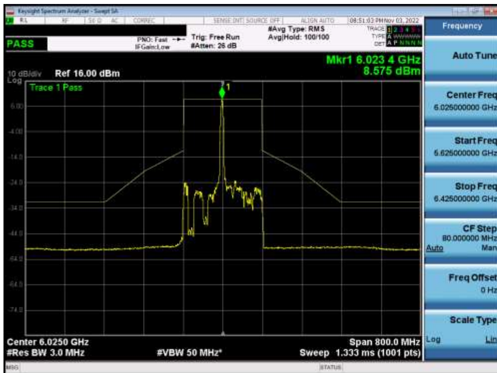
Plot 7-574. In-Band Emission Plot MIMO ANT2 (160MHz BW 802.11ax (26 Tones) (UNII Band 5) – Ch. 15) - SP
