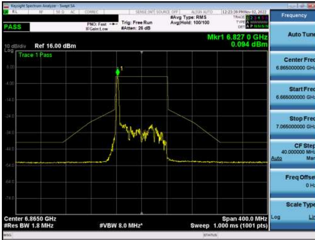
Plot 7-553. In-Band Emission Plot MIMO ANT2 (80MHz BW 802.11ax (26 Tones) (UNII Band 7) – Ch. 183) – LPI
