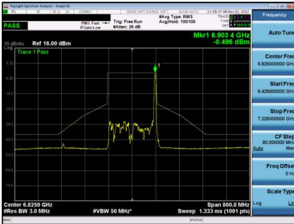
Plot 7-555. In-Band Emission Plot MIMO ANT2 (160MHz BW 802.11ax (26 Tones) (UNII Band 7) – Ch. 175) – LPI
