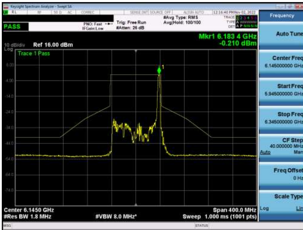
Plot 7-532. In-Band Emission Plot MIMO ANT2 (80MHz BW 802.11ax (26 Tones) (UNII Band 5) – Ch. 39) – LPI
