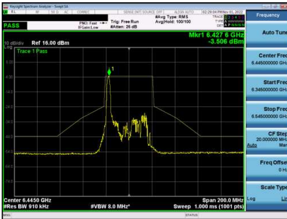
Plot 7-540. In-Band Emission Plot MIMO ANT2 (40MHz BW 802.11ax (26 Tones) (UNII Band 6) – Ch. 99) – LPI
