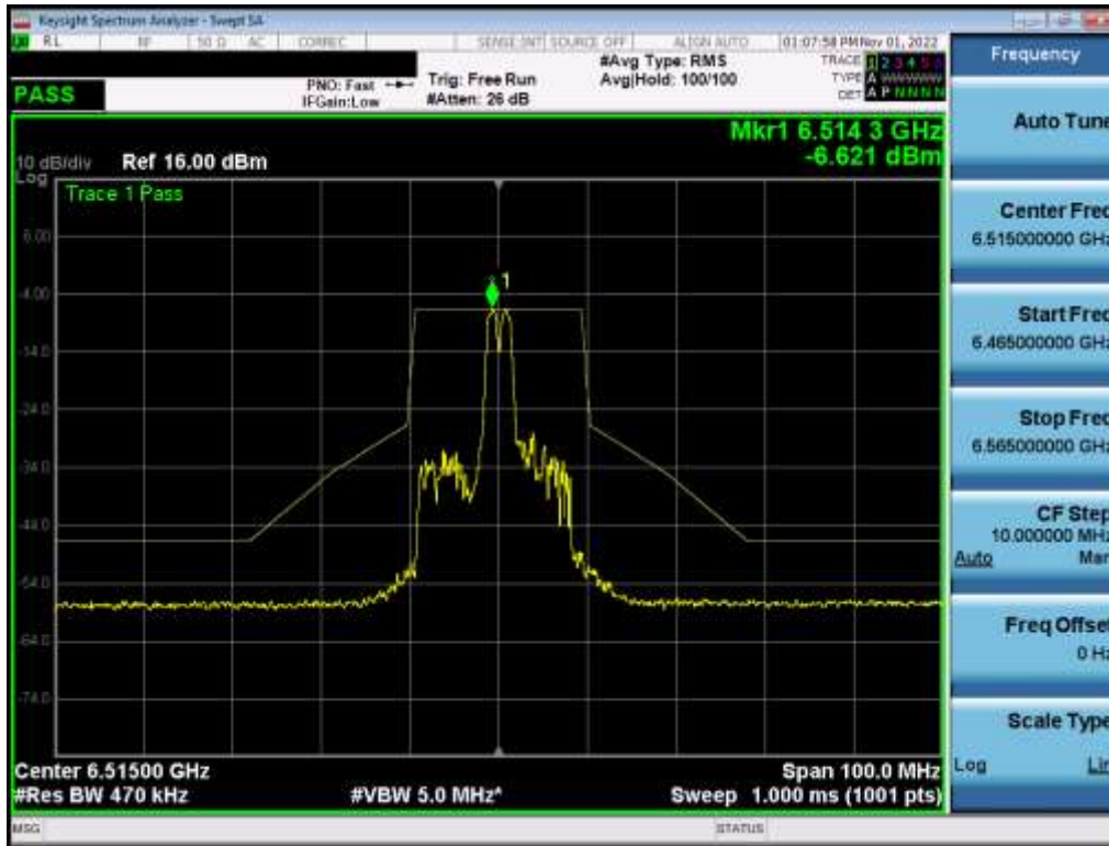
Plot 7-539. In-Band Emission Plot MIMO ANT2 (20MHz BW 802.11ax (26 Tones) (UNII Band 6) – Ch. 113) – LPI
