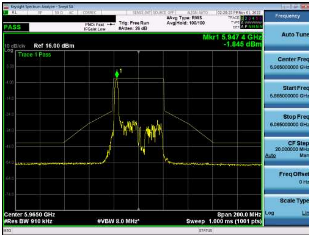
Plot 7-528. In-Band Emission Plot MIMO ANT2 (40MHz BW 802.11ax (26 Tones) (UNII Band 5) – Ch. 3) – LPI
