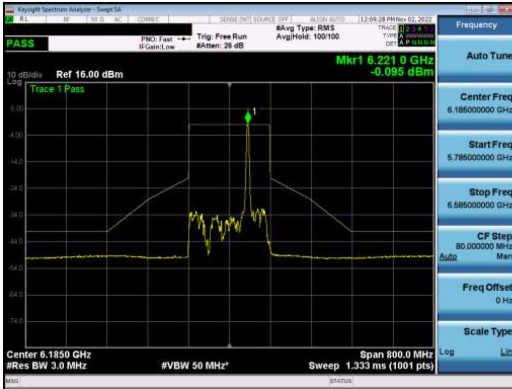
Plot 7-535. In-Band Emission Plot MIMO ANT2 (160MHz BW 802.11ax (26 Tones) (UNII Band 5) – Ch. 47) – LPI
