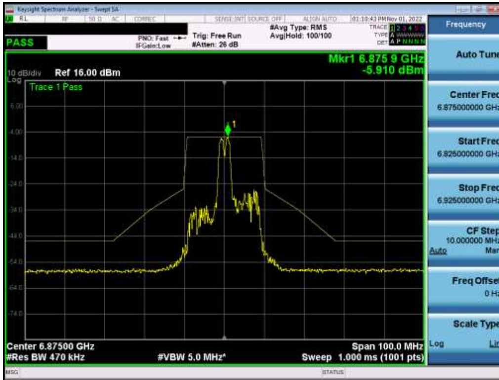
Plot 7-547. In-Band Emission Plot MIMO ANT2 (20MHz BW 802.11ax (26 Tones) (UNII Band 7) – Ch. 185) – LPI
