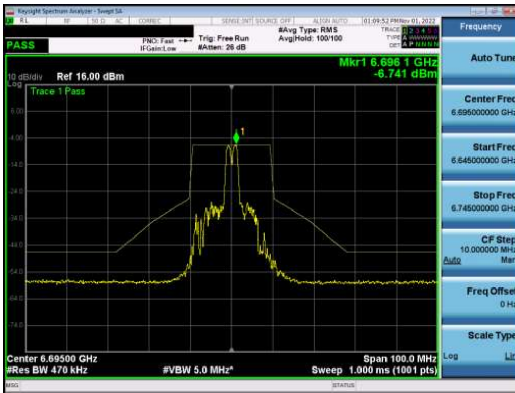
Plot 7-546. In-Band Emission Plot MIMO ANT2 (20MHz BW 802.11ax (26 Tones) (UNII Band 7) – Ch. 149) – LPI
