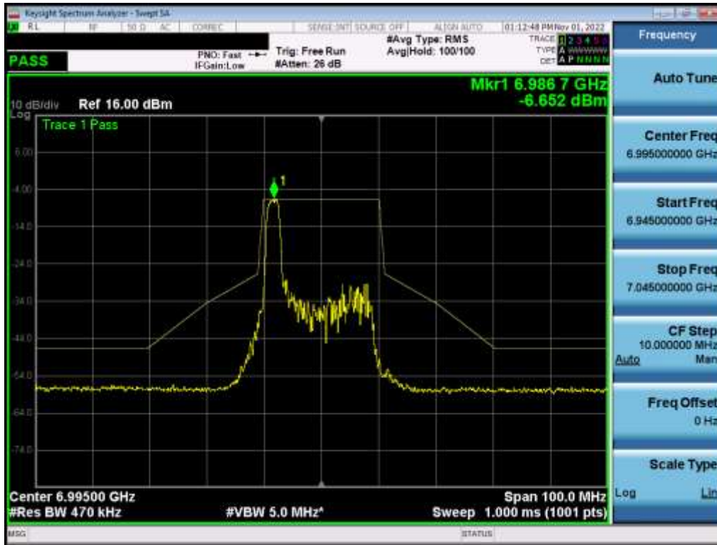
Plot 7-557. In-Band Emission Plot MIMO ANT2 (20MHz BW 802.11ax (26 Tones) (UNII Band 8) – Ch. 209) – LPI
