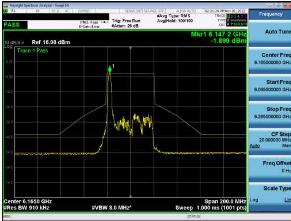
Plot 7-529. In-Band Emission Plot MIMO ANT2 (40MHz BW 802.11ax (26 Tones) (UNII Band 5) – Ch. 43) – LPI
