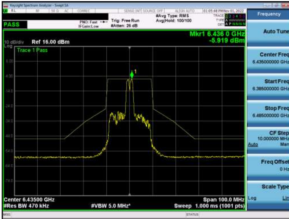
Plot 7-537. In-Band Emission Plot MIMO ANT2 (20MHz BW 802.11ax (26 Tones) (UNII Band 6) – Ch. 97) – LPI
