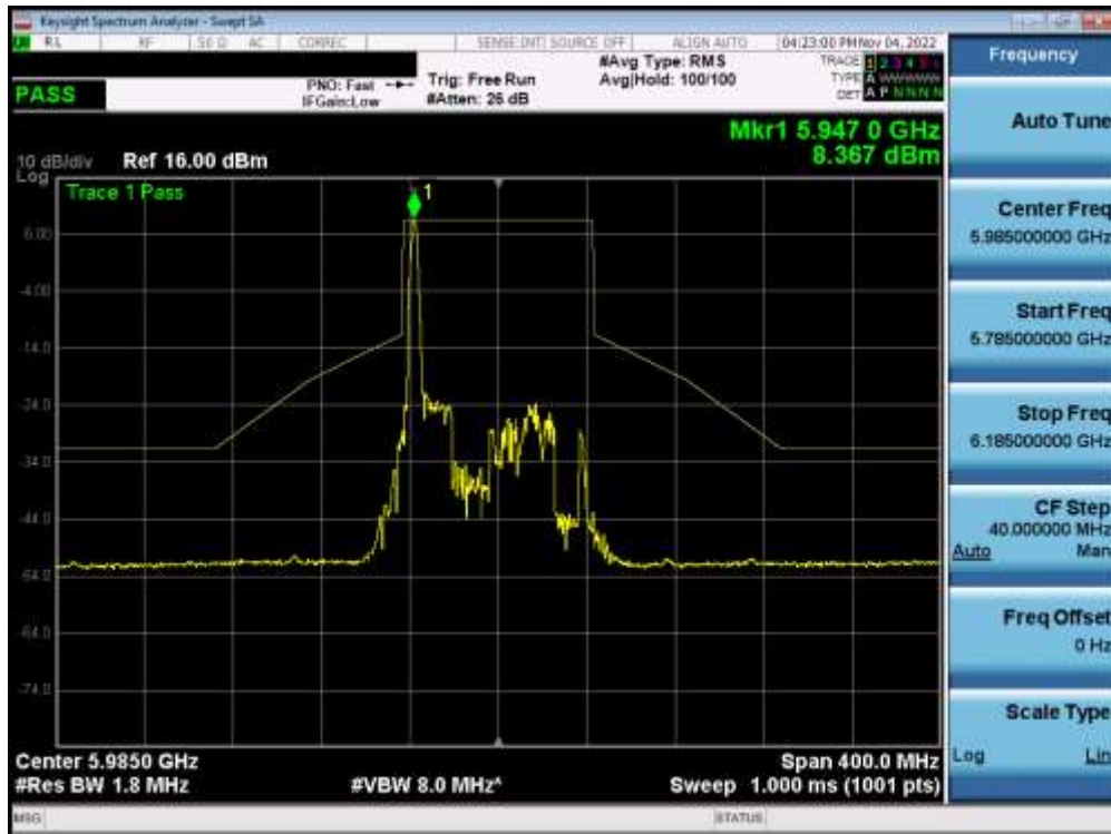
Plot 7-465. In-Band Emission Plot MIMO ANT1 (80MHz BW 802.11ax (26 Tones) (UNII Band 5) – Ch. 7) - SP
