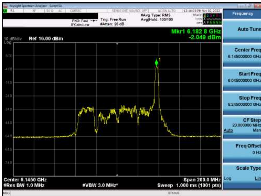
Plot 7-320. Power Spectral Density Plot MIMO ANT2 (80MHz BW 802.11ax (26 Tones) (UNII Band 5) – Ch. 39) – LPI
