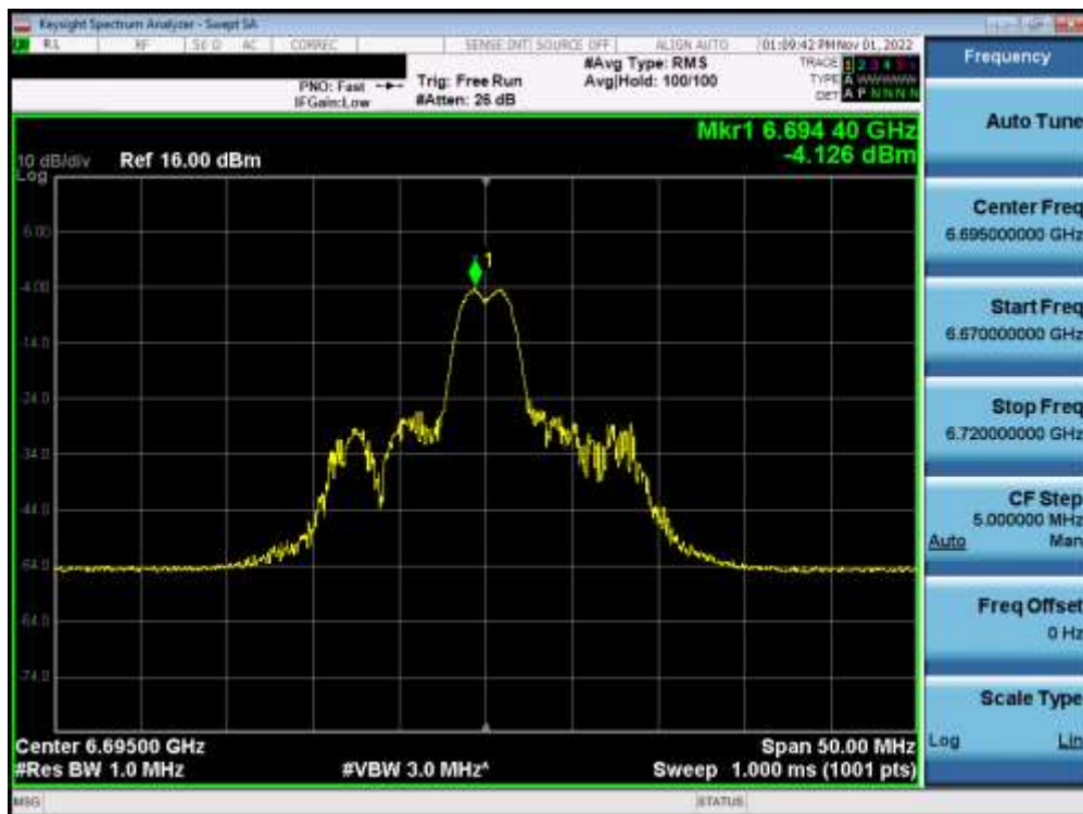
Plot 7-334. Power Spectral Density Plot MIMO ANT2 (20MHz BW 802.11ax (26 Tones) (UNII Band 7) – Ch. 149) – LPI
