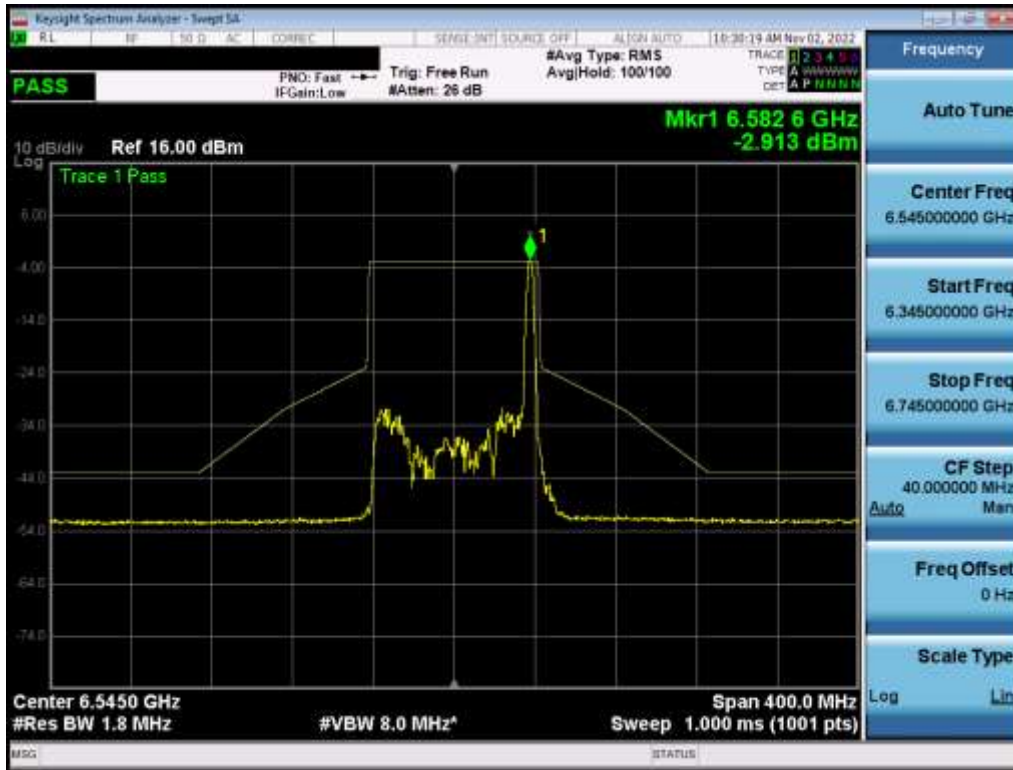
Plot 7-445. In-Band Emission Plot MIMO ANT1 (80MHz BW 802.11ax (26 Tones) (UNII Band 7) – Ch. 119) – LPI
