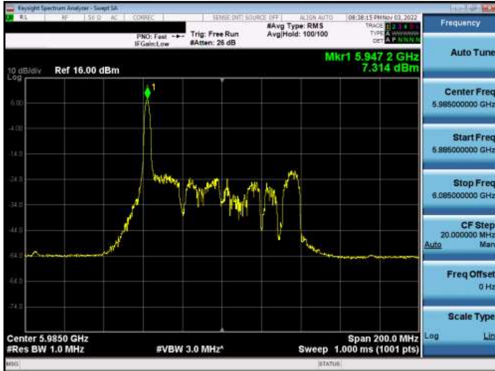
Plot 7-359. Power Spectral Density Plot MIMO ANT2 (80MHz BW 802.11ax (26 Tones) (UNII Band 5) – Ch. 7) – SP
