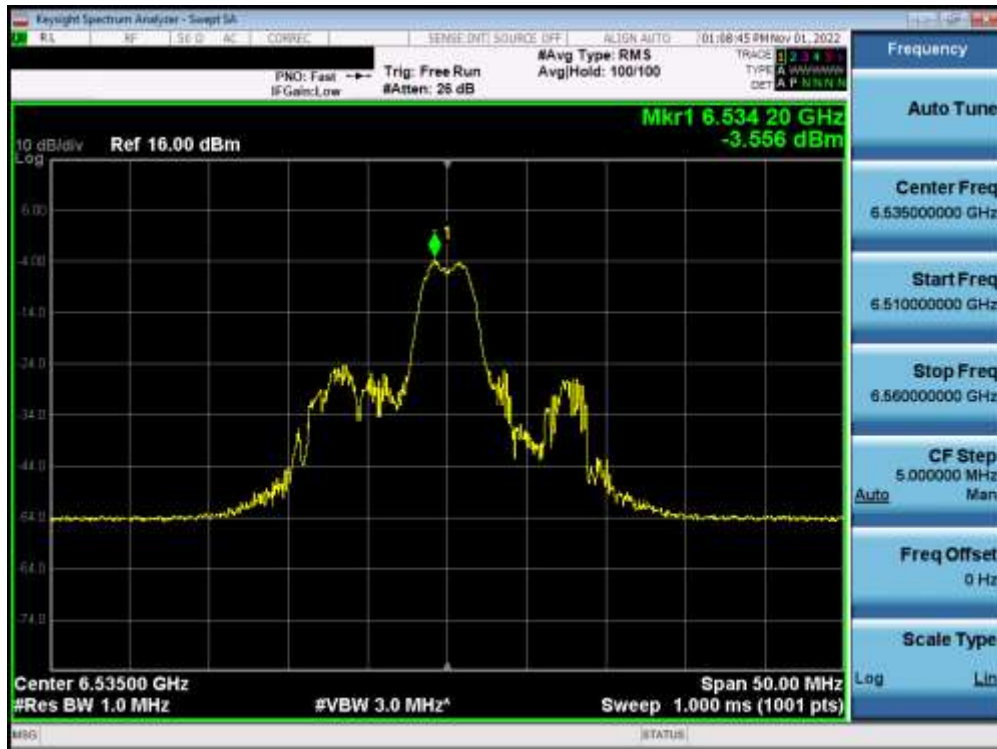
Plot 7-333. Power Spectral Density Plot MIMO ANT2 (20MHz BW 802.11ax (26 Tones) (UNII Band 7) – Ch. 117) – LPI
