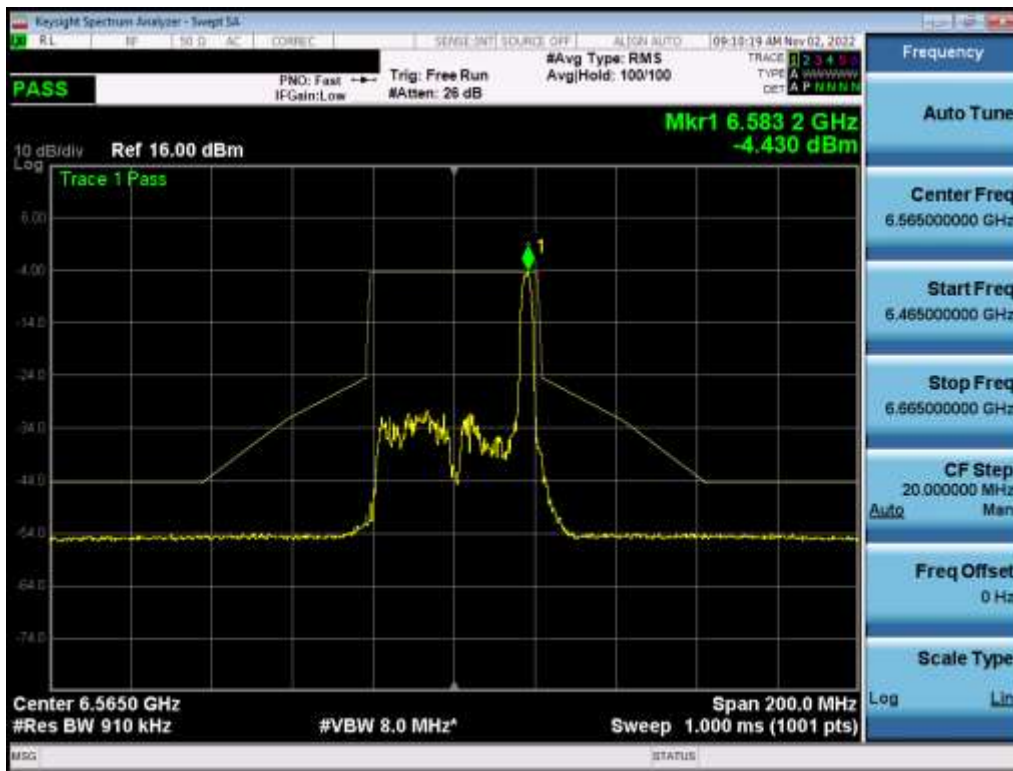
Plot 7-442. In-Band Emission Plot MIMO ANT1 (40MHz BW 802.11ax (26 Tones) (UNII Band 7) – Ch. 123) – LPI
