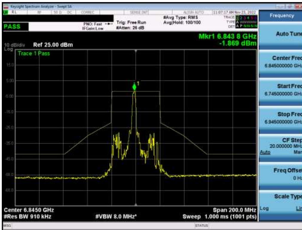
Plot 7-444. In-Band Emission Plot MIMO ANT1 (40MHz BW 802.11ax (26 Tones) (UNII Band 7) – Ch. 179) – LPI
