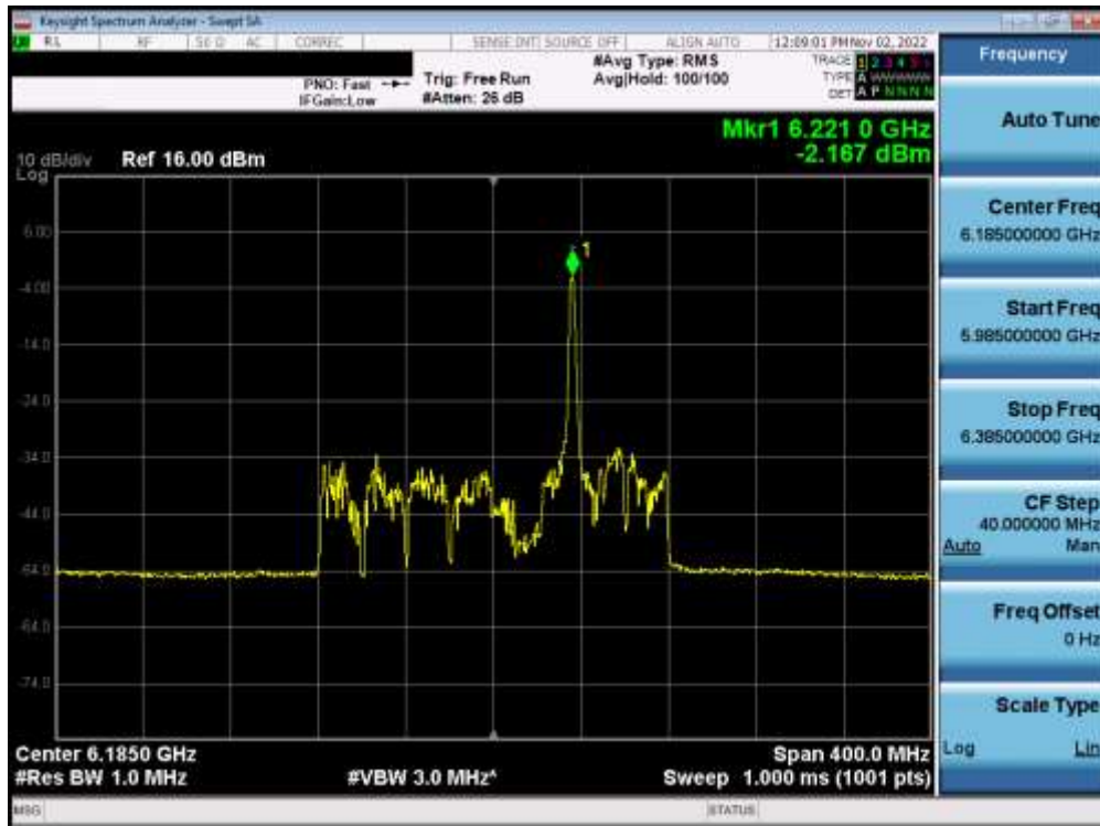
Plot 7-323. Power Spectral Density Plot MIMO ANT2 (160MHz BW 802.11ax (26 Tones) (UNII Band 5) – Ch. 47) – LPI
