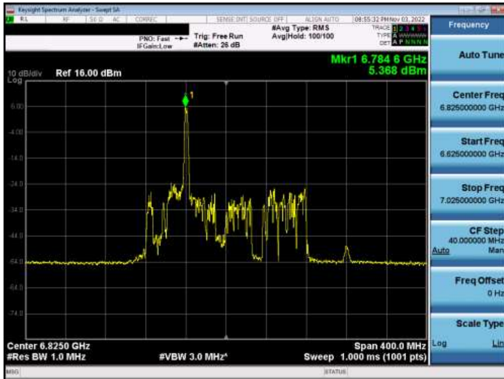
Plot 7-375. Power Spectral Density Plot MIMO ANT2 (160MHz BW 802.11ax (26 Tones) (UNII Band 7) – Ch. 175) – SP
