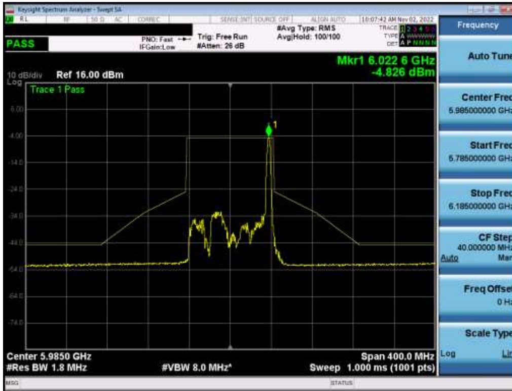
Plot 7-425. In-Band Emission Plot MIMO ANT1 (80MHz BW 802.11ax (26 Tones) (UNII Band 5) – Ch. 7) – LPI
