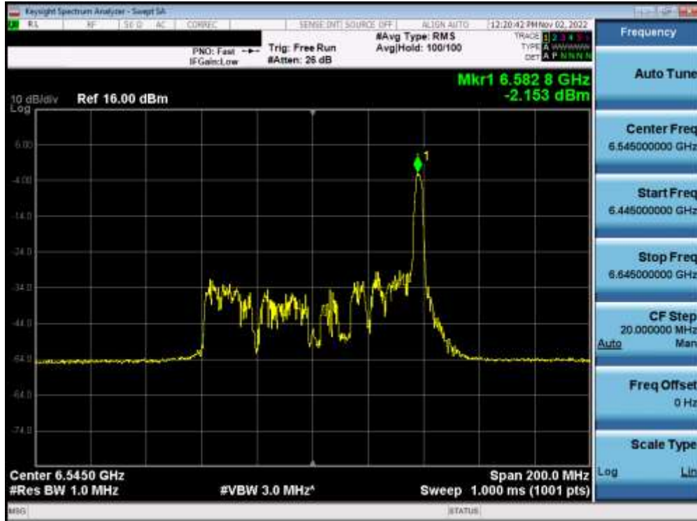
Plot 7-339. Power Spectral Density Plot MIMO ANT2 (80MHz BW 802.11ax (26 Tones) (UNII Band 7) – Ch. 119) – LPI
