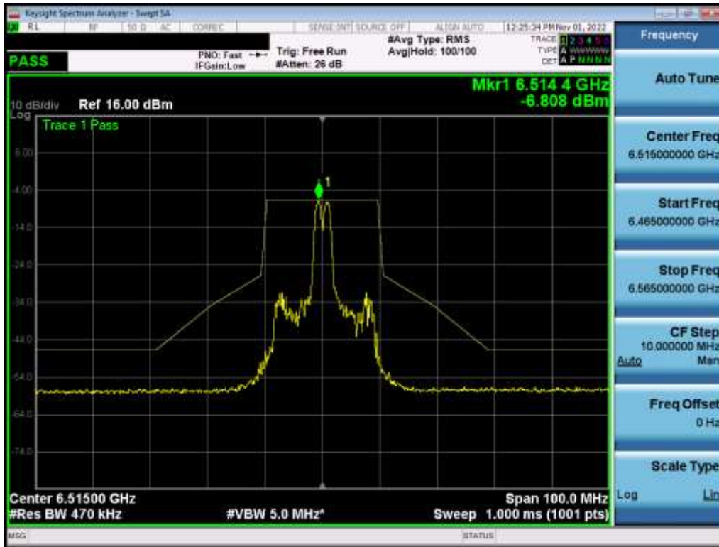
Plot 7-433. In-Band Emission Plot MIMO ANT1 (20MHz BW 802.11ax (26 Tones) (UNII Band 6) – Ch. 113) – LPI
