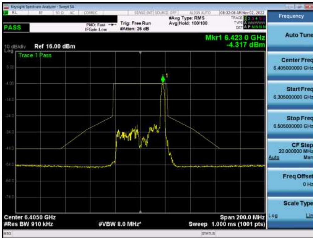
Plot 7-424. In-Band Emission Plot MIMO ANT1 (40MHz BW 802.11ax (26 Tones) (UNII Band 5) – Ch. 91) – LPI
