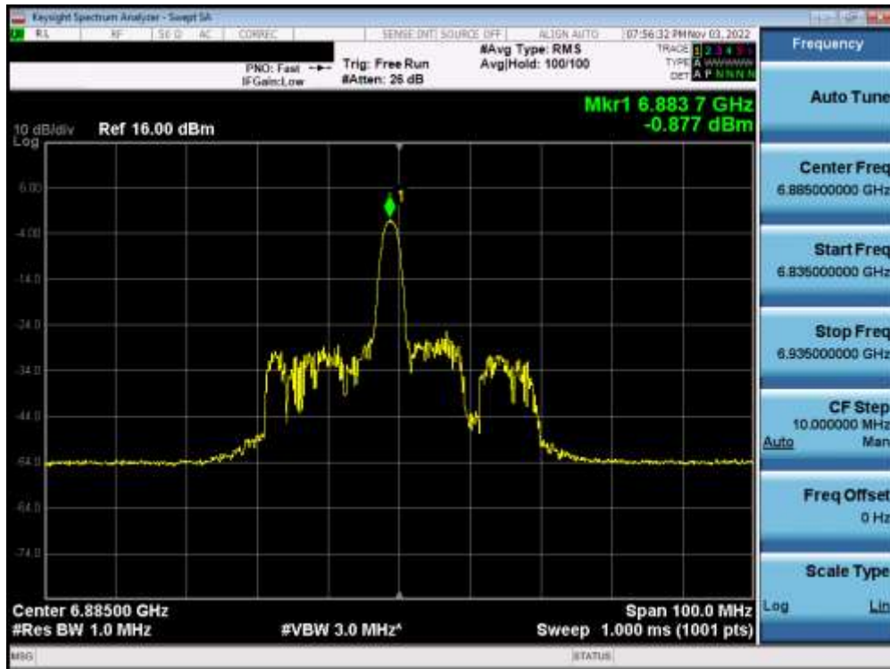
Plot 7-347. Power Spectral Density Plot MIMO ANT2 (40MHz BW 802.11ax (26 Tones) (UNII Band 8) – Ch. 187) – LPI
