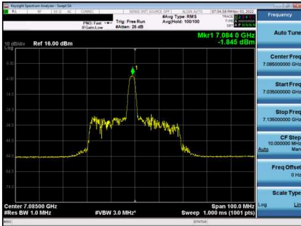
Plot 7-349. Power Spectral Density Plot MIMO ANT2 (40MHz BW 802.11ax (26 Tones) (UNII Band 8) – Ch. 227) – LPI
