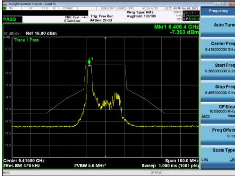
Plot 7-421. In-Band Emission Plot MIMO ANT1 (20MHz BW 802.11ax (26 Tones) UNII Band 5) – Ch. 93) – LPI
