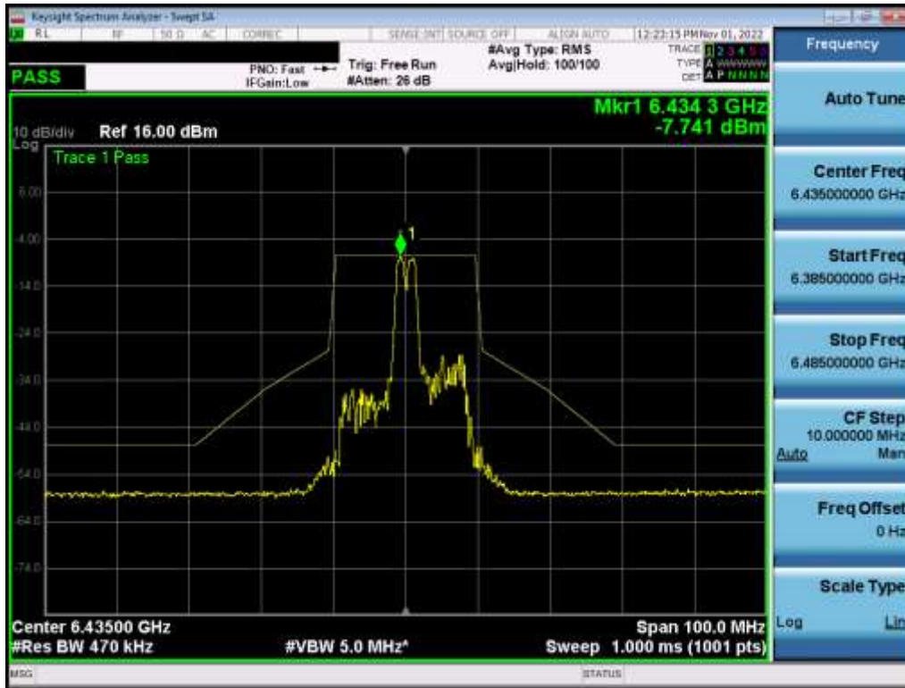
Plot 7-431. In-Band Emission Plot MIMO ANT1 (20MHz BW 802.11ax (26 Tones) (UNII Band 6) – Ch. 97) – LPI
