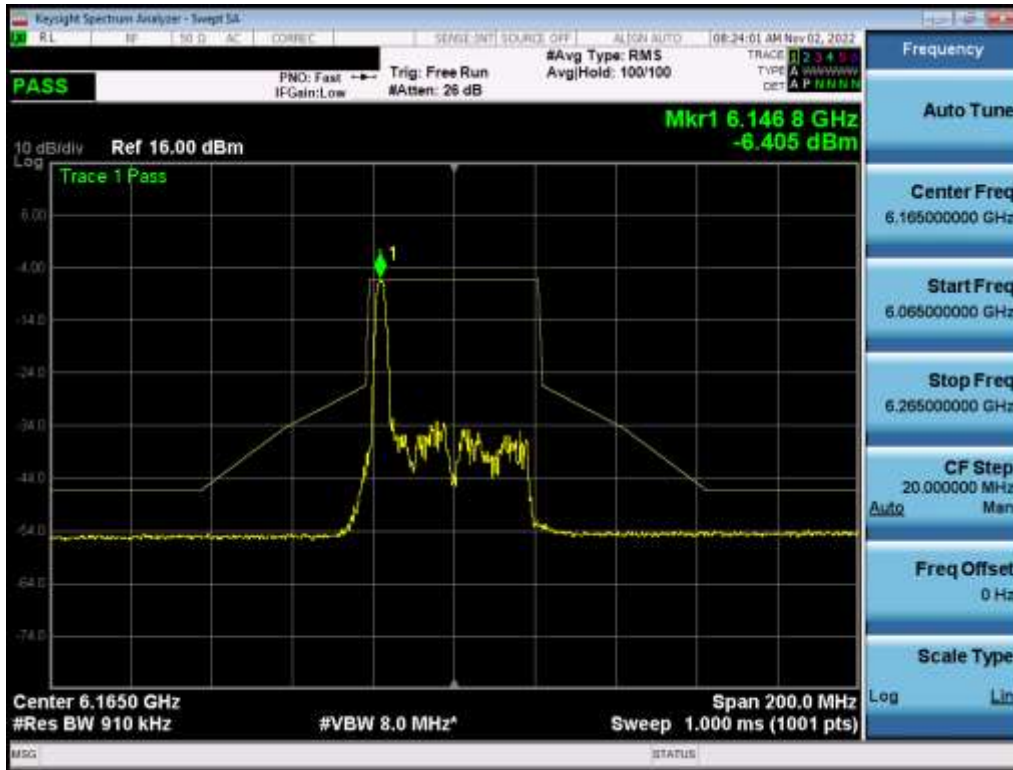
Plot 7-423. In-Band Emission Plot MIMO ANT1 (40MHz BW 802.11ax (26 Tones) (UNII Band 5) – Ch. 43) – LPI
