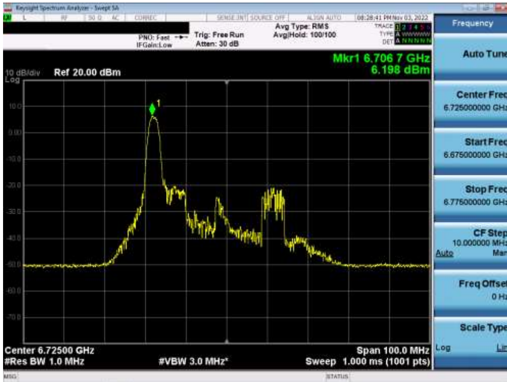
Plot 7-369. Power Spectral Density Plot MIMO ANT2 (40MHz BW 802.11ax (26 Tones) (UNII Band 7) – Ch. 155) – SP
