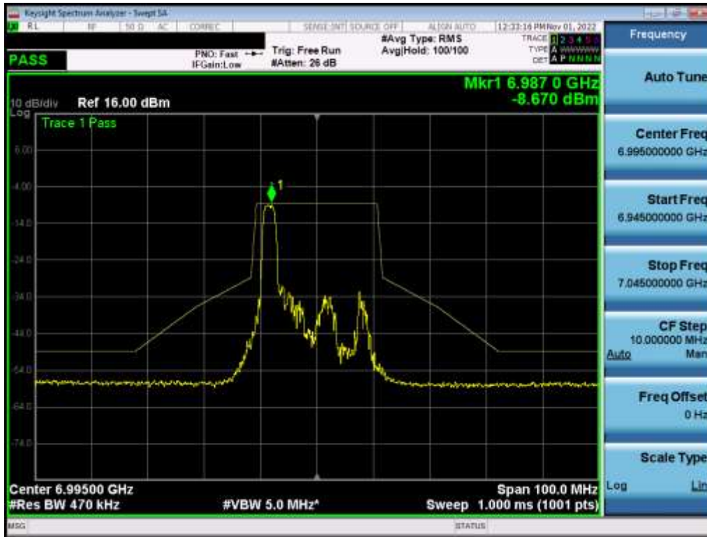
Plot 7-451. In-Band Emission Plot MIMO ANT1 (20MHz BW 802.11ax (26 Tones) (UNII Band 8) – Ch. 209) – LPI
