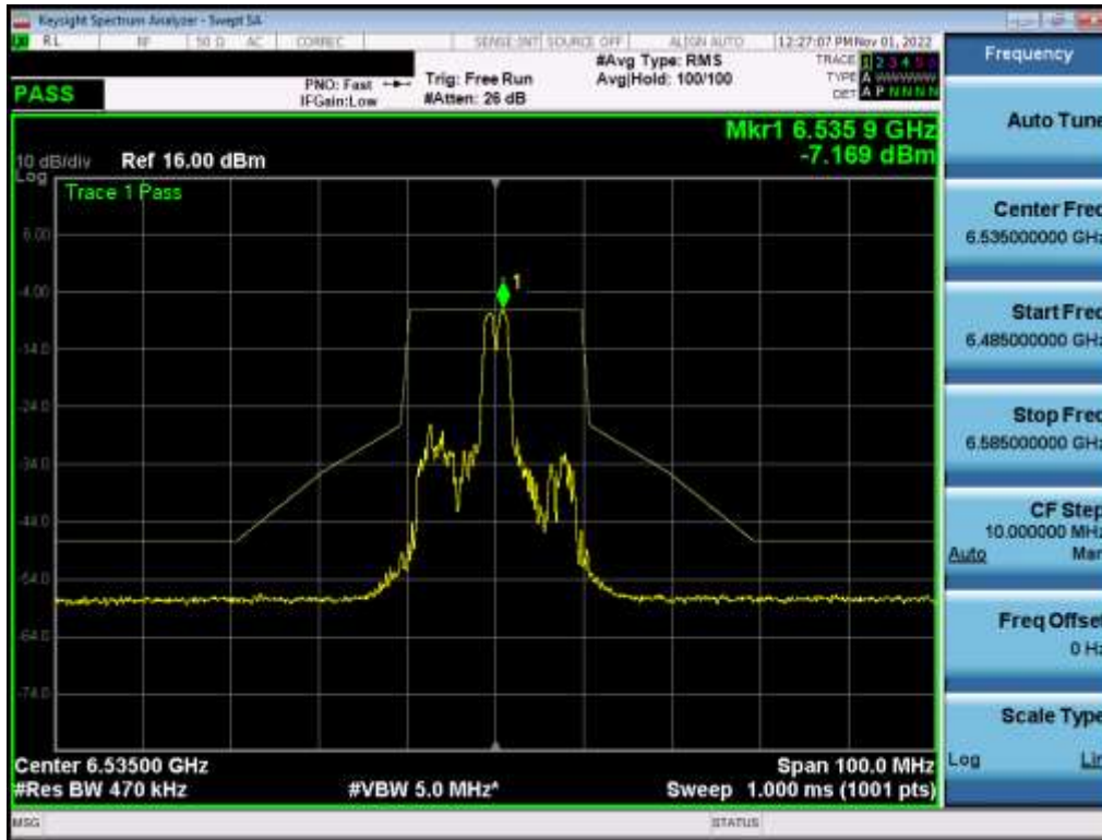
Plot 7-439. In-Band Emission Plot MIMO ANT1 (20MHz BW 802.11ax (26 Tones) (UNII Band 7) – Ch. 117) – LPI
