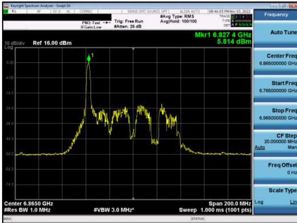
Plot 7-373. Power Spectral Density Plot MIMO ANT2 (80MHz BW 802.11ax (26 Tones) (UNII Band 7) – Ch. 183) – SP
