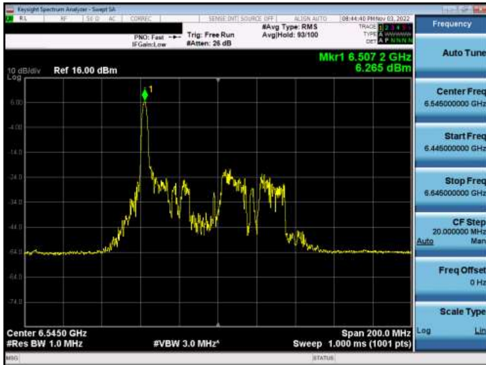
Plot 7-371. Power Spectral Density Plot MIMO ANT2 (80MHz BW 802.11ax (26 Tones) (UNII Band 7) – Ch. 119) – SP
