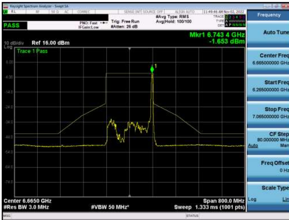
Plot 7-448. In-Band Emission Plot MIMO ANT1 (160MHz BW 802.11ax (26 Tones) (UNII Band 7) – Ch. 143) – LPI
