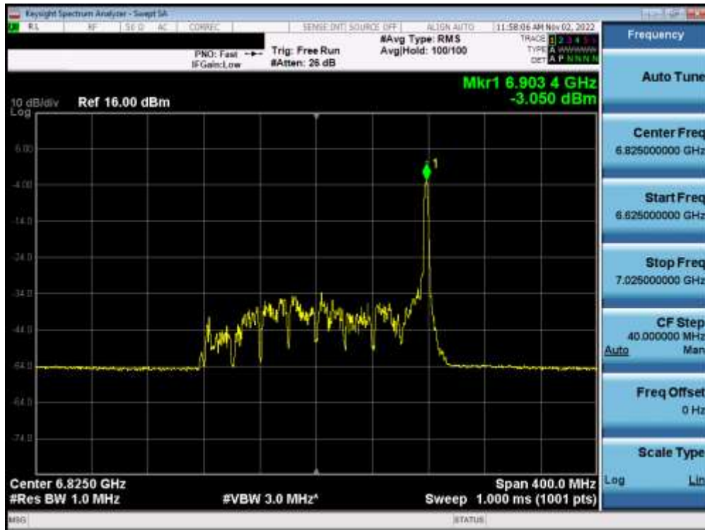
Plot 7-343. Power Spectral Density Plot MIMO ANT2 (160MHz BW 802.11ax (26 Tones) (UNII Band 7) – Ch. 175) – LPI
