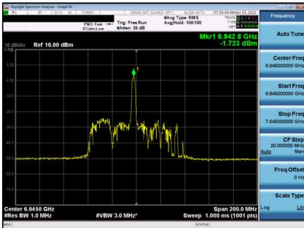
Plot 7-350. Power Spectral Density Plot MIMO ANT2 (80MHz BW 802.11ax (26 Tones) (UNII Band 8) – Ch. 199) – LPI
