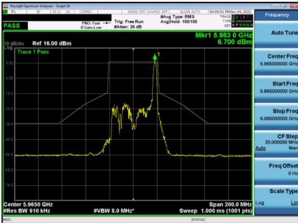
Plot 7-462. In-Band Emission Plot MIMO ANT1 (40MHz BW 802.11ax (26 Tones) (UNII Band 5) – Ch. 3) - SP
