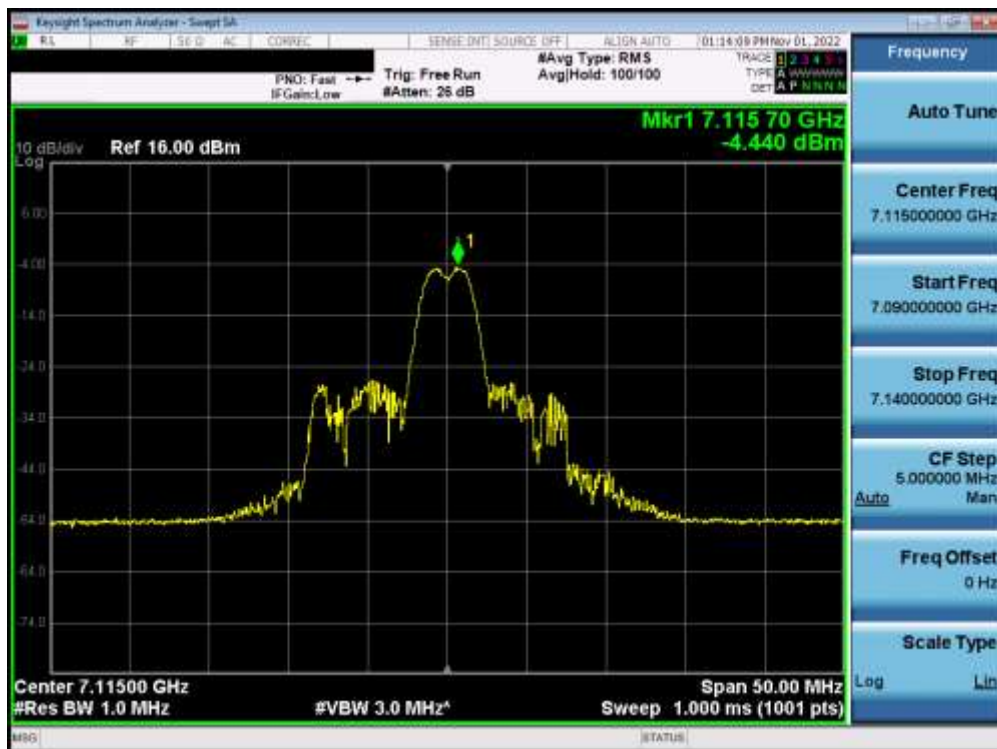
Plot 7-346. Power Spectral Density Plot MIMO ANT2 (20MHz BW 802.11ax (26 Tones) (UNII Band 8) – Ch. 233) – LPI
