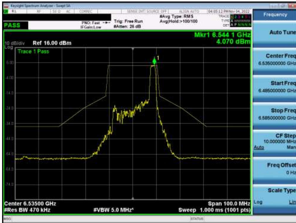
Plot 7-471. In-Band Emission Plot MIMO ANT1 (20MHz BW 802.11ax (26 Tones) (UNII Band 7) – Ch. 117) – SP
