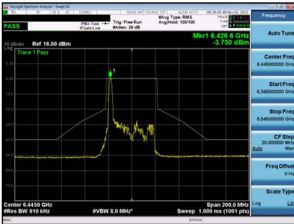
Plot 7-434. In-Band Emission Plot MIMO ANT1 (40MHz BW 802.11ax (26 Tones) (UNII Band 6) – Ch. 99) – LPI
