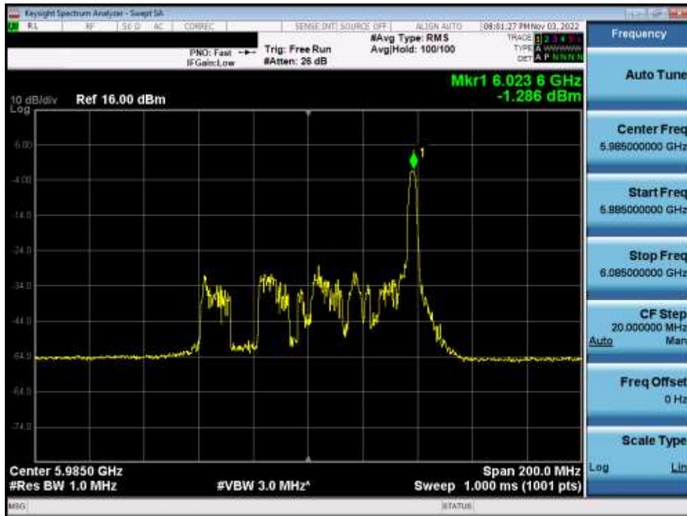
Plot 7-319. Power Spectral Density Plot MIMO ANT2 (80MHz BW 802.11ax (26 Tones) (UNII Band 5) – Ch. 7) – LPI
