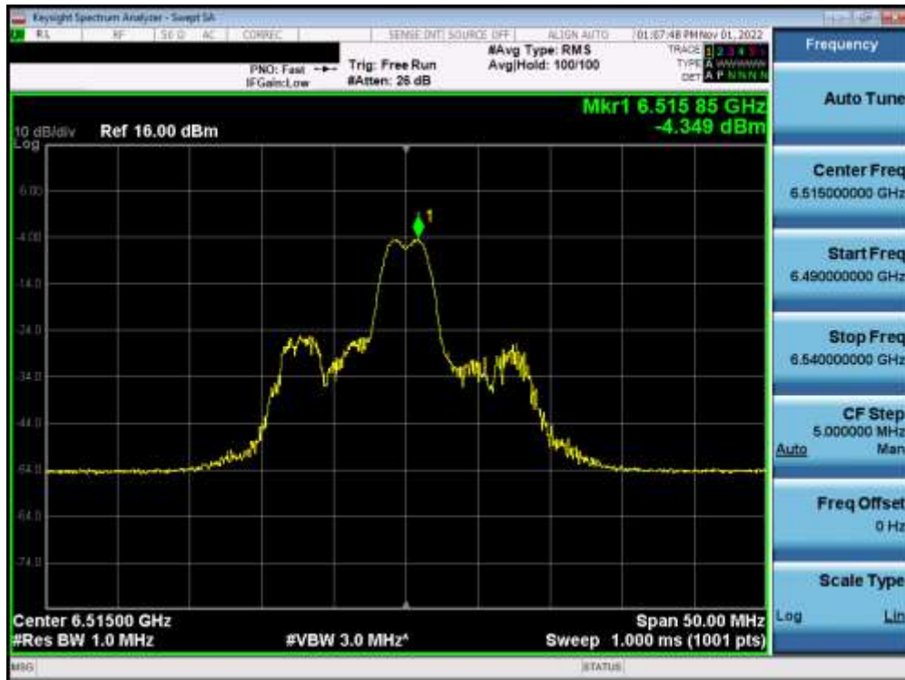
Plot 7-327. Power Spectral Density Plot MIMO ANT2 (20MHz BW 802.11ax (26 Tones) (UNII Band 6) – Ch. 113) – LPI
