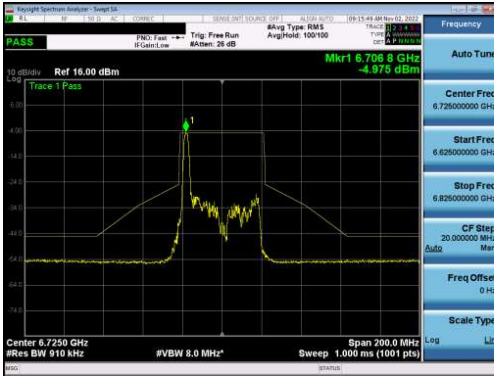
Plot 7-443. In-Band Emission Plot MIMO ANT1 (40MHz BW 802.11ax (26 Tones) (UNII Band 7) – Ch. 155) – LPI
