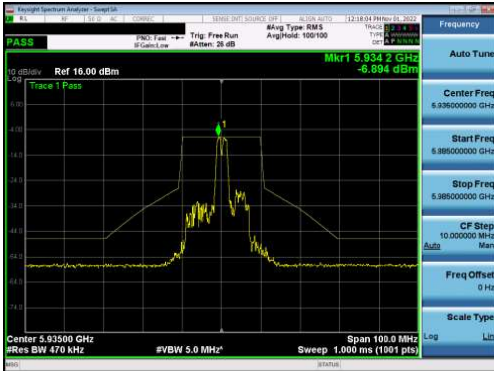
Plot 7-419. In-Band Emission Plot MIMO ANT1 (20MHz BW 802.11ax (26 Tones) UNII Band 5) – Ch. 2 – LPI
