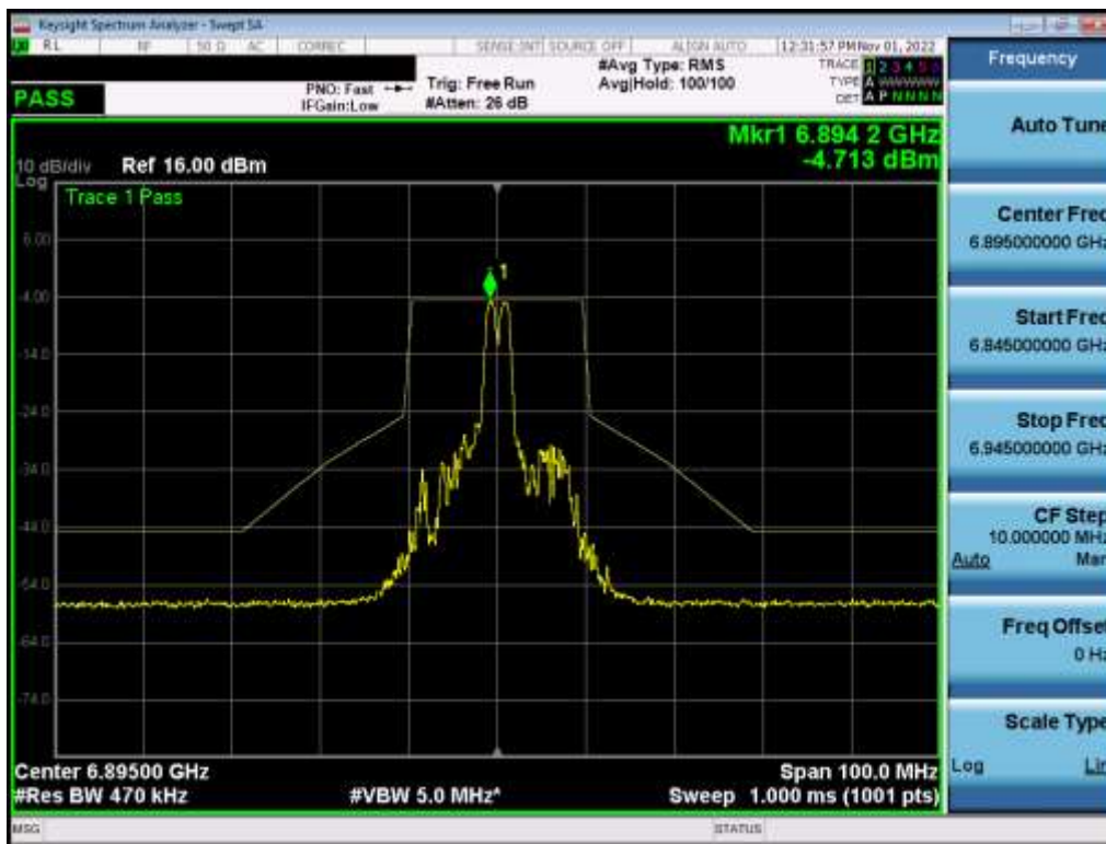
Plot 7-450. In-Band Emission Plot MIMO ANT1 (20MHz BW 802.11ax (26 Tones) (UNII Band 8) – Ch. 189) – LPI
