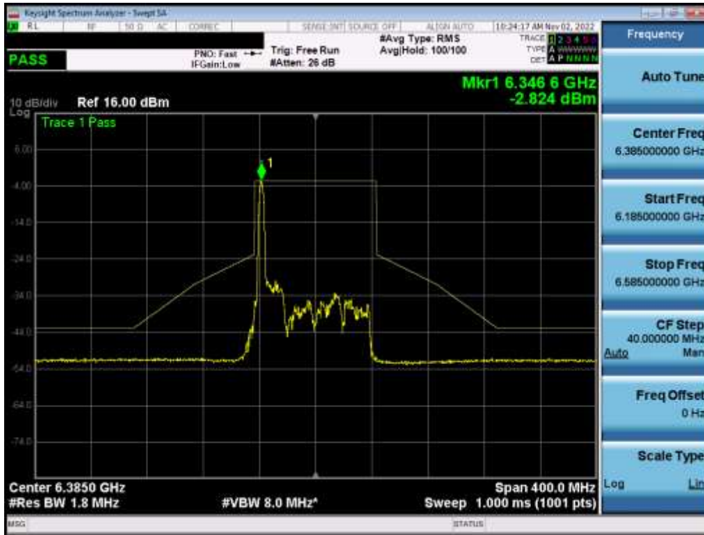
Plot 7-427. In-Band Emission Plot MIMO ANT1 (80MHz BW 802.11ax (26 Tones) (UNII Band 5) – Ch. 87) – LPI
