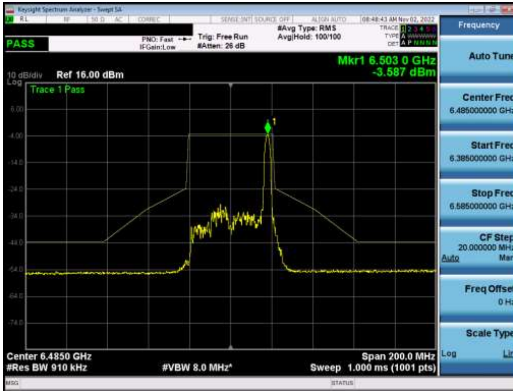
Plot 7-435. In-Band Emission Plot MIMO ANT1 (40MHz BW 802.11ax (26 Tones) (UNII Band 6) – Ch. 107) – LPI
