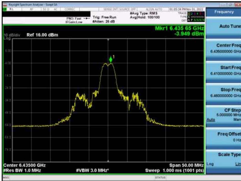
Plot 7-325. Power Spectral Density Plot MIMO ANT2 (20MHz BW 802.11ax (26 Tones) (UNII Band 6) – Ch. 97) – LPI
