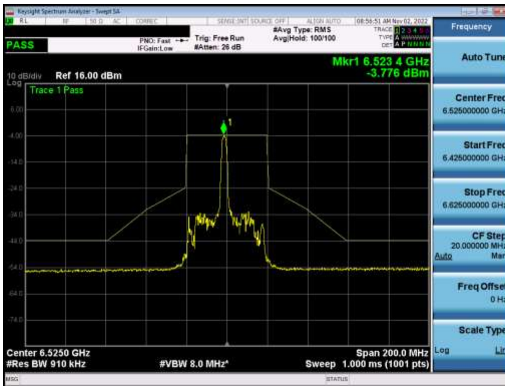
Plot 7-436. In-Band Emission Plot MIMO ANT1 (40MHz BW 802.11ax (26 Tones) (UNII Band 6) – Ch. 115) – LPI
