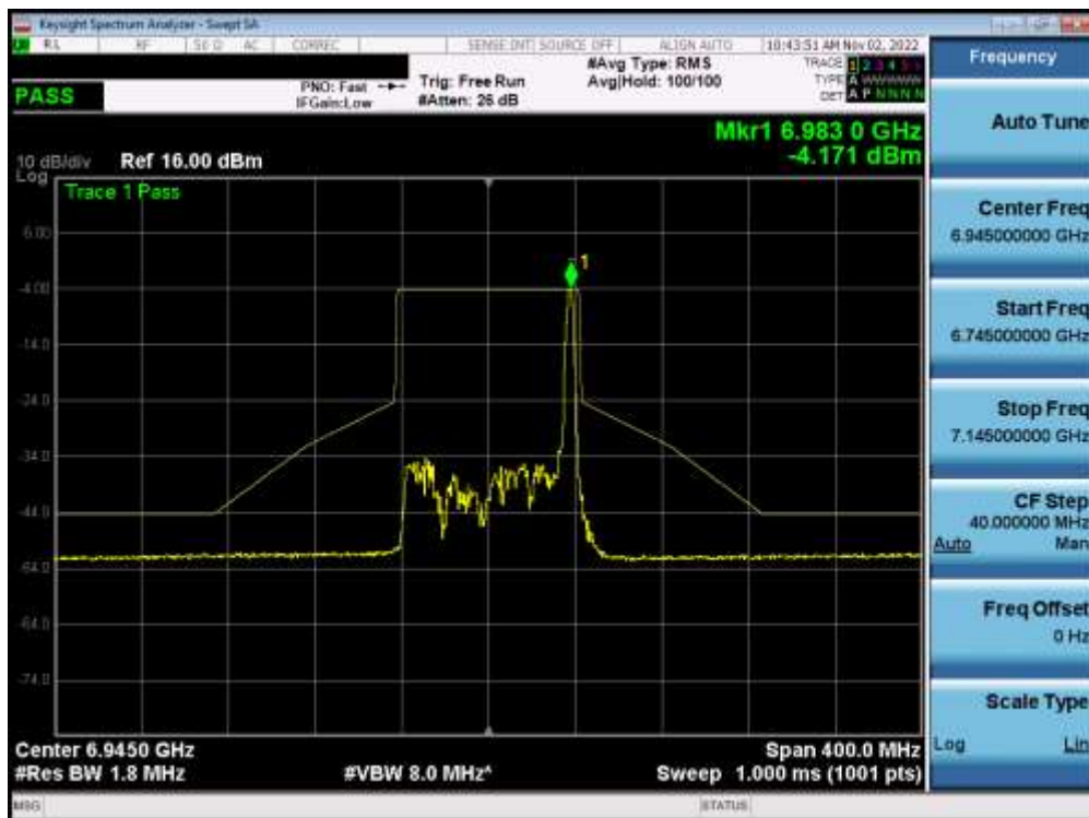
Plot 7-456. In-Band Emission Plot MIMO ANT1 (80MHz BW 802.11ax (26 Tones) (UNII Band 8) – Ch. 199) – LPI
