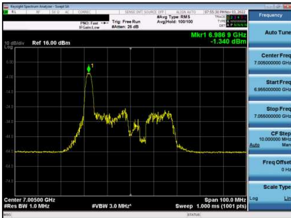
Plot 7-348. Power Spectral Density Plot MIMO ANT2 (40MHz BW 802.11ax (26 Tones) (UNII Band 8) – Ch. 211) – LPI
