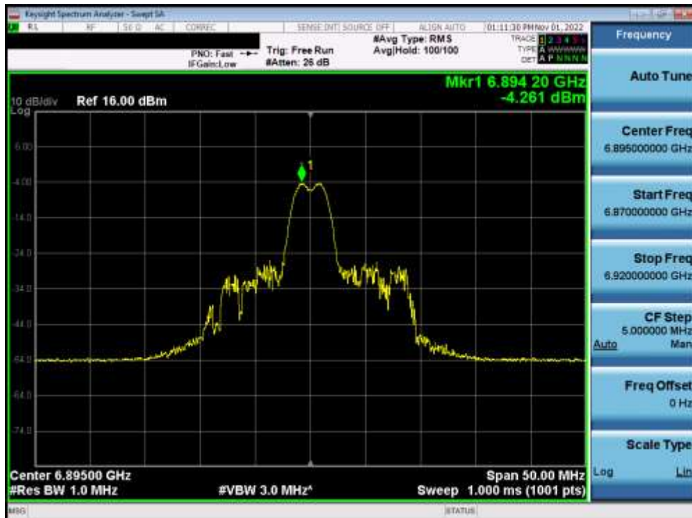
Plot 7-344. Power Spectral Density Plot MIMO ANT2 (20MHz BW 802.11ax (26 Tones) (UNII Band 8) – Ch. 189) – LPI
