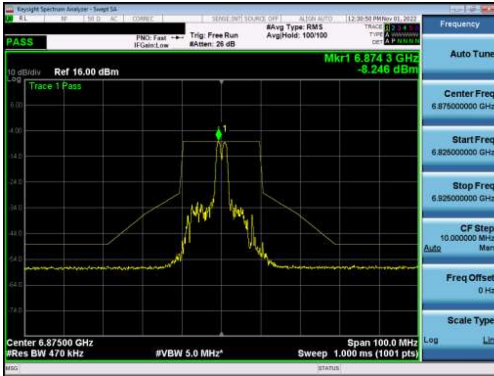
Plot 7-441. In-Band Emission Plot MIMO ANT1 (20MHz BW 802.11ax (26 Tones) (UNII Band 7) – Ch. 185) – LPI
