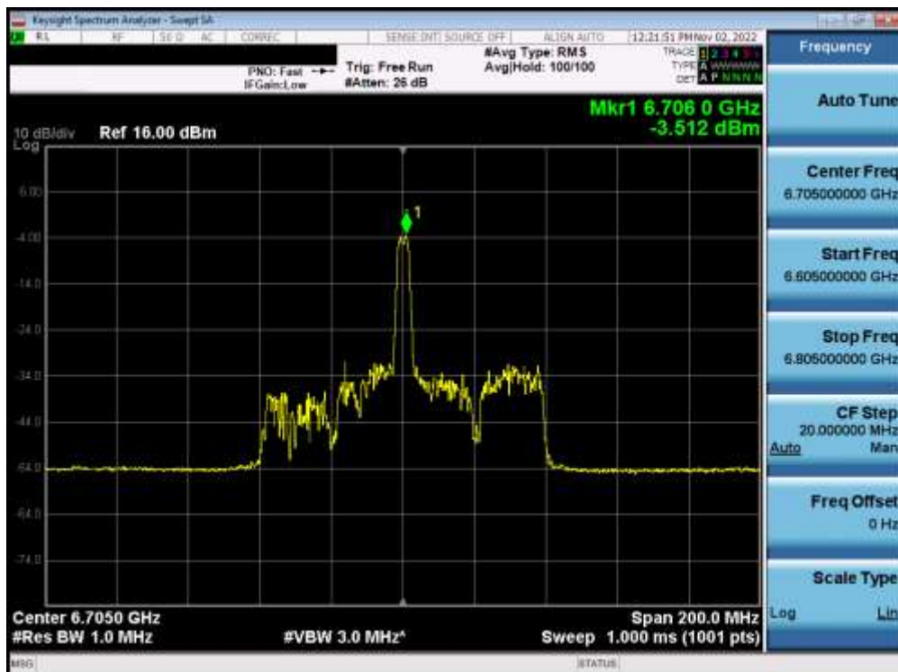
Plot 7-340. Power Spectral Density Plot MIMO ANT2 (80MHz BW 802.11ax (26 Tones) (UNII Band 7) – Ch. 151) – LPI
