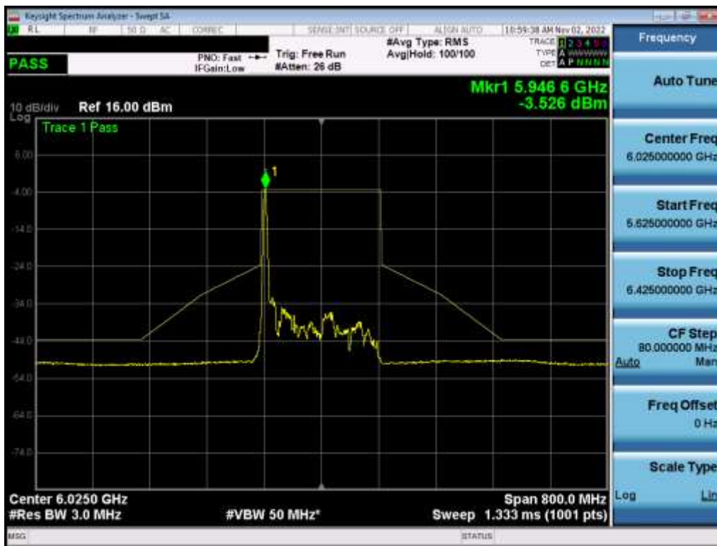
Plot 7-428. In-Band Emission Plot MIMO ANT1 (160MHz BW 802.11ax (26 Tones) (UNII Band 5) – Ch. 15) – LPI
