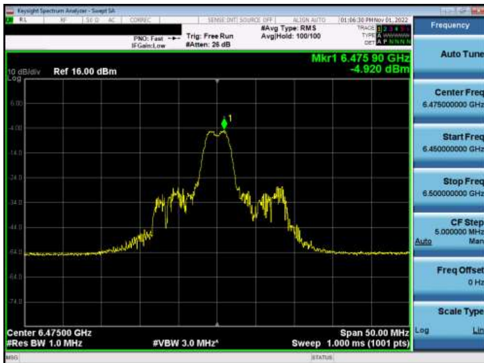
Plot 7-326. Power Spectral Density Plot MIMO ANT2 (20MHz BW 802.11ax (26 Tones) (UNII Band 6) – Ch. 105) – LPI
