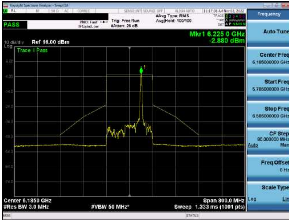
Plot 7-429. In-Band Emission Plot MIMO ANT1 (160MHz BW 802.11ax (26 Tones) (UNII Band 5) – Ch. 47) – LPI
