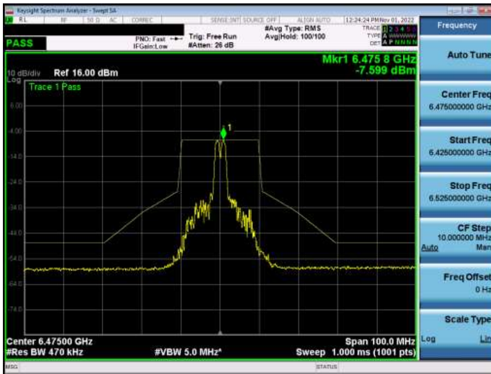
Plot 7-432. In-Band Emission Plot MIMO ANT1 (20MHz BW 802.11ax (26 Tones) (UNII Band 6) – Ch. 105) – LPI
