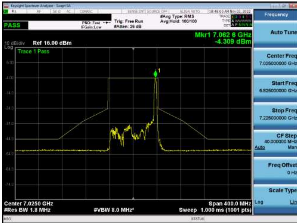
Plot 7-457. In-Band Emission Plot MIMO ANT1 (80MHz BW 802.11ax (26 Tones) (UNII Band 8) – Ch. 215) – LPI
