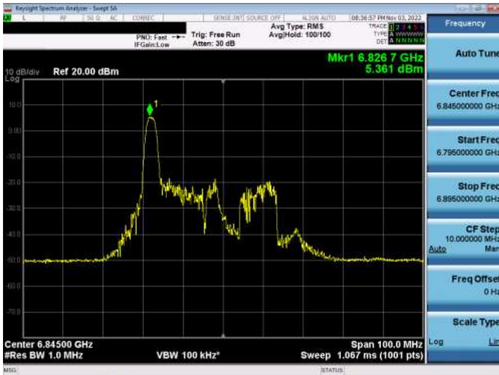
Plot 7-370. Power Spectral Density Plot MIMO ANT2 (40MHz BW 802.11ax (26 Tones) (UNII Band 7) – Ch. 179) – SP
