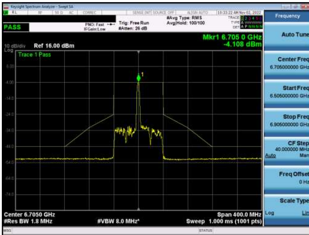
Plot 7-446. In-Band Emission Plot MIMO ANT1 (80MHz BW 802.11ax (26 Tones) (UNII Band 7) – Ch. 151) – LPI
