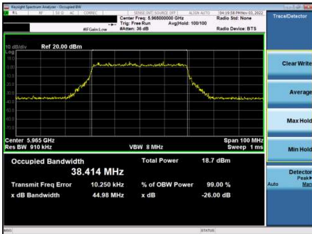
Plot 7-170. Occupied Bandwidth Plot MIMO ANT2 (40MHz BW 802.11ax (Full Tone) (UNII Band 5) – Ch. 3) – LPI/SP
