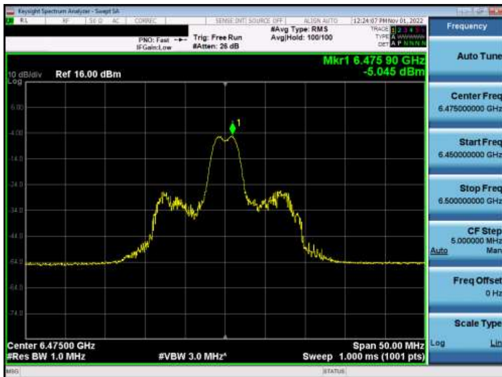
Plot 7-220. Power Spectral Density Plot MIMO ANT1 (20MHz BW 802.11ax (26 Tones) (UNII Band 6) – Ch. 105) – LPI
