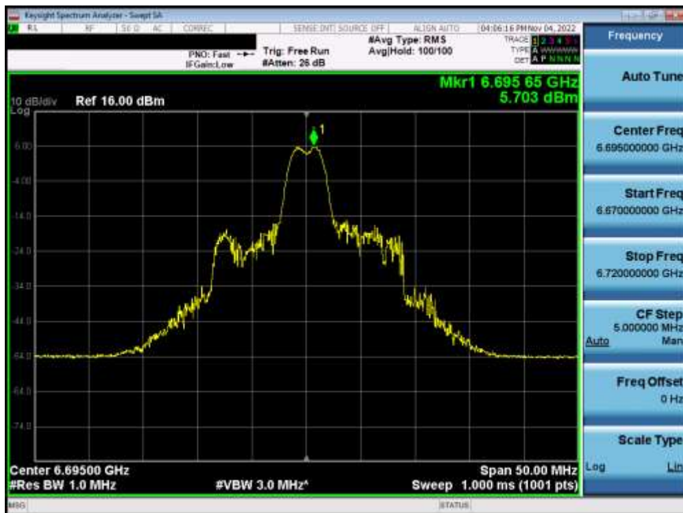
Plot 7-260. Power Spectral Density Plot MIMO ANT1 (20MHz BW 802.11ax (26 Tones) (UNII Band 7) – Ch. 149) – SP
