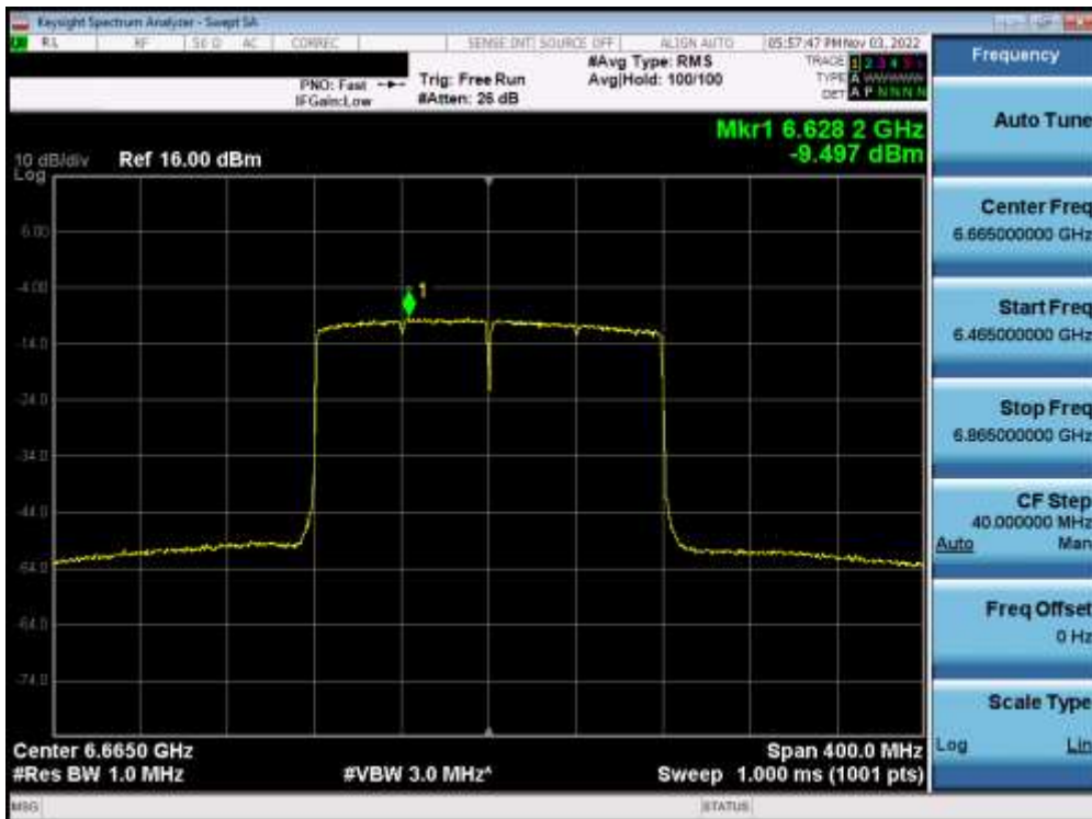
Plot 7-299. Power Spectral Density Plot MIMO ANT1 (160MHz BW 802.11ax (Full Tone) (UNII Band 7) – Ch. 143) – LPI/SP
