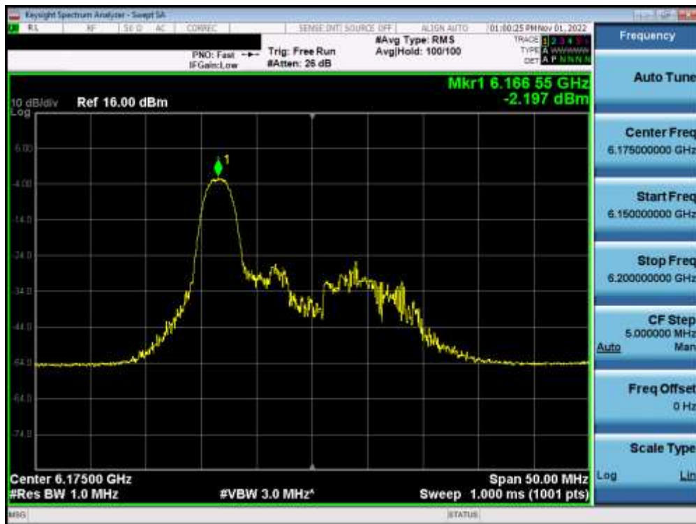
Plot 7-314. Power Spectral Density Plot MIMO ANT2 (20MHz BW 802.11ax (26 Tones) (UNII Band 5) – Ch. 45) – LPI
