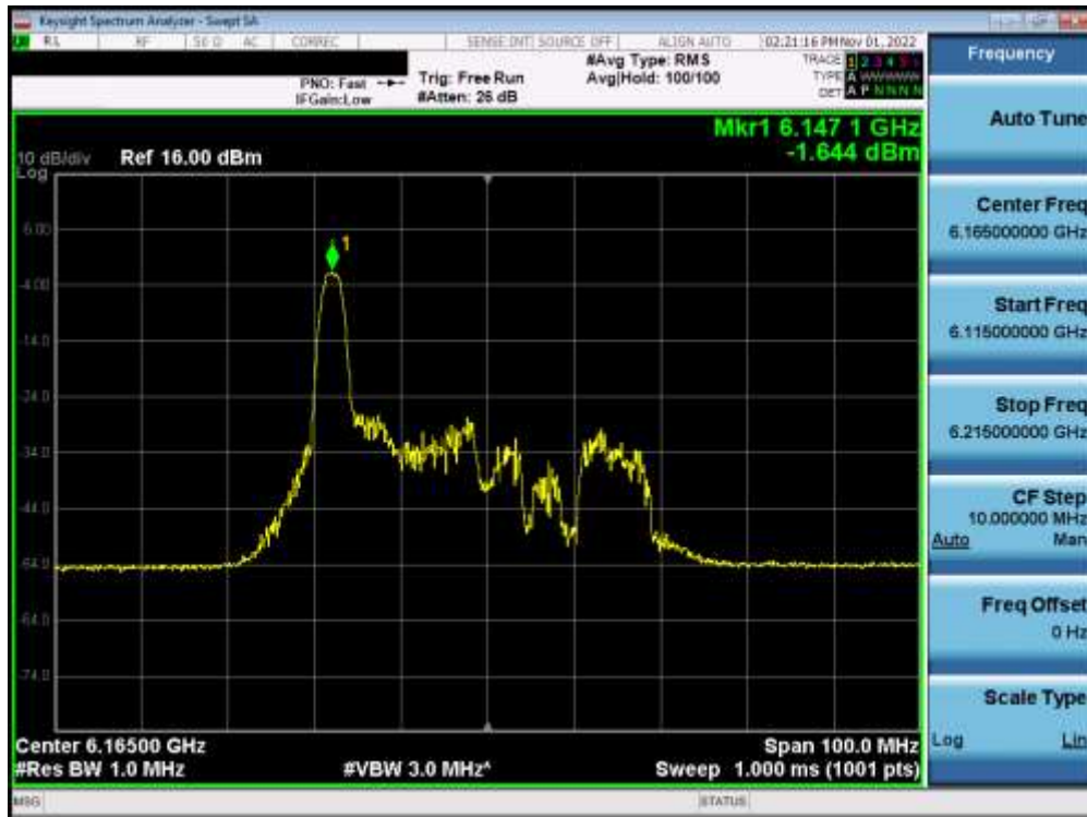
Plot 7-317. Power Spectral Density Plot MIMO ANT2 (40MHz BW 802.11ax (26 Tones) (UNII Band 5) – Ch. 43) – LPI
