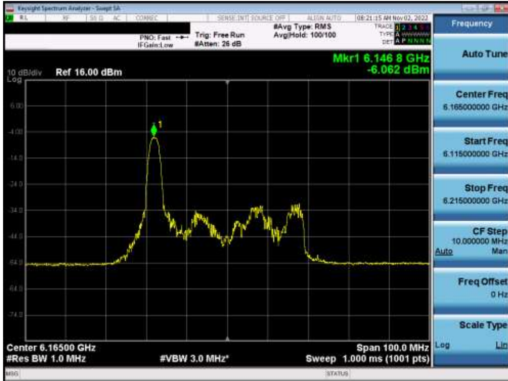
Plot 7-211. Power Spectral Density Plot MIMO ANT1 (40MHz BW 802.11ax (26 Tones) (UNII Band 5) – Ch. 43) – LPI
