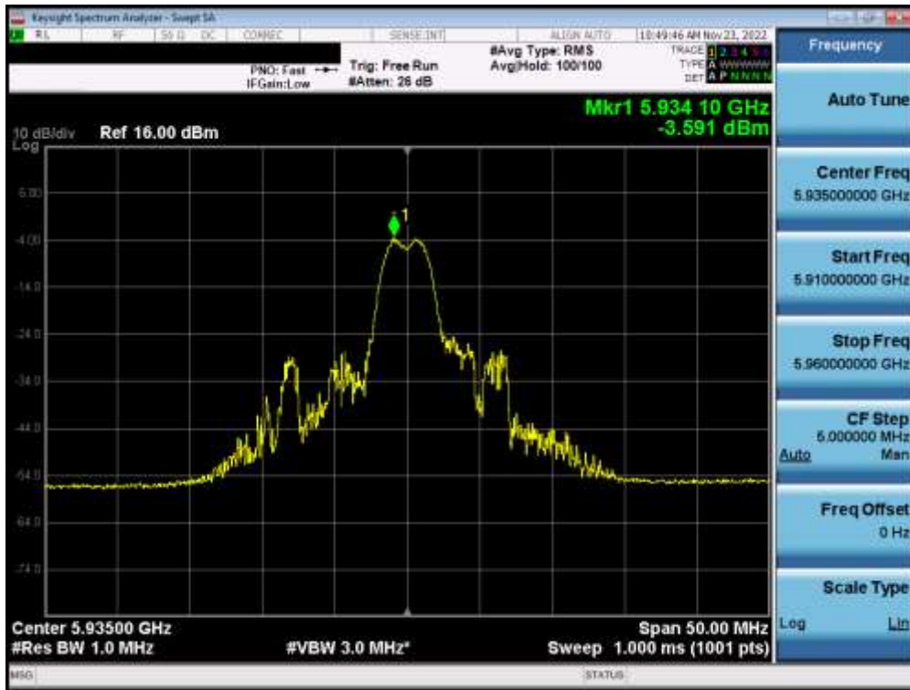
Plot 7-207. Power Spectral Density Plot MIMO ANT1 (20MHz BW 802.11ax (26 Tones) UNII Band 5) – Ch. 2 – LPI
