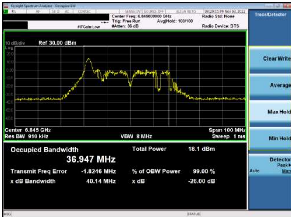
Plot 7-161. Occupied Bandwidth Plot MIMO ANT2 (40MHz BW 802.11ax (26 Tones) (UNII Band 7) – Ch. 179) – SP
