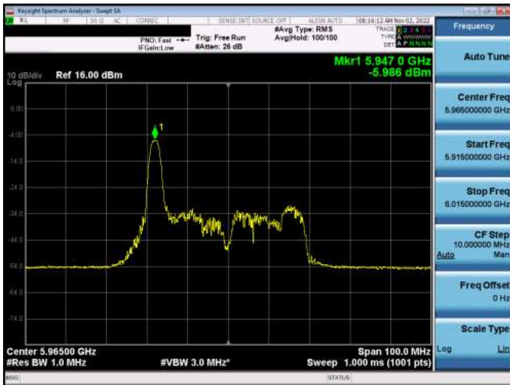
Plot 7-210. Power Spectral Density Plot MIMO ANT1 (40MHz BW 802.11ax (26 Tones) (UNII Band 5) – Ch. 3) – LPI
