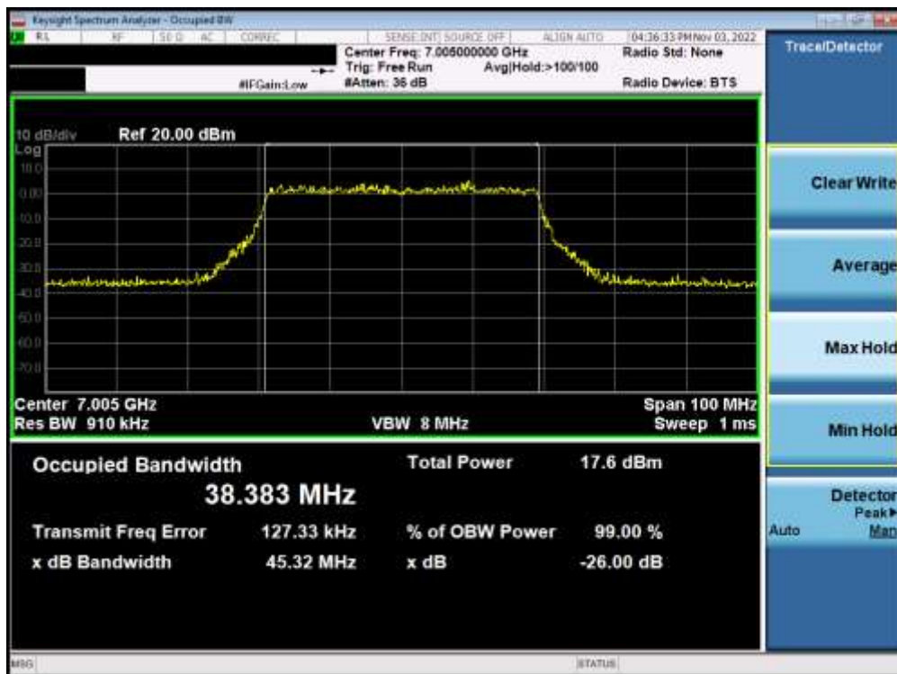
Plot 7-202. Occupied Bandwidth Plot MIMO ANT2 (40MHz BW 802.11ax (Full Tone) (UNII Band 8) – Ch. 211) – LPI
