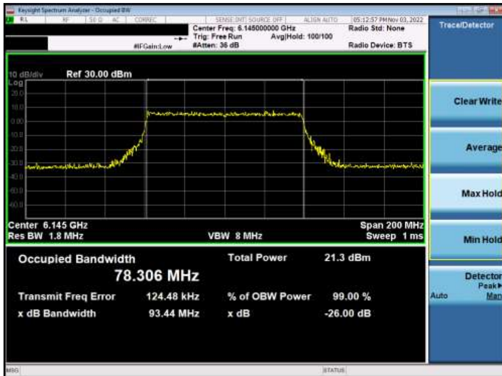
Plot 7-174. Occupied Bandwidth Plot MIMO ANT2 (80MHz BW 802.11ax (Full Tone) (UNII Band 5) – Ch. 39) – LPI/SP
