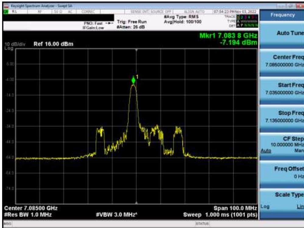
Plot 7-243. Power Spectral Density Plot MIMO ANT1 (40MHz BW 802.11ax (26 Tones) (UNII Band 8) – Ch. 227) – LPI
