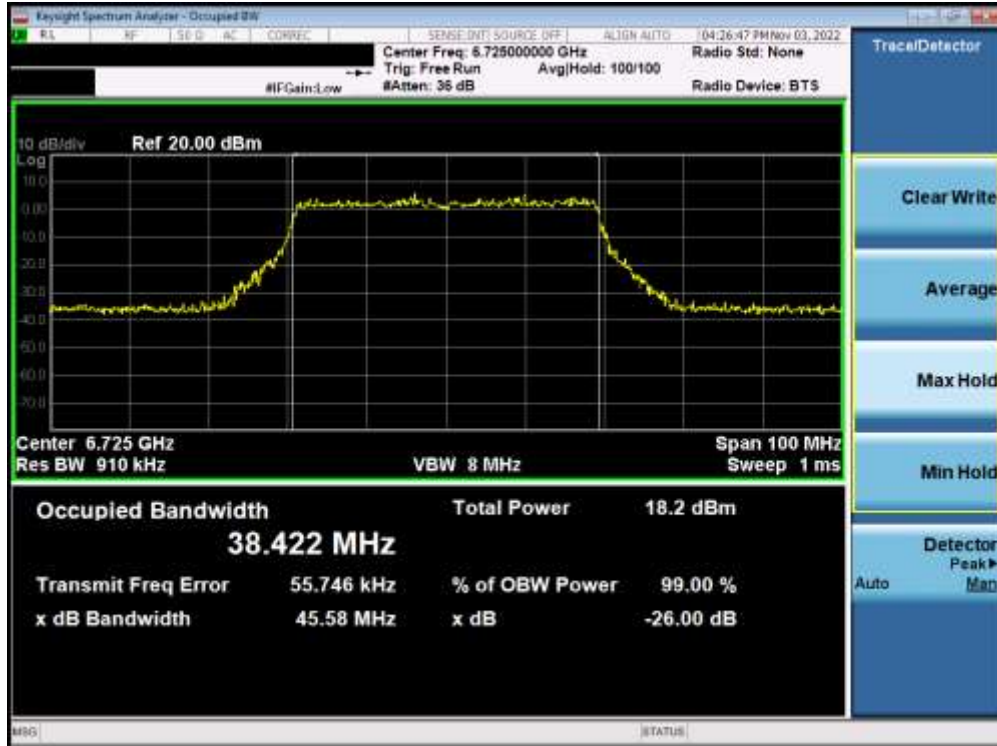
Plot 7-191. Occupied Bandwidth Plot MIMO ANT2 (40MHz BW 802.11ax (Full Tone) (UNII Band 7) – Ch. 155) – LPI/SP
