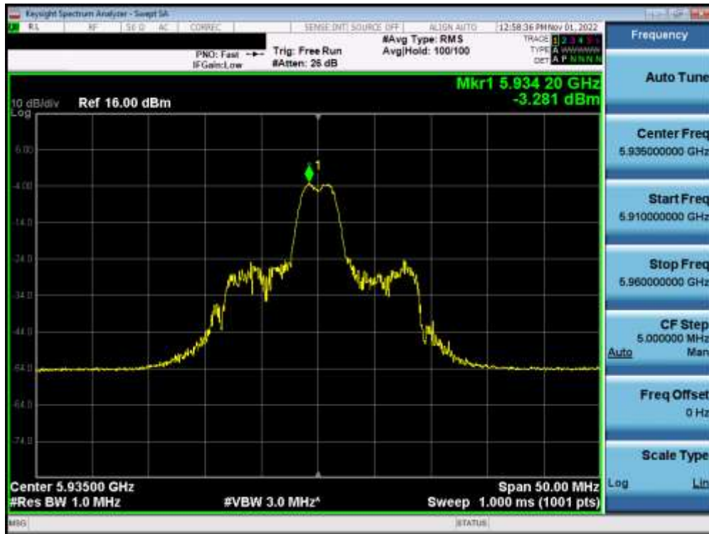
Plot 7-313. Power Spectral Density Plot MIMO ANT2 (20MHz BW 802.11ax (26 Tones) UNII Band 5) – Ch. 2 – LPI
