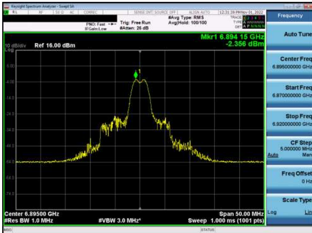
Plot 7-238. Power Spectral Density Plot MIMO ANT1 (20MHz BW 802.11ax (26 Tones) (UNII Band 8) – Ch. 189) – LPI
