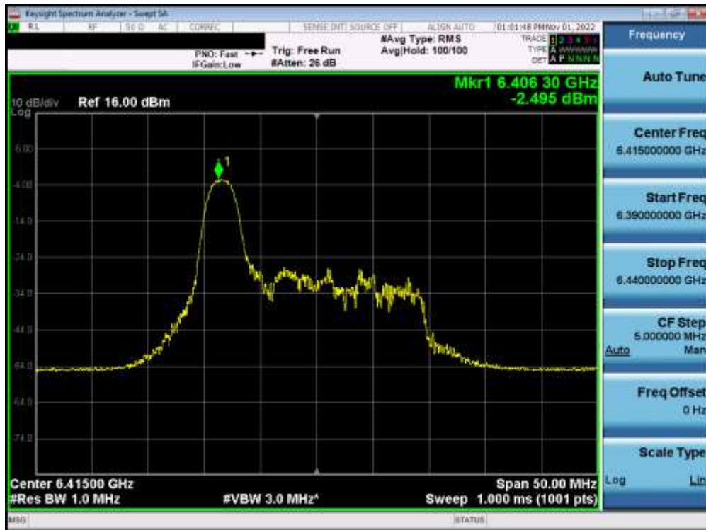
Plot 7-315. Power Spectral Density Plot MIMO ANT2 (20MHz BW 802.11ax (26 Tones) UNII Band 5) – Ch. 93) – LPI
