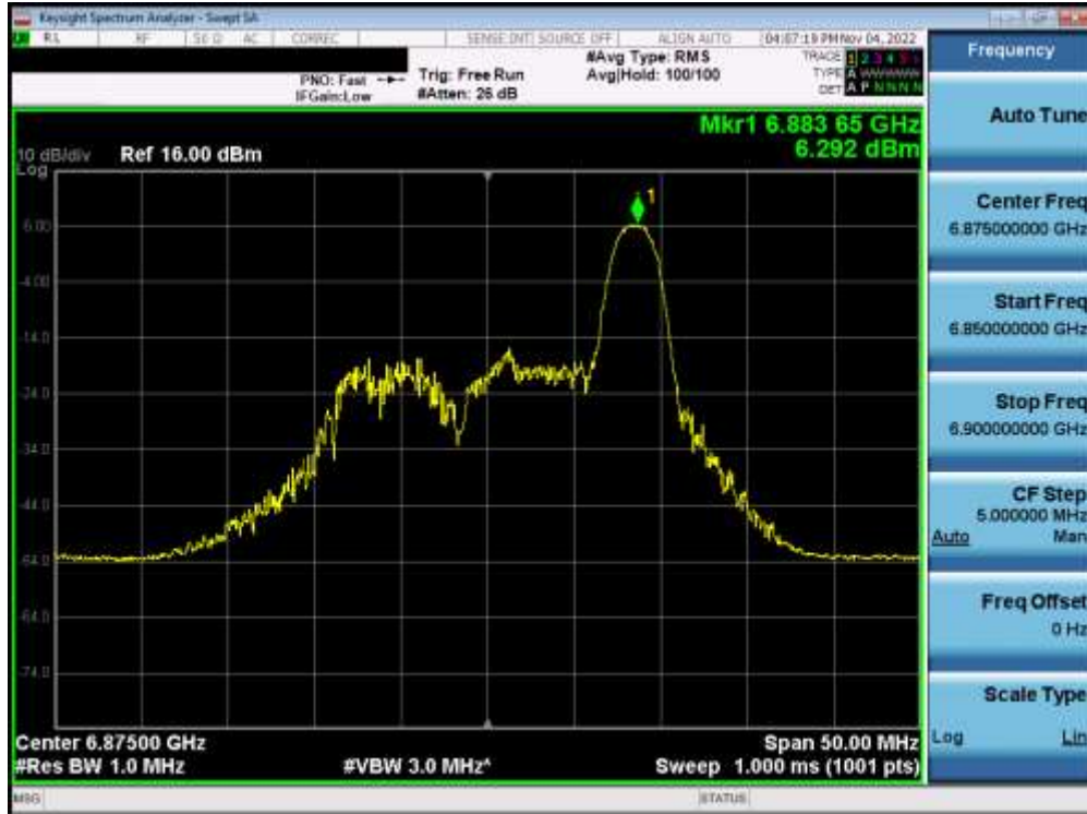
Plot 7-261. Power Spectral Density Plot MIMO ANT1 (20MHz BW 802.11ax (26 Tones) (UNII Band 7) – Ch. 185) – SP
