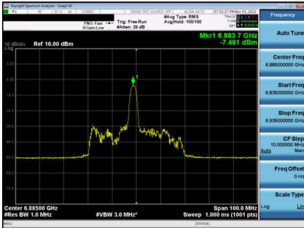
Plot 7-241. Power Spectral Density Plot MIMO ANT1 (40MHz BW 802.11ax (26 Tones) (UNII Band 8) – Ch. 187) – LPI
