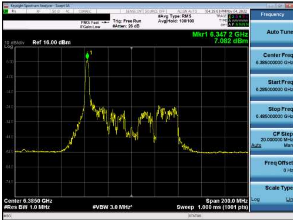
Plot 7-255. Power Spectral Density Plot MIMO ANT1 (80MHz BW 802.11ax (26 Tones) (UNII Band 5) – Ch. 87) – SP
