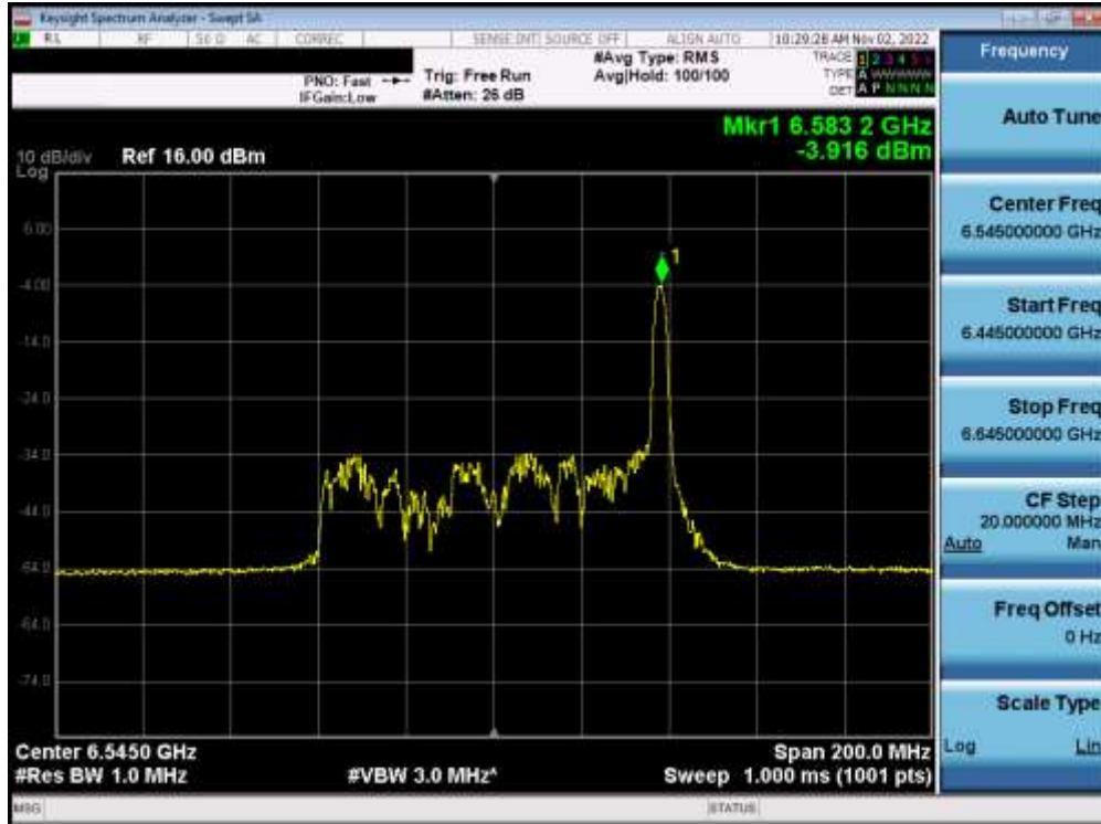
Plot 7-233. Power Spectral Density Plot MIMO ANT1 (80MHz BW 802.11ax (26 Tones) (UNII Band 7) – Ch. 119) – LPI
