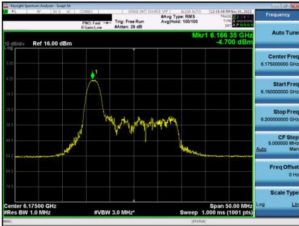
Plot 7-208. Power Spectral Density Plot MIMO ANT1 (20MHz BW 802.11ax (26 Tones) (UNII Band 5) – Ch. 45) – LPI
