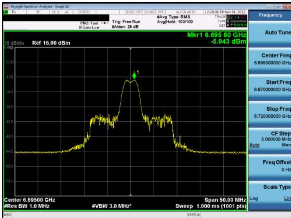
Plot 7-228. Power Spectral Density Plot MIMO ANT1 (20MHz BW 802.11ax (26 Tones) (UNII Band 7) – Ch. 149) – LPI
