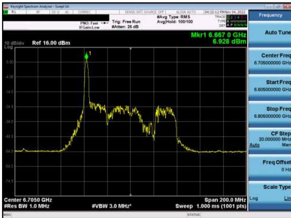
Plot 7-266. Power Spectral Density Plot MIMO ANT1 (80MHz BW 802.11ax (26 Tones) (UNII Band 7) – Ch. 151) – SP
