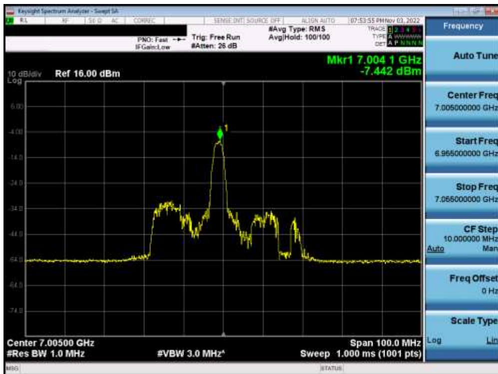
Plot 7-242. Power Spectral Density Plot MIMO ANT1 (40MHz BW 802.11ax (26 Tones) (UNII Band 8) – Ch. 211) – LPI
