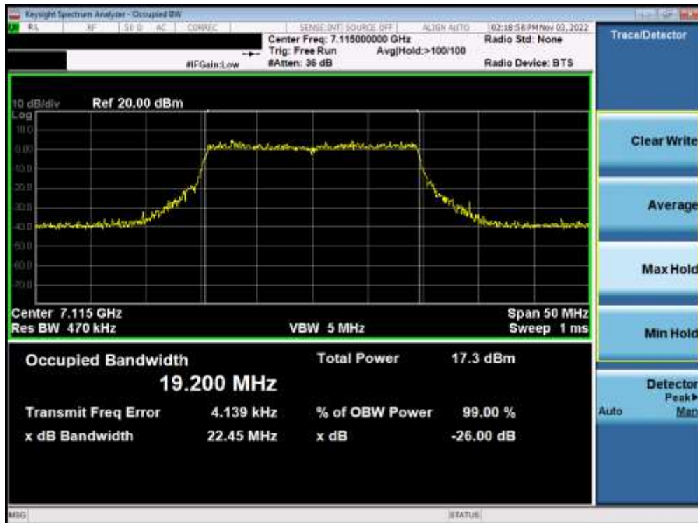
Plot 7-200. Occupied Bandwidth Plot MIMO ANT2 (20MHz BW 802.11ax (Full Tone) (UNII Band 8) – Ch. 233) – LPI
