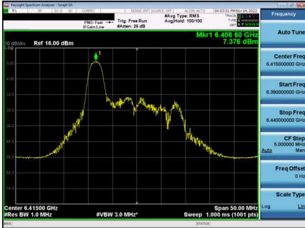
Plot 7-249. Power Spectral Density Plot MIMO ANT1 (20MHz BW 802.11ax (26 Tones) UNII Band 5) – Ch. 93) – SP
