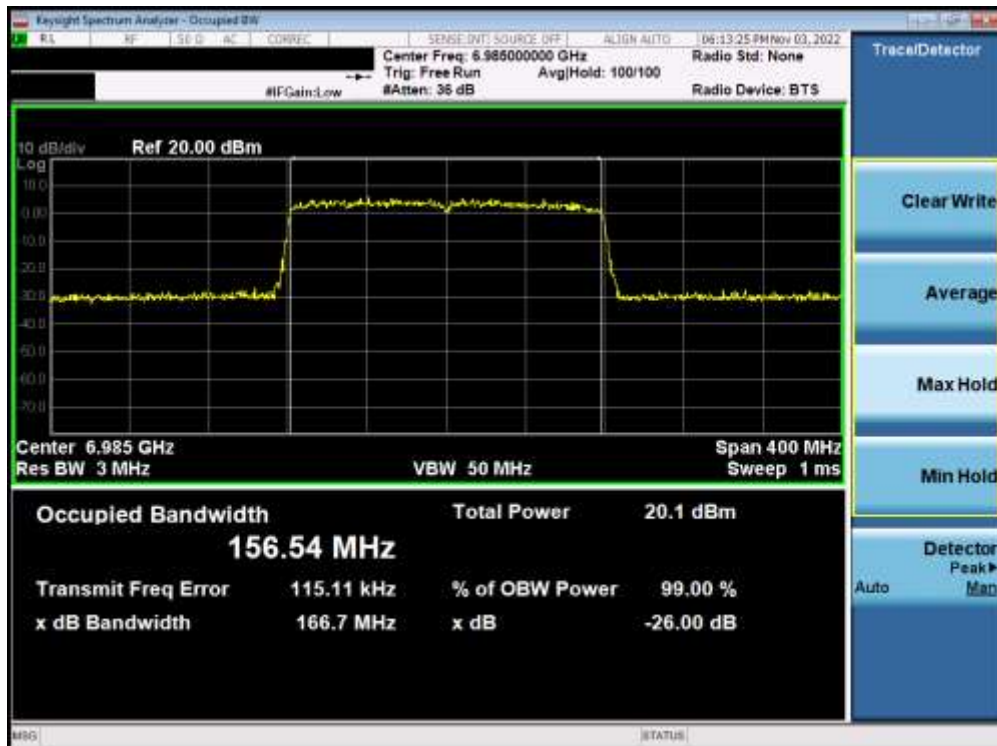
Plot 7-206. Occupied Bandwidth Plot MIMO ANT2 (160MHz BW 802.11ax (Full Tone) (UNII Band 8) – Ch. 207) – LPI
