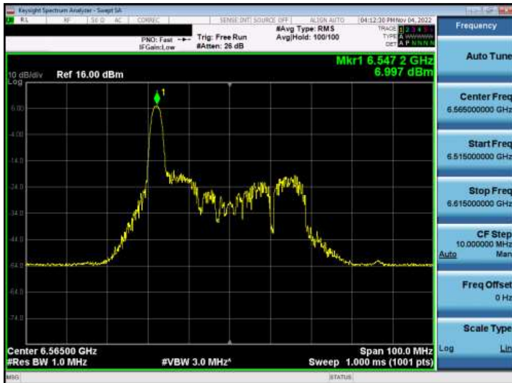
Plot 7-262. Power Spectral Density Plot MIMO ANT1 (40MHz BW 802.11ax (26 Tones) (UNII Band 7) – Ch. 123) – SP
