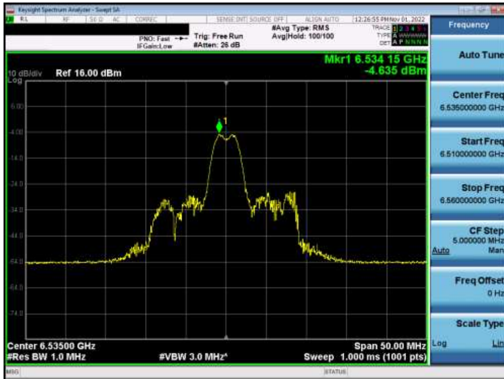
Plot 7-227. Power Spectral Density Plot MIMO ANT1 (20MHz BW 802.11ax (26 Tones) (UNII Band 7) – Ch. 117) – LPI
