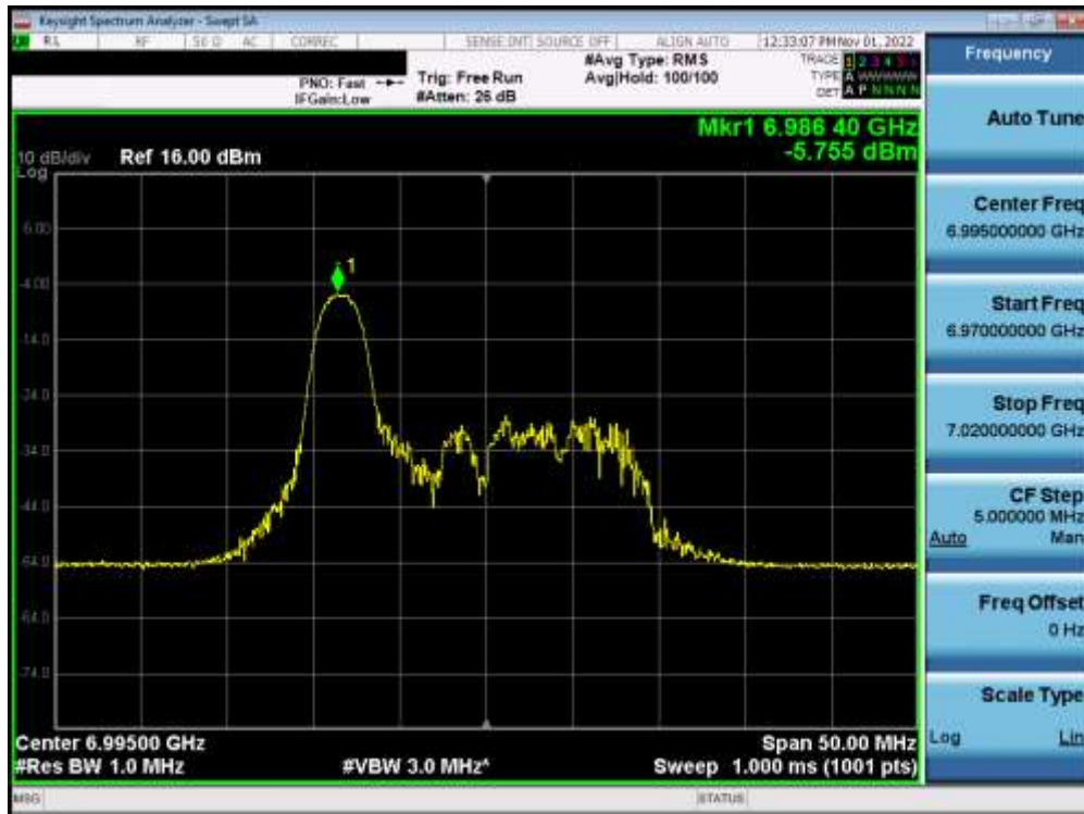
Plot 7-239. Power Spectral Density Plot MIMO ANT1 (20MHz BW 802.11ax (26 Tones) (UNII Band 8) – Ch. 209) – LPI
