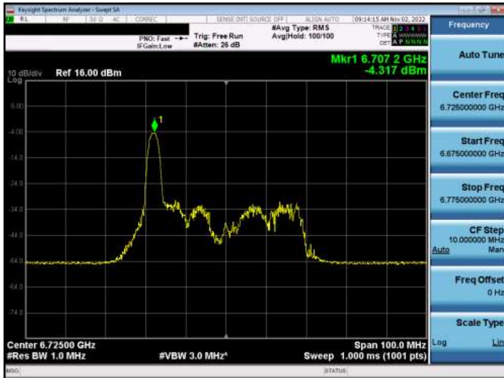
Plot 7-231. Power Spectral Density Plot MIMO ANT1 (40MHz BW 802.11ax (26 Tones) (UNII Band 7) – Ch. 155) – LPI
