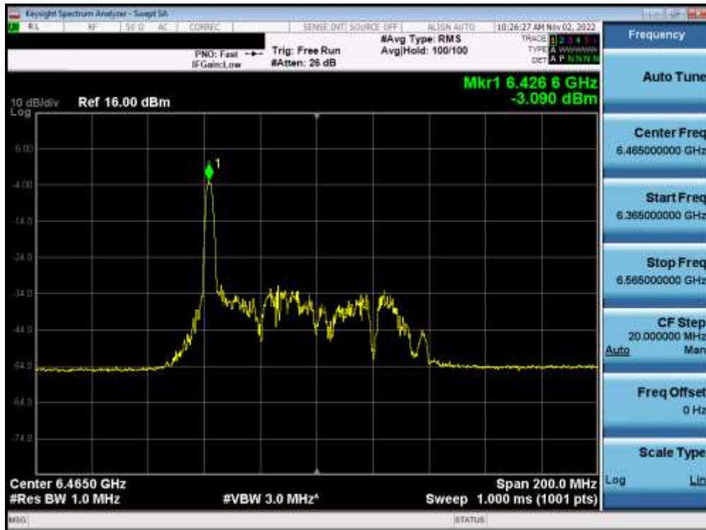
Plot 7-225. Power Spectral Density Plot MIMO ANT1 (80MHz BW 802.11ax (26 Tones) (UNII Band 6) – Ch. 103) – LPI
