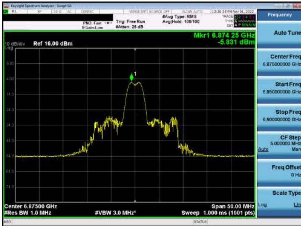
Plot 7-229. Power Spectral Density Plot MIMO ANT1 (20MHz BW 802.11ax (26 Tones) (UNII Band 7) – Ch. 185) – LPI
