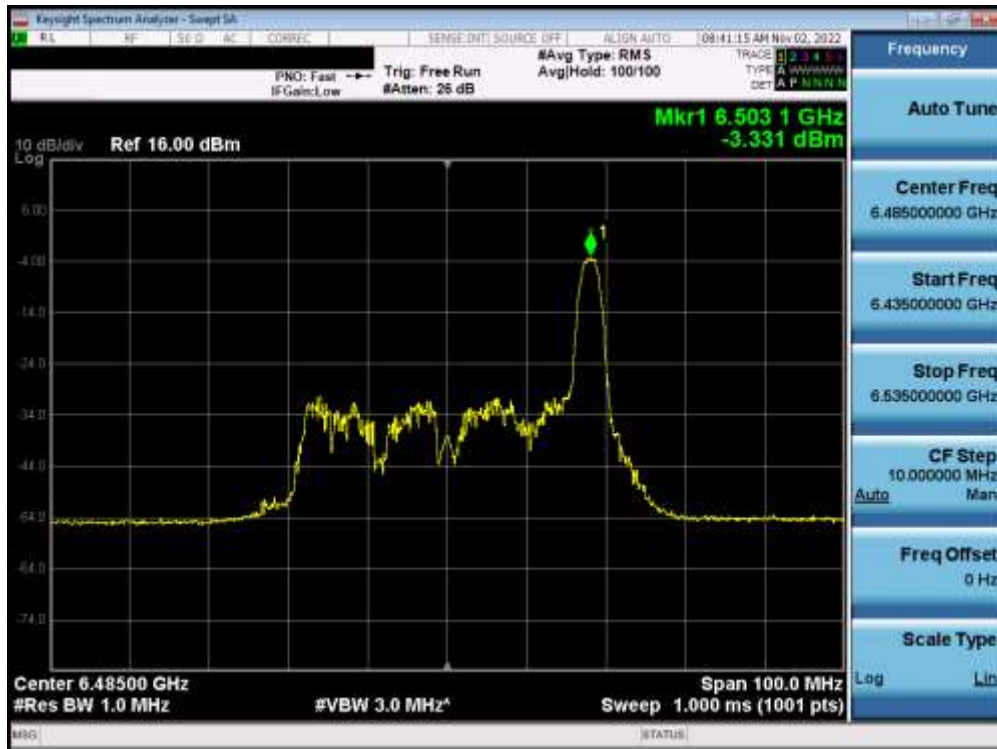
Plot 7-223. Power Spectral Density Plot MIMO ANT1 (40MHz BW 802.11ax (26 Tones) (UNII Band 6) – Ch. 107) – LPI
