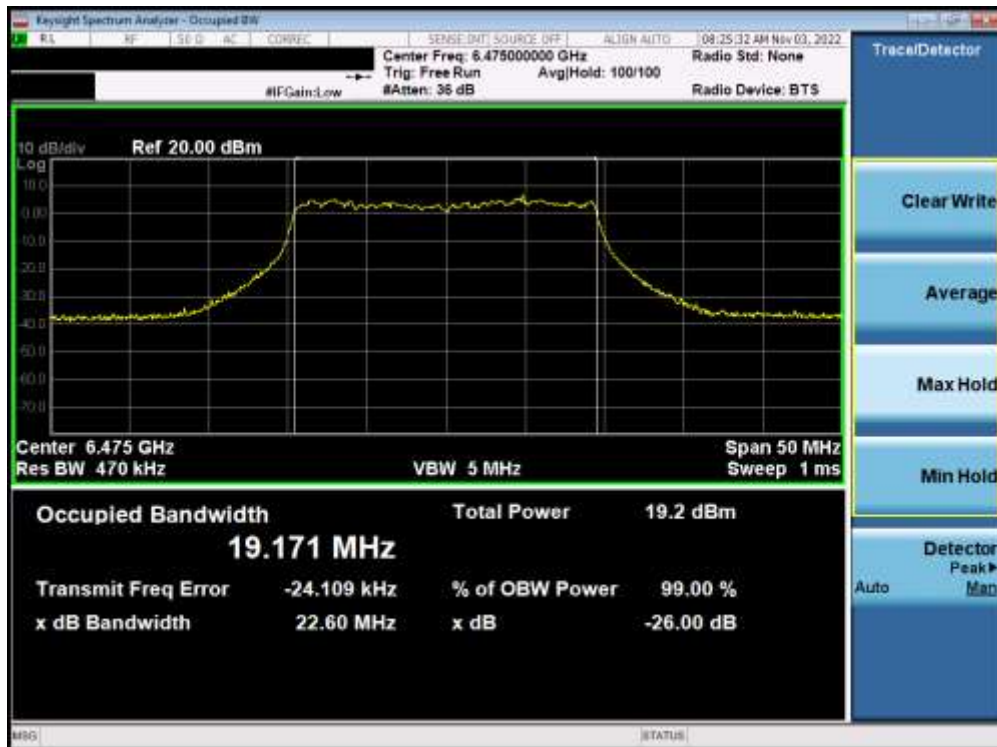
Plot 7-180. Occupied Bandwidth Plot MIMO ANT2 (20MHz BW 802.11ax (Full Tone) (UNII Band 6) – Ch. 105) – LPI
