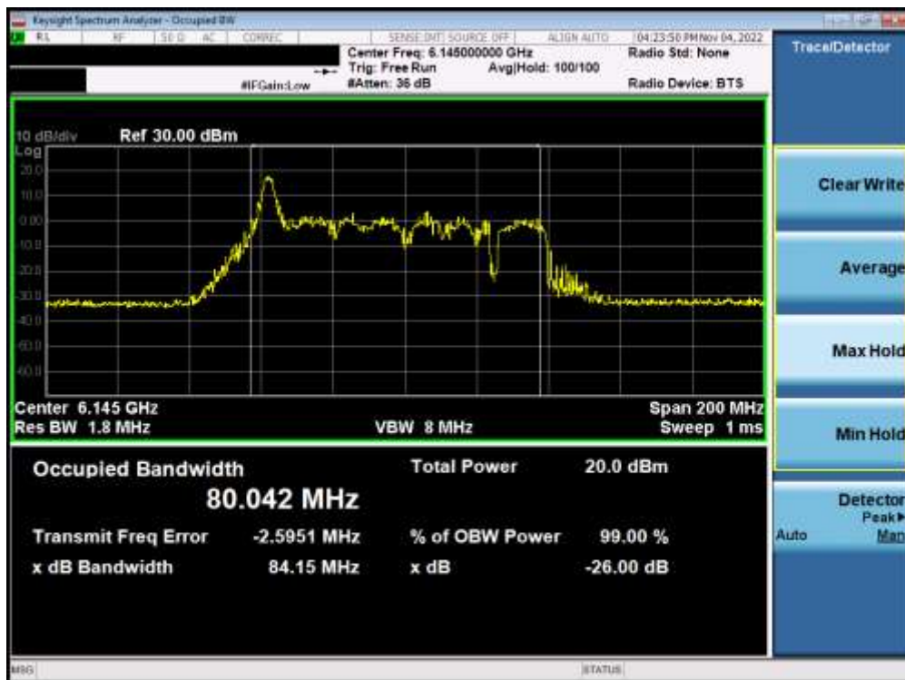
Plot 7-48. Occupied Bandwidth Plot MIMO ANT1 (80MHz BW 802.11ax (26 Tones) (UNII Band 5) – Ch. 39) - SP
