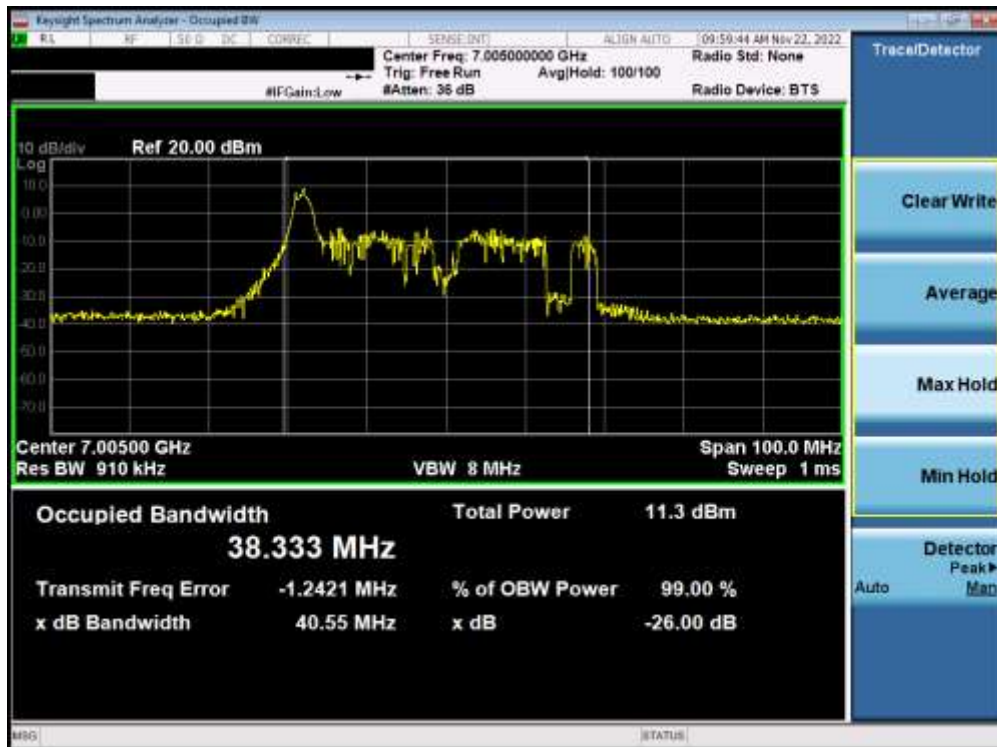
Plot 7-139. Occupied Bandwidth Plot MIMO ANT2 (40MHz BW 802.11ax (26 Tones) (UNII Band 8) – Ch. 211) – LPI
