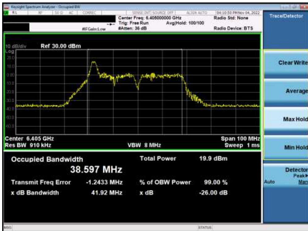
Plot 7-46. Occupied Bandwidth Plot MIMO ANT1 (40MHz BW 802.11ax (26 Tones) (UNII Band 5) – Ch. 91) - SP
