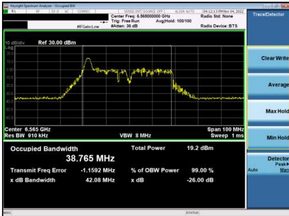
Plot 7-56. Occupied Bandwidth Plot MIMO ANT1 (40MHz BW 802.11ax (26 Tones) (UNII Band 7) – Ch. 123) – SP
