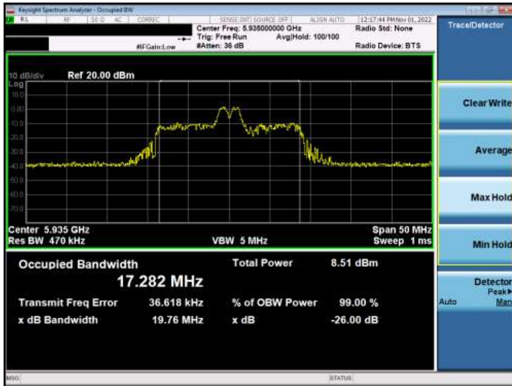
Plot 7-1. Occupied Bandwidth Plot MIMO ANT1 (20MHz BW 802.11ax (26 Tones) UNII Band 5) – Ch. 2 – LPI
