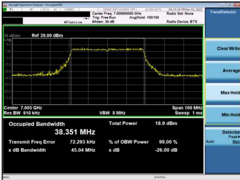
Plot 7-99. Occupied Bandwidth Plot MIMO ANT1 (40MHz BW 802.11ax (Full Tone) (UNII Band 8) – Ch. 211) – LPI
