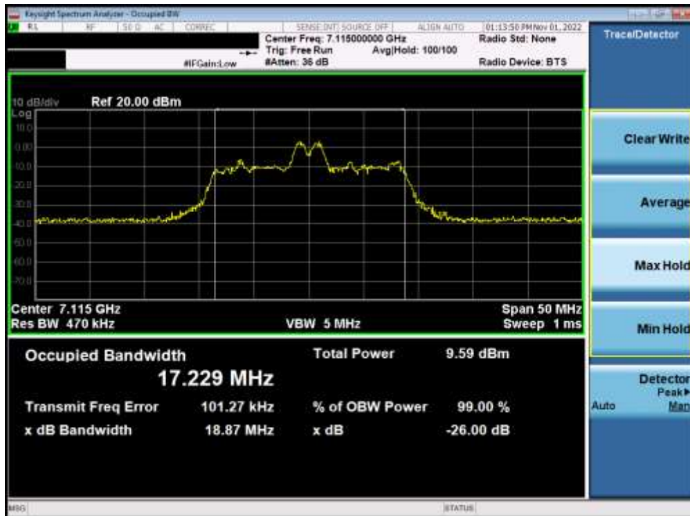
Plot 7-137. Occupied Bandwidth Plot MIMO ANT2 (20MHz BW 802.11ax (26 Tones) (UNII Band 8) – Ch. 233) – LPI
