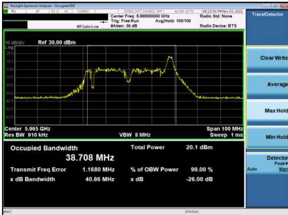
Plot 7-147. Occupied Bandwidth Plot MIMO ANT2 (40MHz BW 802.11ax (26 Tones) UNII Band 5) – Ch. 3) – SP
