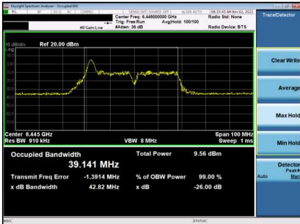
Plot 7-16. Occupied Bandwidth Plot MIMO ANT1 (40MHz BW 802.11ax (26 Tones) (UNII Band 6) – Ch. 99) – LPI
