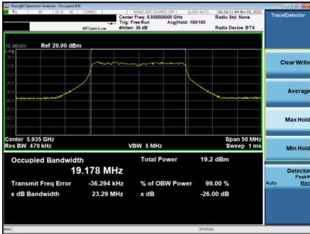
Plot 7-64. Occupied Bandwidth Plot MIMO ANT1 (20MHz BW 802.11ax (Full Tone) UNII Band 5) – Ch. 2 – LPI/SP
