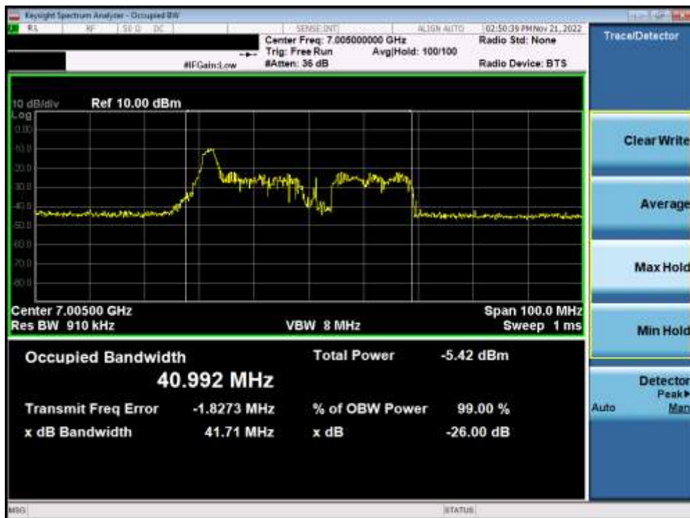
Plot 7-36. Occupied Bandwidth Plot MIMO ANT1 (40MHz BW 802.11ax (26 Tones) (UNII Band 8) – Ch. 211) – LPI
