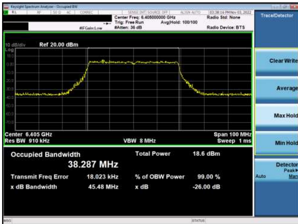
Plot 7-69. Occupied Bandwidth Plot MIMO ANT1 (40MHz BW 802.11ax (Full Tone) (UNII Band 5) – Ch. 91) – LPI/SP
