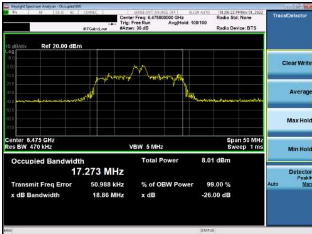
Plot 7-117. Occupied Bandwidth Plot MIMO ANT2 (20MHz BW 802.11ax (26 Tones) (UNII Band 6) – Ch. 105) – LPI
