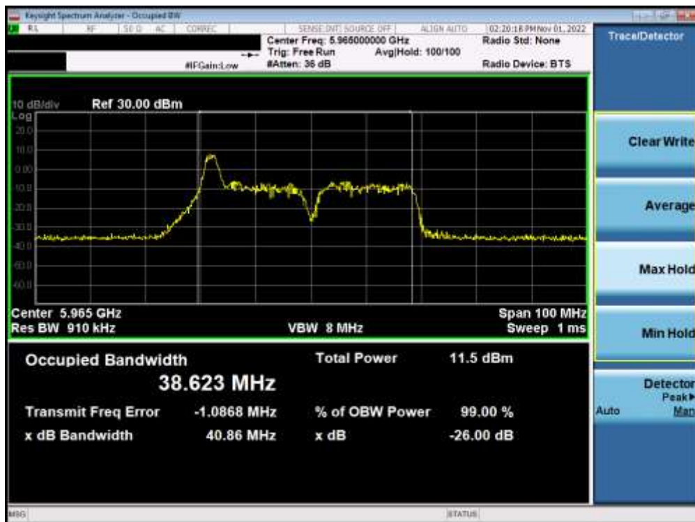
Plot 7-107. Occupied Bandwidth Plot MIMO ANT2 (40MHz BW 802.11ax (26 Tones) (UNII Band 5) – Ch. 3) – LPI
