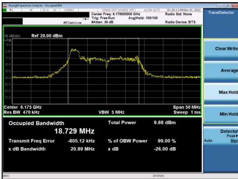
Plot 7-105. Occupied Bandwidth Plot MIMO ANT2 (20MHz BW 802.11ax (26 Tones) (UNII Band 5) – Ch. 45) – LPI
