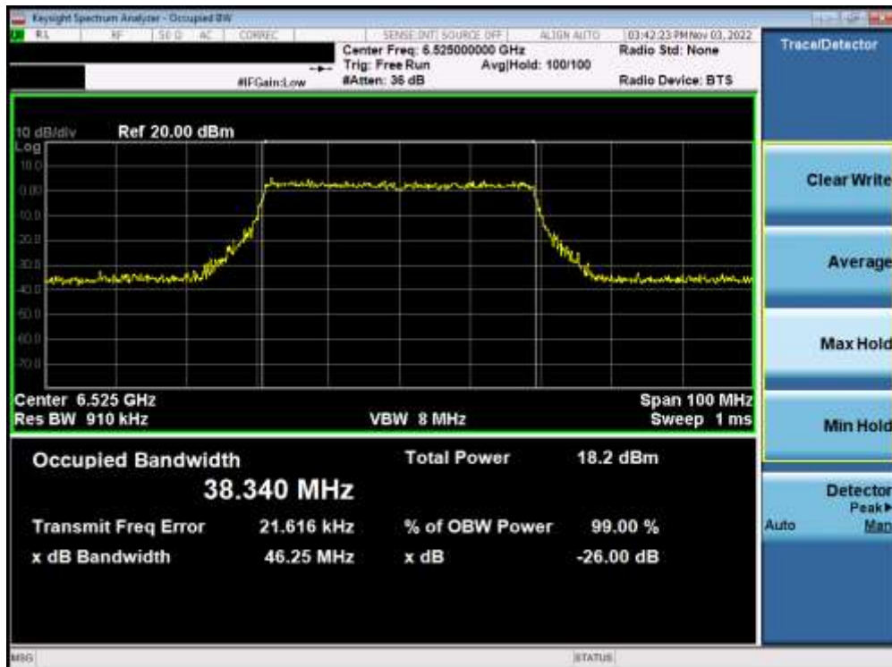
Plot 7-81. Occupied Bandwidth Plot MIMO ANT1 (40MHz BW 802.11ax (Full Tone) (UNII Band 6) – Ch. 115) – LPI
