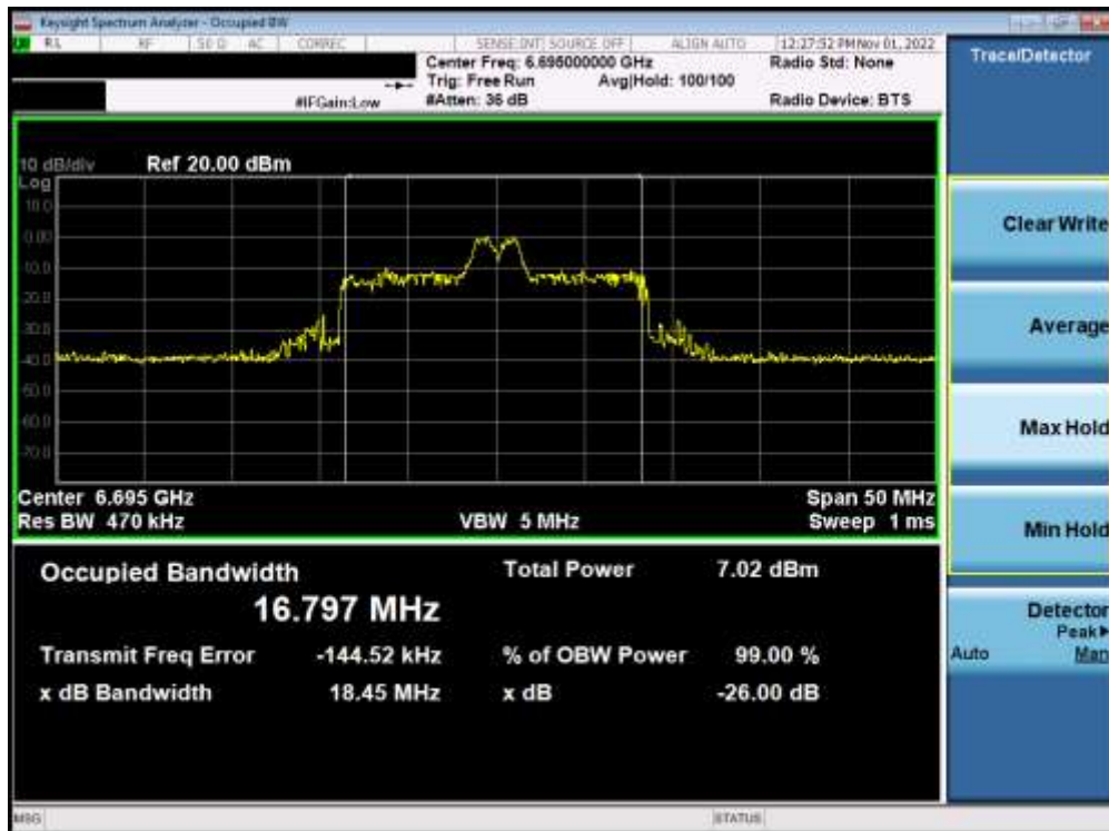
Plot 7-22. Occupied Bandwidth Plot MIMO ANT1 (20MHz BW 802.11ax (26 Tones) (UNII Band 7) – Ch. 149) – LPI
