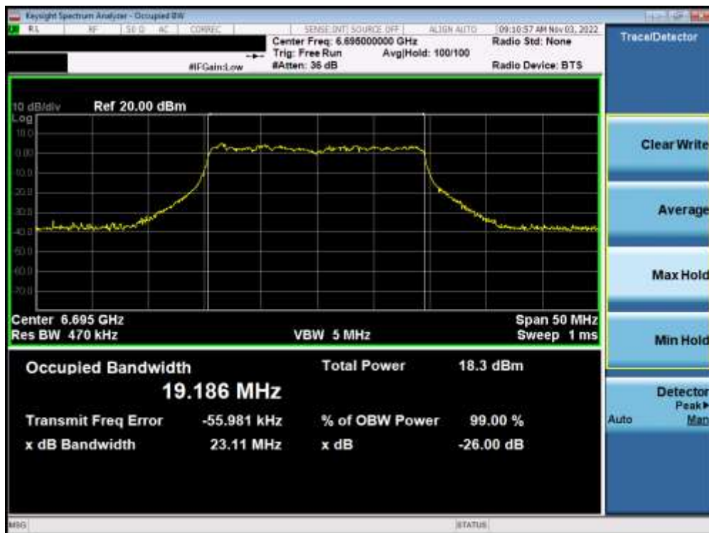
Plot 7-85. Occupied Bandwidth Plot MIMO ANT1 (20MHz BW 802.11ax (Full Tone) (UNII Band 7) – Ch. 149) – LPI/SP
