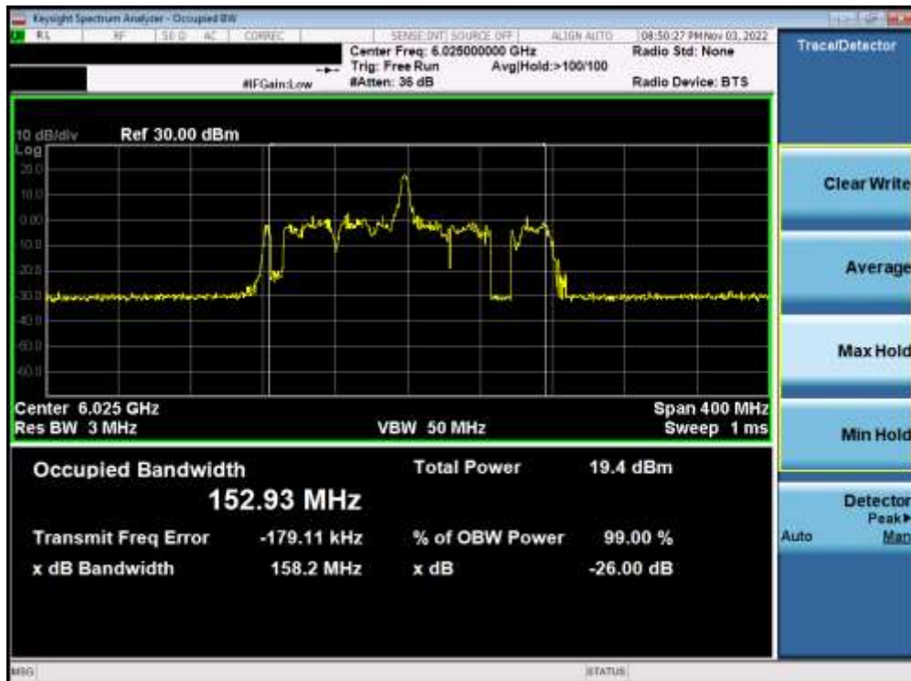
Plot 7-153. Occupied Bandwidth Plot MIMO ANT2 (160MHz BW 802.11ax (26 Tones) (UNII Band 5) – Ch. 15) - SP
