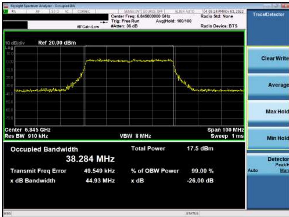
Plot 7-89. Occupied Bandwidth Plot MIMO ANT1 (40MHz BW 802.11ax (Full Tone) (UNII Band 7) – Ch. 179) – LPI/SP
