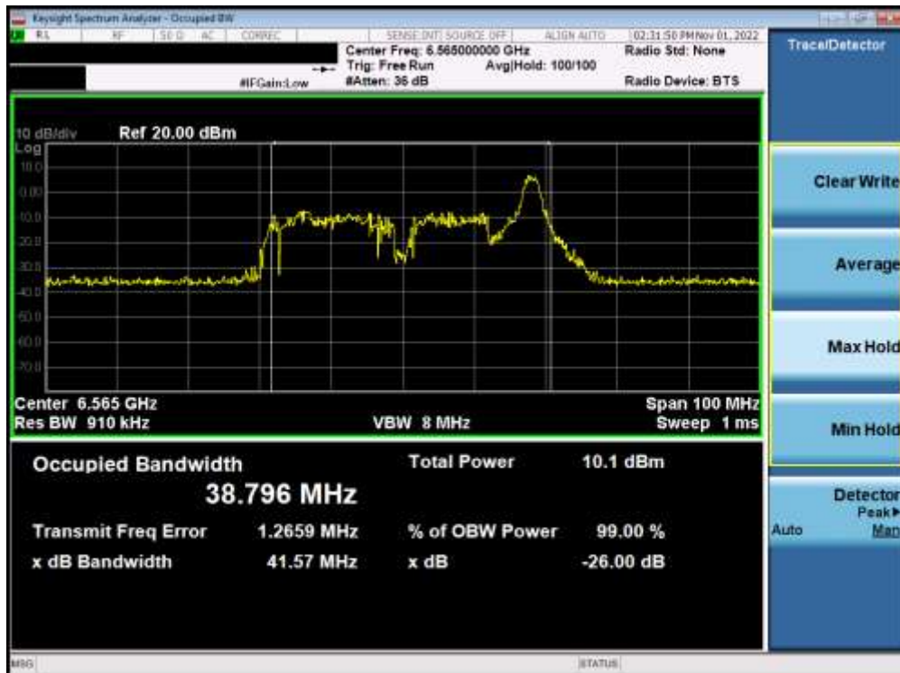
Plot 7-127. Occupied Bandwidth Plot MIMO ANT2 (40MHz BW 802.11ax (26 Tones) (UNII Band 7) – Ch. 123) – LPI
