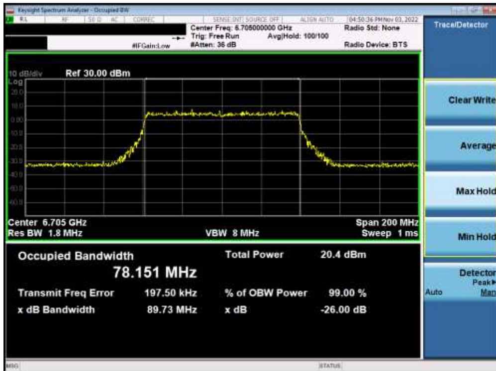
Plot 7-91. Occupied Bandwidth Plot MIMO ANT1 (80MHz BW 802.11ax (Full Tone) (UNII Band 7) – Ch. 151) – LPI/SP
