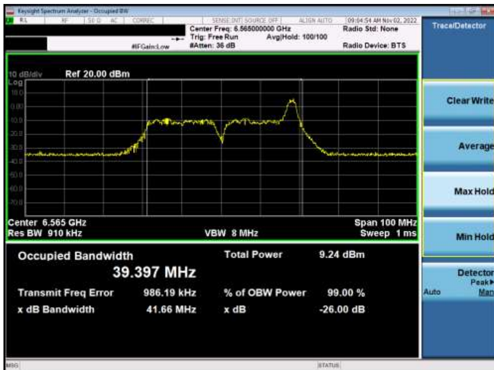
Plot 7-24. Occupied Bandwidth Plot MIMO ANT1 (40MHz BW 802.11ax (26 Tones) (UNII Band 7) – Ch. 123) – LPI
