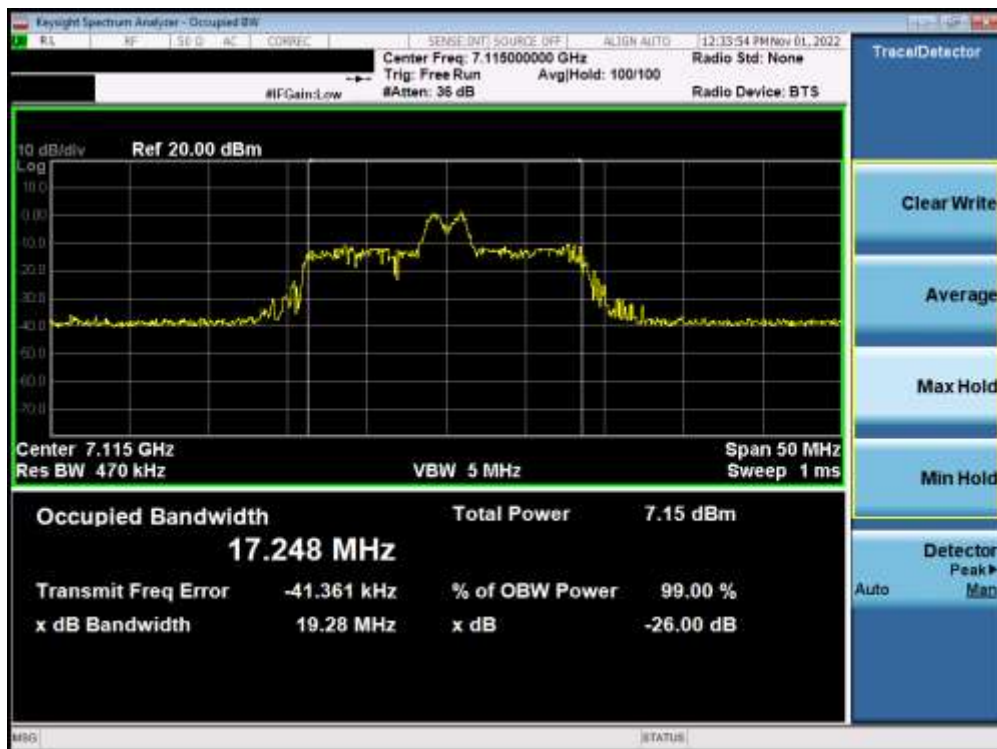
Plot 7-34. Occupied Bandwidth Plot MIMO ANT1 (20MHz BW 802.11ax (26 Tones) (UNII Band 8) – Ch. 233) – LPI
