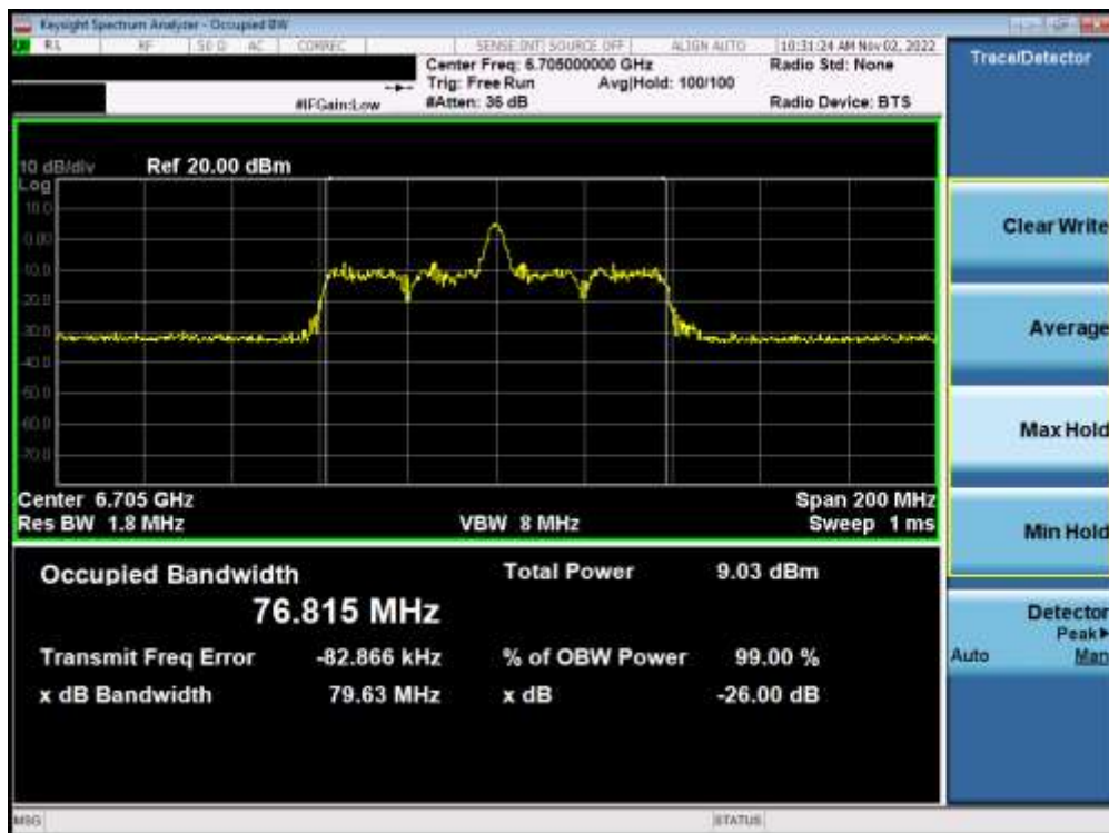
Plot 7-28. Occupied Bandwidth Plot MIMO ANT1 (80MHz BW 802.11ax (26 Tones) (UNII Band 7) – Ch. 151) – LPI
