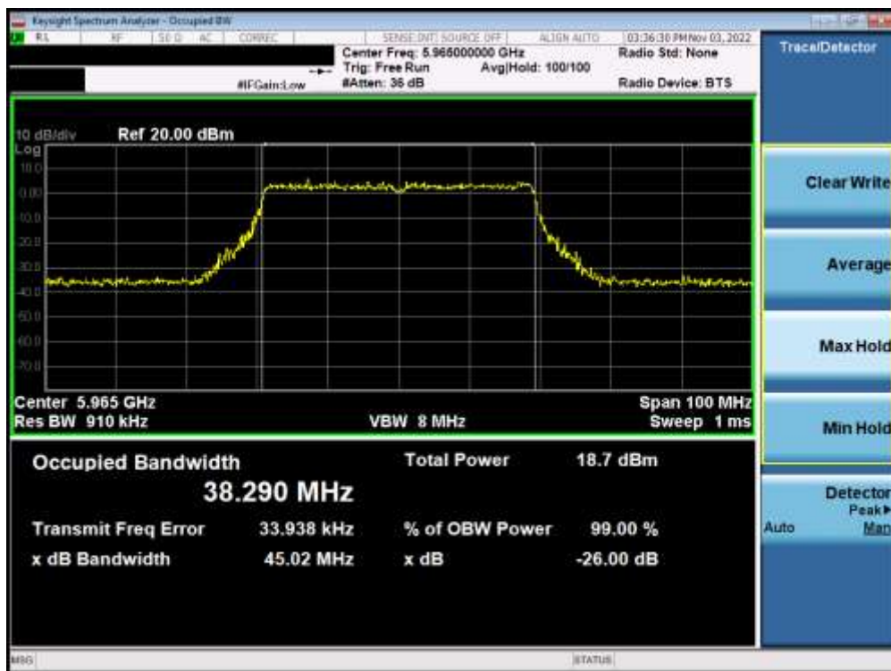
Plot 7-67. Occupied Bandwidth Plot MIMO ANT1 (40MHz BW 802.11ax (Full Tone) (UNII Band 5) – Ch. 3) – LPI/SP
