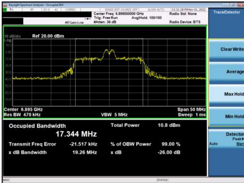
Plot 7-32. Occupied Bandwidth Plot MIMO ANT1 (20MHz BW 802.11ax (26 Tones) (UNII Band 8) – Ch. 189) – LPI
