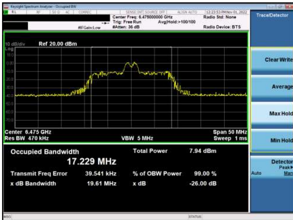
Plot 7-14. Occupied Bandwidth Plot MIMO ANT1 (20MHz BW 802.11ax (26 Tones) (UNII Band 6) – Ch. 105) – LPI
