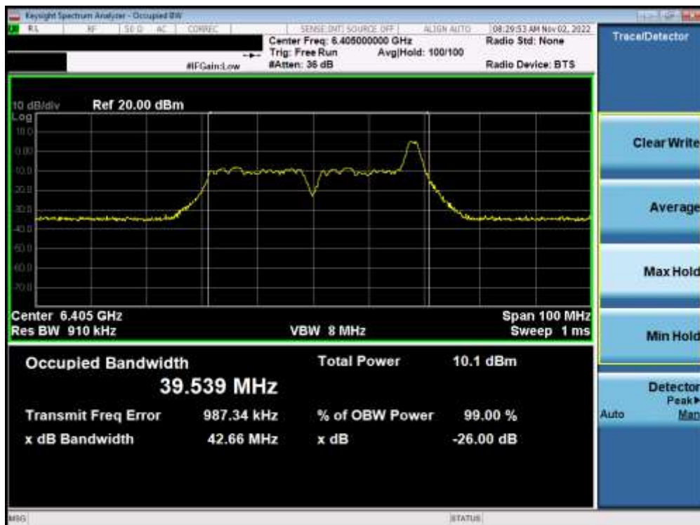
Plot 7-6. Occupied Bandwidth Plot MIMO ANT1 (40MHz BW 802.11ax (26 Tones) (UNII Band 5) – Ch. 91) – LPI
