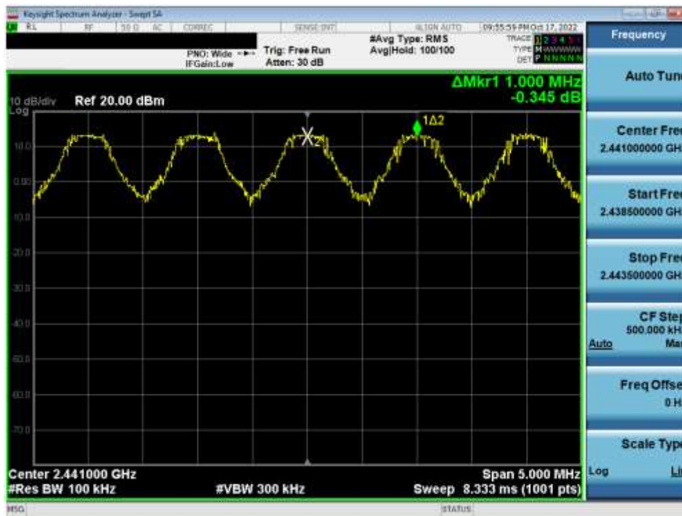
Plot 7-64. Channel Spacing Plot (Bluetooth) – ANT 2
