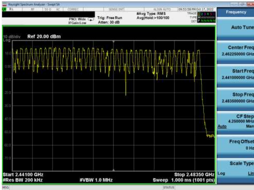
Plot 7-70. High End Spectrum Channel Hopping Plot (Bluetooth) – ANT 2
