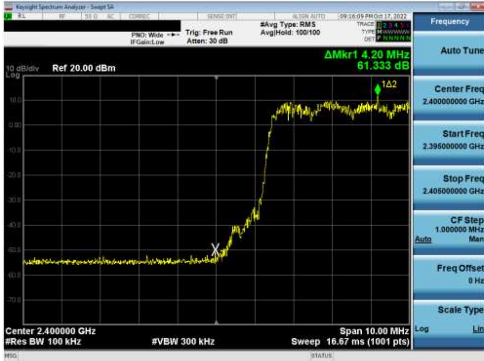
Plot 7-57. Band Edge Plot (Bluetooth with Hopping Enabled, 3 Mbps – Ch. 0) – Ant 1
