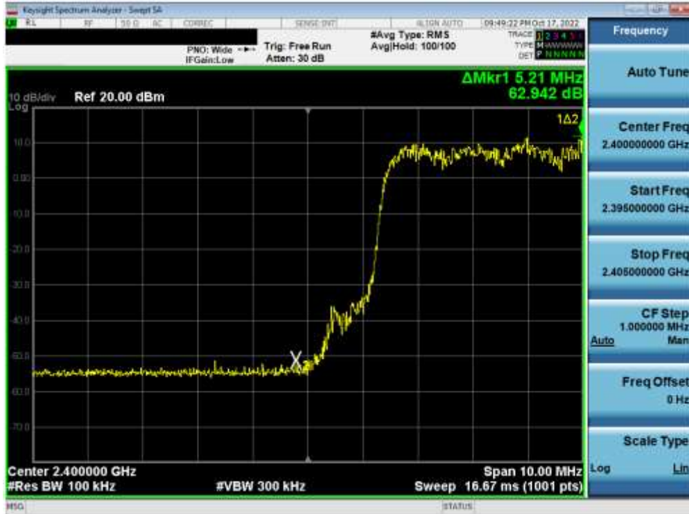
Plot 7-61. Band Edge Plot (Bluetooth with Hopping Enabled, 3Mbps – Ch. 0) – ANT 2
