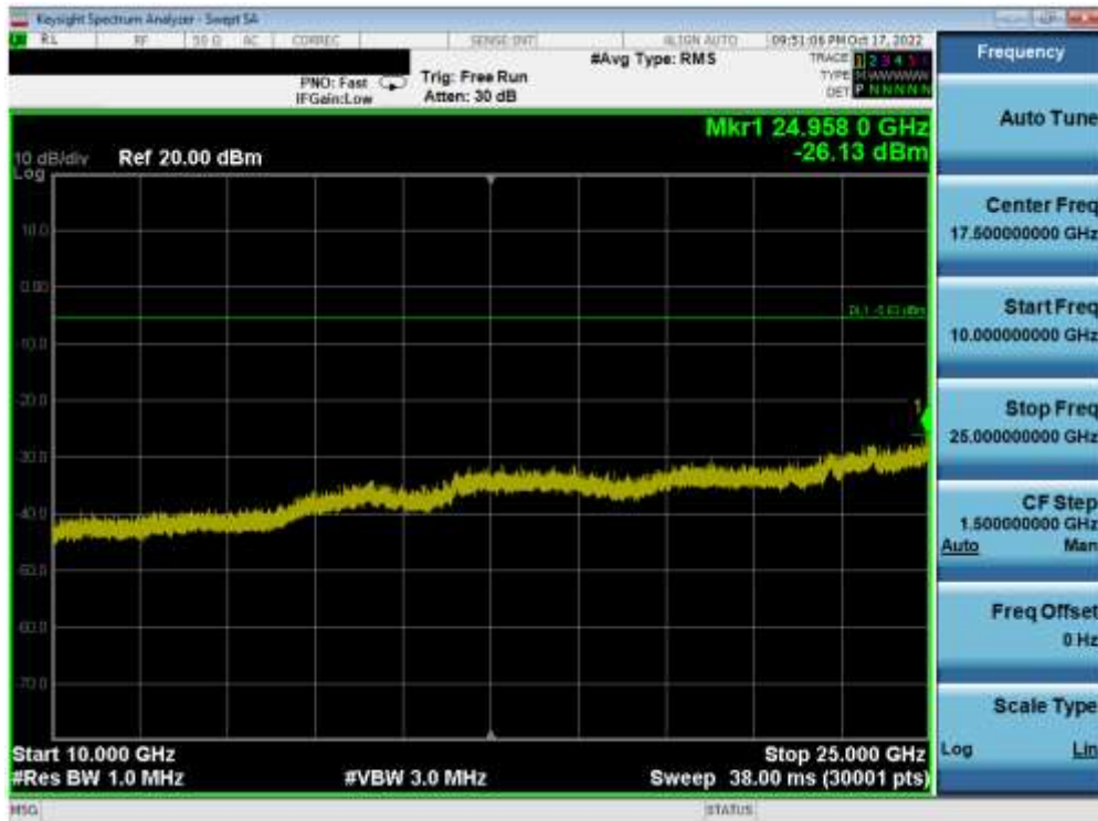
Plot 7-78. Conducted Spurious Plot (Bluetooth, 1Mbps – Ch. 0) – ANT 2
