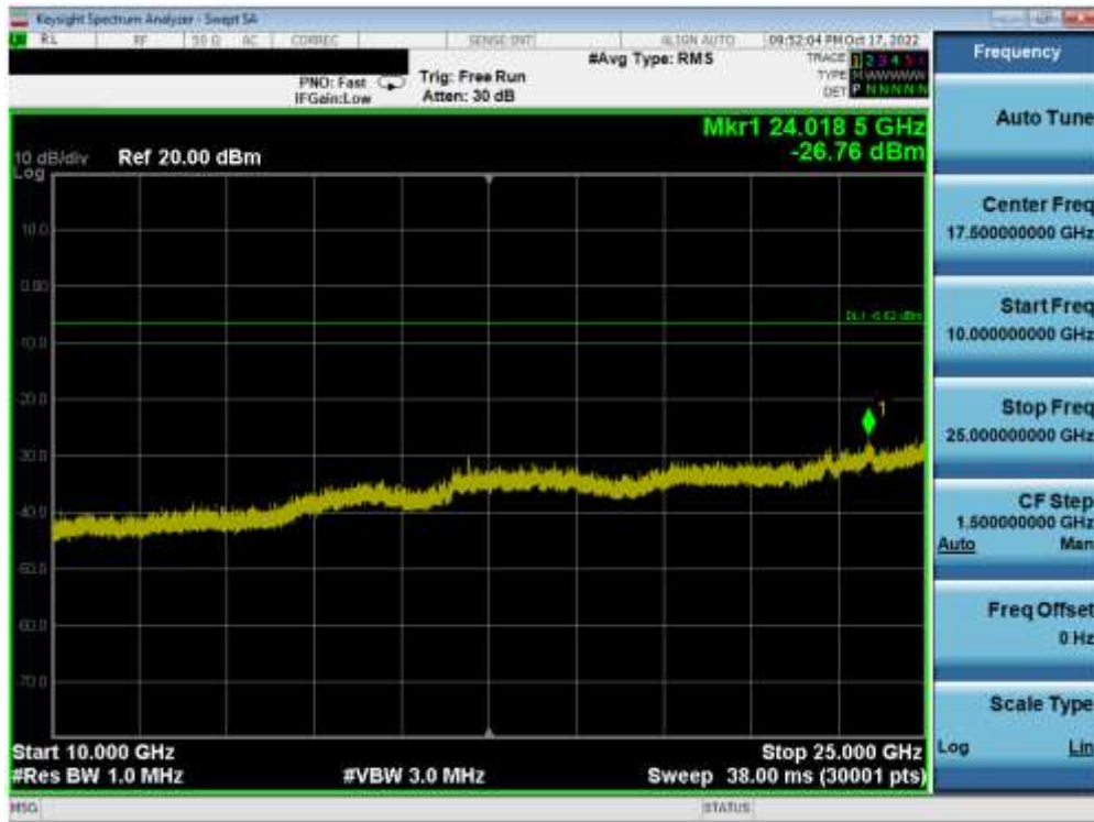
Plot 7-80. Conducted Spurious Plot (Bluetooth, 1Mbps – Ch. 39) – ANT 2
