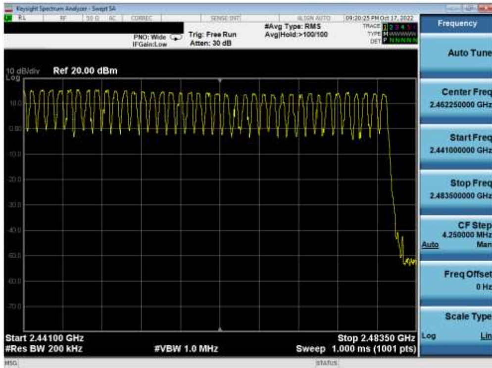
Plot 7-68. High End Spectrum Channel Hopping Plot (Bluetooth) – Ant 1
