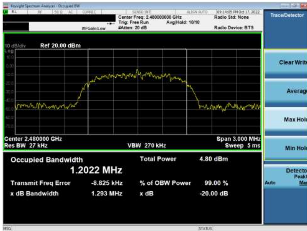
Plot 7-9. 20dB Bandwidth Plot (Bluetooth, 3Mbps – Ch. 78) – Ant 1
