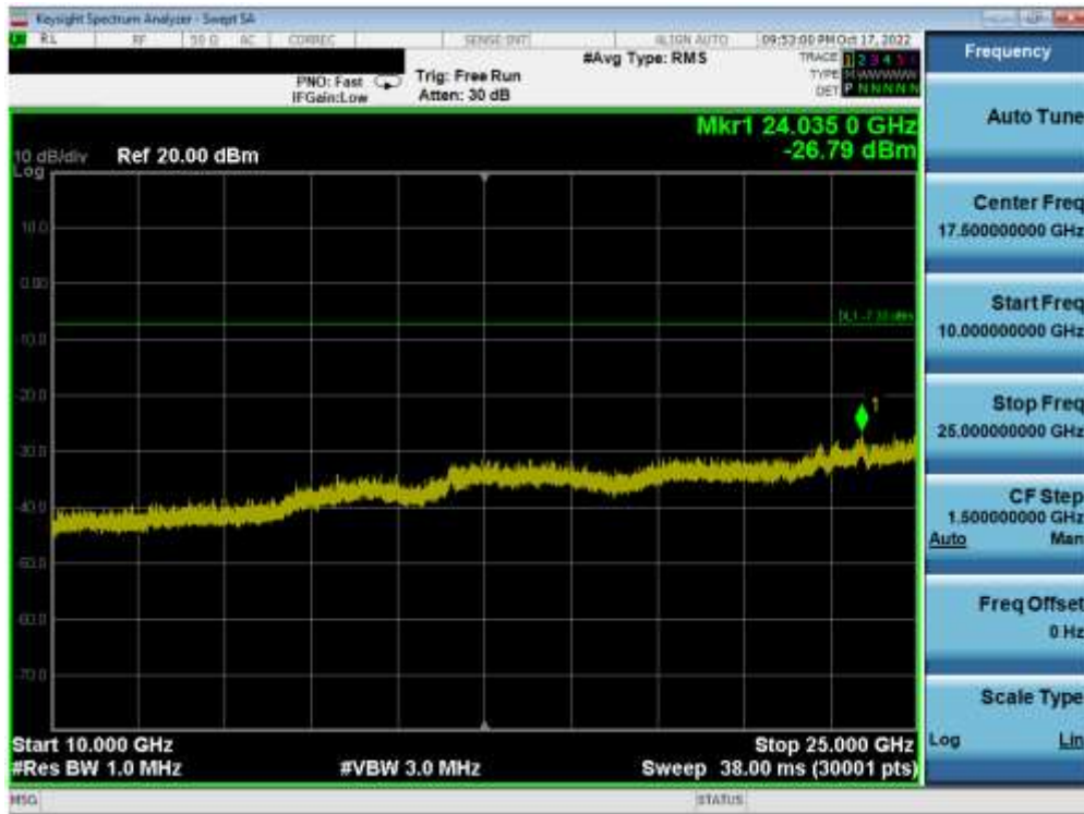
Plot 7-82. Conducted Spurious Plot (Bluetooth, 1Mbps – Ch. 78) – ANT 2
