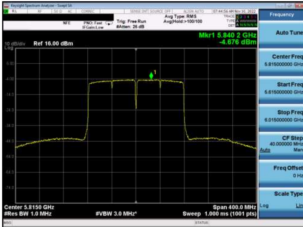
Plot 7-259. Power Spectral Density Plot MIMO ANT1 (160MHz BW 802.11ac (UNII Band 3/4) – Ch. 163)
