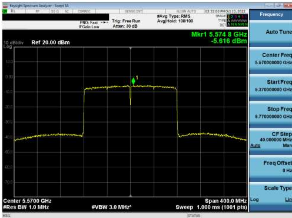
Plot 7-228. Power Spectral Density Plot MIMO ANT1 (160MHz BW 802.11ax (UNII Band 2C) – Ch. 114)
