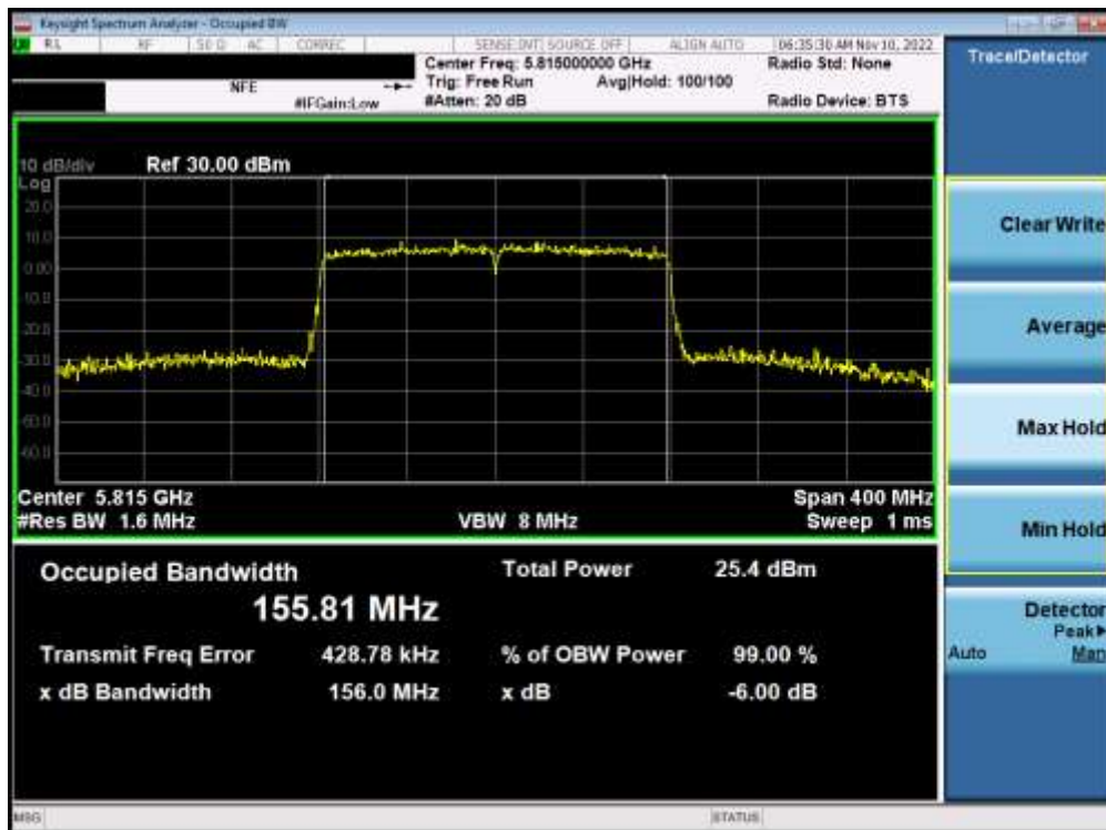
Plot 7-174. 6dB Bandwidth Plot MIMO ANT2 (160MHz BW 802.11ax (UNII Band 3/4) – Ch. 163)
