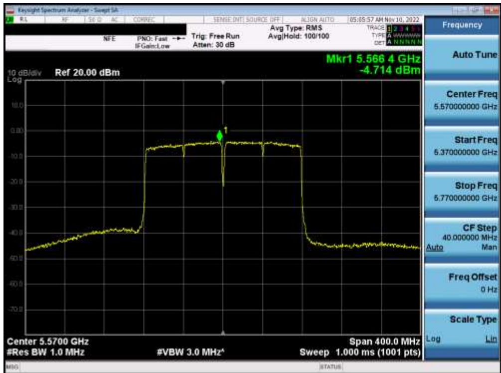
Plot 7-314. Power Spectral Density Plot MIMO ANT2 (160MHz BW 802.11ax (UNII Band 2C) – Ch. 114)
