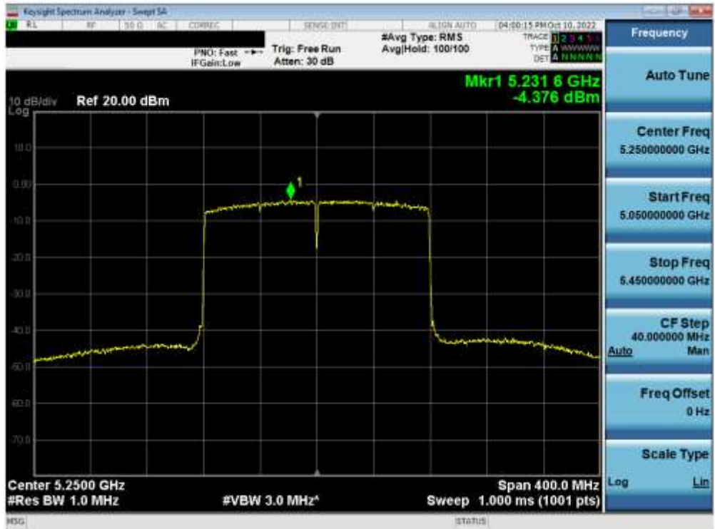
Plot 7-277. Power Spectral Density Plot MIMO ANT2 (160MHz BW 802.11ax (UNII Band 1/2A) – Ch. 50)
