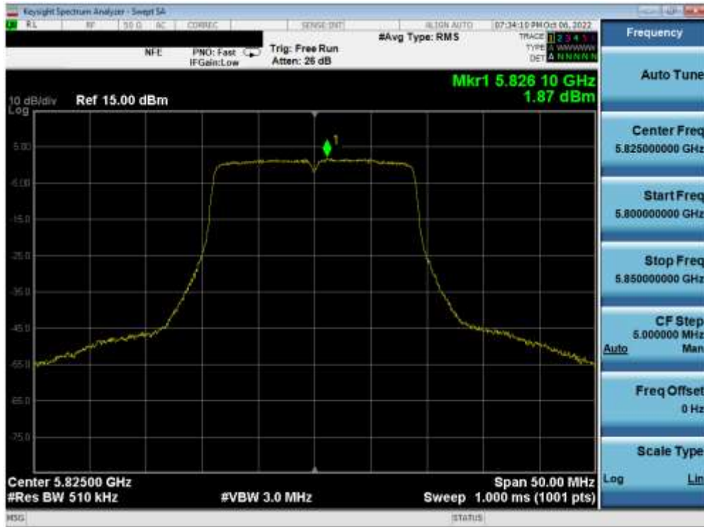
Plot 7-321. Power Spectral Density Plot MIMO ANT2 (20MHz BW 802.11n (UNII Band 3) – Ch. 165)
