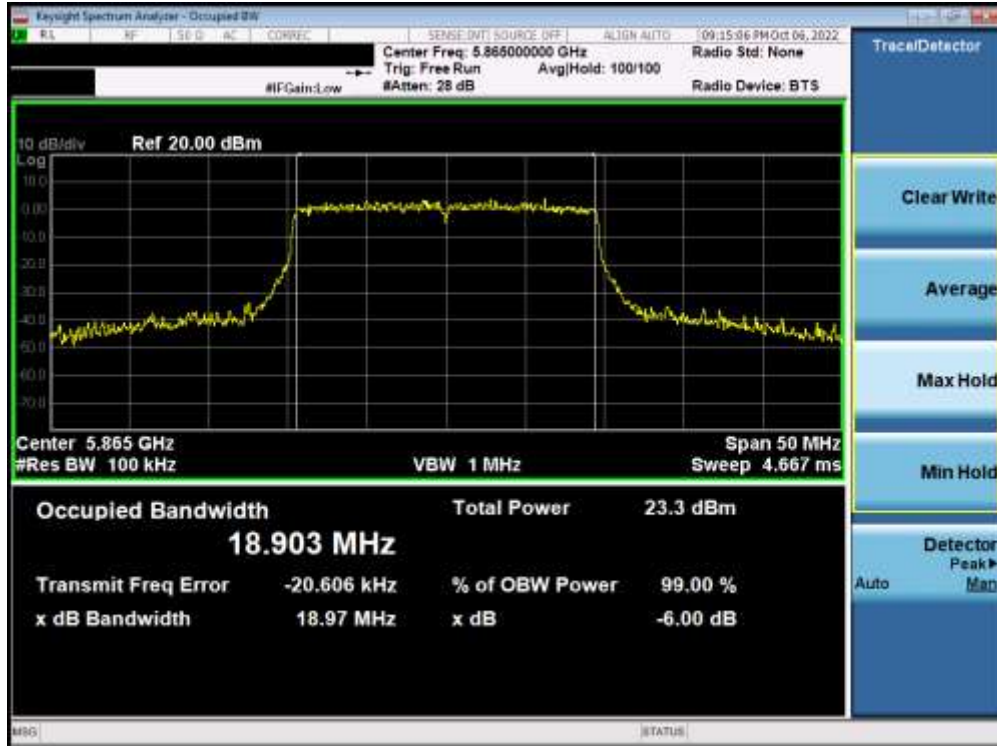
Plot 7-165. 6dB Bandwidth Plot MIMO ANT2 (20MHz BW 802.11ax (UNII Band 4) – Ch. 173)
