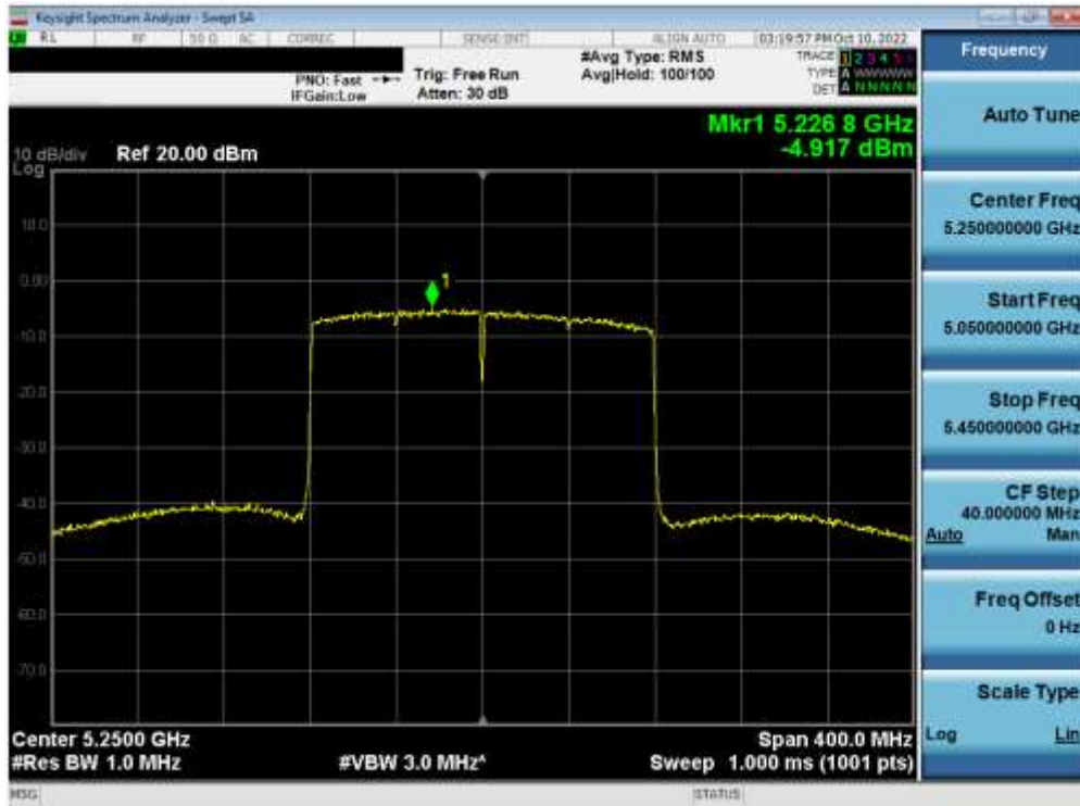
Plot 7-191. Power Spectral Density Plot MIMO ANT1 (160MHz BW 802.11ax (UNII Band 1/2A) – Ch. 50)
