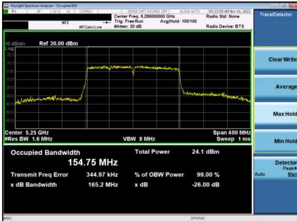
Plot 7-16. 26dB Bandwidth Plot ANT1 (160MHz BW 802.11ac (UNII Band 1) – Ch. 50)
