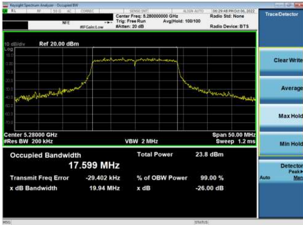
Plot 7-22. 26dB Bandwidth Plot ANT1 (20MHz BW 802.11n (UNII Band 2A) – Ch. 56)
