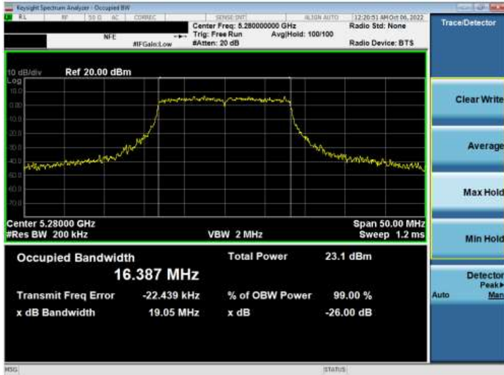
Plot 7-74. 26dB Bandwidth Plot ANT2 (802.11a (UNII Band 2A) – Ch. 56)
