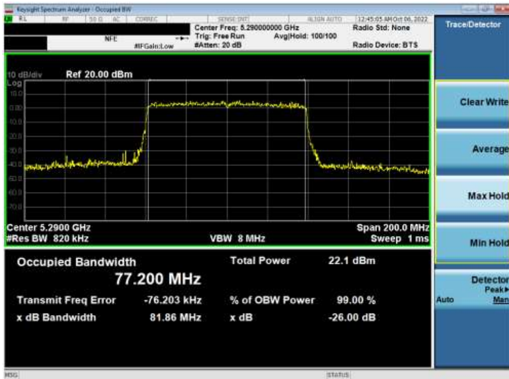
Plot 7-32. 26dB Bandwidth Plot ANT1 (80MHz BW 802.11ax (UNII Band 2A) – Ch. 58)
