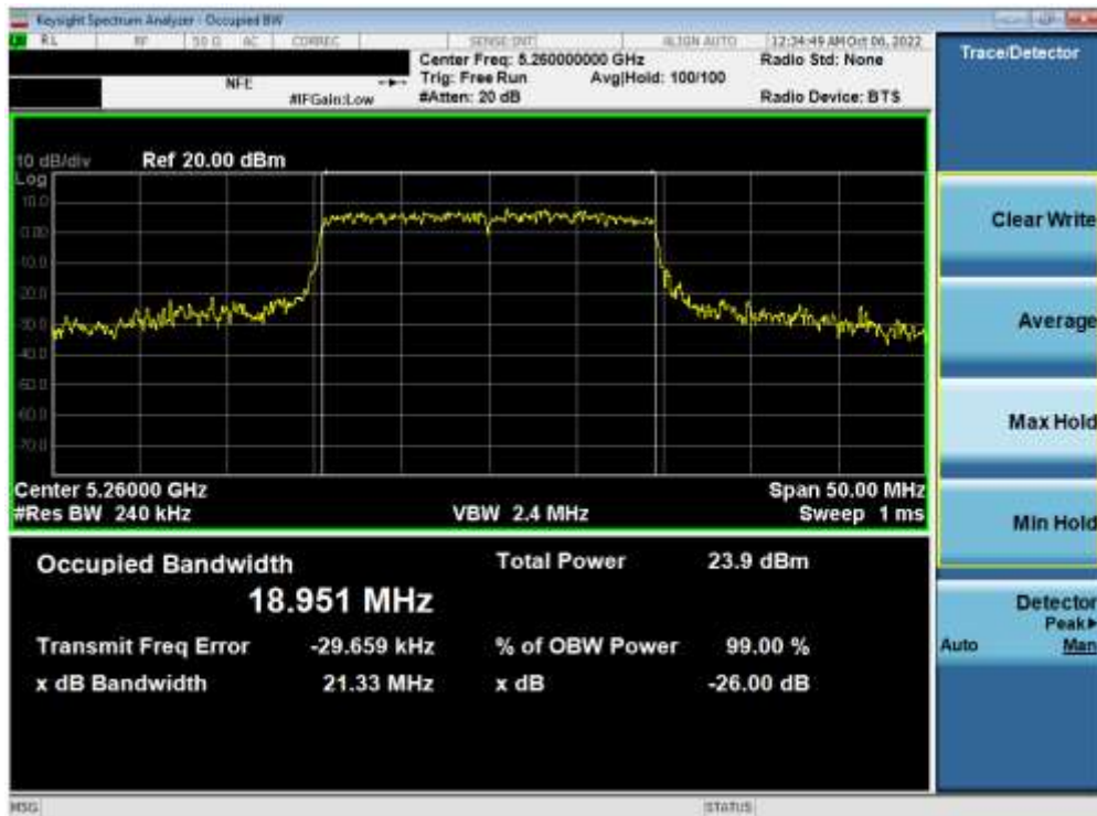
Plot 7-24. 26dB Bandwidth Plot ANT1 (20MHz BW 802.11ax (UNII Band 2A) – Ch. 52)
