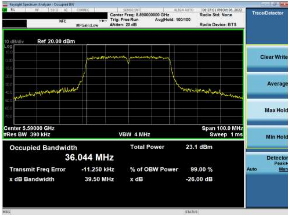
Plot 7-43. 26dB Bandwidth Plot ANT1 (40MHz BW 802.11n (UNII Band 2C) – Ch. 118)
