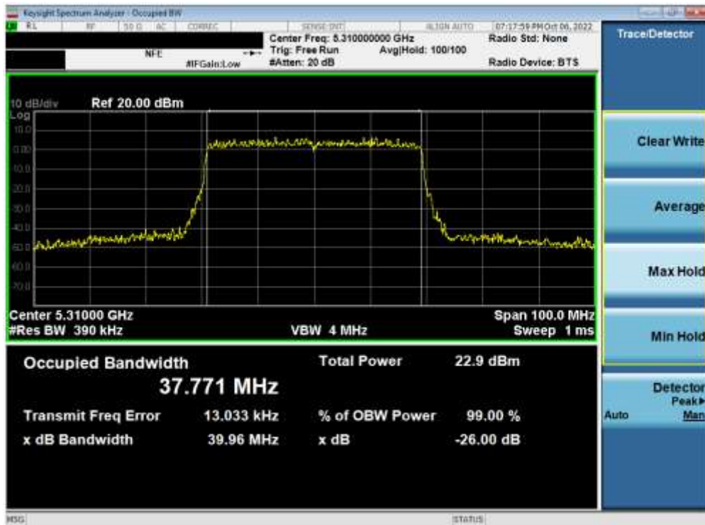
Plot 7-85. 26dB Bandwidth Plot ANT2 (40MHz BW 802.11ax (UNII Band 2A) – Ch. 62)
