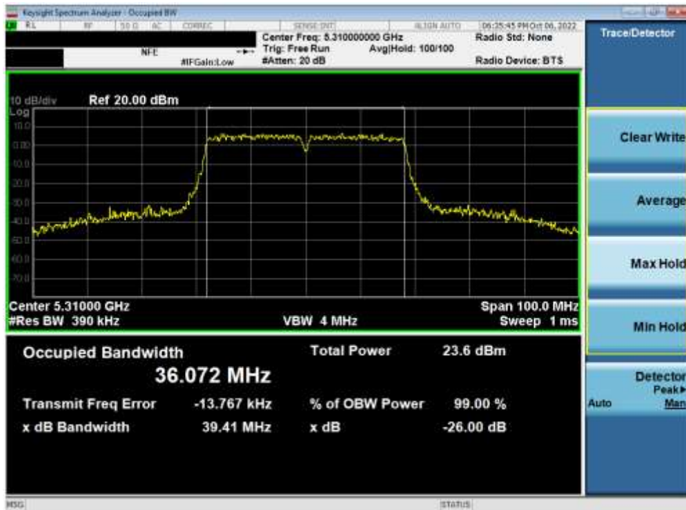
Plot 7-28. 26dB Bandwidth Plot ANT1 (40MHz BW 802.11n (UNII Band 2A) – Ch. 62)
