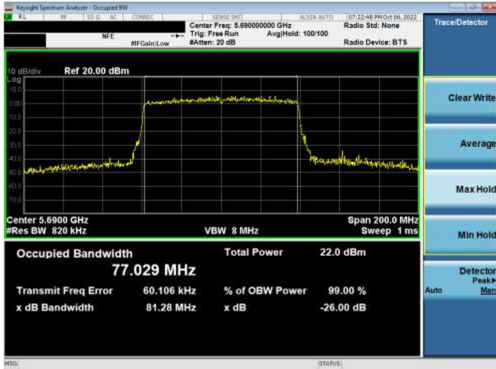
Plot 7-108. 26dB Bandwidth Plot ANT2 (80MHz BW 802.11ax (UNII Band 2C) – Ch. 138)
