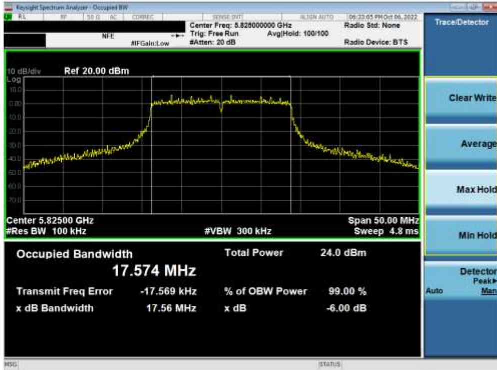
Plot 7-116. 6dB Bandwidth Plot ANT1 (20MHz BW 802.11n (UNII Band 3) – Ch. 165)
