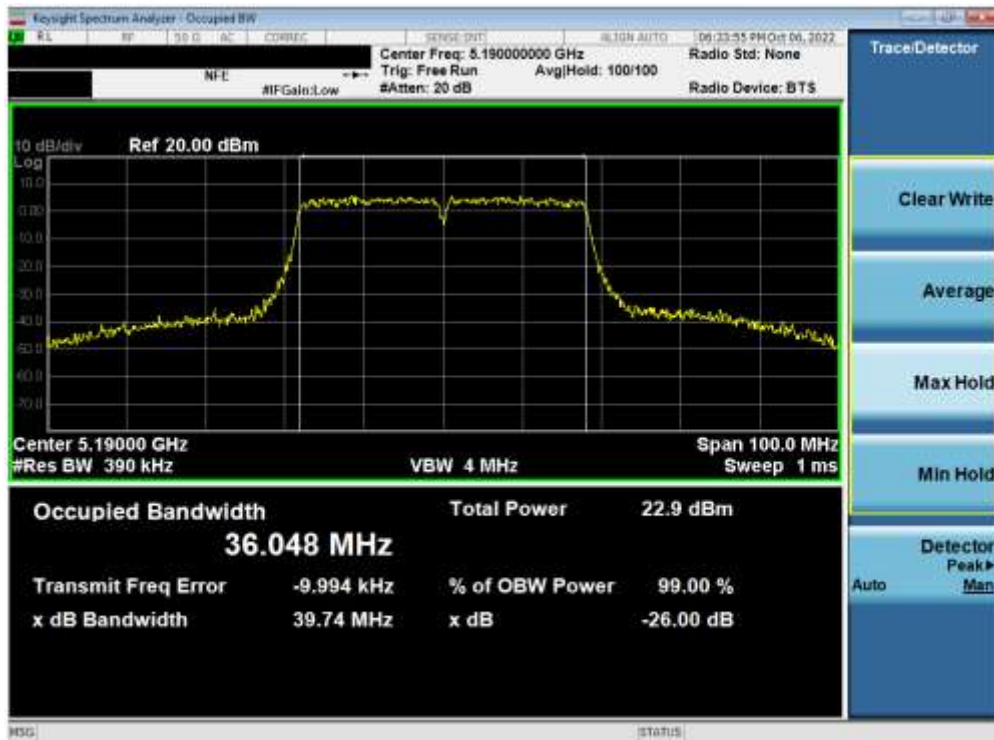
Plot 7-10. 26dB Bandwidth Plot ANT1 (40MHz BW 802.11n (UNII Band 1) – Ch. 38)
