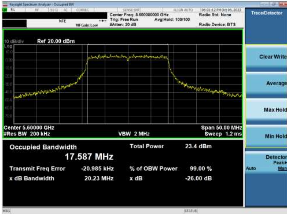
Plot 7-37. 26dB Bandwidth Plot ANT1 (20MHz BW 802.11n (UNII Band 2C) – Ch. 120)
