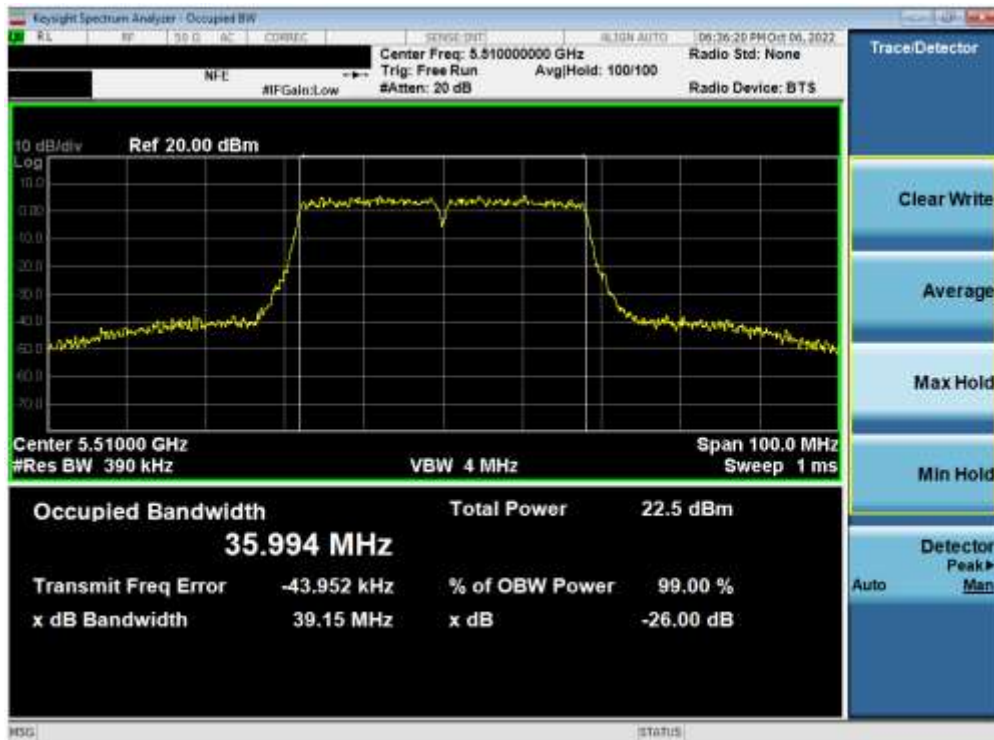
Plot 7-42. 26dB Bandwidth Plot ANT1 (40MHz BW 802.11n (UNII Band 2C) – Ch. 102)
