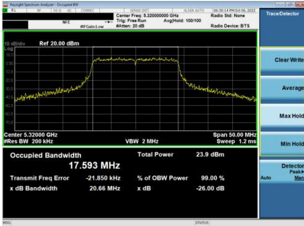
Plot 7-23. 26dB Bandwidth Plot ANT1 (20MHz BW 802.11n (UNII Band 2A) – Ch. 64)
