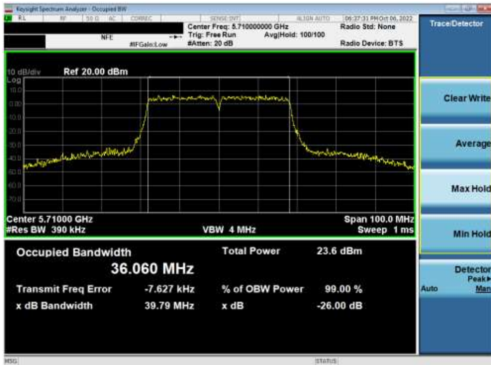
Plot 7-44. 26dB Bandwidth Plot ANT1 (40MHz BW 802.11n (UNII Band 2C) – Ch. 142)
