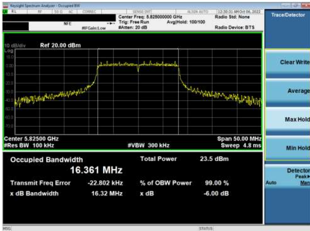
Plot 7-113. 6dB Bandwidth Plot ANT1 (802.11a (UNII Band 3) – Ch. 165)
