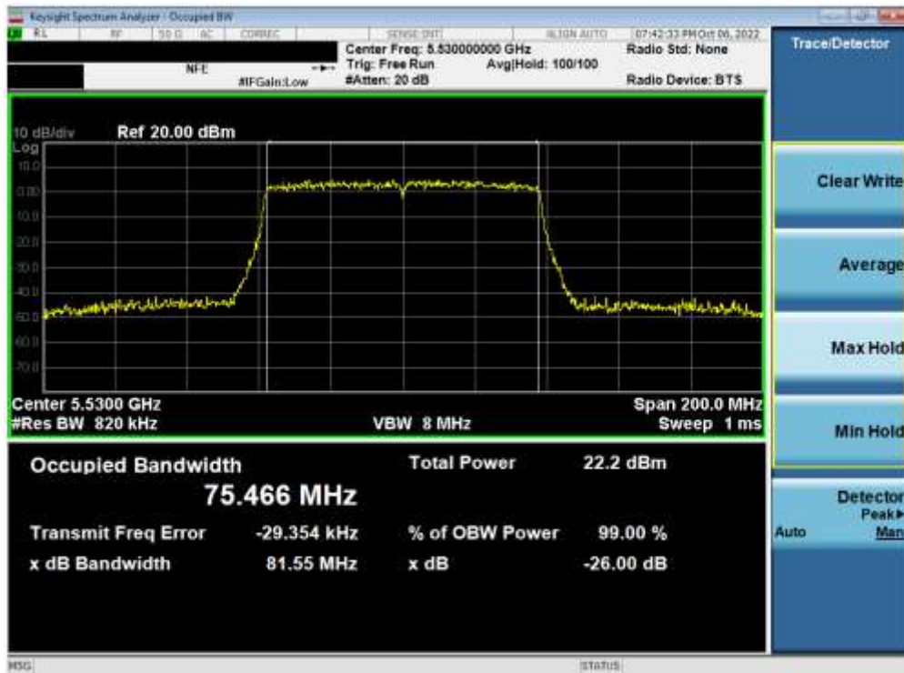
Plot 7-103. 26dB Bandwidth Plot ANT2 (80MHz BW 802.11ac (UNII Band 2C) – Ch. 106)
