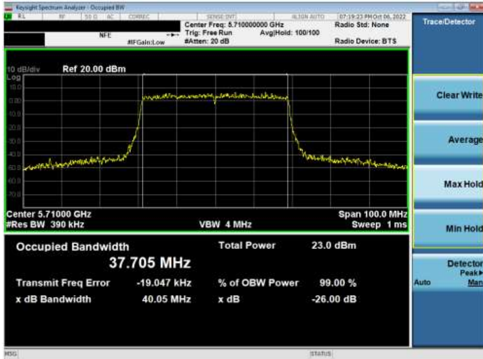
Plot 7-102. 26dB Bandwidth Plot ANT2 (40MHz BW 802.11ax (UNII Band 2C) – Ch. 142)
