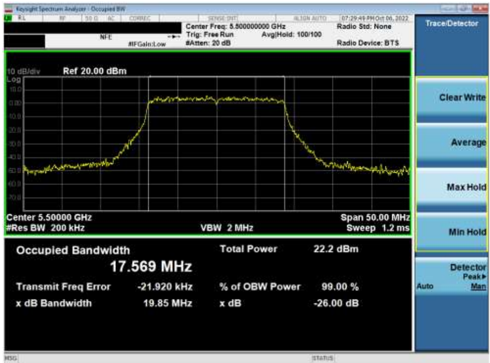
Plot 7-91. 26dB Bandwidth Plot ANT2 (20MHz BW 802.11n (UNII Band 2C) – Ch. 100)
