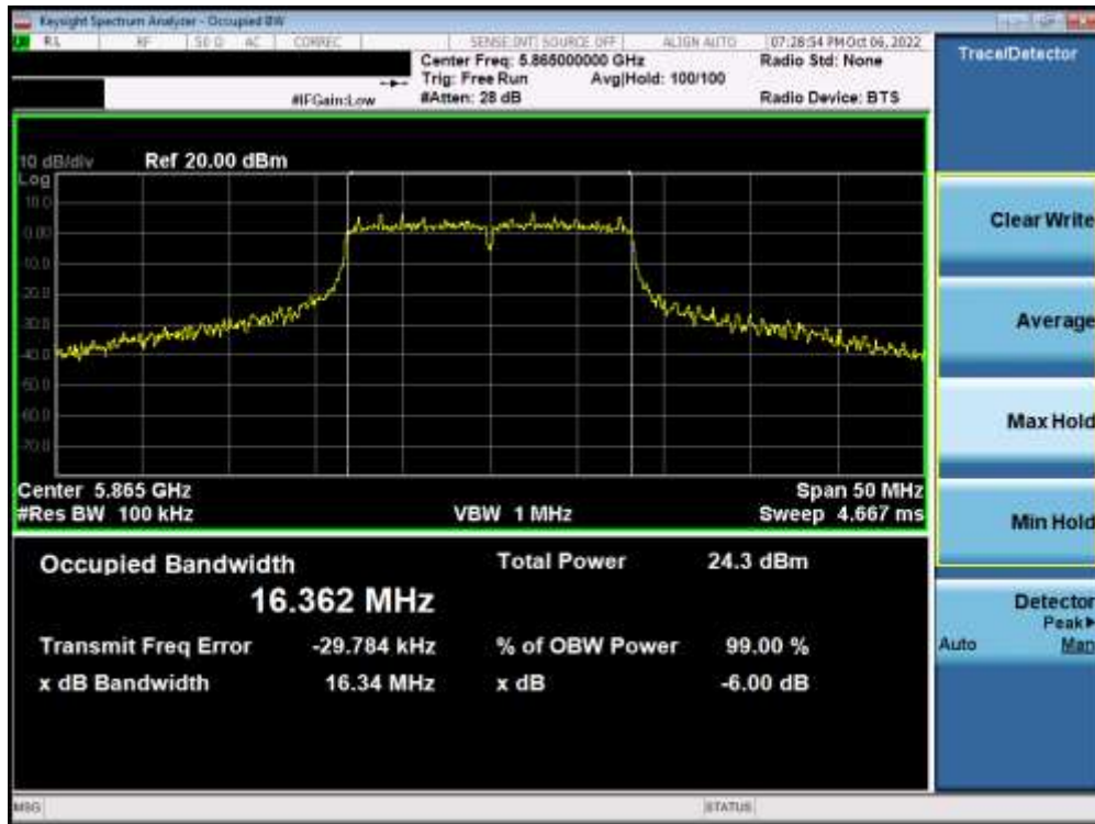
Plot 7-127. 6dB Bandwidth Plot MIMO ANT1 (802.11a (UNII Band 4) – Ch. 173)
