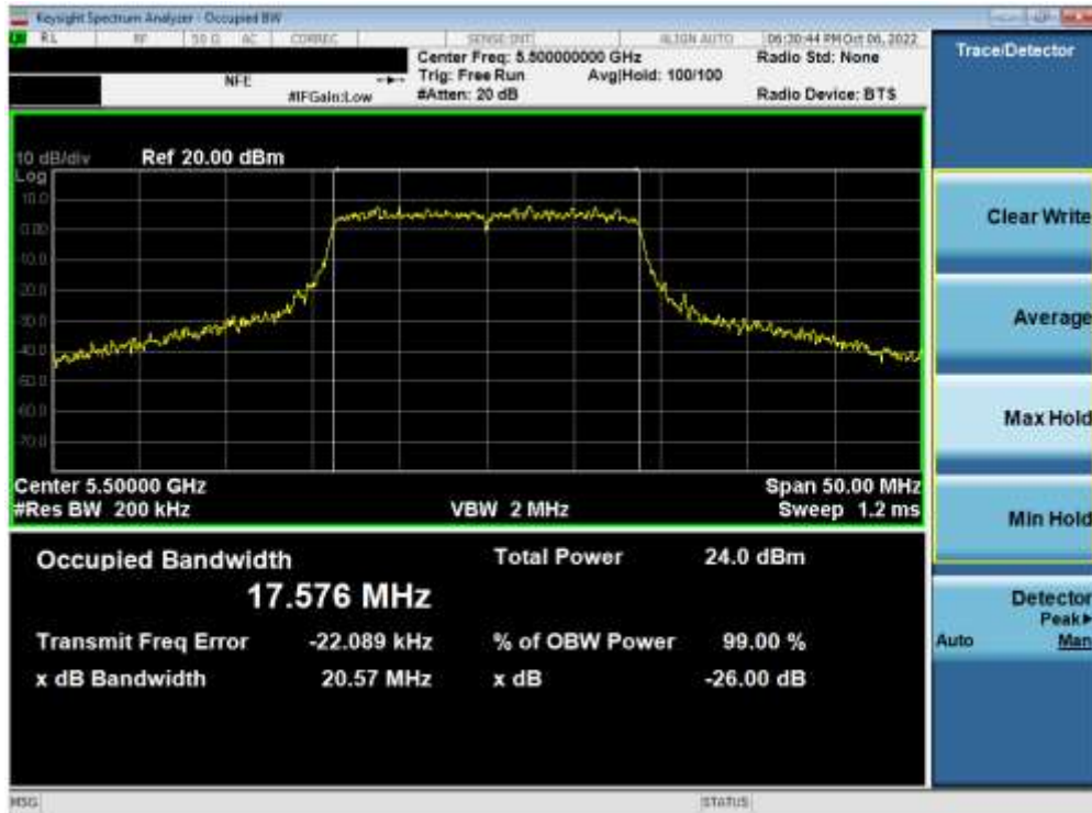
Plot 7-36. 26dB Bandwidth Plot ANT1 (20MHz BW 802.11n (UNII Band 2C) – Ch. 100)
