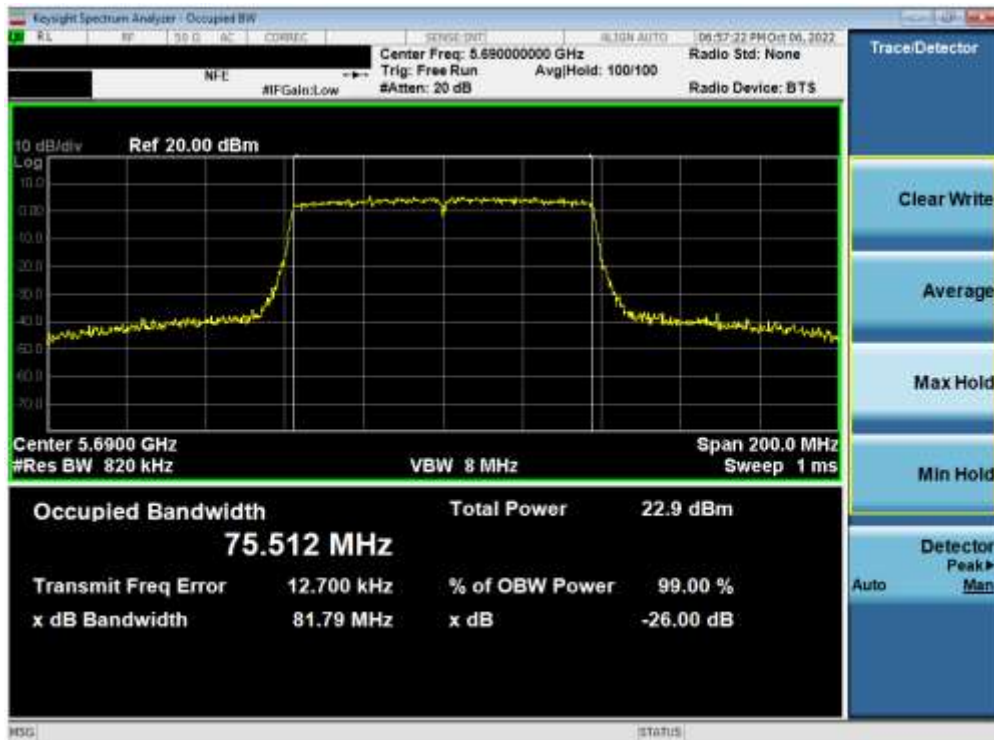
Plot 7-50. 26dB Bandwidth Plot ANT1 (80MHz BW 802.11ac (UNII Band 2C) – Ch. 138)
