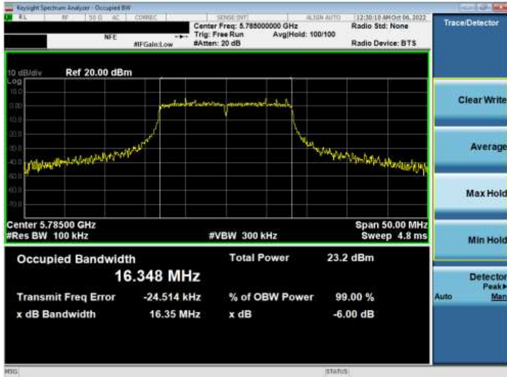
Plot 7-112. 6dB Bandwidth Plot ANT1 (802.11a (UNII Band 3) – Ch. 157)
