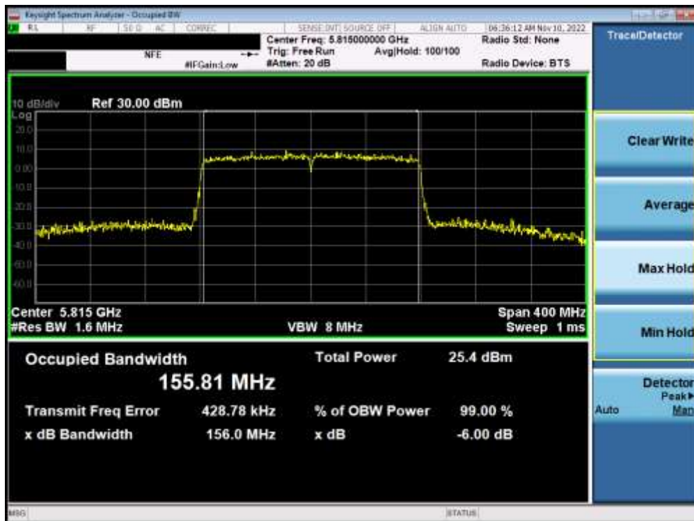
Plot 7-142. 6dB Bandwidth Plot MIMO ANT1 (160MHz BW 802.11ax (UNII Band 3/4) – Ch. 163)
