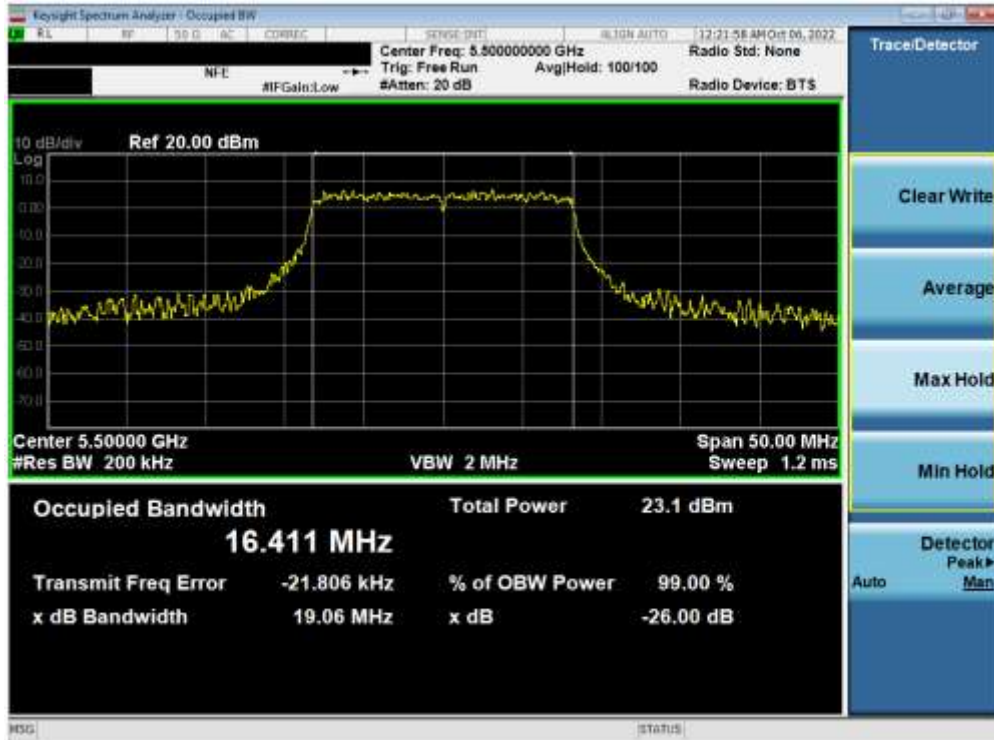
Plot 7-88. 26dB Bandwidth Plot ANT2 (802.11a (UNII Band 2C) – Ch. 100)
