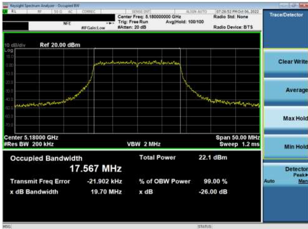
Plot 7-59. 26dB Bandwidth Plot ANT2 (20MHz BW 802.11n (UNII Band 1) – Ch. 36)
