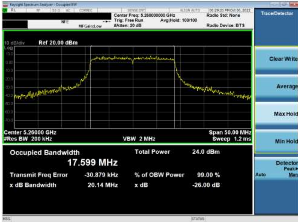
Plot 7-21. 26dB Bandwidth Plot ANT1 (20MHz BW 802.11n (UNII Band 2A) – Ch. 52)
