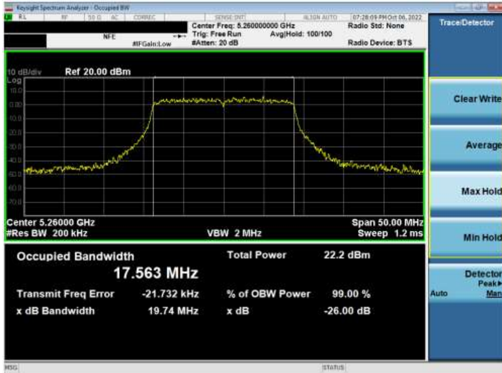
Plot 7-76. 26dB Bandwidth Plot ANT2 (20MHz BW 802.11n (UNII Band 2A) – Ch. 52)
