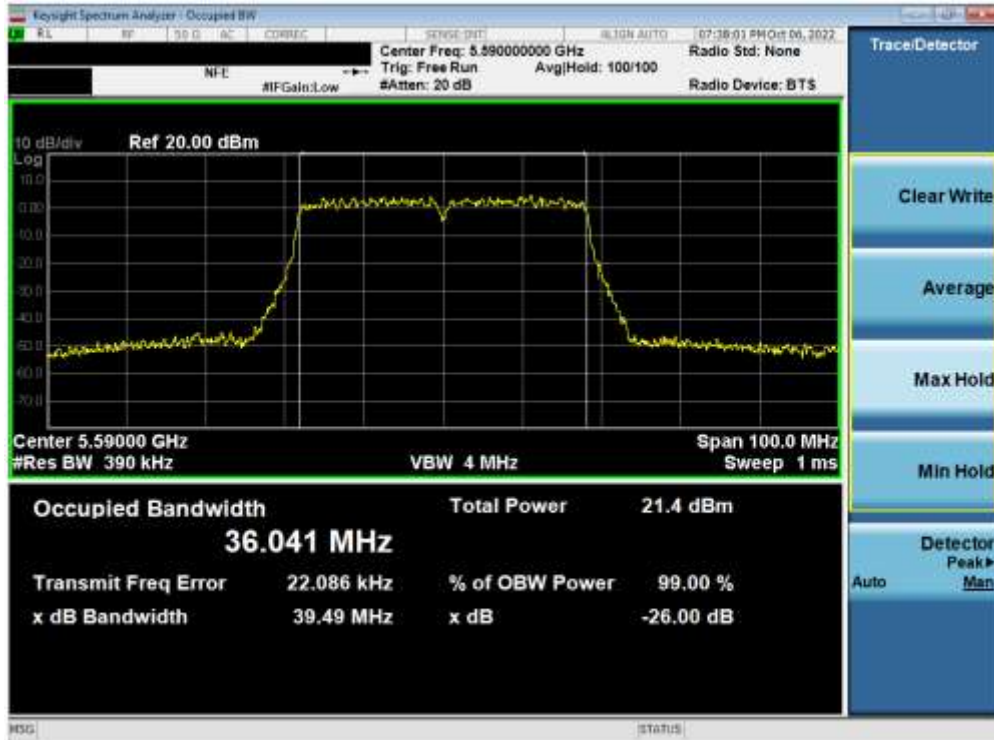
Plot 7-98. 26dB Bandwidth Plot ANT2 (40MHz BW 802.11n (UNII Band 2C) – Ch. 118)
