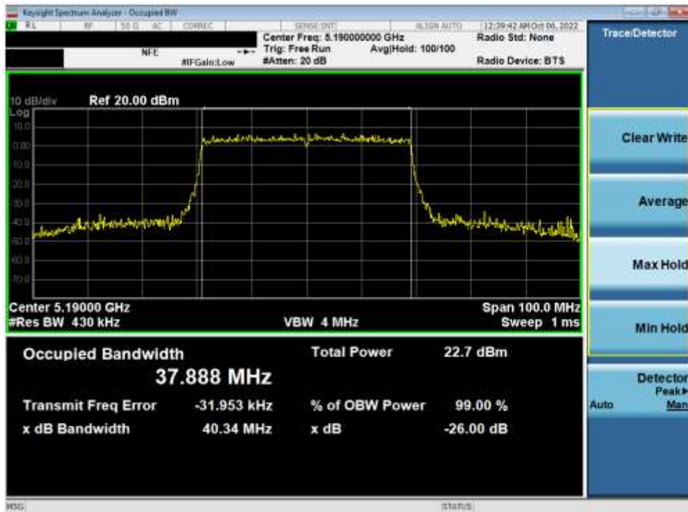
Plot 7-12. 26dB Bandwidth Plot ANT1 (40MHz BW 802.11ax (UNII Band 1) – Ch. 38)
