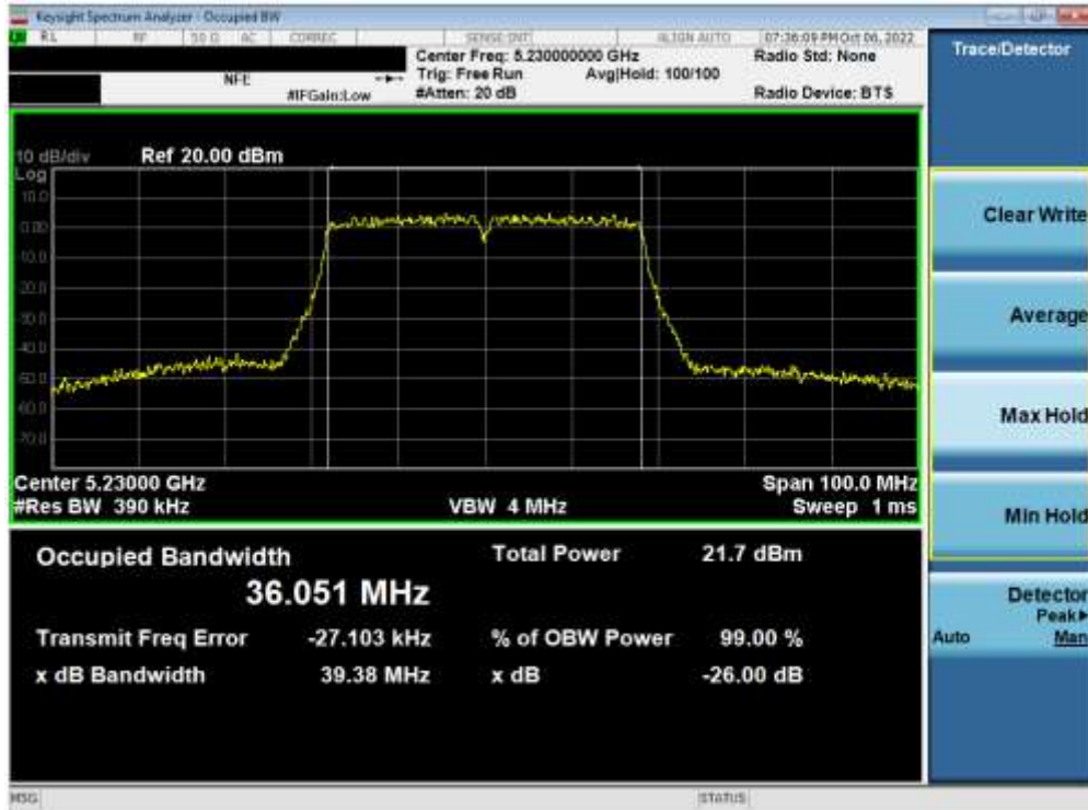
Plot 7-66. 26dB Bandwidth Plot ANT2 (40MHz BW 802.11n (UNII Band 1) – Ch. 46)
