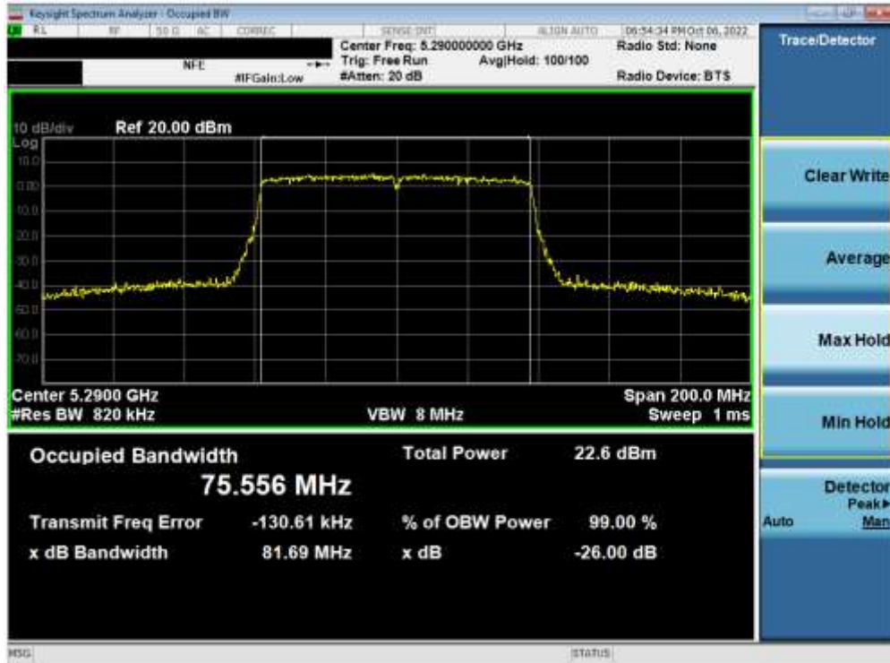
Plot 7-31. 26dB Bandwidth Plot ANT1 (80MHz BW 802.11ac (UNII Band 2A) – Ch. 58)
