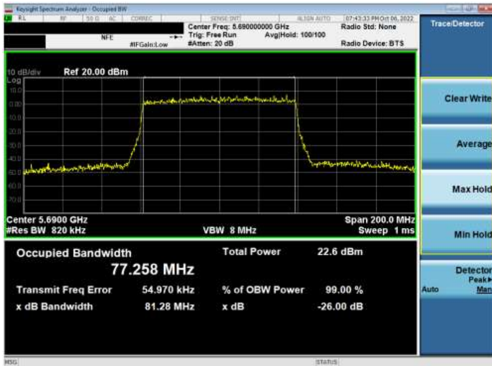
Plot 7-105. 26dB Bandwidth Plot ANT2 (80MHz BW 802.11ac (UNII Band 2C) – Ch. 138)
