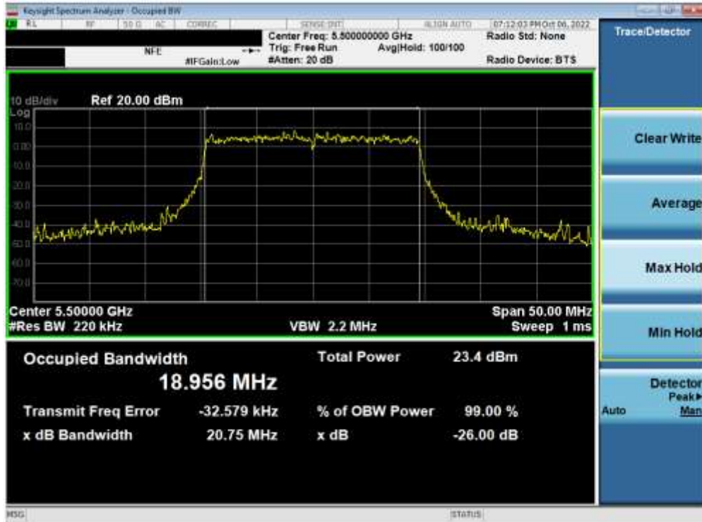
Plot 7-94. 26dB Bandwidth Plot ANT2 (20MHz BW 802.11ax (UNII Band 2C) – Ch. 100)
