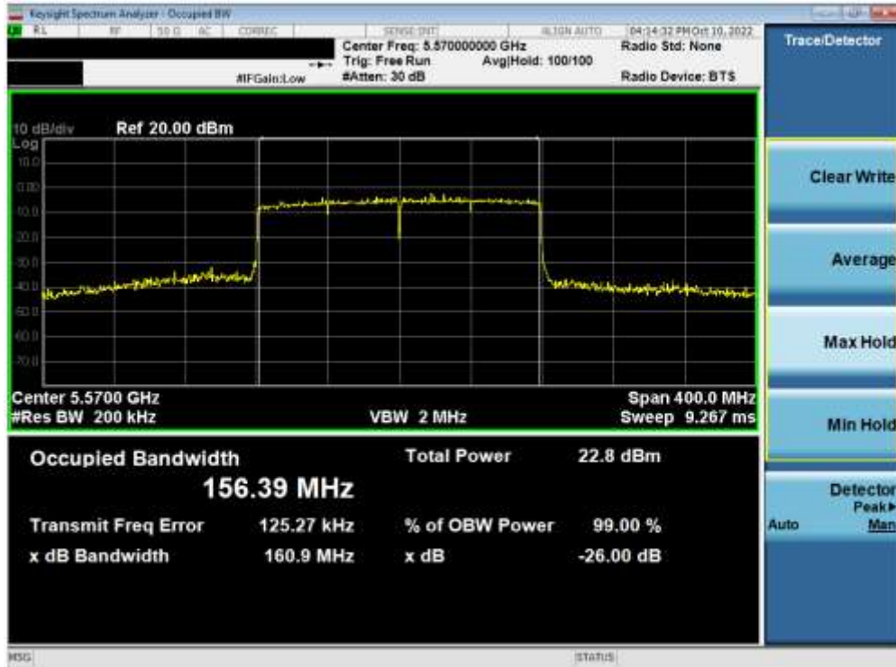
Plot 7-110. 26dB Bandwidth Plot ANT2 (160MHz BW 802.11ax (UNII Band 2C) – Ch. 114)
