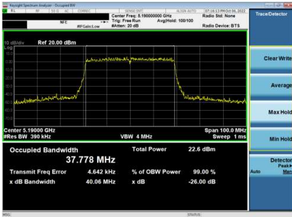
Plot 7-67. 26dB Bandwidth Plot ANT2 (40MHz BW 802.11ax (UNII Band 1) – Ch. 38)
