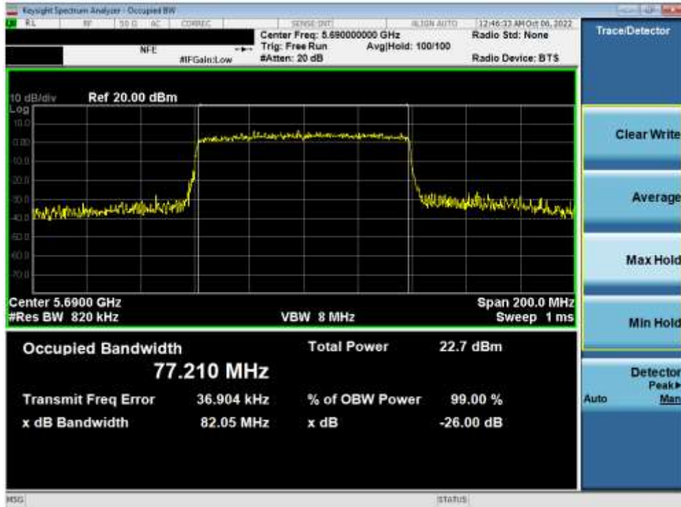
Plot 7-53. 26dB Bandwidth Plot ANT1 (80MHz BW 802.11ax (UNII Band 2C) – Ch. 138)
