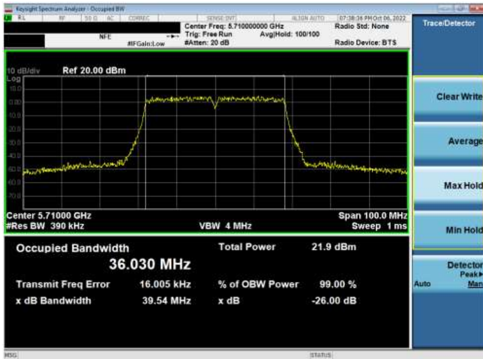
Plot 7-99. 26dB Bandwidth Plot ANT2 (40MHz BW 802.11n (UNII Band 2C) – Ch. 142)
