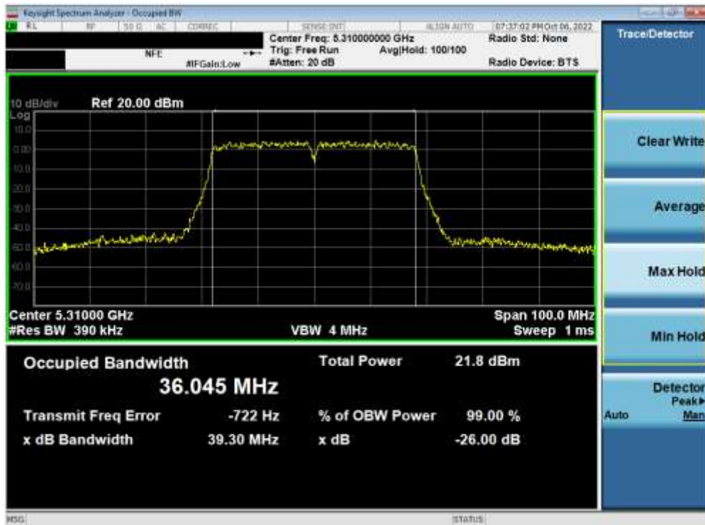
Plot 7-83. 26dB Bandwidth Plot ANT2 (40MHz BW 802.11n (UNII Band 2A) – Ch. 62)
