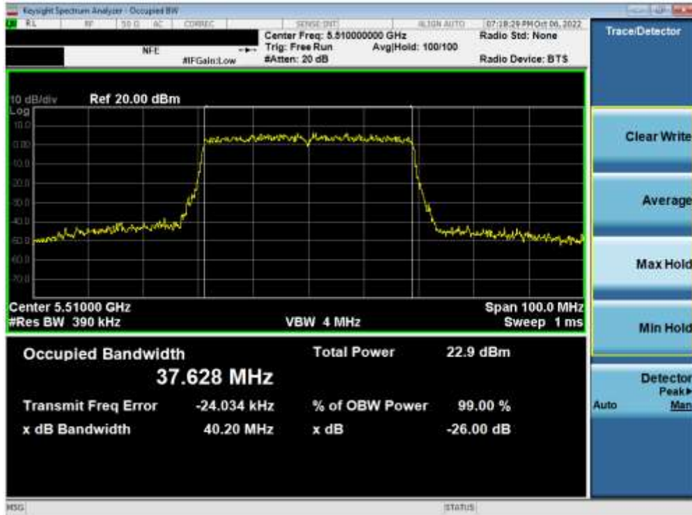
Plot 7-100. 26dB Bandwidth Plot ANT2 (40MHz BW 802.11ax (UNII Band 2C) – Ch. 102)
