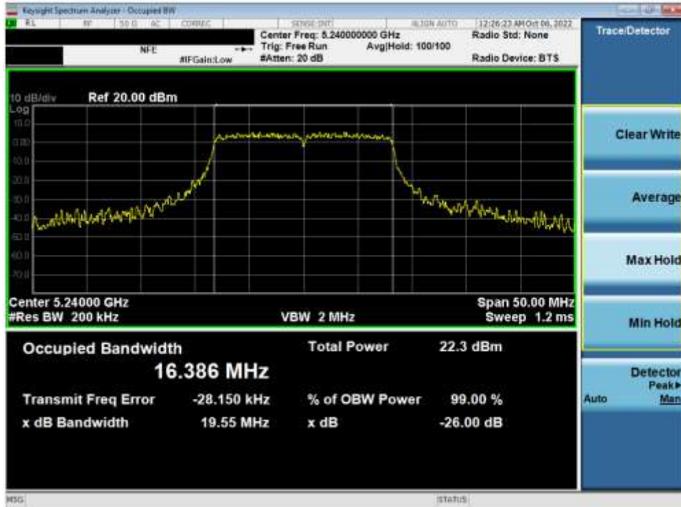
Plot 7-3. 26dB Bandwidth Plot ANT1 (802.11a (UNII Band 1) – Ch. 48)
