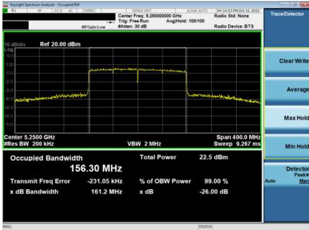
Plot 7-17. 26dB Bandwidth Plot ANT1 (160MHz BW 802.11ax (UNII Band 1) – Ch. 50)
