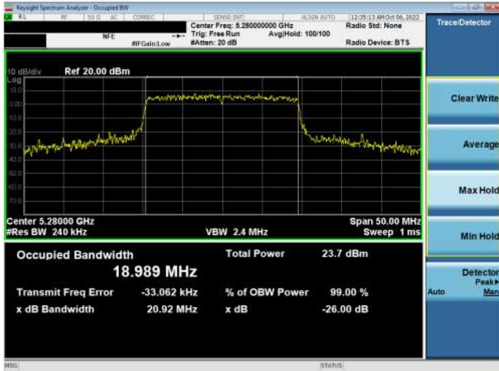
Plot 7-25. 26dB Bandwidth Plot ANT1 (20MHz BW 802.11ax (UNII Band 2A) – Ch. 56)
