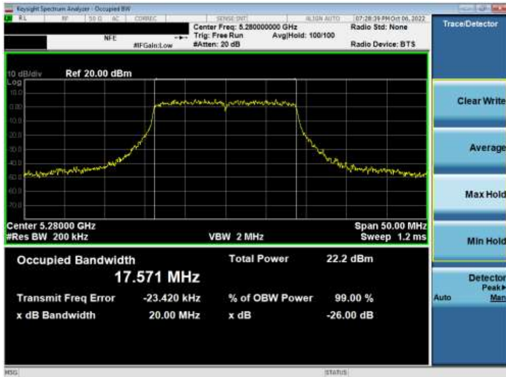
Plot 7-77. 26dB Bandwidth Plot ANT2 (20MHz BW 802.11n (UNII Band 2A) – Ch. 56)
