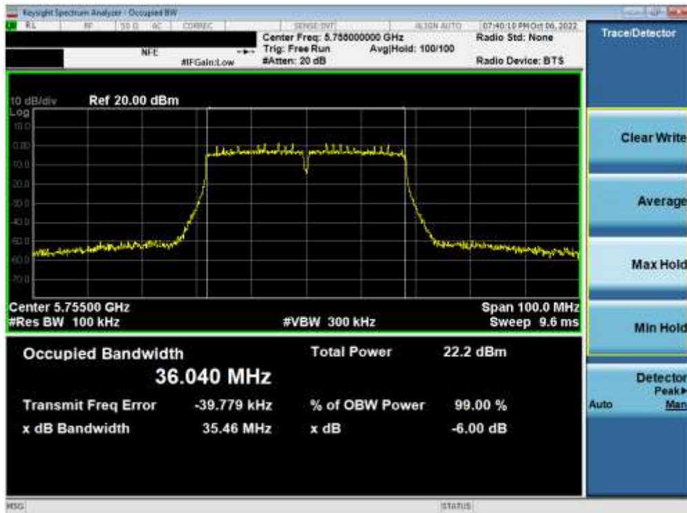
Plot 7-152. 6dB Bandwidth Plot ANT2 (40MHz BW 802.11n (UNII Band 3) – Ch. 151)
