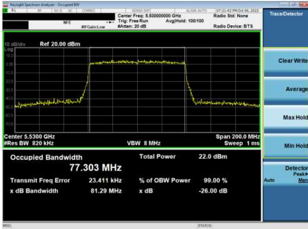
Plot 7-106. 26dB Bandwidth Plot ANT2 (80MHz BW 802.11ax (UNII Band 2C) – Ch. 106)
