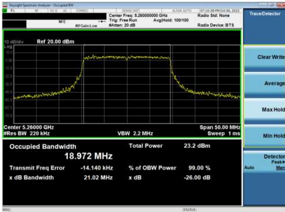
Plot 7-79. 26dB Bandwidth Plot ANT2 (20MHz BW 802.11ax (UNII Band 2A) – Ch. 52)
