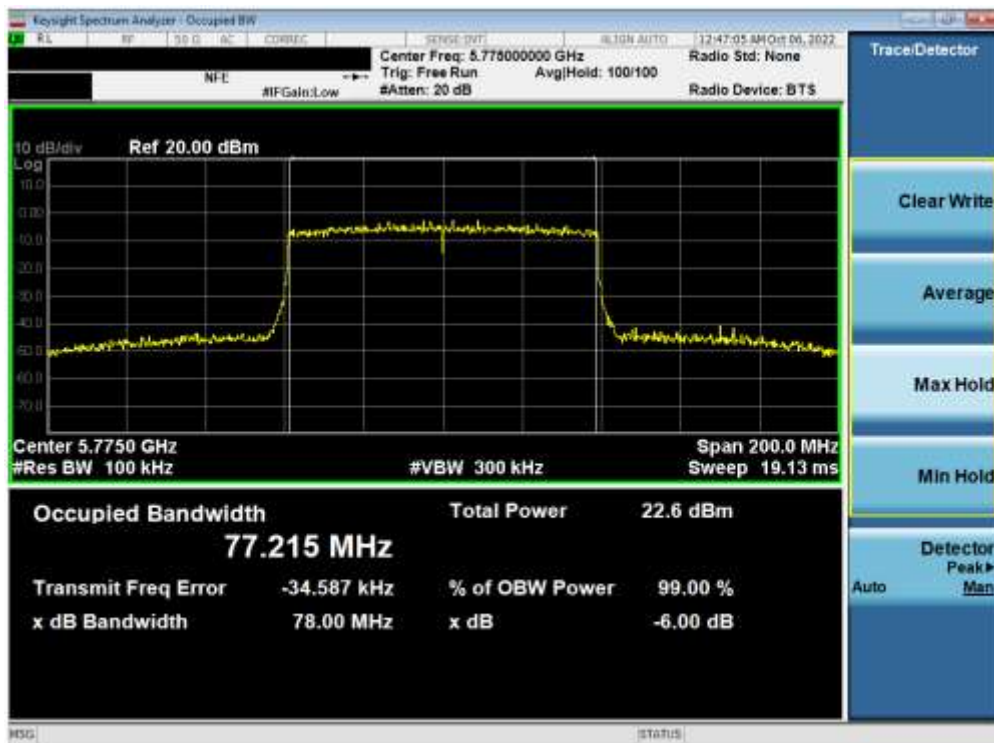
Plot 7-125. 6dB Bandwidth Plot ANT1 (80MHz BW 802.11ax (UNII Band 3) – Ch. 155)
