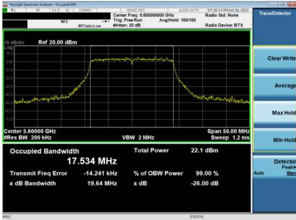
Plot 7-92. 26dB Bandwidth Plot ANT2 (20MHz BW 802.11n (UNII Band 2C) – Ch. 120)
