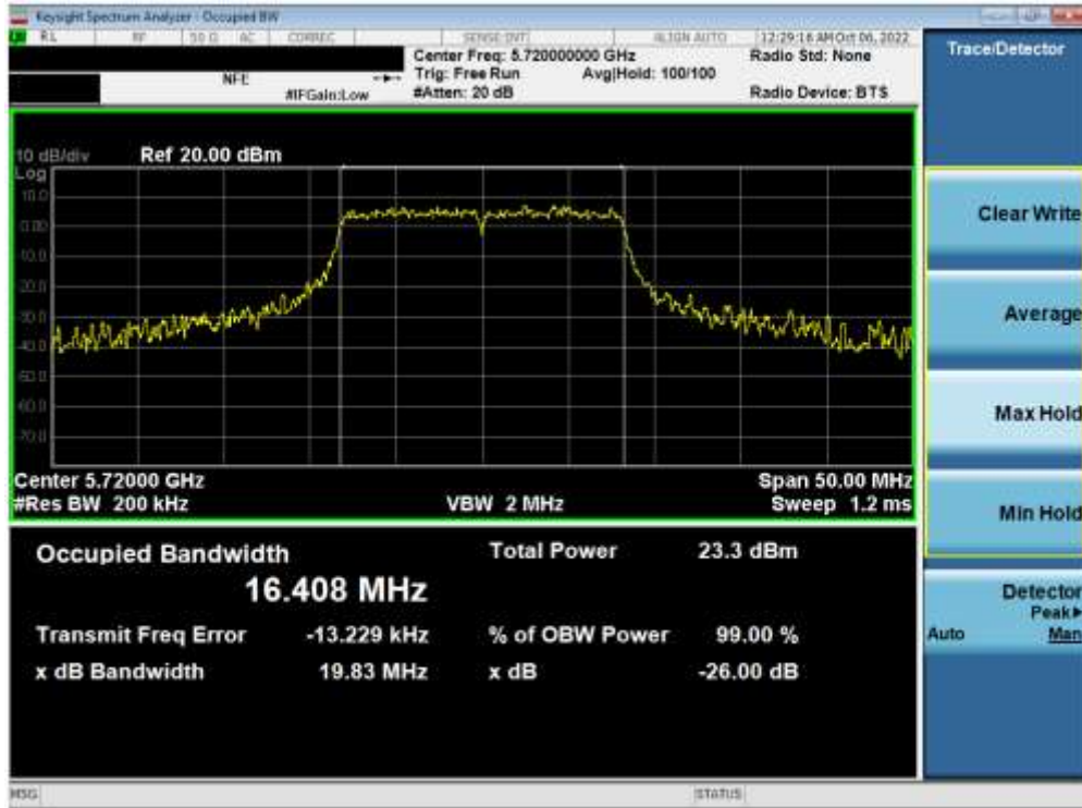
Plot 7-35. 26dB Bandwidth Plot ANT1 (802.11a (UNII Band 2C) – Ch. 144)
