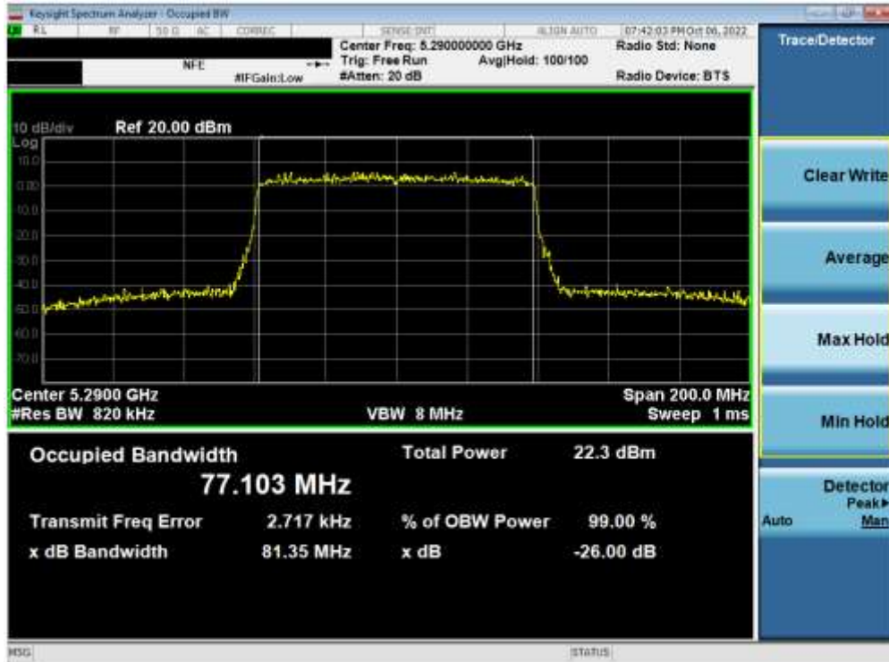
Plot 7-86. 26dB Bandwidth Plot ANT2 (80MHz BW 802.11ac (UNII Band 2A) – Ch. 58)
