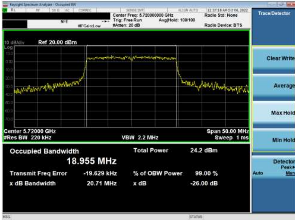
Plot 7-41. 26dB Bandwidth Plot ANT1 (20MHz BW 802.11ax (UNII Band 2C) – Ch. 144)
