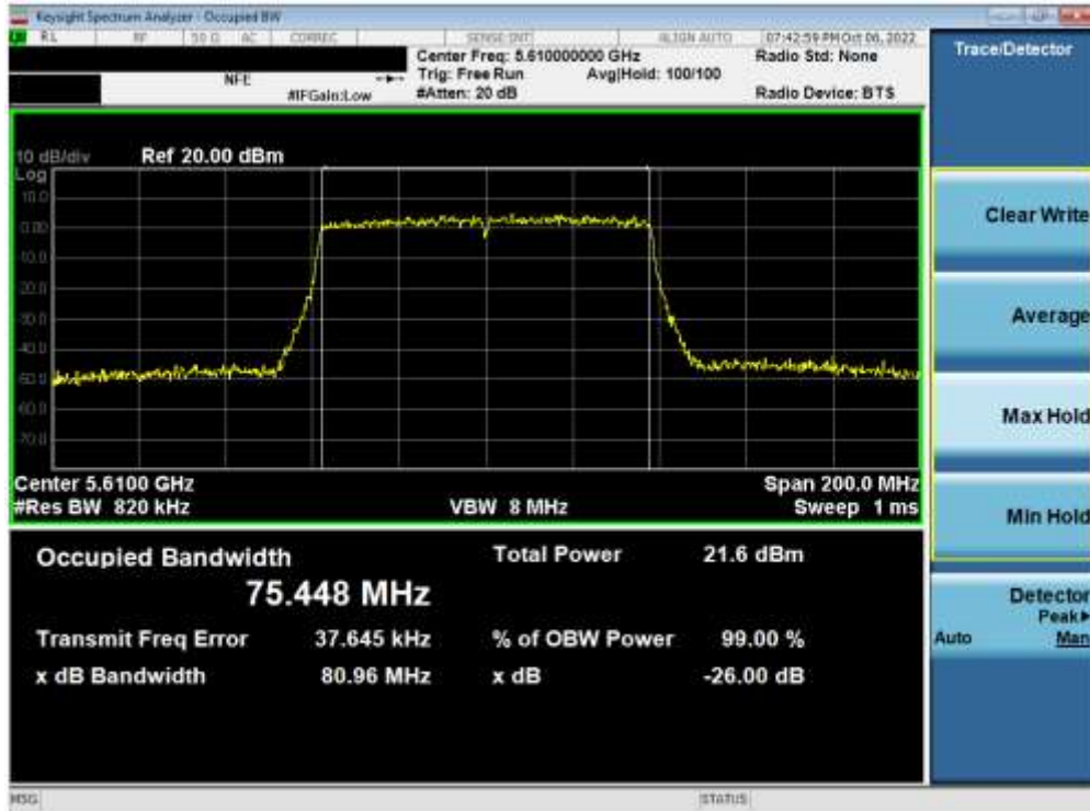
Plot 7-104. 26dB Bandwidth Plot ANT2 (80MHz BW 802.11ac (UNII Band 2C) – Ch. 122)
