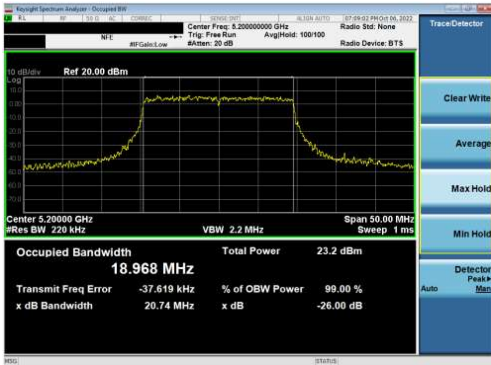
Plot 7-63. 26dB Bandwidth Plot ANT2 (20MHz BW 802.11ax (UNII Band 1) – Ch. 40)
