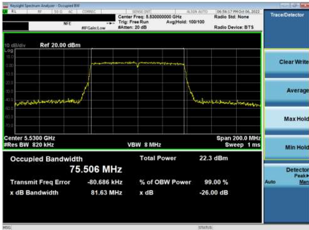
Plot 7-48. 26dB Bandwidth Plot ANT1 (80MHz BW 802.11ac (UNII Band 2C) – Ch. 106)
