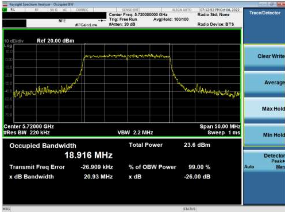
Plot 7-96. 26dB Bandwidth Plot ANT2 (20MHz BW 802.11ax (UNII Band 2C) – Ch. 144)
