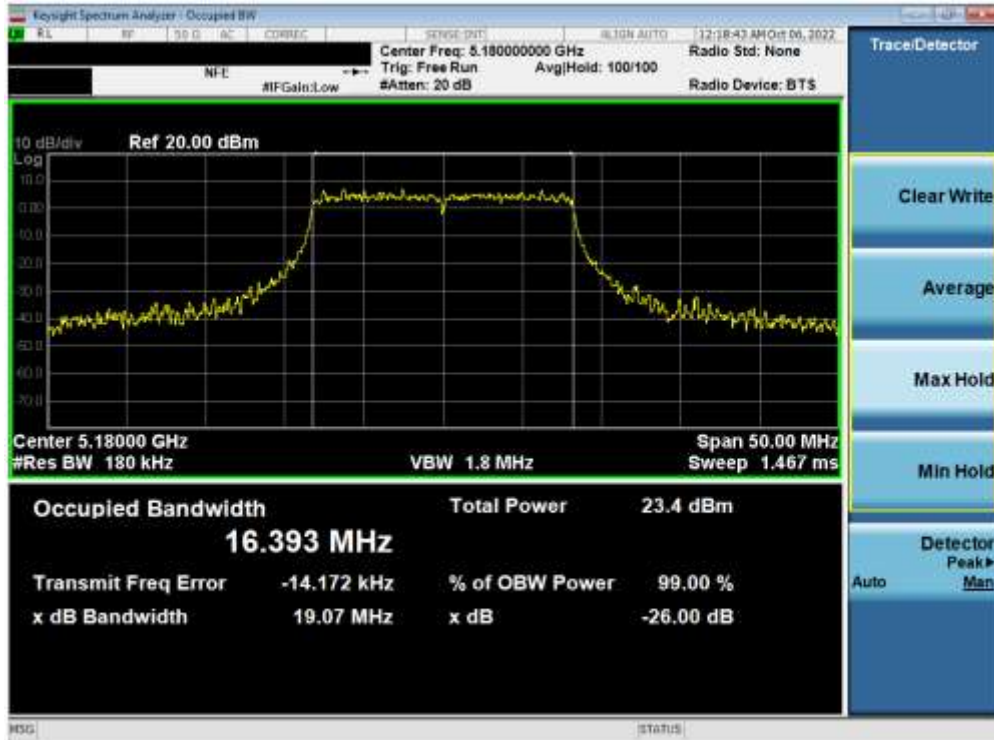
Plot 7-56. 26dB Bandwidth Plot ANT2 (802.11a (UNII Band 1) – Ch. 36)
