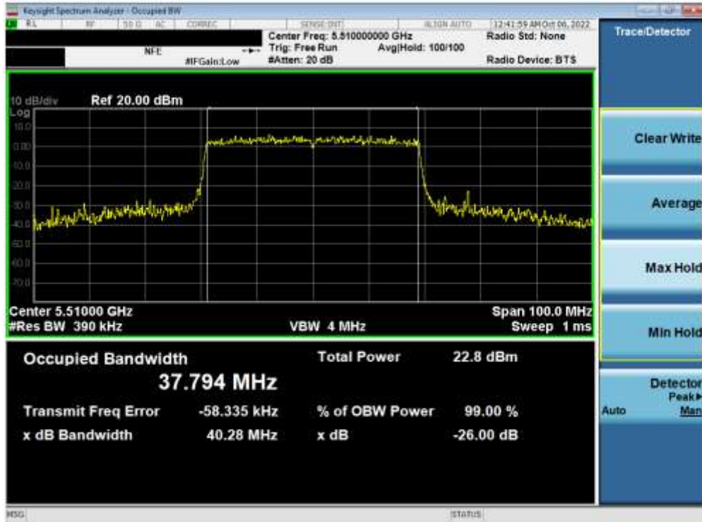
Plot 7-45. 26dB Bandwidth Plot ANT1 (40MHz BW 802.11ax (UNII Band 2C) – Ch. 102)
