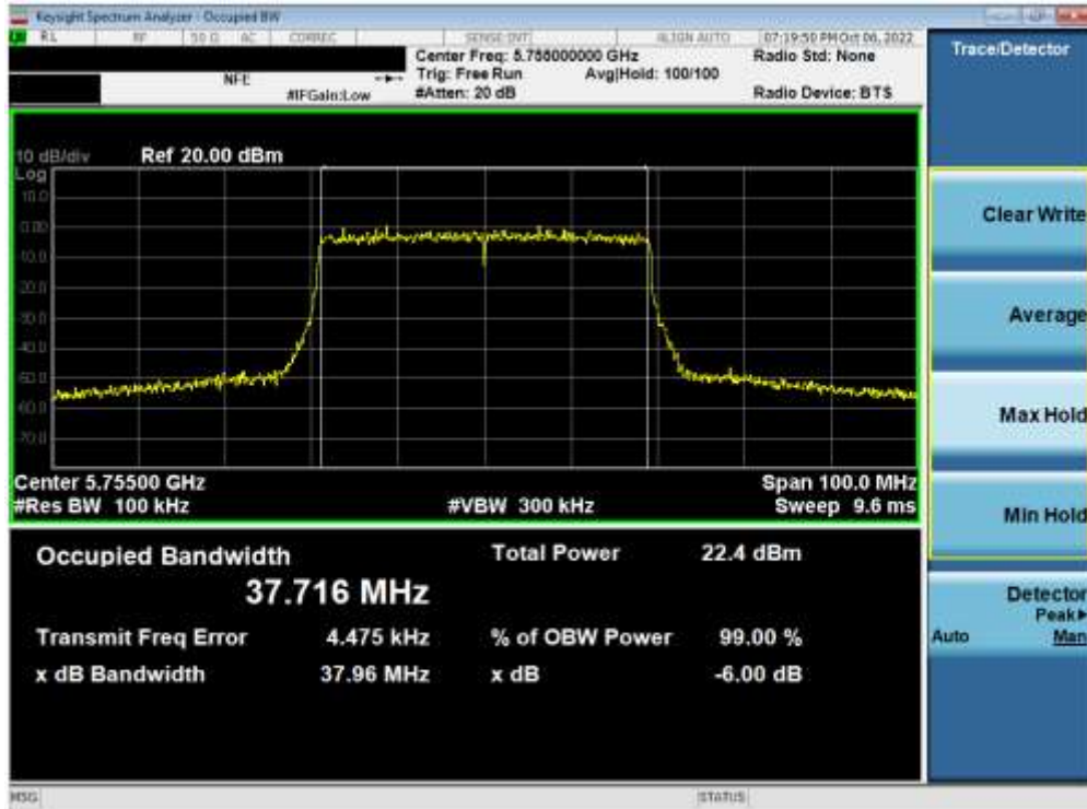
Plot 7-154. 6dB Bandwidth Plot ANT2 (40MHz BW 802.11ax (UNII Band 3) – Ch. 151)
