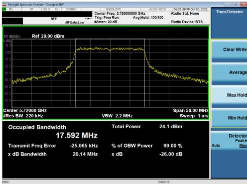
Plot 7-38. 26dB Bandwidth Plot ANT1 (20MHz BW 802.11n (UNII Band 2C) – Ch. 144)
