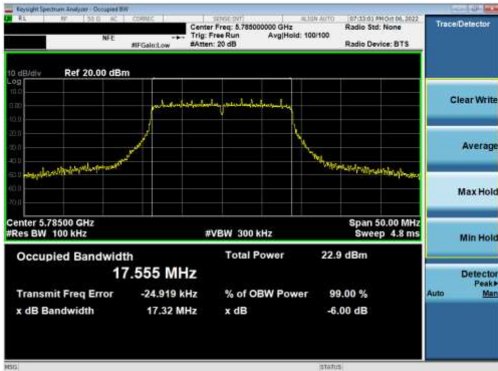
Plot 7-147. 6dB Bandwidth Plot ANT2 (20MHz BW 802.11n (UNII Band 3) – Ch. 157)
