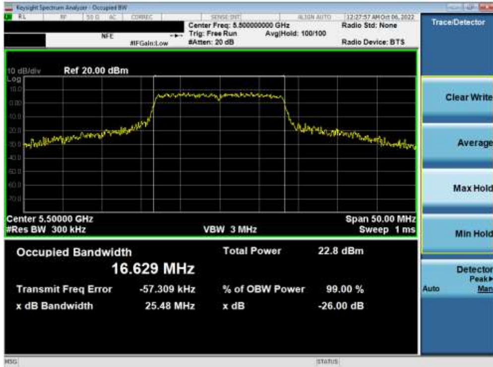
Plot 7-33. 26dB Bandwidth Plot ANT1 (802.11a (UNII Band 2C) – Ch. 100)
