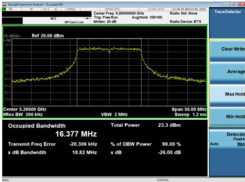
Plot 7-73. 26dB Bandwidth Plot ANT2 (802.11a (UNII Band 2A) – Ch. 52)
