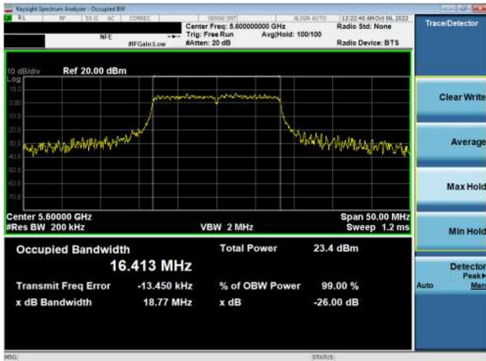
Plot 7-89. 26dB Bandwidth Plot ANT2 (802.11a (UNII Band 2C) – Ch. 120)
