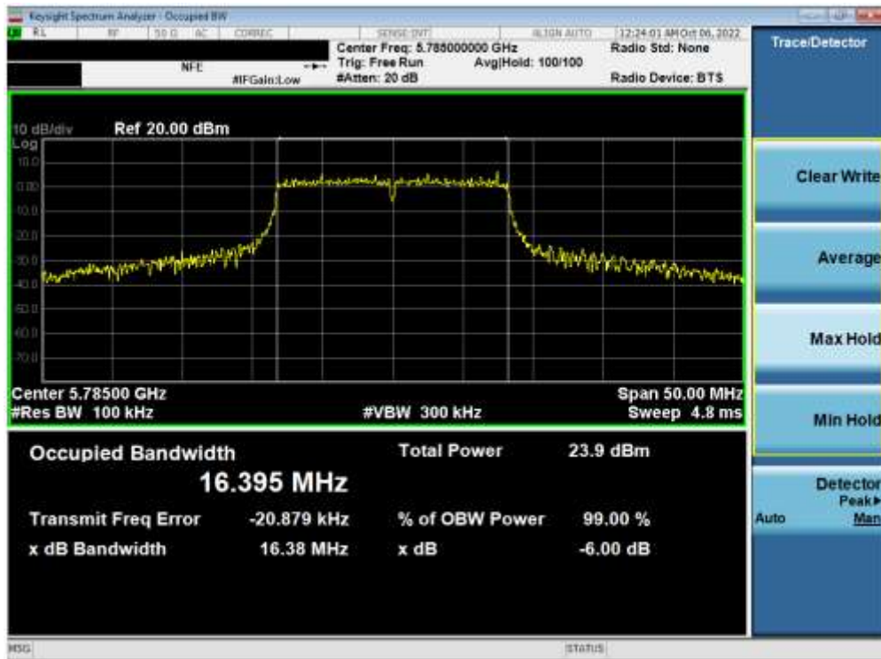
Plot 7-144. 6dB Bandwidth Plot ANT2 (802.11a (UNII Band 3) – Ch. 157)
