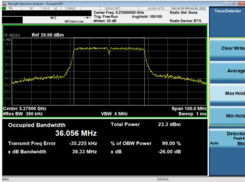
Plot 7-27. 26dB Bandwidth Plot ANT1 (40MHz BW 802.11n (UNII Band 2A) – Ch. 54)
