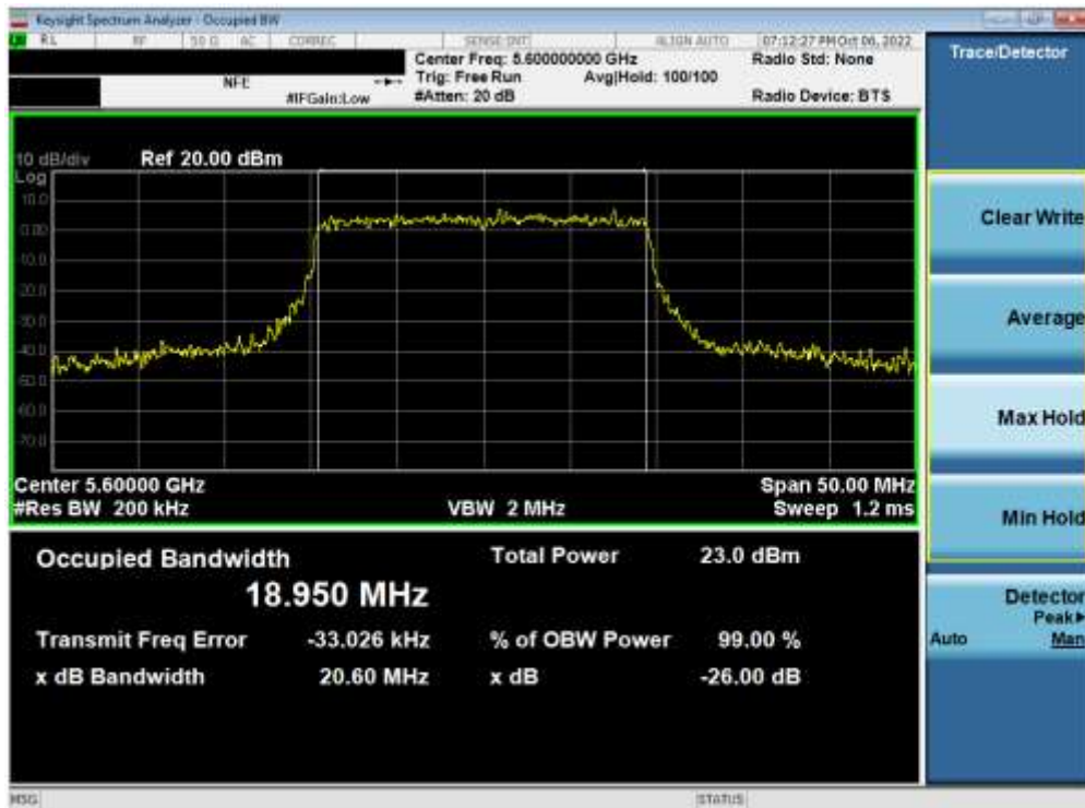
Plot 7-95. 26dB Bandwidth Plot ANT2 (20MHz BW 802.11ax (UNII Band 2C) – Ch. 120)
