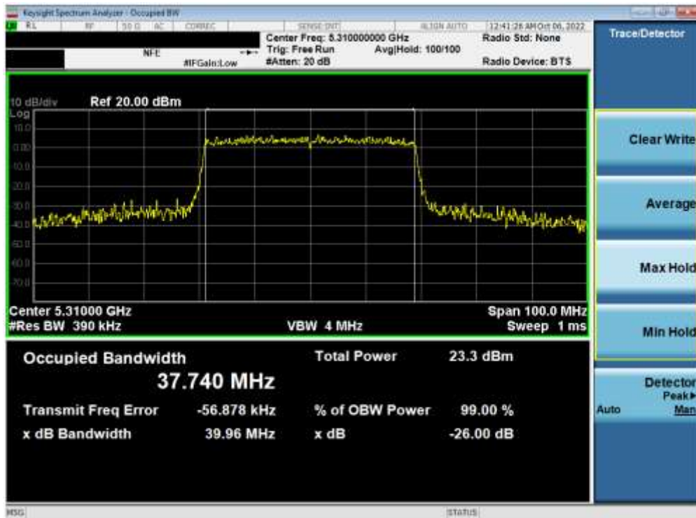
Plot 7-30. 26dB Bandwidth Plot ANT1 (40MHz BW 802.11ax (UNII Band 2A) – Ch. 62)
