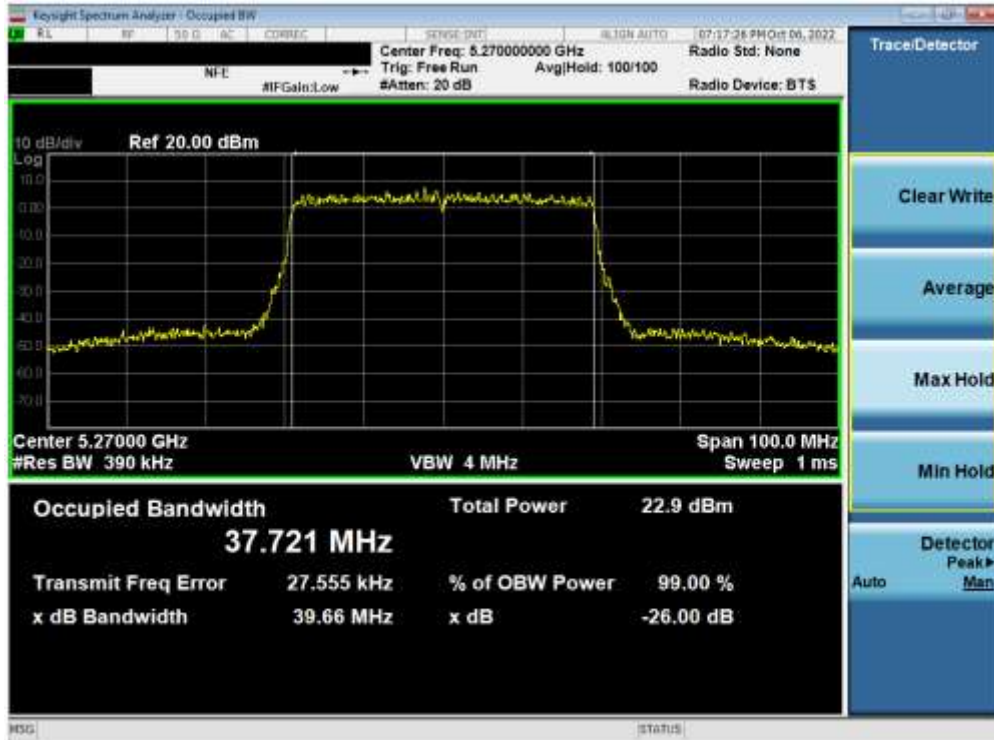
Plot 7-84. 26dB Bandwidth Plot ANT2 (40MHz BW 802.11ax (UNII Band 2A) – Ch. 54)
