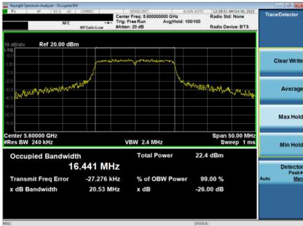
Plot 7-34. 26dB Bandwidth Plot ANT1 (802.11a (UNII Band 2C) – Ch. 120)
