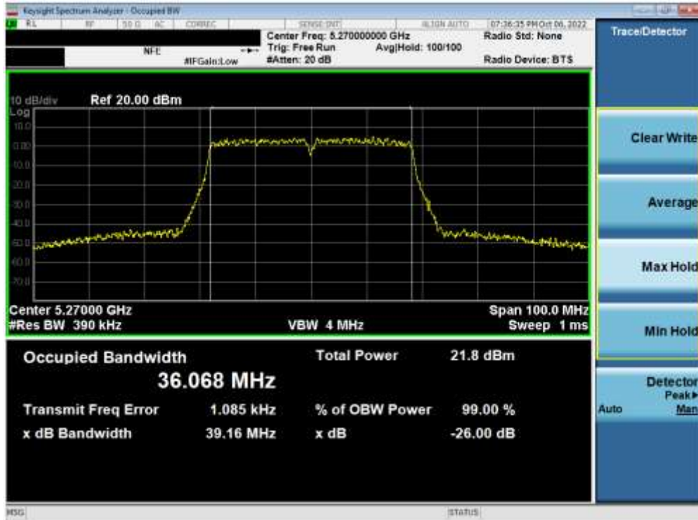
Plot 7-82. 26dB Bandwidth Plot ANT2 (40MHz BW 802.11n (UNII Band 2A) – Ch. 54)
