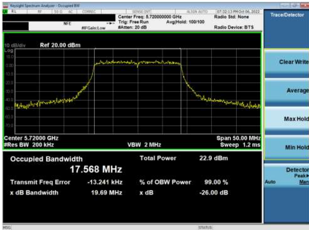
Plot 7-93. 26dB Bandwidth Plot ANT2 (20MHz BW 802.11n (UNII Band 2C) – Ch. 144)
