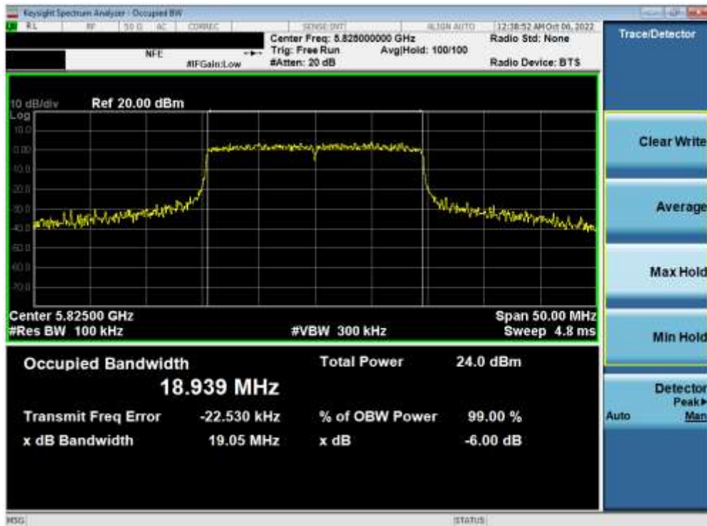
Plot 7-119. 6dB Bandwidth Plot ANT1 (20MHz BW 802.11ax (UNII Band 3) – Ch. 165)
