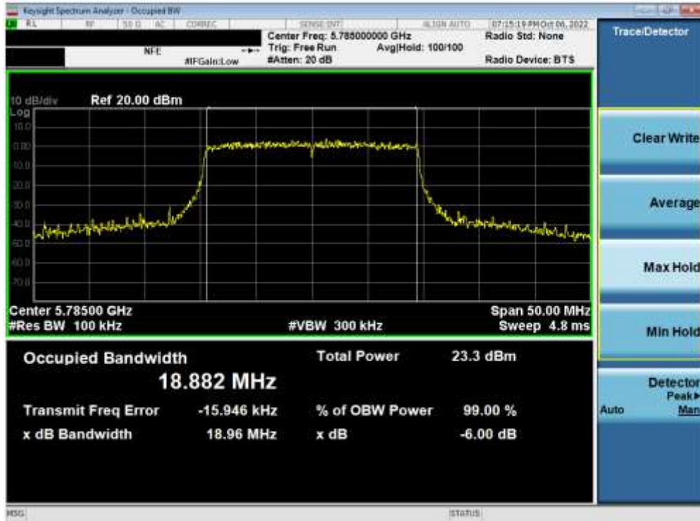
Plot 7-150. 6dB Bandwidth Plot ANT2 (20MHz BW 802.11ax (UNII Band 3) – Ch. 157)
