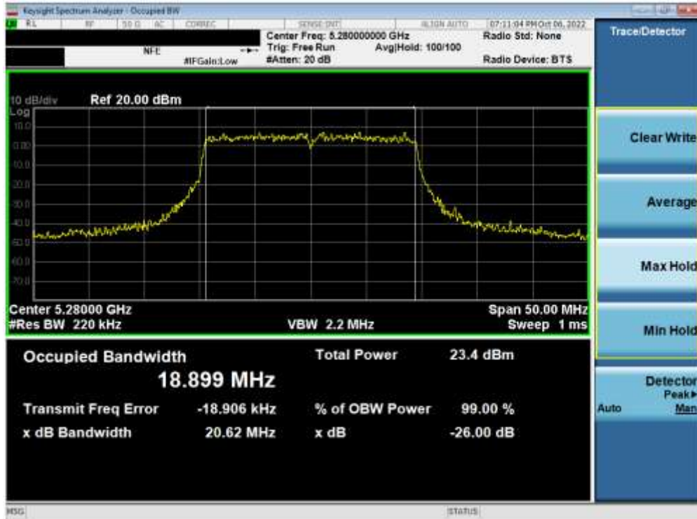
Plot 7-80. 26dB Bandwidth Plot ANT2 (20MHz BW 802.11ax (UNII Band 2A) – Ch. 56)
