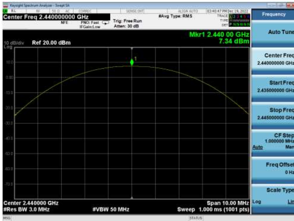
Plot 7-26. Peak Power Plot (Bluetooth (LE), 1Mbps – Ch. 19) – ANT 1
