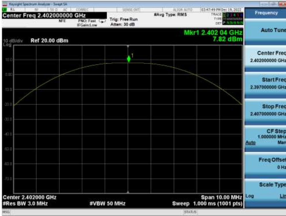
Plot 7-34. Peak Power Plot (Bluetooth (LE), 2Mbps – Ch. 0) – ANT 2
