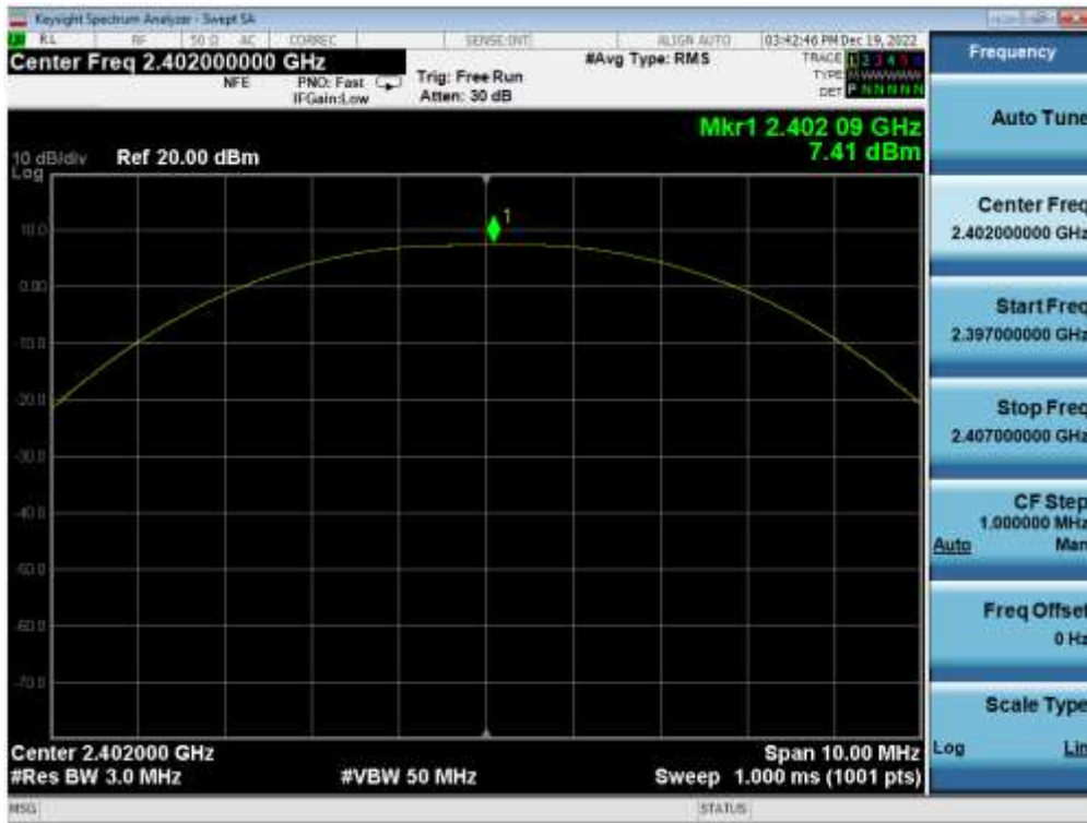
Plot 7-28. Peak Power Plot (Bluetooth (LE), 2Mbps – Ch. 0) – ANT 1
