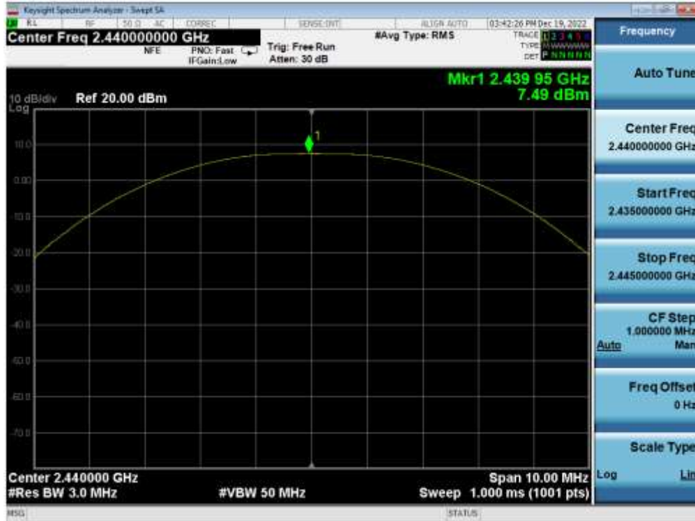
Plot 7-29. Peak Power Plot (Bluetooth (LE), 2Mbps – Ch. 19) – ANT 1
