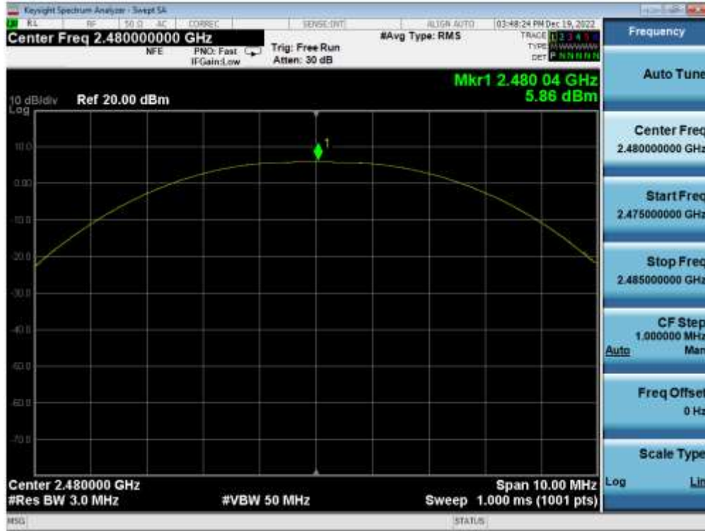
Plot 7-36. Peak Power Plot (Bluetooth (LE), 2Mbps – Ch. 39) – ANT 2
