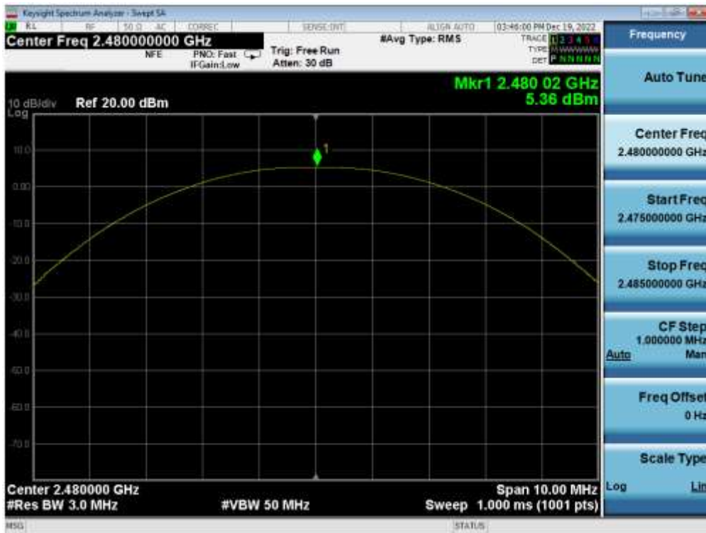
Plot 7-33. Peak Power Plot (Bluetooth (LE), 1Mbps – Ch. 39) – ANT 2
