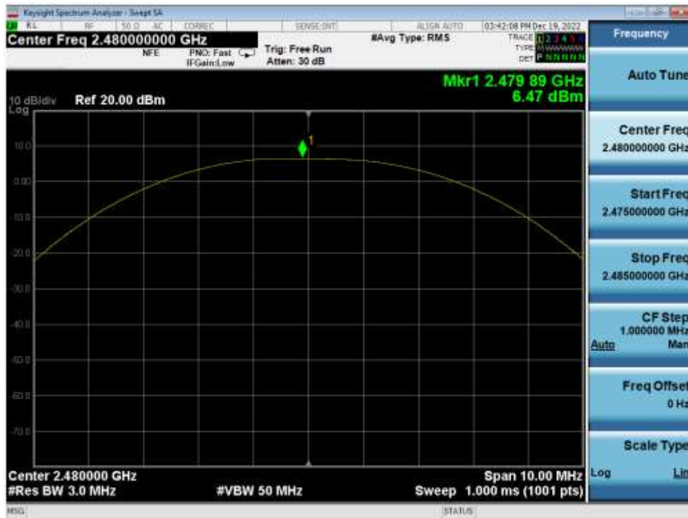
Plot 7-30. Peak Power Plot (Bluetooth (LE), 2Mbps – Ch. 39) – ANT 1
