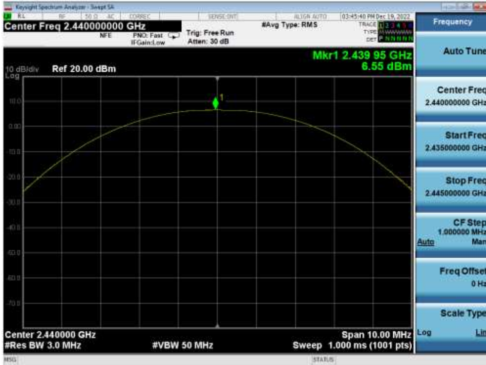
Plot 7-32. Peak Power Plot (Bluetooth (LE), 1Mbps – Ch. 19) – ANT 2
