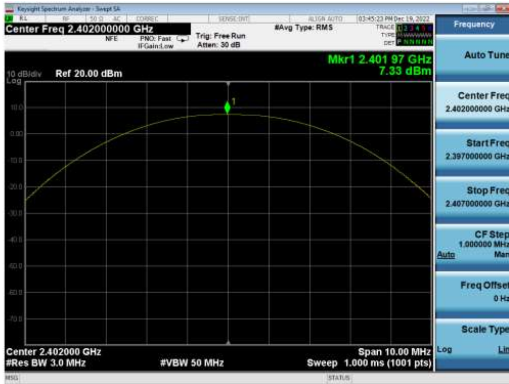
Plot 7-31. Peak Power Plot (Bluetooth (LE), 1Mbps – Ch. 0) – ANT 2
