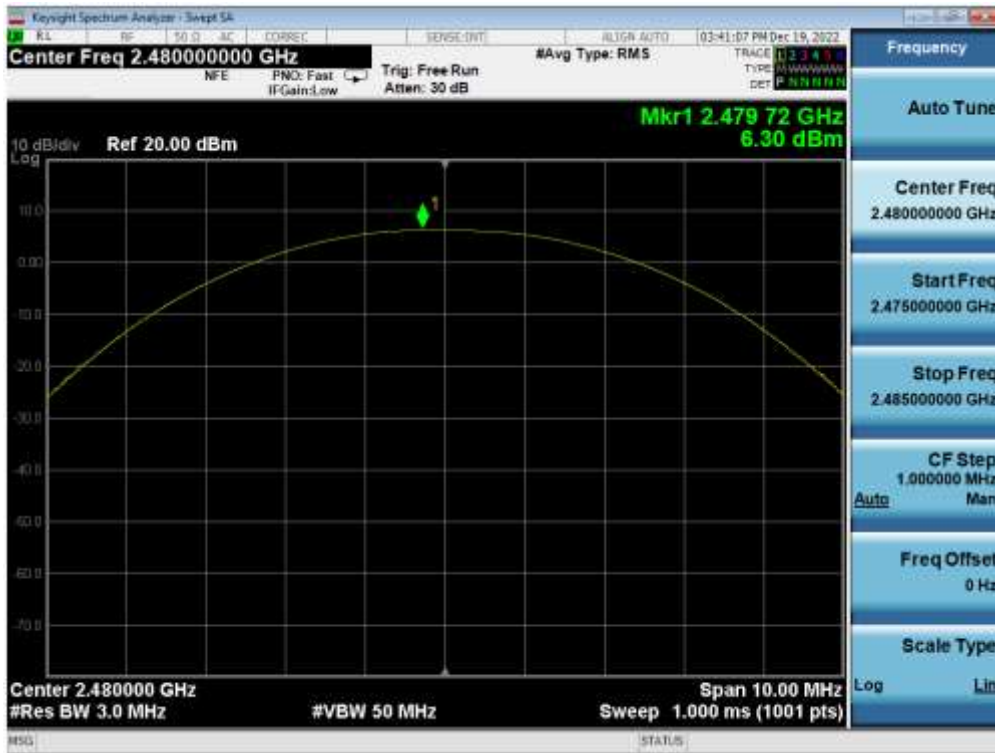
Plot 7-27. Peak Power Plot (Bluetooth (LE), 1Mbps – Ch. 39) – ANT 1
