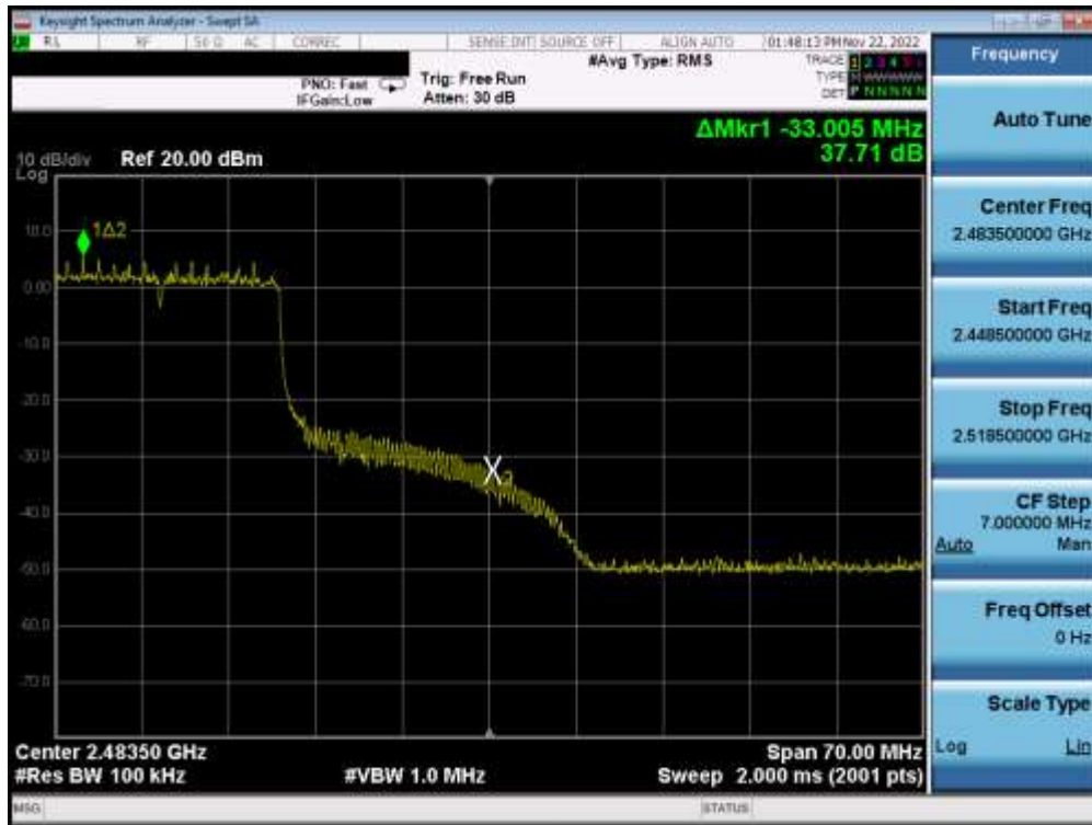
Plot 7-44. Band Edge Plot SISO ANT2 (802.11ax OFDMA – 242 Tones – Ch. 10)
