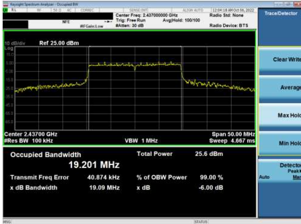
Plot 7-5. 6dB Bandwidth Plot SISO ANT2 (802.11ax OFDMA – 242 Tones – Ch. 6)
