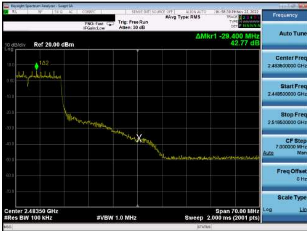
Plot 7-54. Band Edge Plot MIMO ANT1 (802.11ax OFDMA – 242 Tones – Ch. 9)
