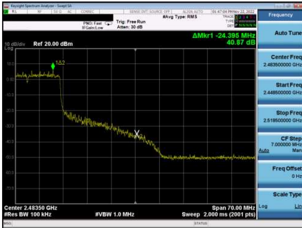
Plot 7-43. Band Edge Plot SISO ANT2 (802.11ax OFDMA – 242 Tones – Ch. 9)
