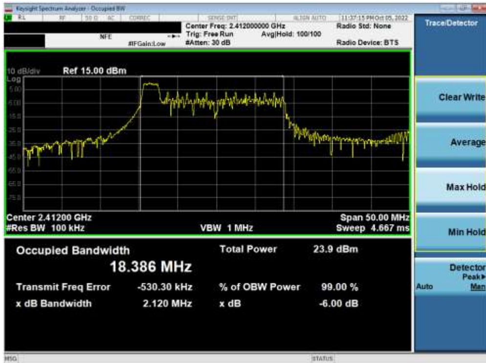
Plot 7-7. 6dB Bandwidth Plot MIMO ANT1 (802.11ax OFDMA – 26 Tones – Ch. 1)
