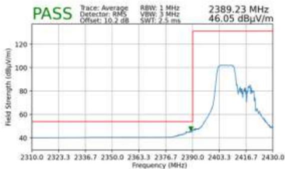
Plot 7-144. Radiated Restricted Lower Band Edge Measurement MIMO (Average – 106 Tones)
