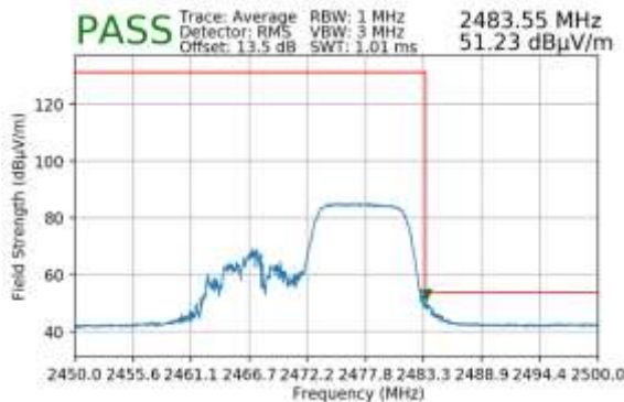
Plot 7-150. Radiated Restricted Upper Band Edge Measurement MIMO (Average – 106 Tones)
