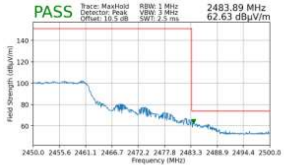
Plot 7-157. Radiated Restricted Upper Band Edge Measurement MIMO (Peak – 242 Tones)
