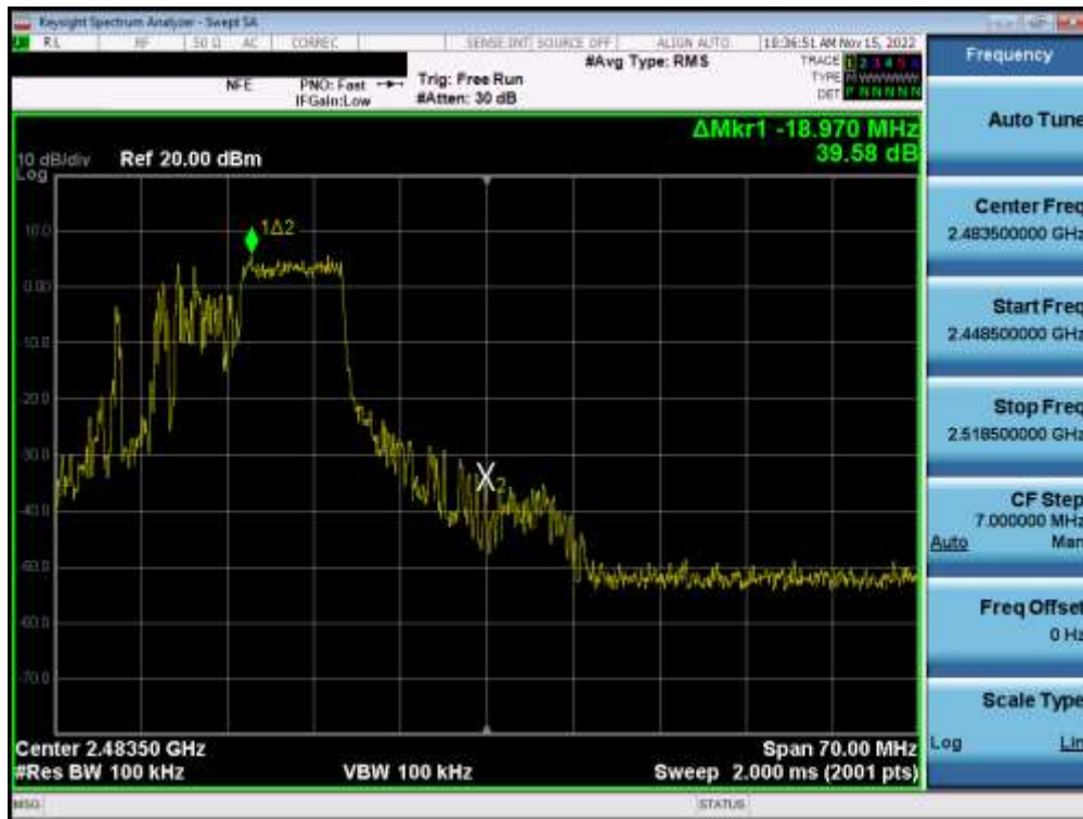
Plot 7-49. Band Edge Plot MIMO ANT1 (802.11ax OFDMA – 106 Tones – Ch. 11)
