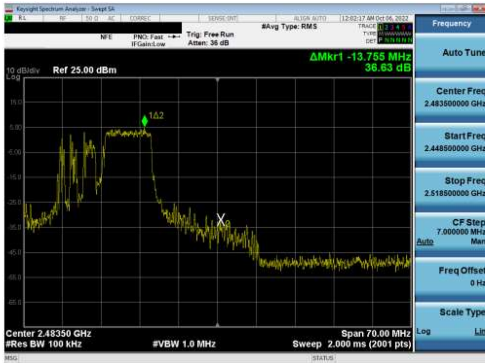
Plot 7-38. Band Edge Plot SISO ANT2 (802.11ax OFDMA – 106 Tones – Ch. 11)
