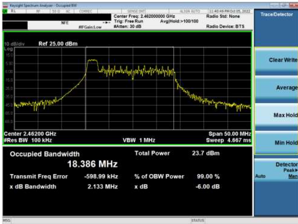
Plot 7-9. 6dB Bandwidth Plot MIMO ANT1 (802.11ax OFDMA – 26 Tones – Ch. 11)
