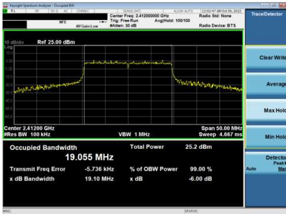
Plot 7-4. 6dB Bandwidth Plot SISO ANT2 (802.11ax OFDMA – 242 Tones – Ch. 1)
