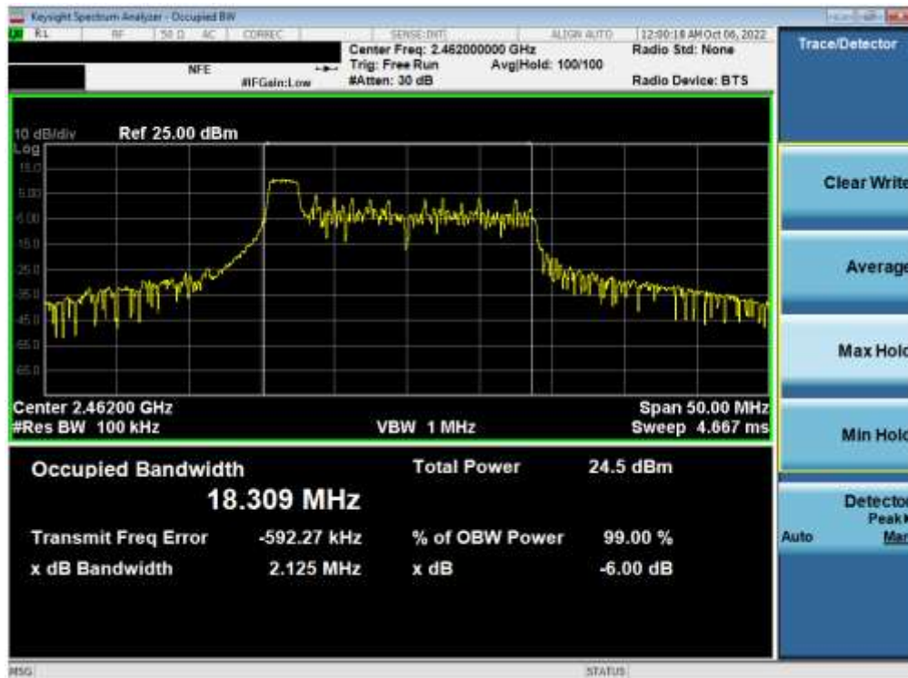
Plot 7-3. 6dB Bandwidth Plot SISO ANT2 (802.11ax OFDMA – 26 Tones – Ch. 11)
