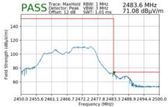
Plot 7-149. Radiated Restricted Upper Band Edge Measurement MIMO (Peak – 106 Tones)
