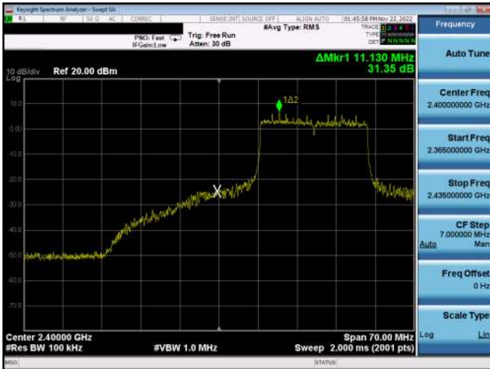
Plot 7-42. Band Edge Plot SISO ANT2 (802.11ax OFDMA – 242 Tones – Ch. 2)
