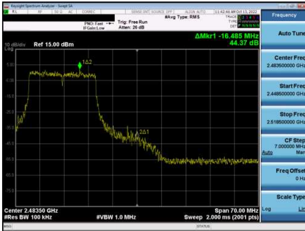
Plot 7-45. Band Edge Plot SISO ANT2 (802.11ax OFDMA – 242 Tones – Ch. 11)
