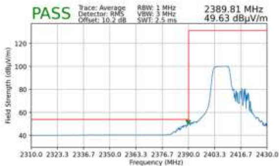
Plot 7-122. Radiated Restricted Lower Band Edge Measurement SISO ANT2 (Average – 106 Tones)
