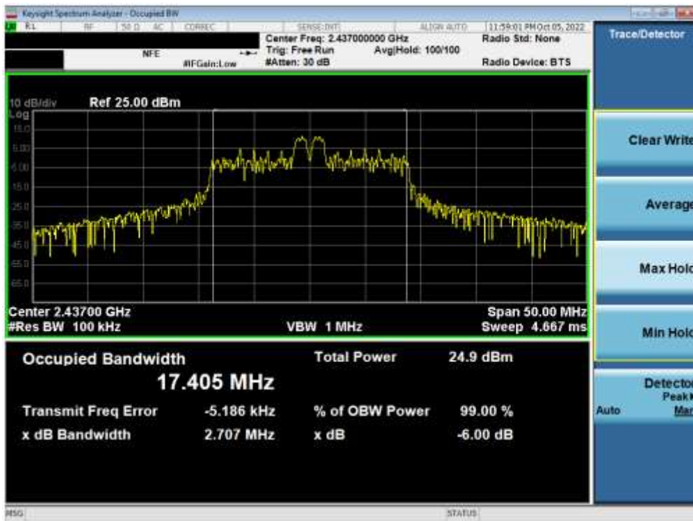
Plot 7-2. 6dB Bandwidth Plot SISO ANT2 (802.11ax OFDMA – 26 Tones – Ch. 6)
