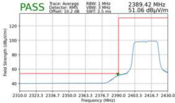
Plot 7-130. Radiated Restricted Lower Band Edge Measurement SISO ANT2 (Average – 242 Tones)
