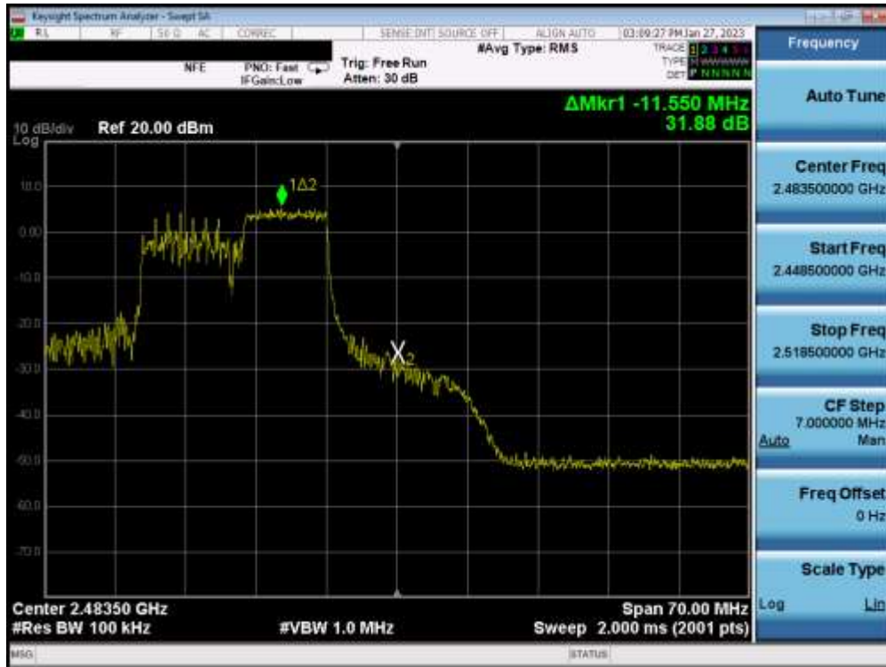
Plot 7-61. Band Edge Plot MIMO ANT2 (802.11ax OFDMA – 106 Tones – Ch. 12)
