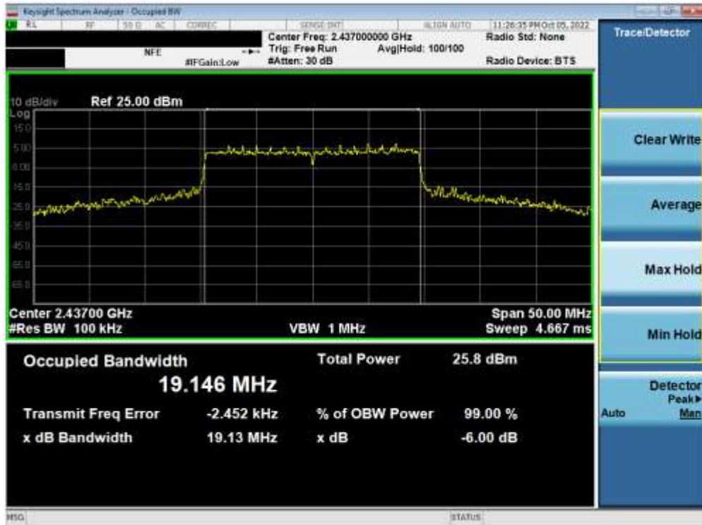
Plot 7-17. 6dB Bandwidth Plot MIMO ANT2 (802.11ax OFDMA – 242 Tones – Ch. 6)
