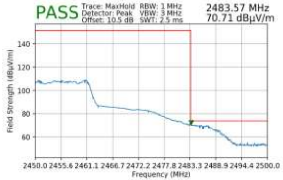
Plot 7-135. Radiated Restricted Upper Band Edge Measurement SISO ANT2 (Peak – 242 Tones)
