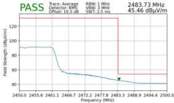
Plot 7-156. Radiated Restricted Upper Band Edge Measurement MIMO (Average – 242 Tones)
