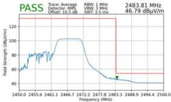
Plot 7-146. Radiated Restricted Upper Band Edge Measurement MIMO (Average – 106 Tones)
