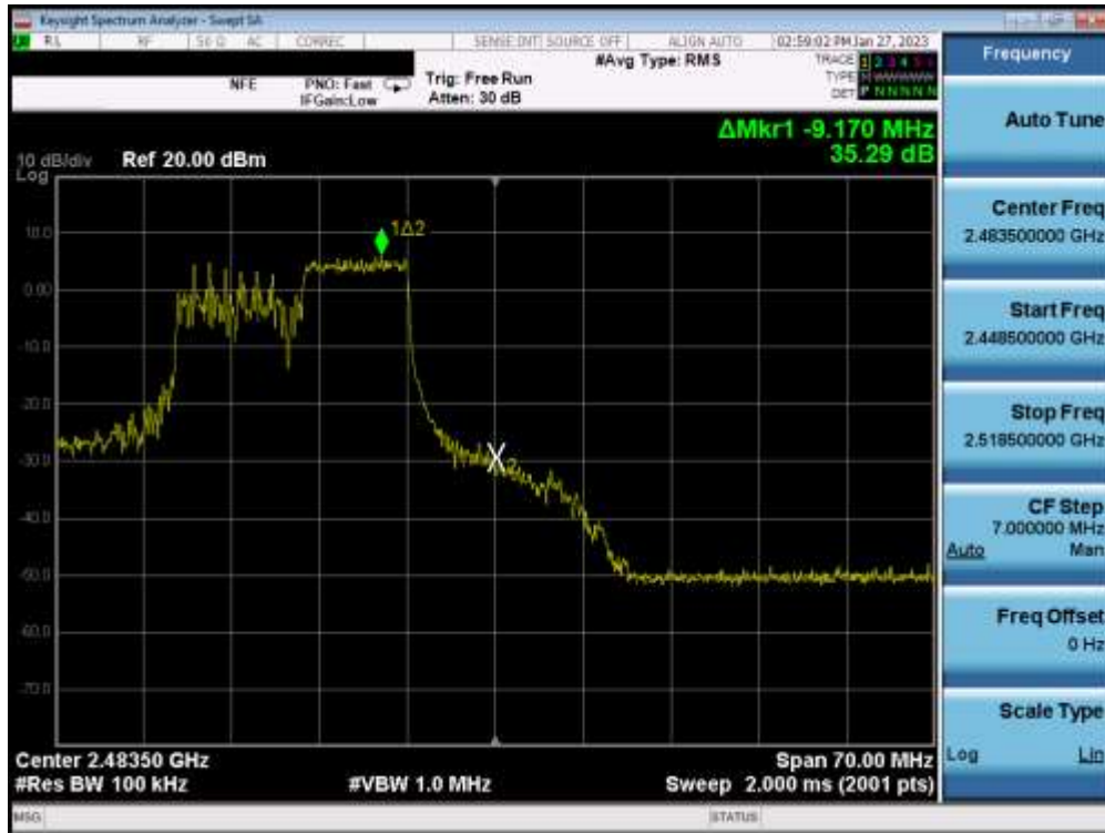
Plot 7-39. Band Edge Plot SISO ANT2 (802.11ax OFDMA – 106 Tones – Ch. 12)
