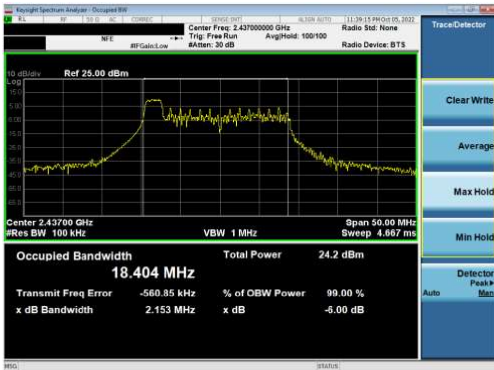
Plot 7-8. 6dB Bandwidth Plot MIMO ANT1 (802.11ax OFDMA – 26 Tones – Ch. 6)
