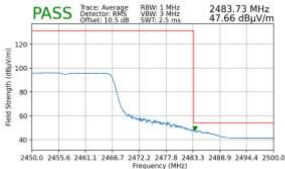
Plot 7-158. Radiated Restricted Upper Band Edge Measurement MIMO (Average – 242 Tones)
