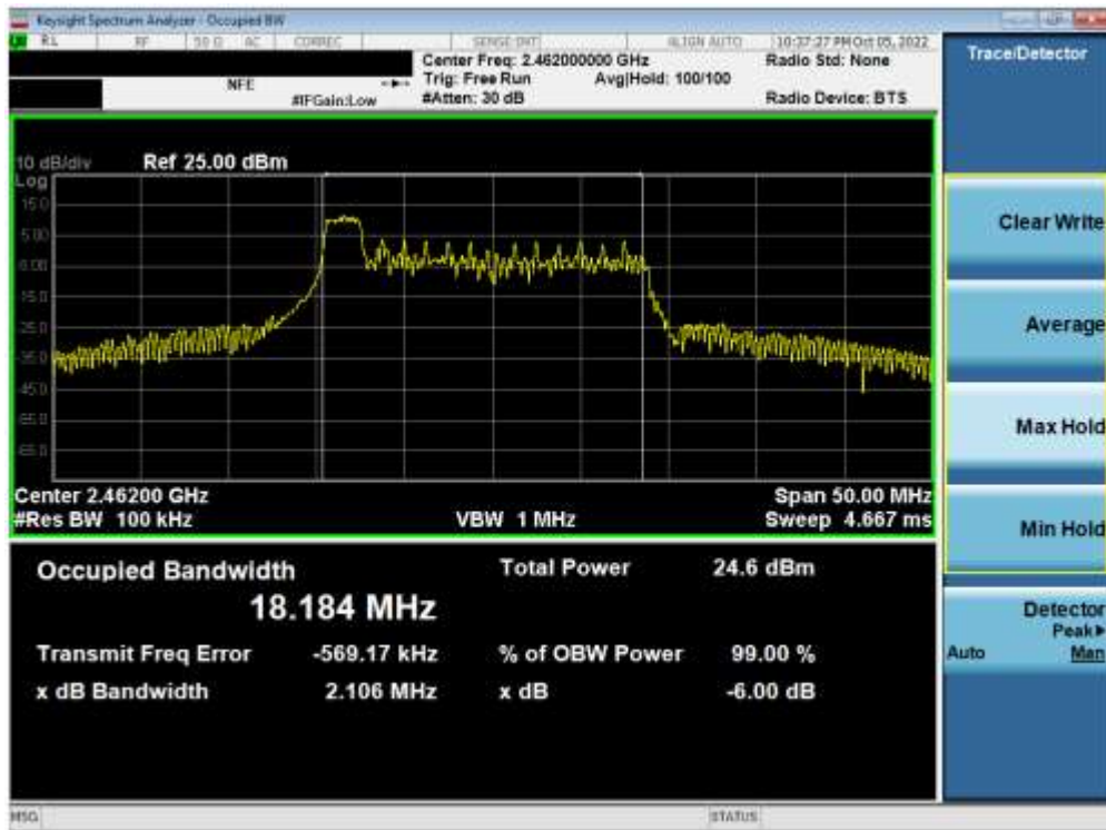
Plot 7-15. 6dB Bandwidth Plot MIMO ANT2 (802.11ax OFDMA – 26 Tones – Ch. 11)
