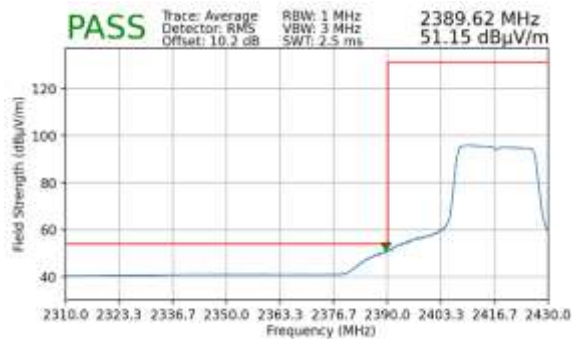
Plot 7-154. Radiated Restricted Lower Band Edge Measurement MIMO (Average – 242 Tones)
