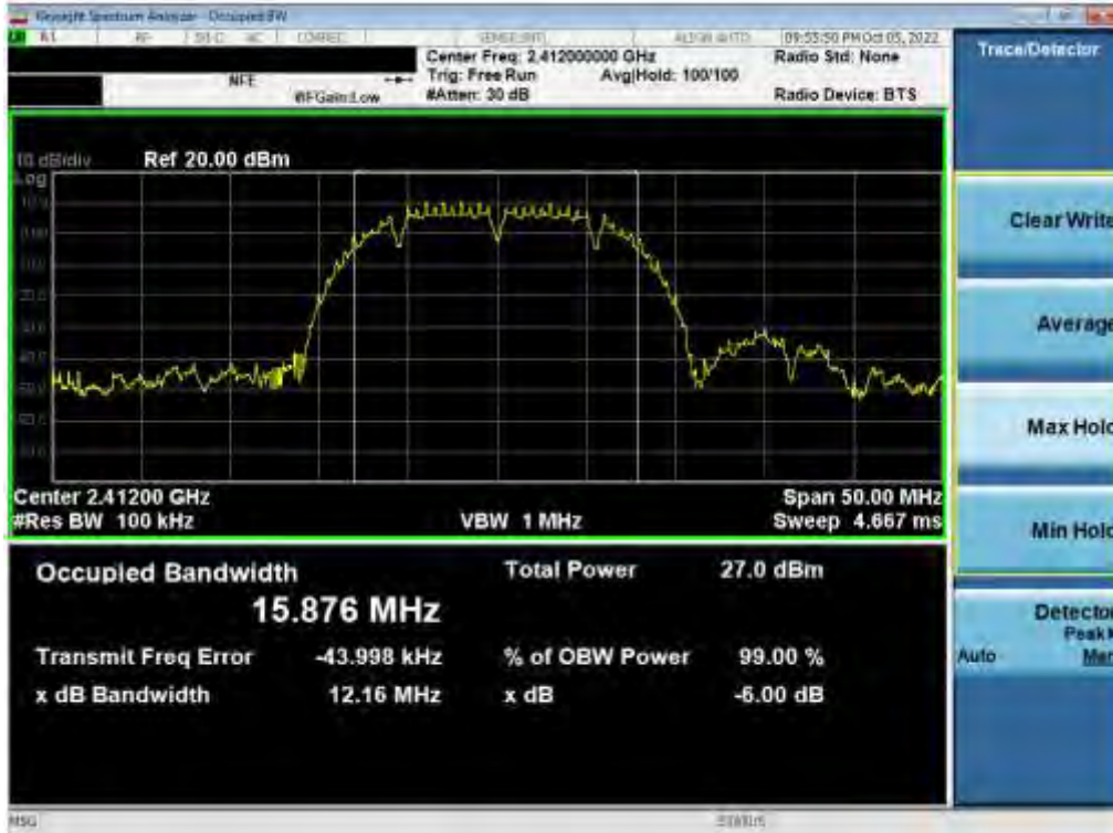
Plot 7-25. 6dB Bandwidth Plot (802.11b – Ch. 1) MIMO ANT 2
