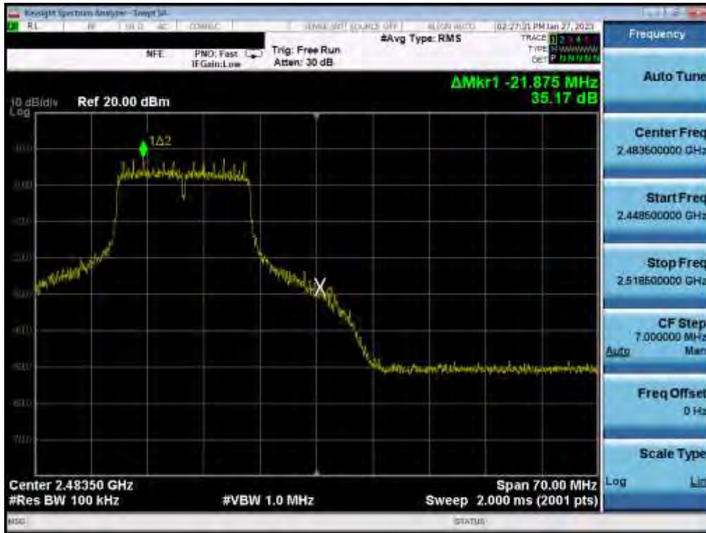
Plot 7-121. Band Edge Plot (802.11g – Ch. 12) MIMO ANT 2
