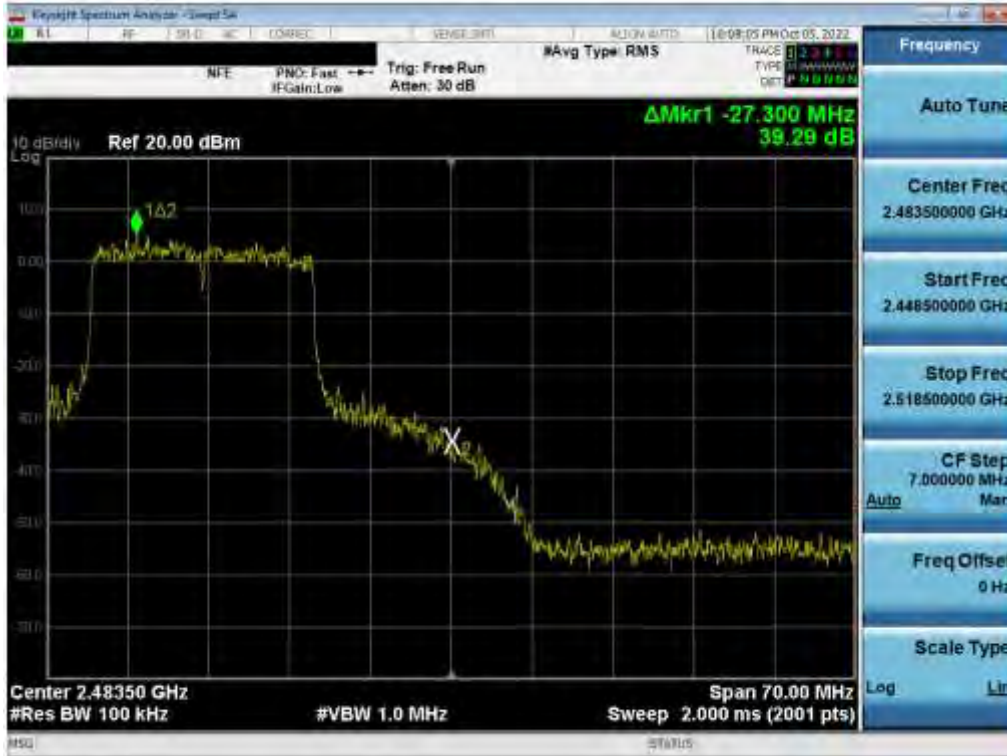
Plot 7-91. Band Edge Plot (802.11ax (2.4GHz) – Ch. 11) SISO ANT 2
