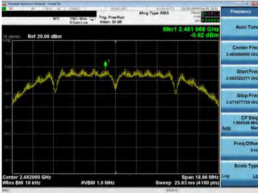
Plot 7-39. Power Spectral Density Plot (802.11b – Ch. 11)
