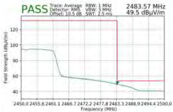
Plot 7-166. Radiated Restricted Upper Band Edge Measurement SISO ANT2 (Average)
