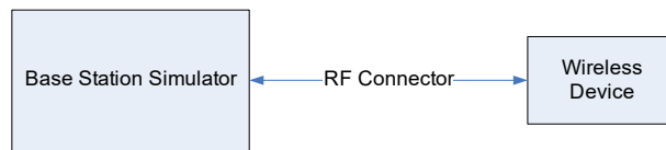
Figure 9-4 Power Measurement Setup – NR FDD
