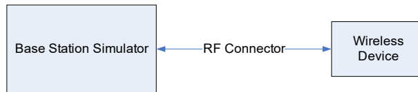
Figure 9-3 Power Measurement Setup
