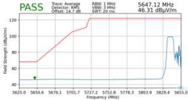
Plot 7-322. Radiated Lower Band Edge Plot MIMO (Average – UNII Band 4 – 106 Tones)
