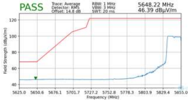
Plot 7-333. Radiated Lower Band Edge Plot MIMO (Average – UNII Band 4 – 242 Tones)
