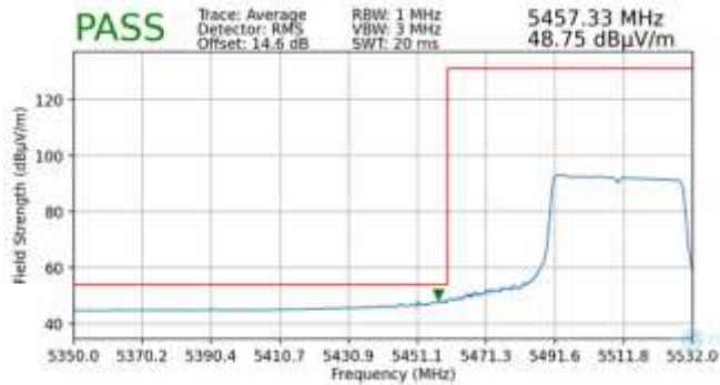
Plot 7-341. Radiated Lower Band Edge Plot MIMO (Average – UNII Band 2C – 484 Tones)
