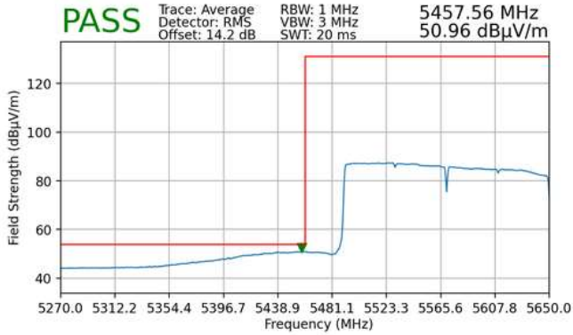
Plot 7-363. Radiated Lower Band Edge Plot MIMO (Average – UNII Band 2C – 996*2 Tones)
