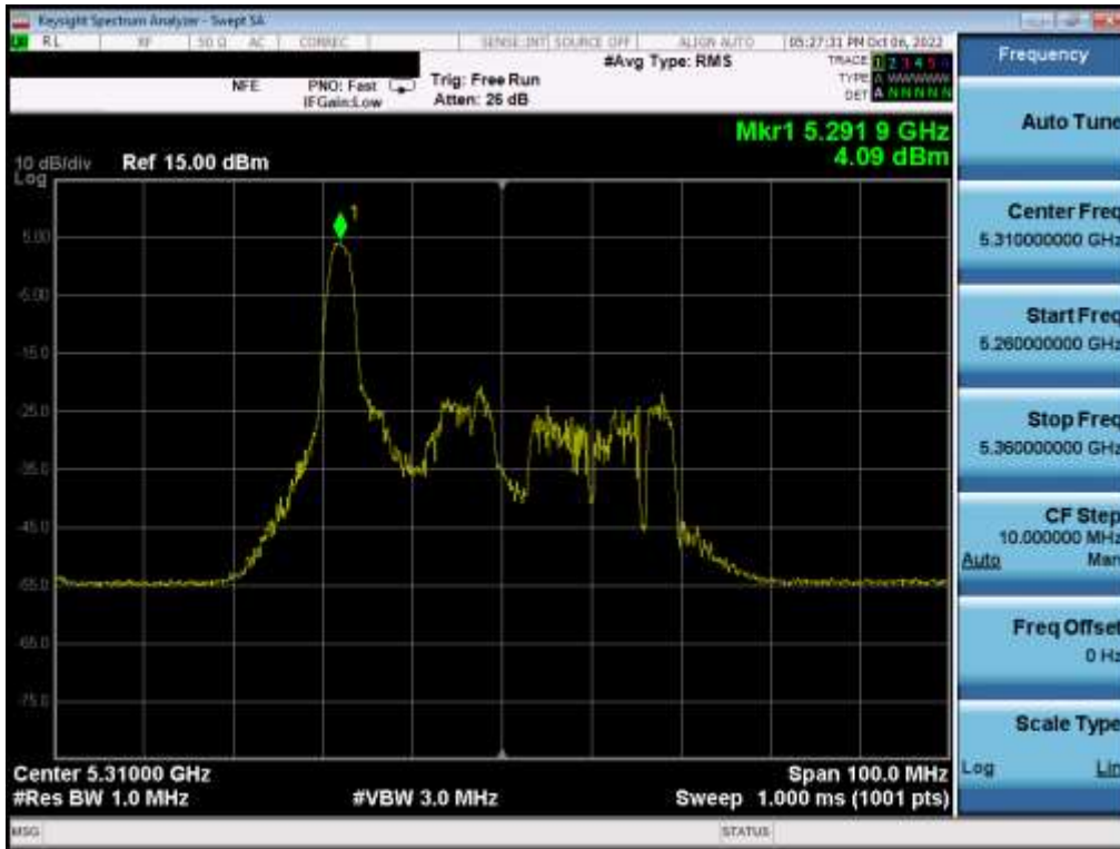
Plot 7-238. Power Spectral Density Plot MIMO ANT2 (40MHz BW 802.11ax – 26 Tones (UNII Band 2A) – Ch. 62)
