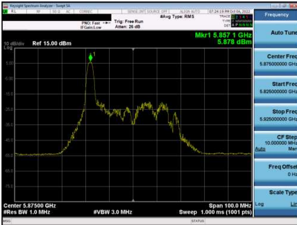
Plot 7-186. Power Spectral Density Plot MIMO ANT1 (40MHz BW 802.11ax – 26 Tones (UNII Band 3) – Ch. 175)
