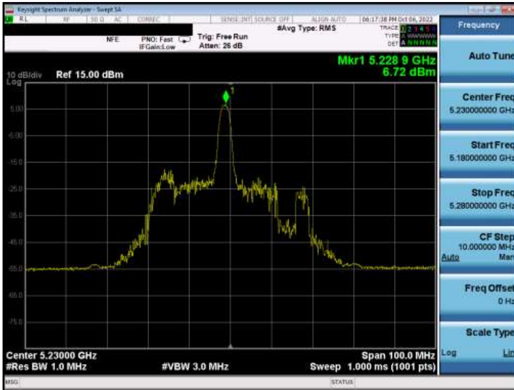
Plot 7-155. Power Spectral Density Plot MIMO ANT1 (40MHz BW 802.11ax – 26 Tones (UNII Band 1) – Ch. 46)
