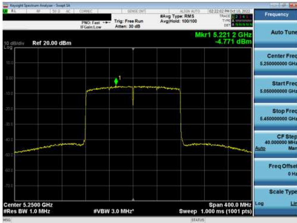
Plot 7-271. Power Spectral Density Plot MIMO ANT2 (160MHz BW 802.11ax – Full Tones (UNII Band 1/2A) – Ch. 50)
