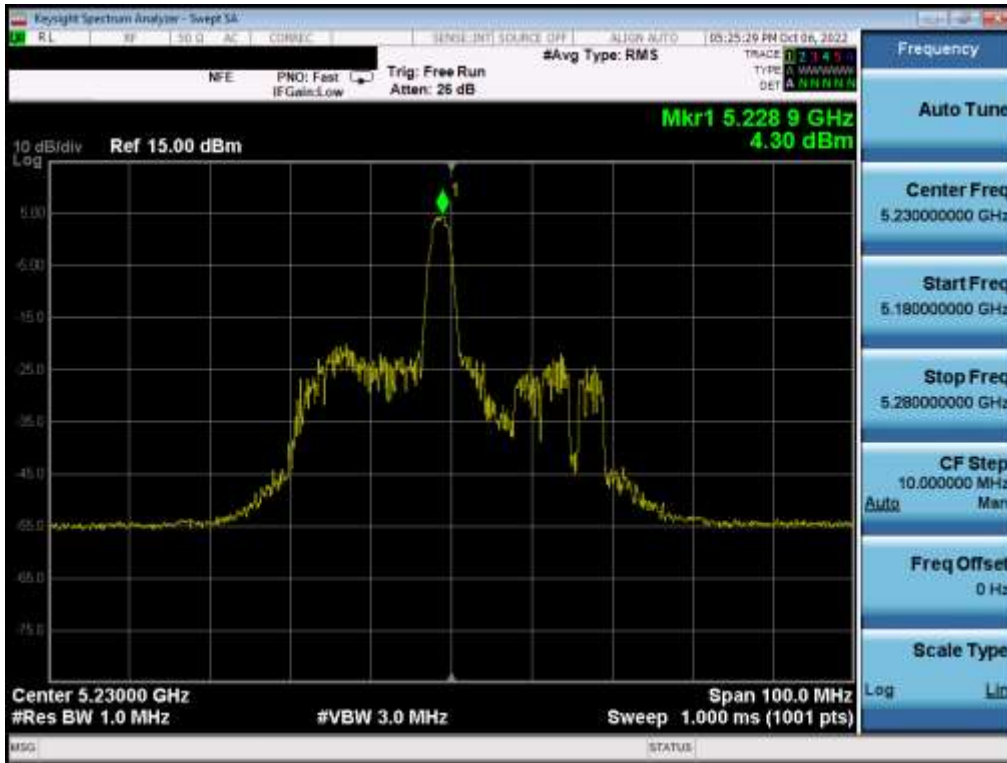
Plot 7-230. Power Spectral Density Plot MIMO ANT2 (40MHz BW 802.11ax – 26 Tones (UNII Band 1) – Ch. 46)
