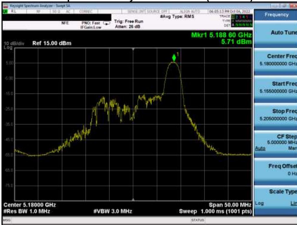
Plot 7-151. Power Spectral Density Plot MIMO ANT1 (20MHz BW 802.11ax – 26 Tones (UNII Band 1) – Ch. 36)
