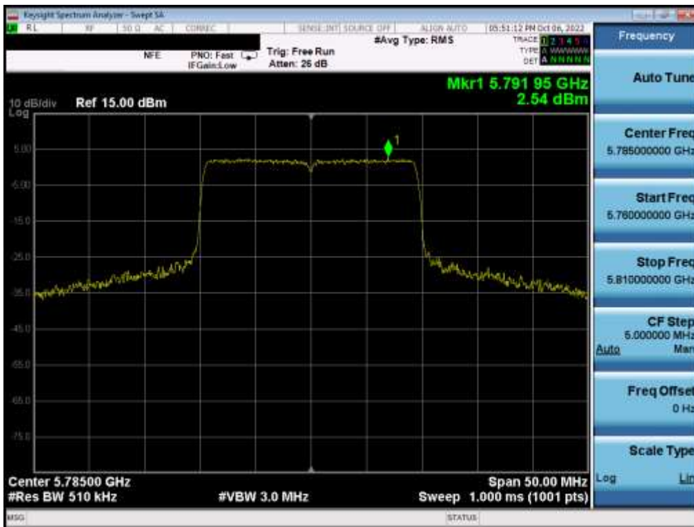
Plot 7-289. Power Spectral Density Plot MIMO ANT2 (20MHz BW 802.11ax – Full Tones (UNII Band 3) – Ch. 157)
