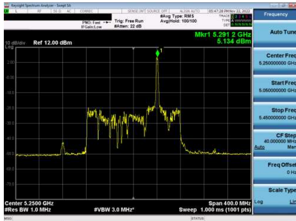
Plot 7-233. Power Spectral Density Plot MIMO ANT2 (160MHz(U) BW 802.11ax – 26 Tones (UNII Band 1/2A) – Ch. 50)
