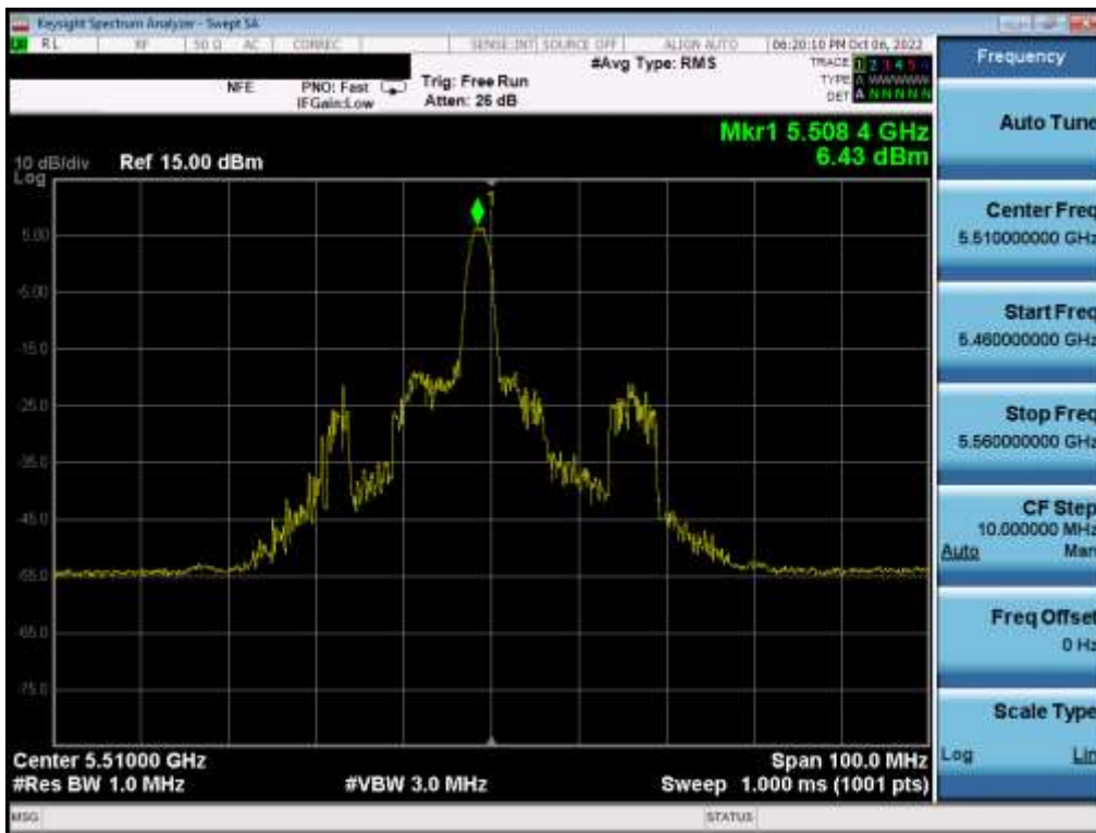
Plot 7-168. Power Spectral Density Plot MIMO ANT1 (40MHz BW 802.11ax – 26 Tones (UNII Band 2C) – Ch. 102)
