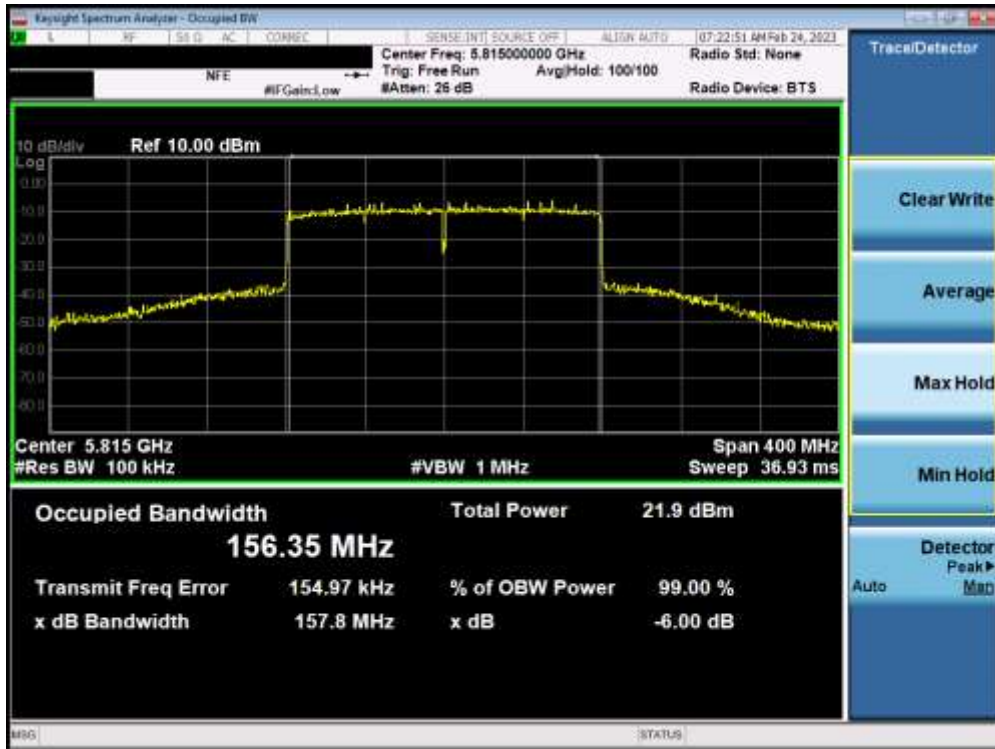
Plot 7-150. 6dB Bandwidth Plot MIMO ANT2 (160MHz BW 802.11ax – 996*2 Tones (UNII Band 3/4) – Ch. 163)
