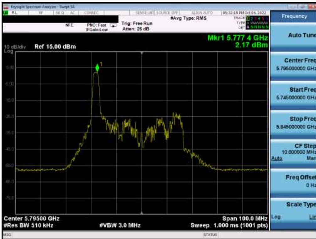
Plot 7-255. Power Spectral Density Plot MIMO ANT2 (40MHz BW 802.11ax – 26 Tones (UNII Band 3) – Ch. 159)
