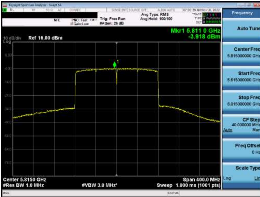
Plot 7-300. Power Spectral Density Plot MIMO ANT2 (160MHz(L) BW 802.11ax – Full Tones (UNII Band 3/4) – Ch. 163)
