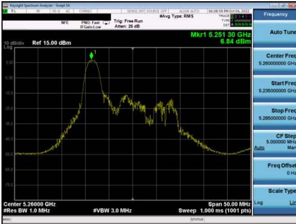
Plot 7-159. Power Spectral Density Plot MIMO ANT1 (20MHz BW 802.11ax – 26 Tones (UNII Band 2A) – Ch. 52)
