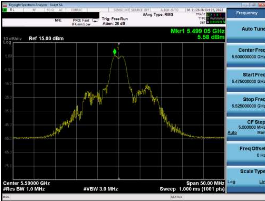
Plot 7-165. Power Spectral Density Plot MIMO ANT1 (20MHz BW 802.11ax – 26 Tones (UNII Band 2C) – Ch. 100)
