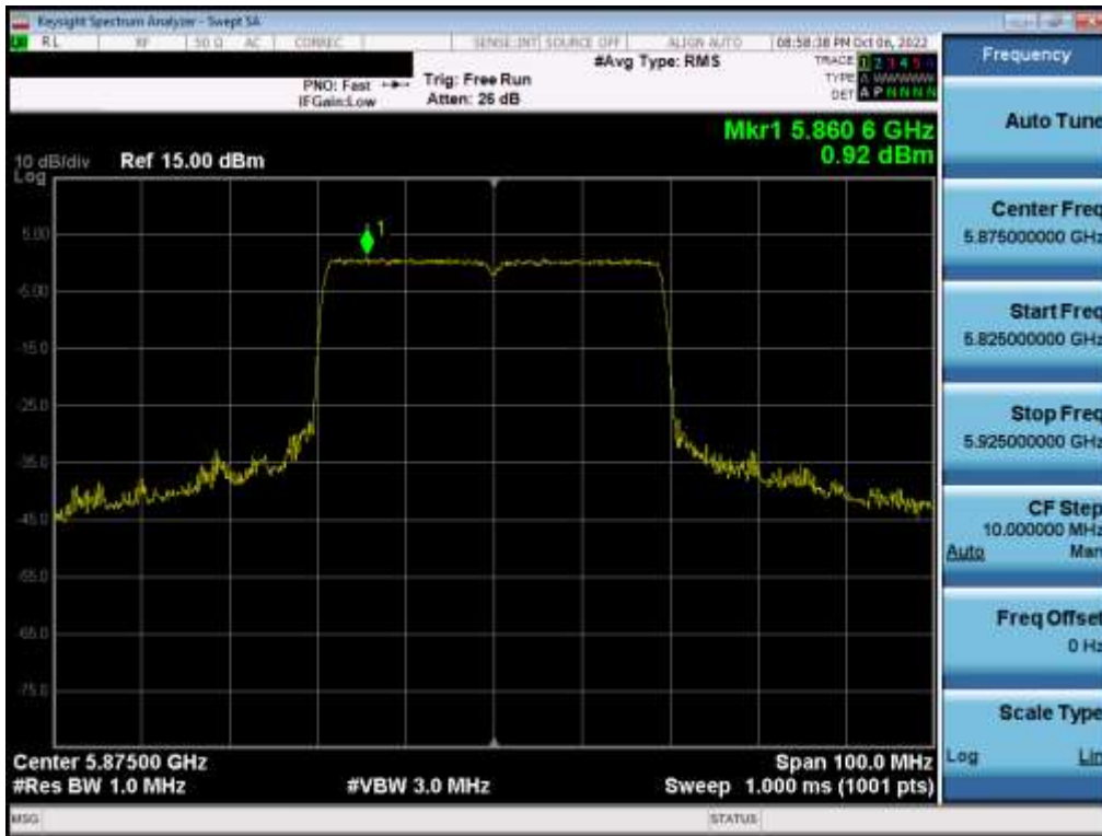
Plot 7-298. Power Spectral Density Plot MIMO ANT2 (40MHz BW 802.11ax – Full Tones (UNII Band 3) – Ch. 175)
