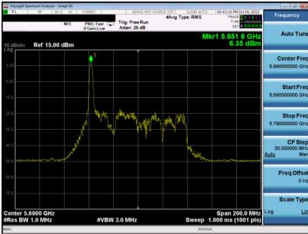
Plot 7-173. Power Spectral Density Plot MIMO ANT1 (80MHz BW 802.11ax – 26 Tones (UNII Band 2C) – Ch. 138)
