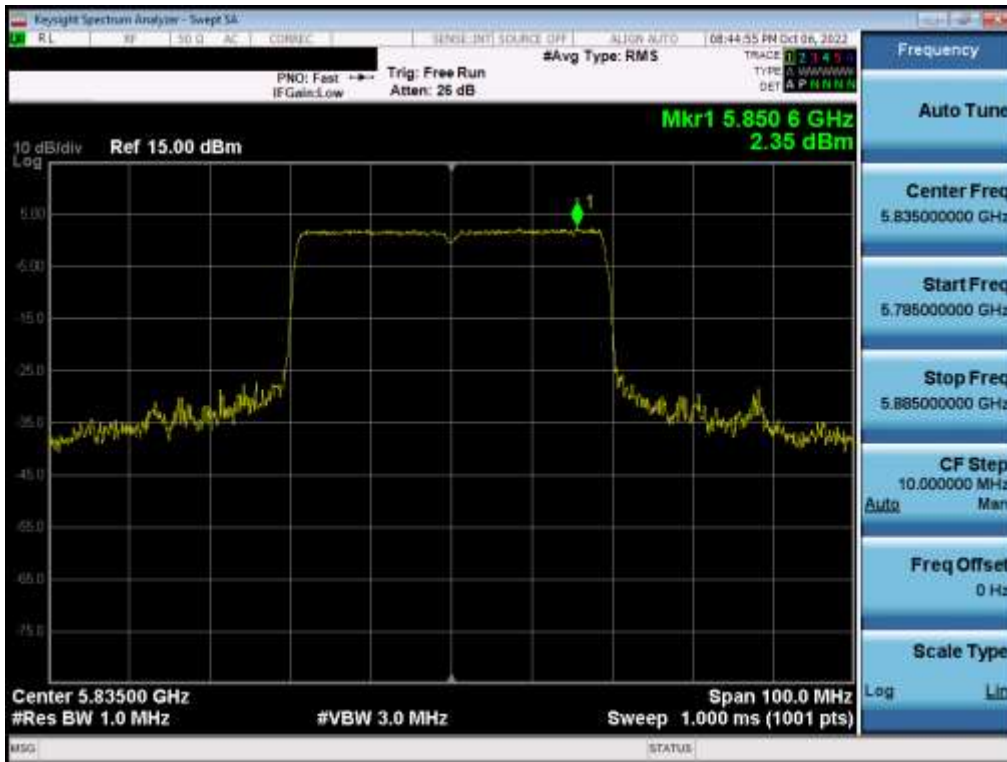
Plot 7-222. Power Spectral Density Plot MIMO ANT1 (40MHz BW 802.11ax – Full Tones (UNII Band 3/4) – Ch. 167)
