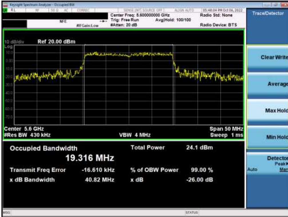
Plot 7-88. 26dB Bandwidth Plot MIMO ANT2 (20MHz BW 802.11ax – 242 Tones (UNII Band 2C) – Ch. 120)
