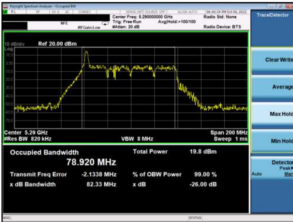
Plot 7-14. 26dB Bandwidth Plot MIMO ANT1 (80MHz BW 802.11ax – 26 Tones (UNII Band 2A) – Ch. 58)
