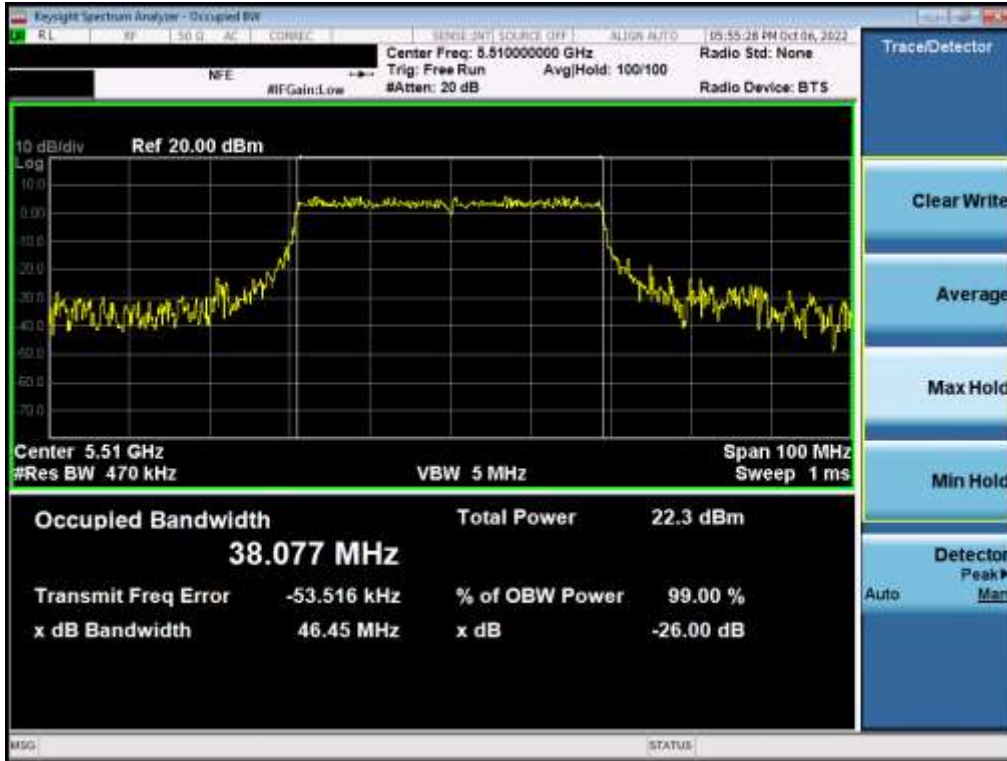
Plot 7-90. 26dB Bandwidth Plot MIMO ANT2 (40MHz BW 802.11ax – 484 Tones (UNII Band 2C) – Ch. 102)
