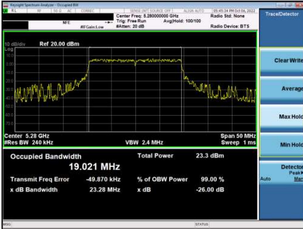
Plot 7-82. 26dB Bandwidth Plot MIMO ANT2 (20MHz BW 802.11ax – 242 Tones (UNII Band 2A) – Ch. 56)
