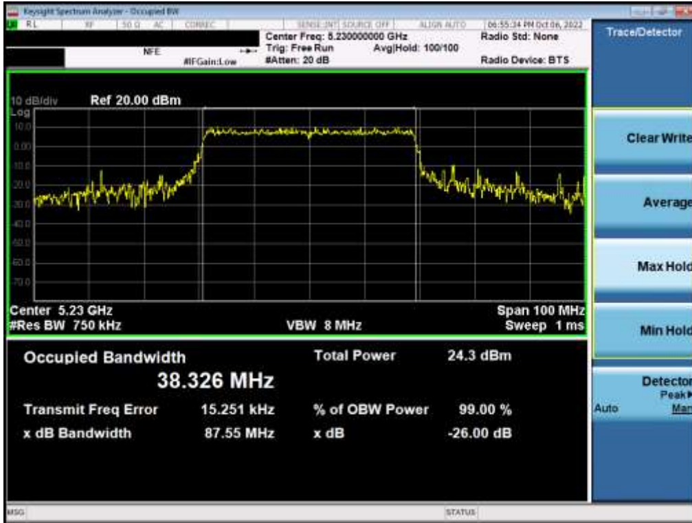
Plot 7-30. 26dB Bandwidth Plot MIMO ANT1 (40MHz BW 802.11ax – 484 Tones (UNII Band 1) – Ch. 46)
