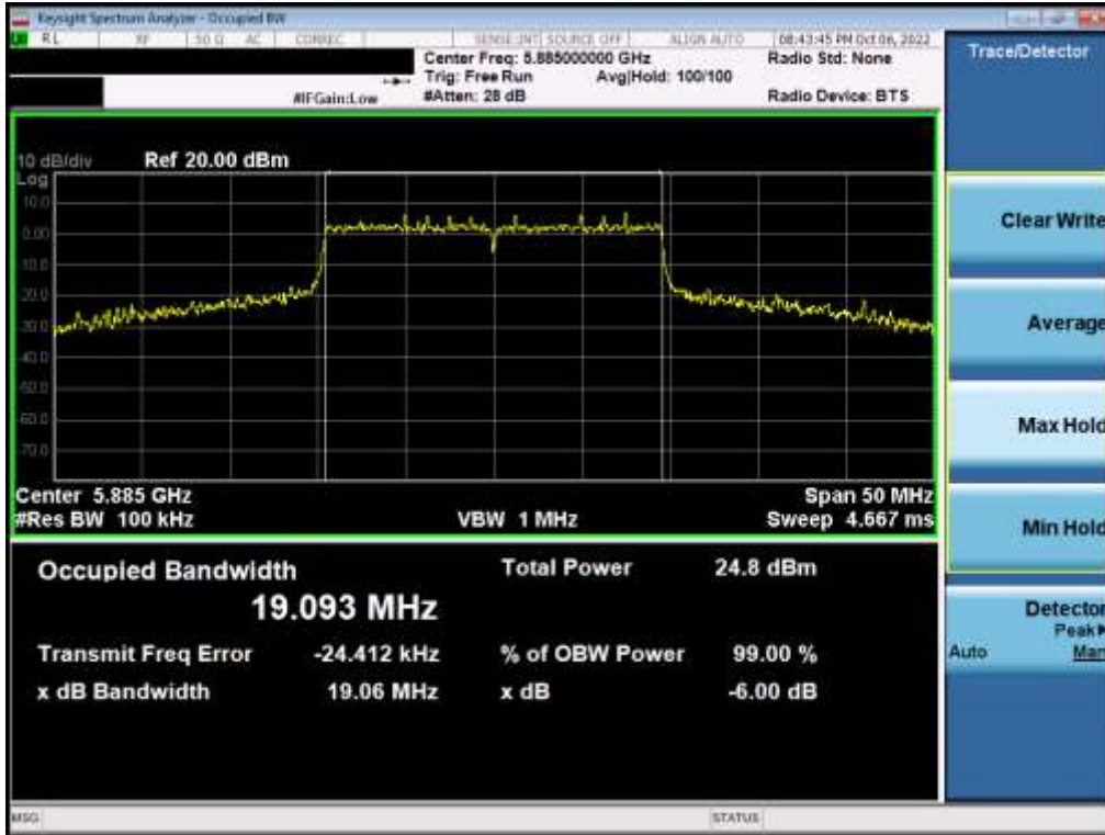
Plot 7-119. 6dB Bandwidth Plot MIMO ANT1 (20MHz BW 802.11ax – 242 Tones (UNII Band 3) – Ch. 177)
