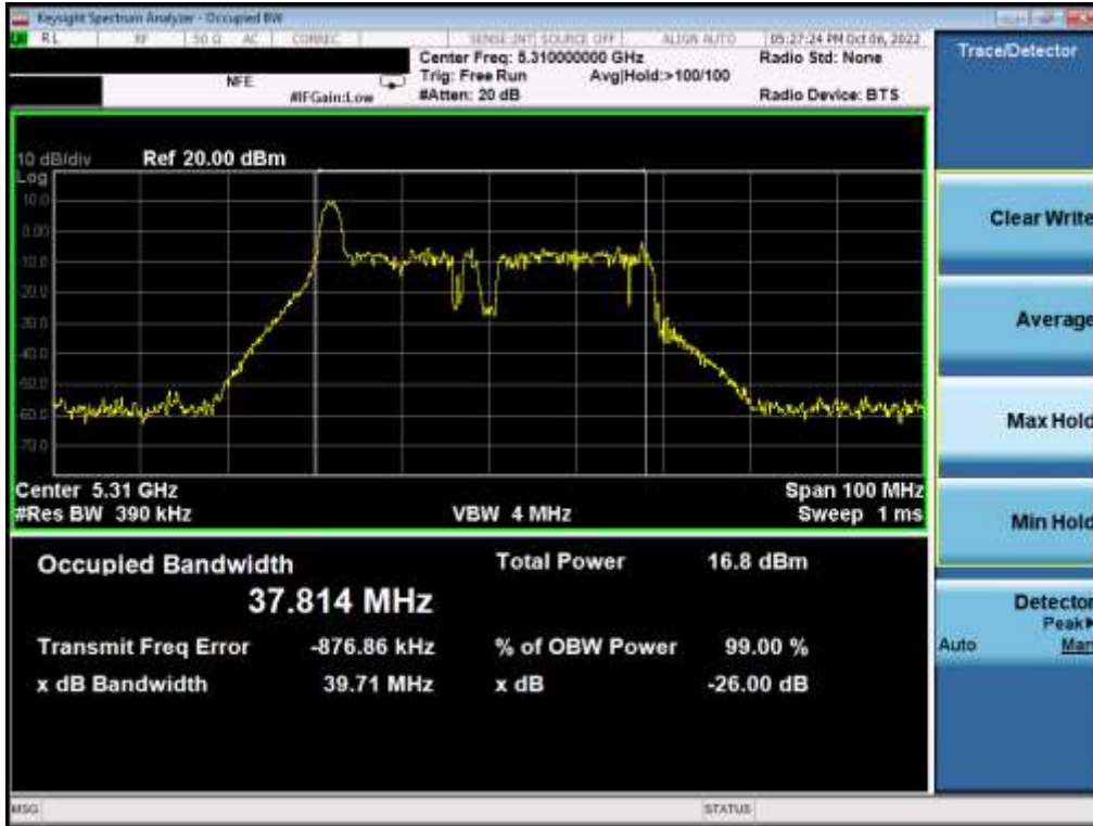
Plot 7-61. 26dB Bandwidth Plot MIMO ANT2 (40MHz BW 802.11ax – 26 Tones (UNII Band 2A) – Ch. 62)
