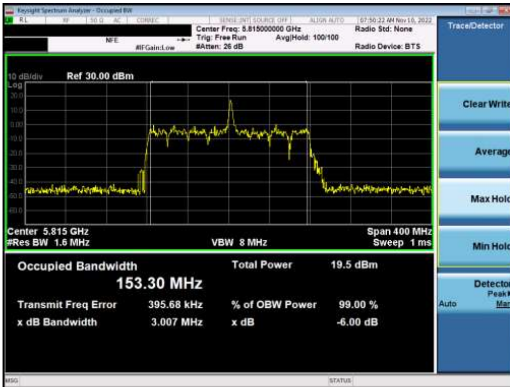
Plot 7-110. 6dB Bandwidth Plot MIMO ANT1 (160MHz(U) BW 802.11ax – 26 Tones (UNII Band 3/4) – Ch. 163)
