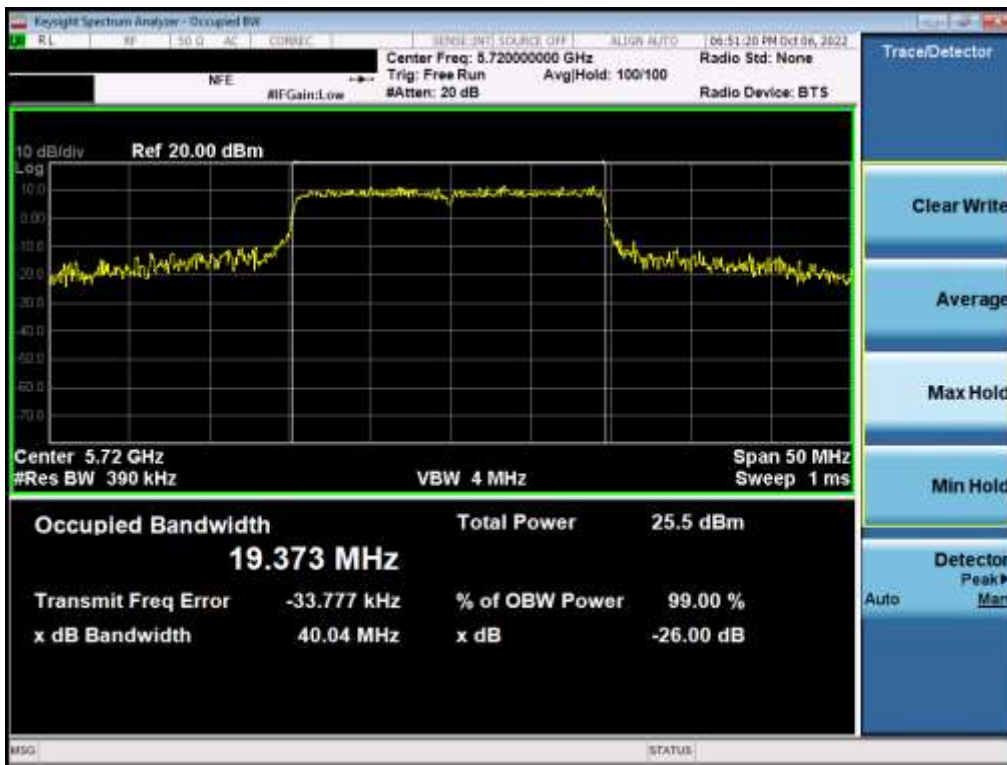
Plot 7-41. 26dB Bandwidth Plot MIMO ANT1 (20MHz BW 802.11ax – 242 Tones (UNII Band 2C) – Ch. 144)
