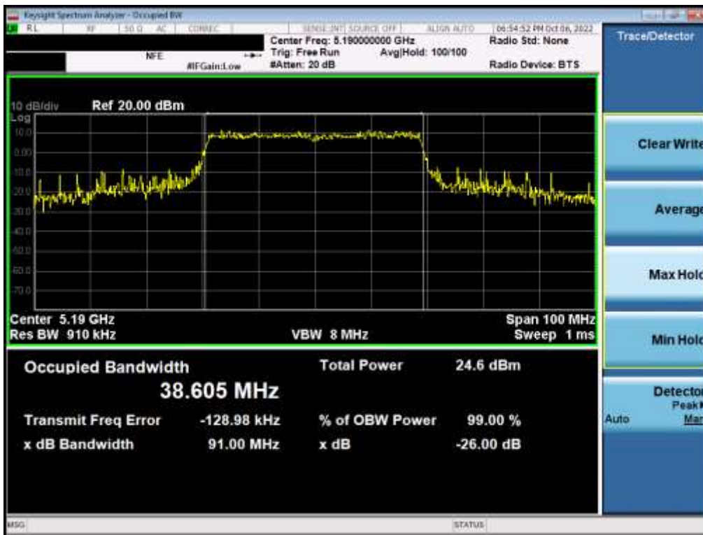
Plot 7-29. 26dB Bandwidth Plot MIMO ANT1 (40MHz BW 802.11ax – 484 Tones (UNII Band 1) – Ch. 38)
