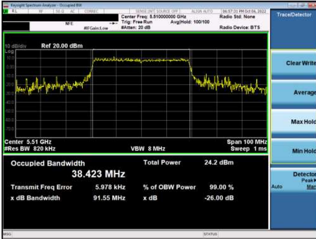
Plot 7-42. 26dB Bandwidth Plot MIMO ANT1 (40MHz BW 802.11ax – 484 Tones (UNII Band 2C) – Ch. 102)
