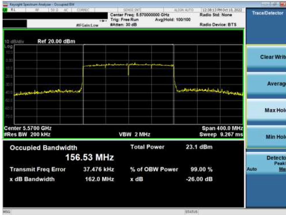
Plot 7-48. 26dB Bandwidth Plot MIMO ANT1 (160MHz BW 802.11ax – 996*2 Tones (UNII Band 2C) – Ch. 114)
