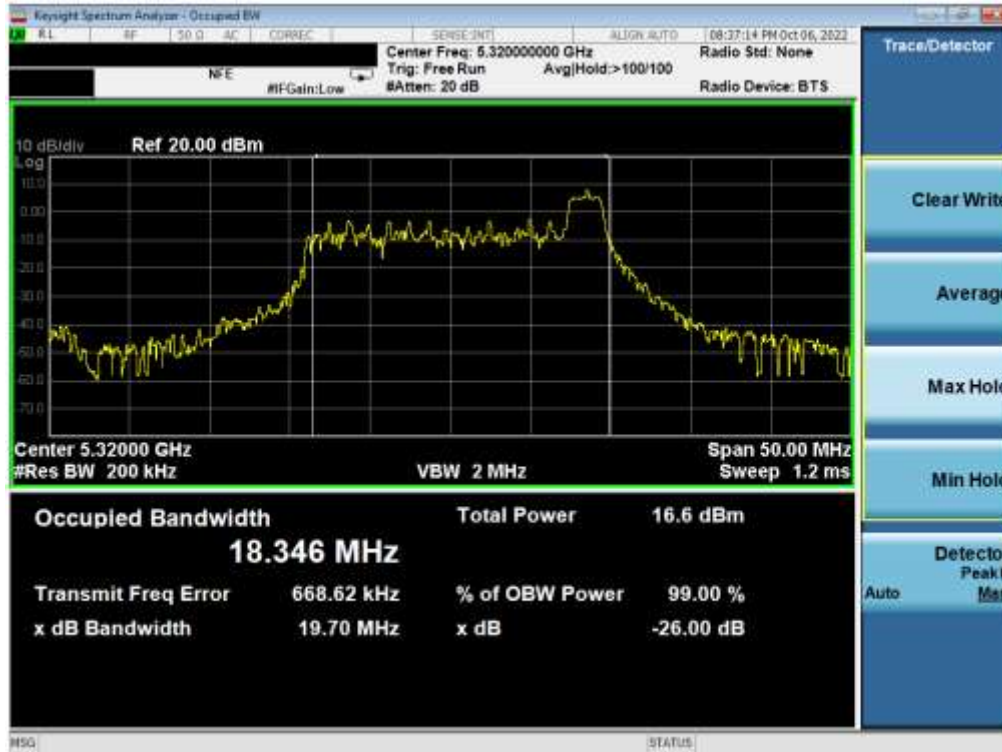
Plot 7-59. 26dB Bandwidth Plot MIMO ANT2 (20MHz BW 802.11ax – 26 Tones (UNII Band 2A) – Ch. 64)
