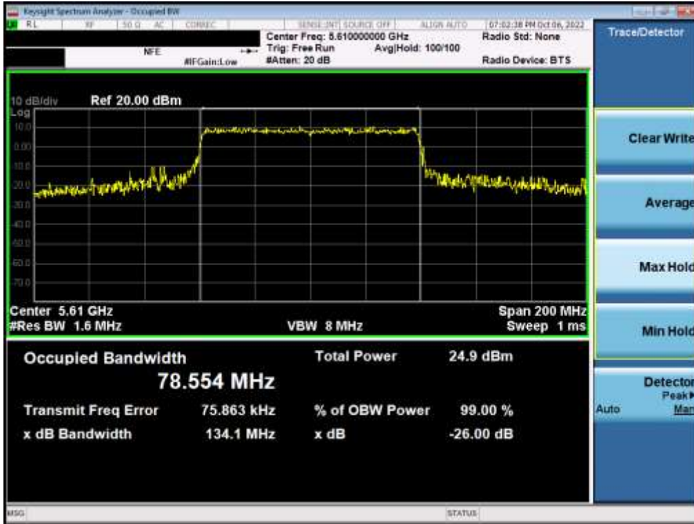
Plot 7-46. 26dB Bandwidth Plot MIMO ANT1 (80MHz BW 802.11ax – 996 Tones (UNII Band 2C) – Ch. 122)
