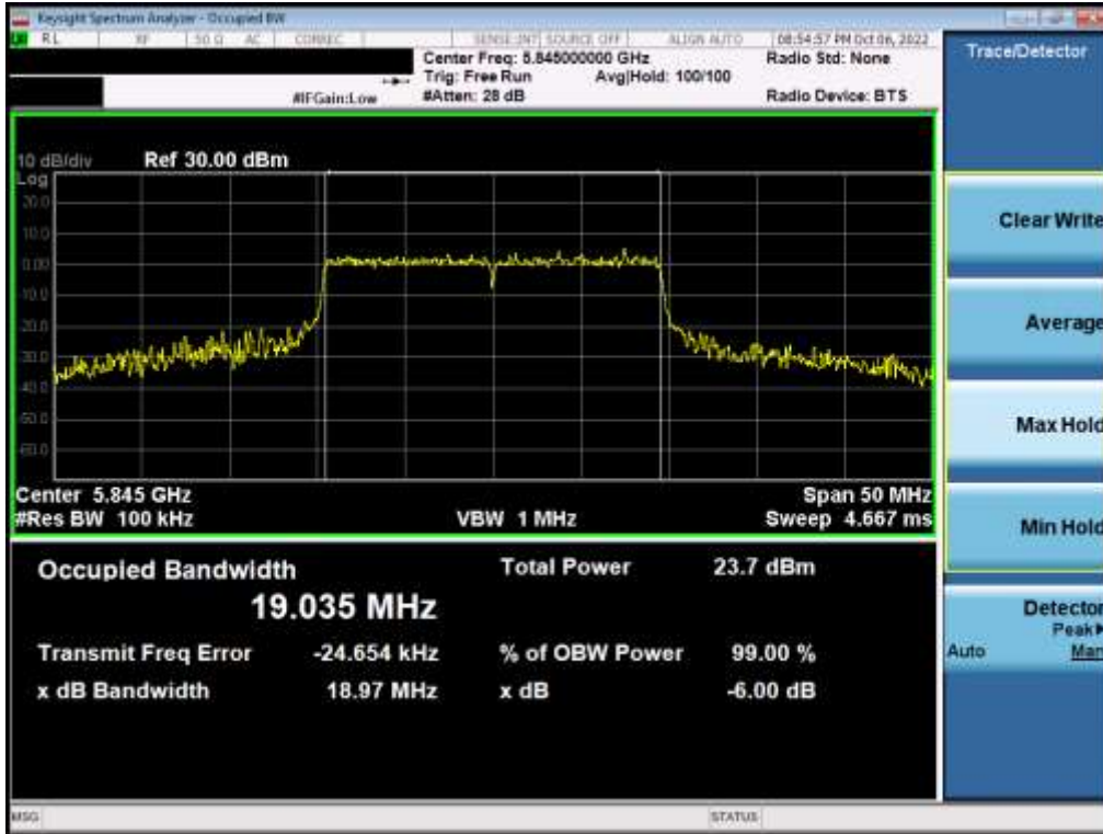
Plot 7-144. 6dB Bandwidth Plot MIMO ANT2 (20MHz BW 802.11ax – 242 Tones (UNII Band 3/4) – Ch. 169)
