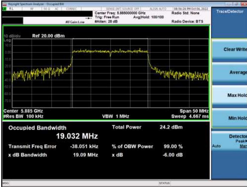
Plot 7-146. 6dB Bandwidth Plot MIMO ANT2 (20MHz BW 802.11ax – 242 Tones (UNII Band 3) – Ch. 177)
