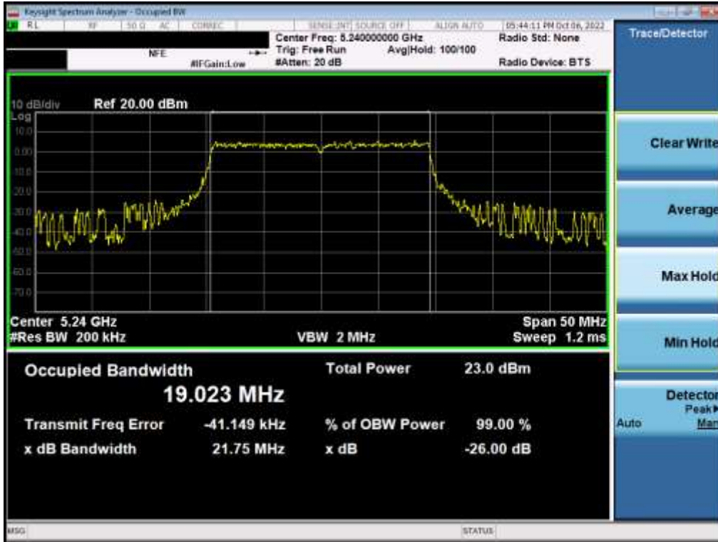
Plot 7-76. 26dB Bandwidth Plot MIMO ANT2 (20MHz BW 802.11ax – 242 Tones (UNII Band 1) – Ch. 48)
