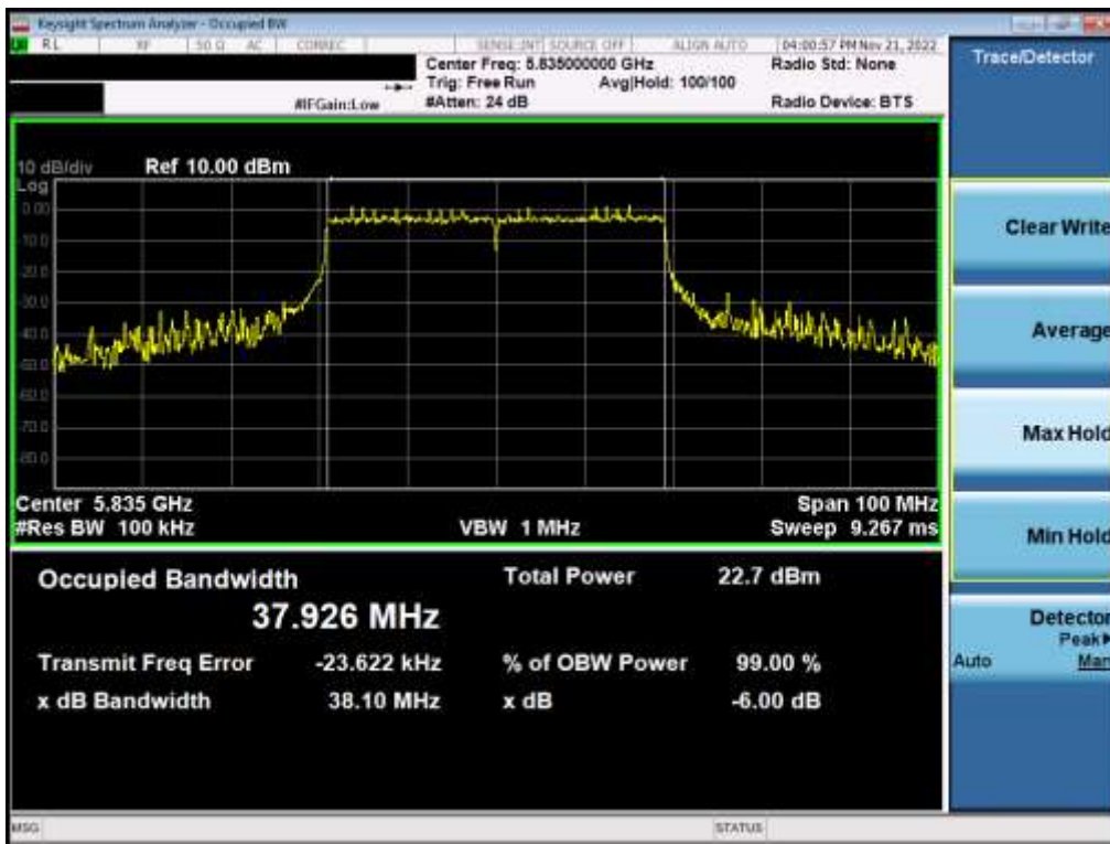
Plot 7-120. 6dB Bandwidth Plot MIMO ANT1 (40MHz BW 802.11ax – 484 Tones (UNII Band 3/4) – Ch. 167)
