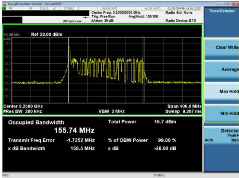
Plot 7-55. 26dB Bandwidth Plot MIMO ANT2 (160MHz(L) BW 802.11ax – 26 Tones (UNII Band 1/2A) – Ch. 50)
