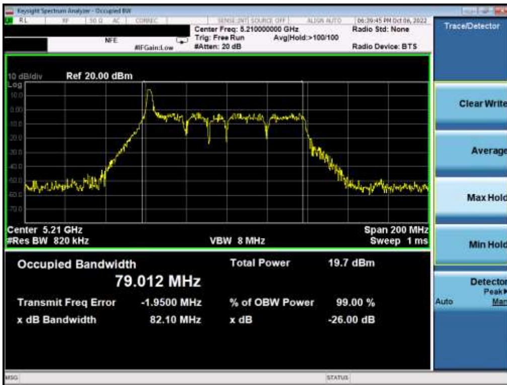
Plot 7-6. 26dB Bandwidth Plot MIMO ANT1 (80MHz BW 802.11ax – 26 Tones (UNII Band 1) – Ch. 42)
