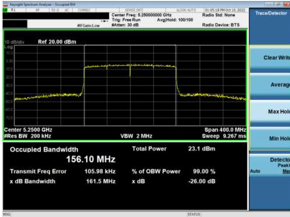
Plot 7-80. 26dB Bandwidth Plot MIMO ANT2 (160MHz BW 802.11ax – 996*2 Tones (UNII Band 1/2A) – Ch. 50)
