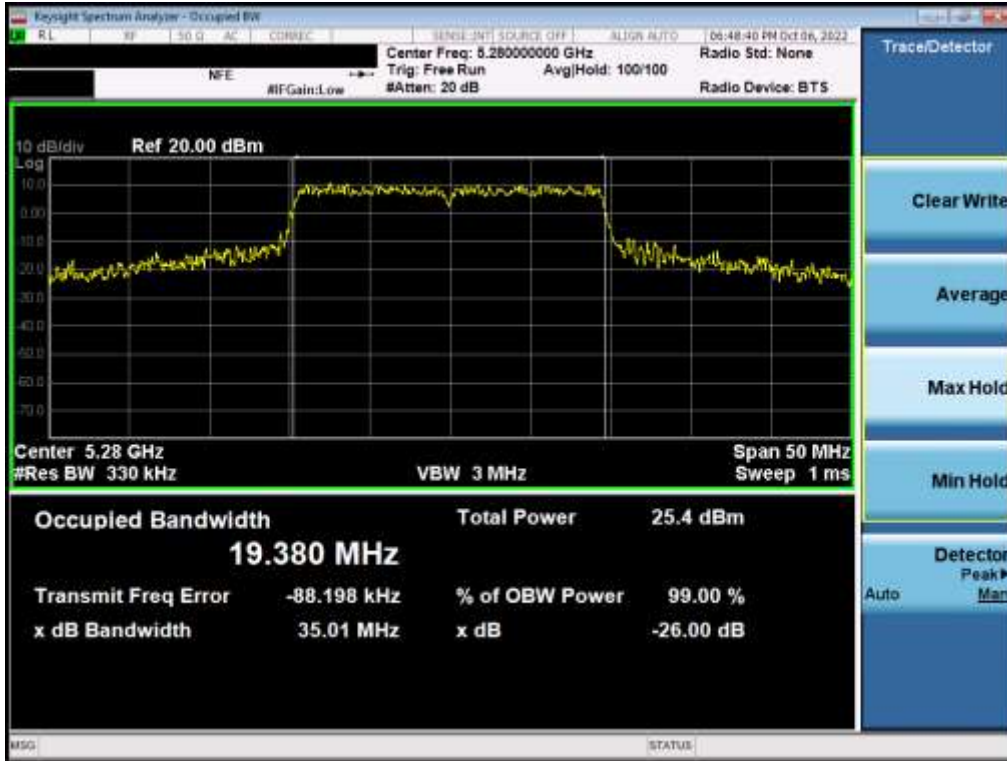
Plot 7-34. 26dB Bandwidth Plot MIMO ANT1 (20MHz BW 802.11ax – 242 Tones (UNII Band 2A) – Ch. 56)
