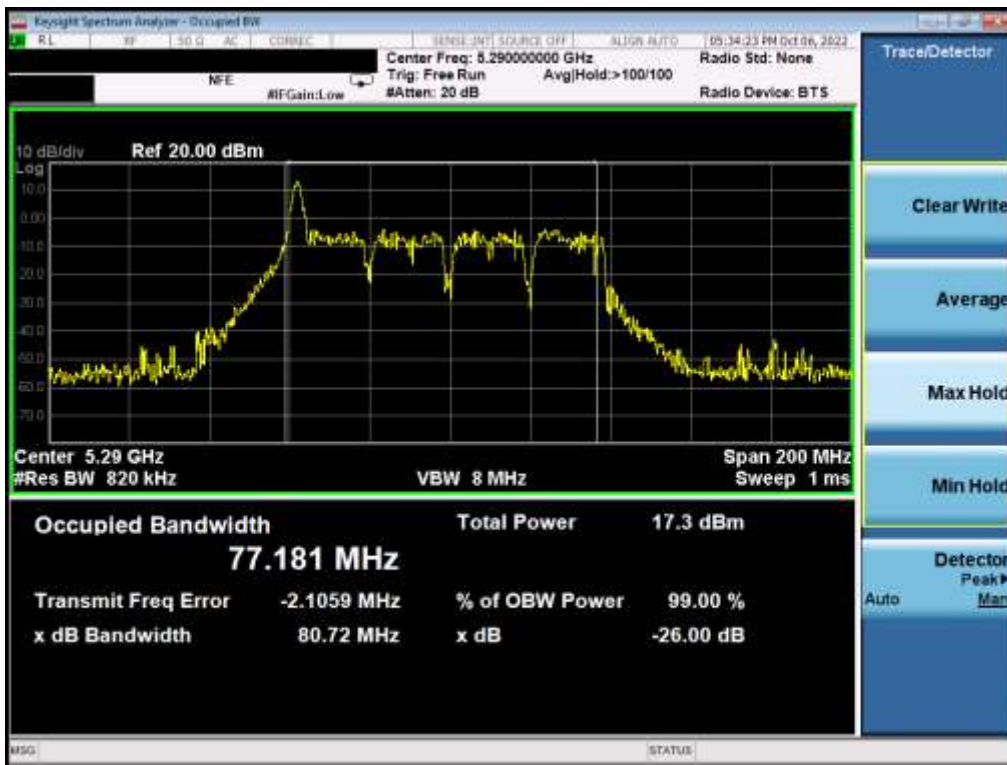
Plot 7-62. 26dB Bandwidth Plot MIMO ANT2 (80MHz BW 802.11ax – 26 Tones (UNII Band 2A) – Ch. 58)
