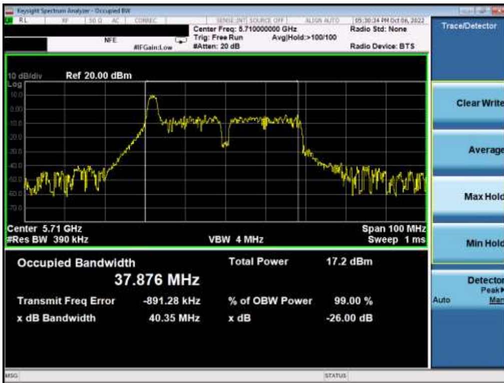
Plot 7-68. 26dB Bandwidth Plot MIMO ANT2 (40MHz BW 802.11ax – 26 Tones (UNII Band 2C) – Ch. 142)
