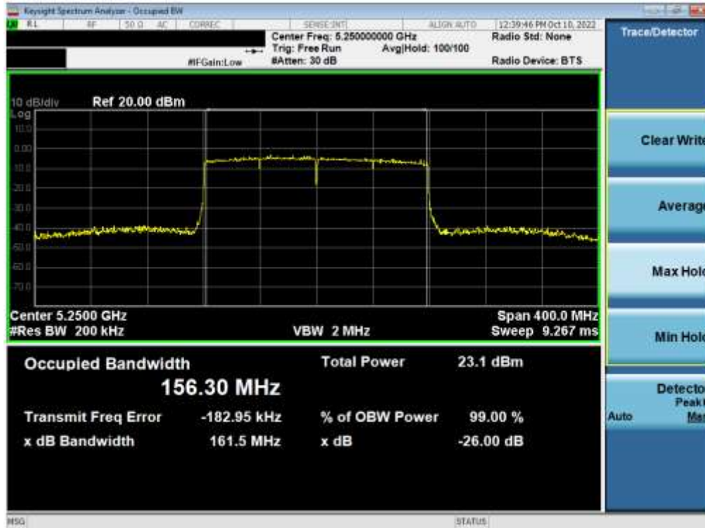
Plot 7-32. 26dB Bandwidth Plot MIMO ANT1 (160MHz BW 802.11ax – 996*2 Tones (UNII Band 1/2A) – Ch. 50)
