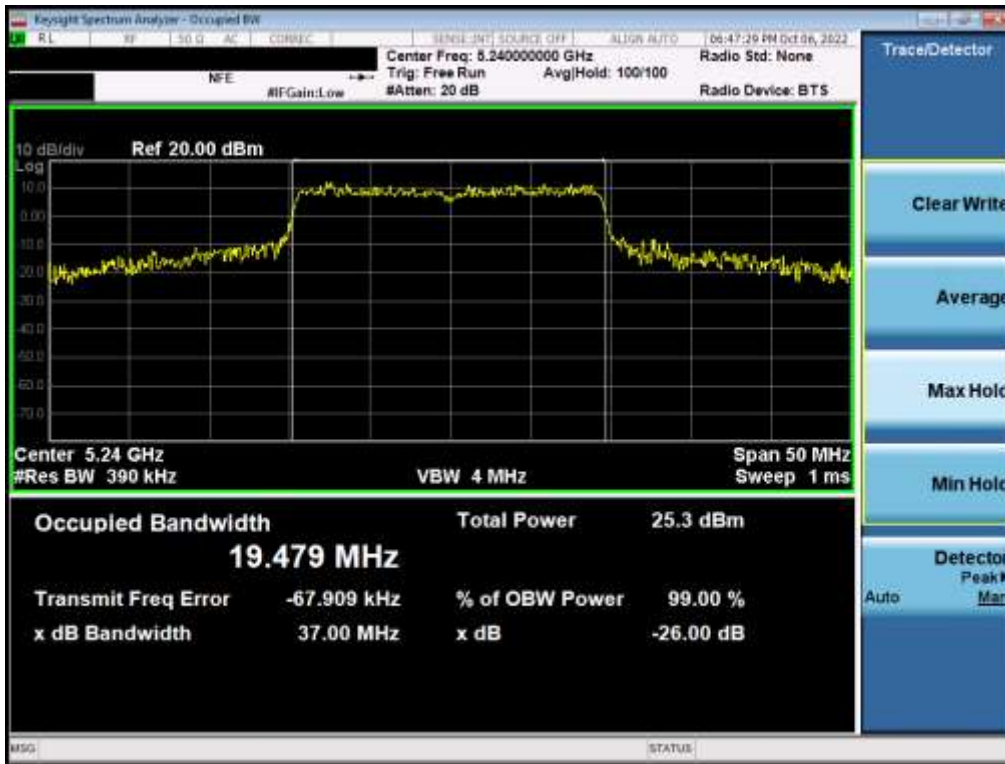
Plot 7-28. 26dB Bandwidth Plot MIMO ANT1 (20MHz BW 802.11ax – 242 Tones (UNII Band 1) – Ch. 48)
