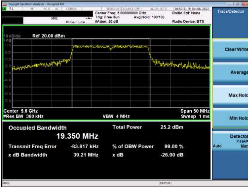
Plot 7-40. 26dB Bandwidth Plot MIMO ANT1 (20MHz BW 802.11ax – 242 Tones (UNII Band 2C) – Ch. 120)
