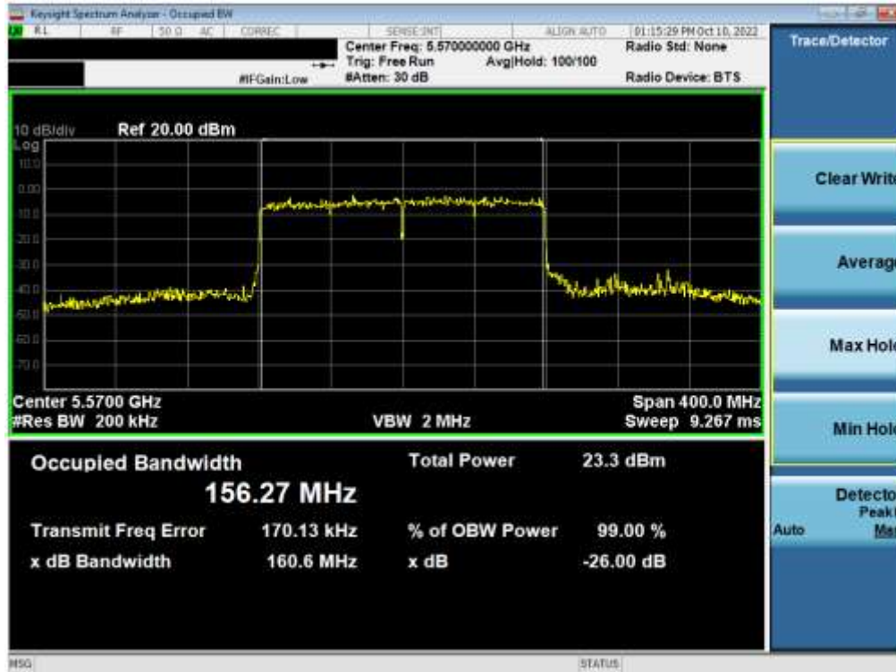
Plot 7-96. 26dB Bandwidth Plot MIMO ANT2 (160MHz BW 802.11ax – 996*2 Tones (UNII Band 2C) – Ch. 114)
