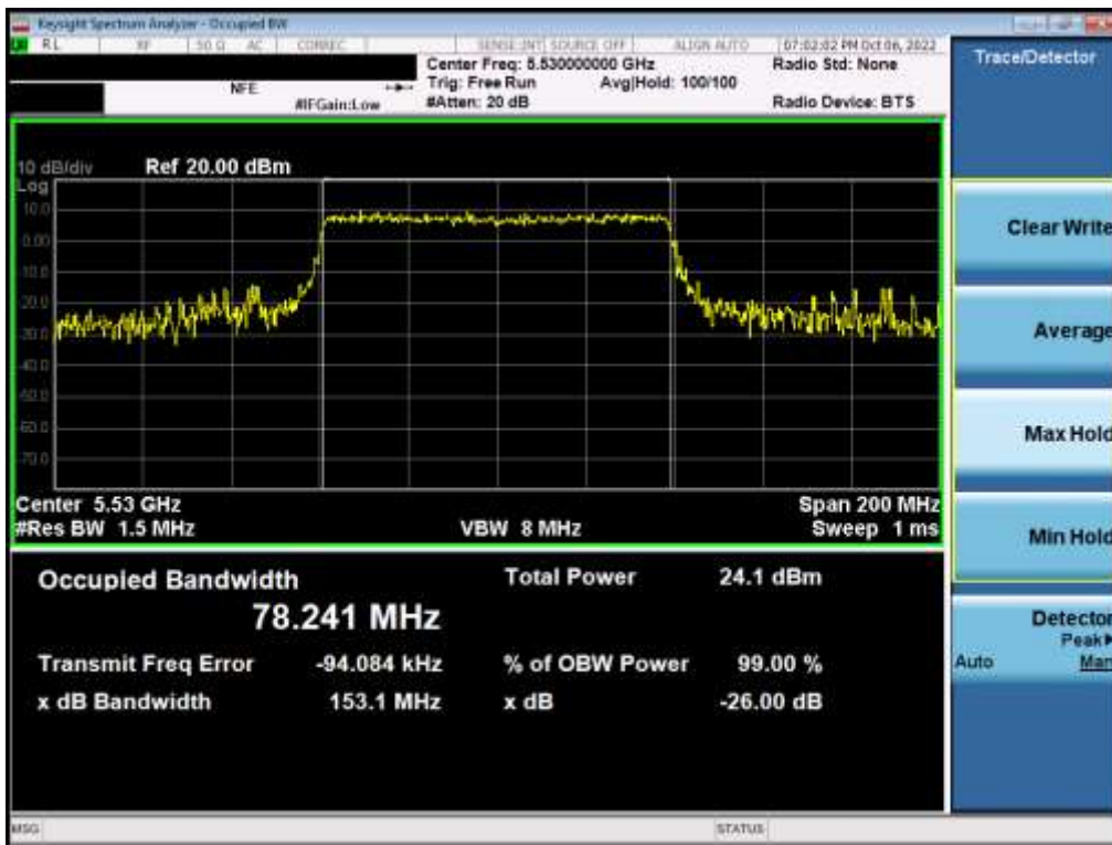
Plot 7-45. 26dB Bandwidth Plot MIMO ANT1 (80MHz BW 802.11ax – 996 Tones (UNII Band 2C) – Ch. 106)
