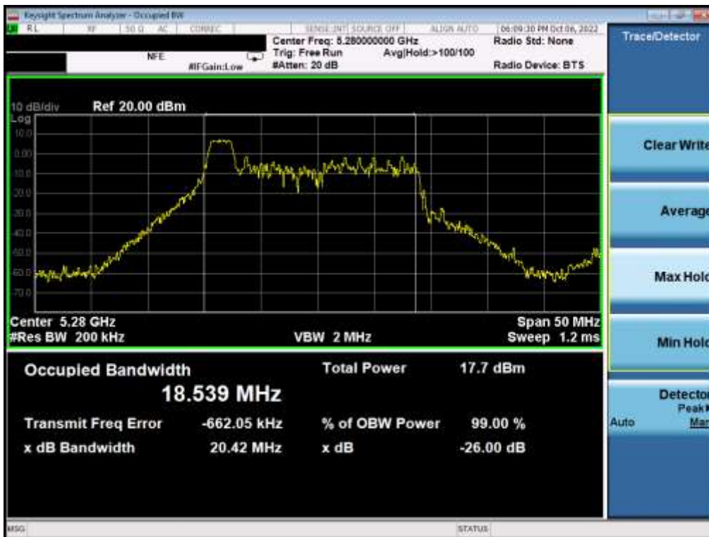
Plot 7-10. 26dB Bandwidth Plot MIMO ANT1 (20MHz BW 802.11ax – 26 Tones (UNII Band 2A) – Ch. 56)
