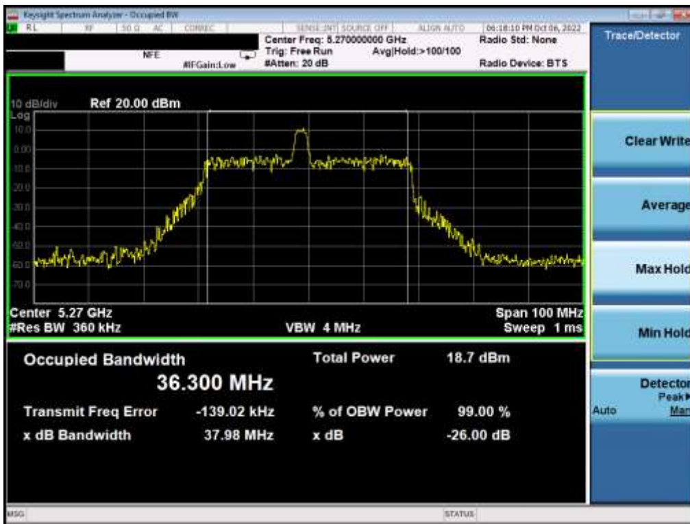
Plot 7-12. 26dB Bandwidth Plot MIMO ANT1 (40MHz BW 802.11ax – 26 Tones (UNII Band 2A) – Ch. 54)
