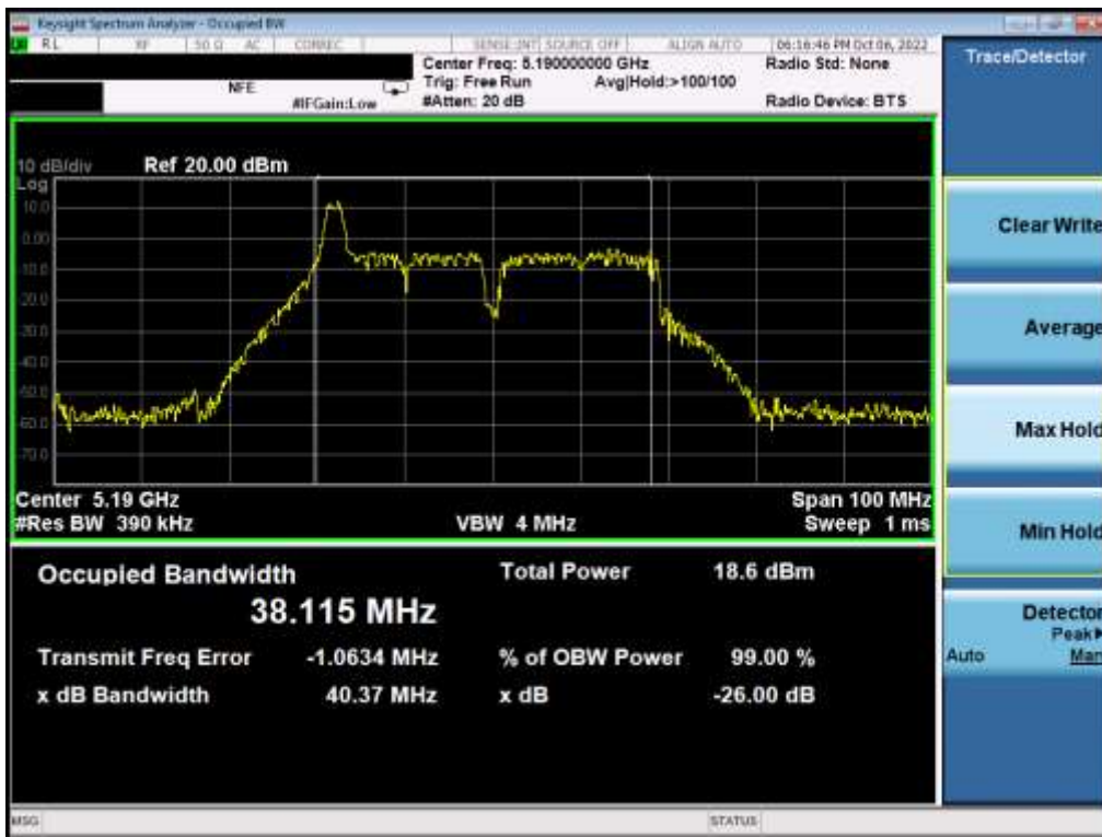
Plot 7-4. 26dB Bandwidth Plot MIMO ANT1 (40MHz BW 802.11ax – 26 Tones (UNII Band 1) – Ch. 38)
