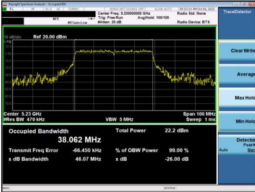
Plot 7-78. 26dB Bandwidth Plot MIMO ANT2 (40MHz BW 802.11ax – 484 Tones (UNII Band 1) – Ch. 46)
