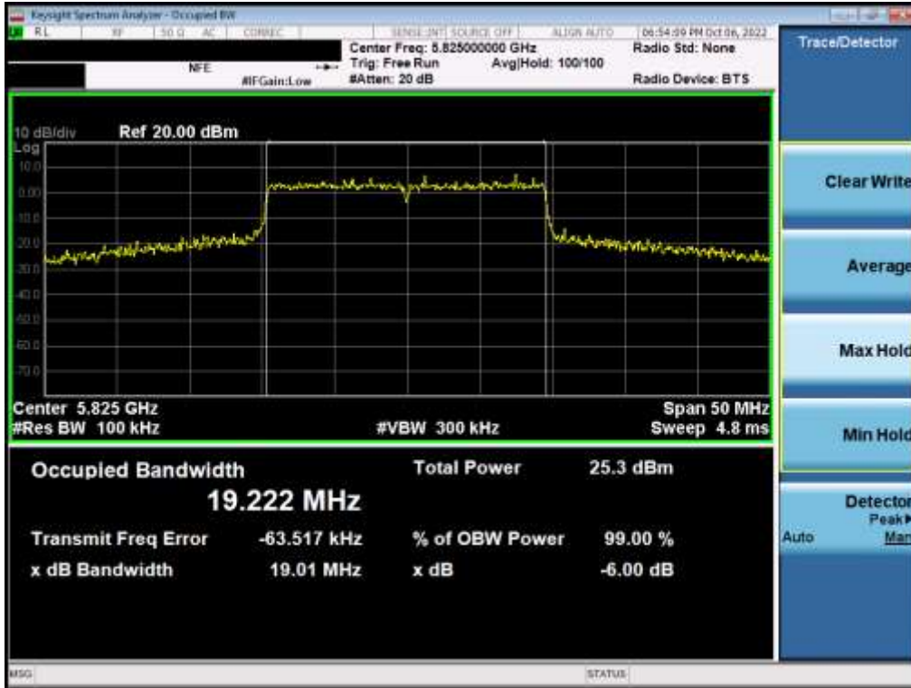
Plot 7-113. 6dB Bandwidth Plot MIMO ANT1 (20MHz BW 802.11ax – 242 Tones (UNII Band 3) – Ch. 165)
