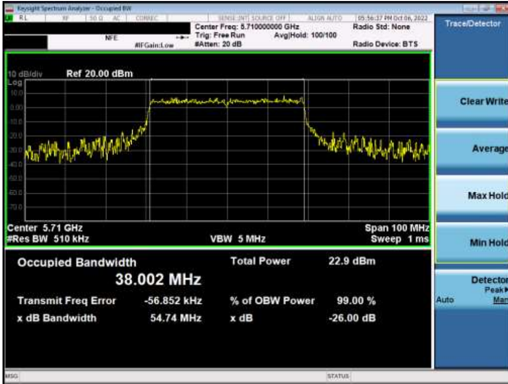
Plot 7-92. 26dB Bandwidth Plot MIMO ANT2 (40MHz BW 802.11ax – 484 Tones (UNII Band 2C) – Ch. 142)
