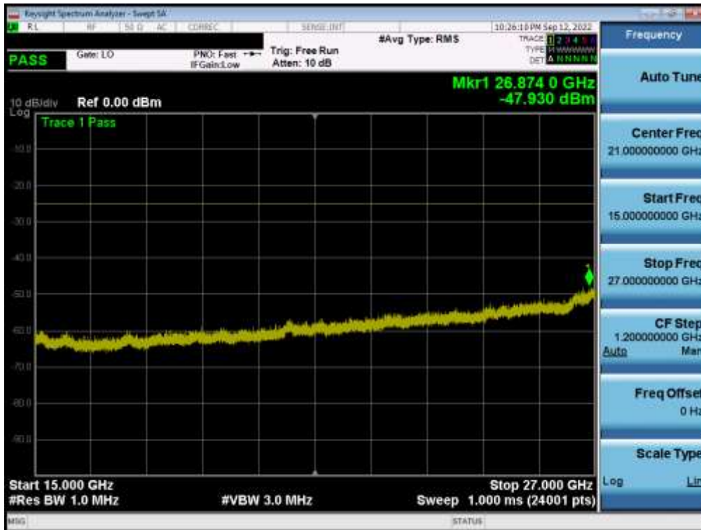
Plot 7-71. Conducted Spurious Plot (ULCA LTE B41(PC3) - 20MHz QPSK - RB Size 1, RB Offset 0 - High Channel)
