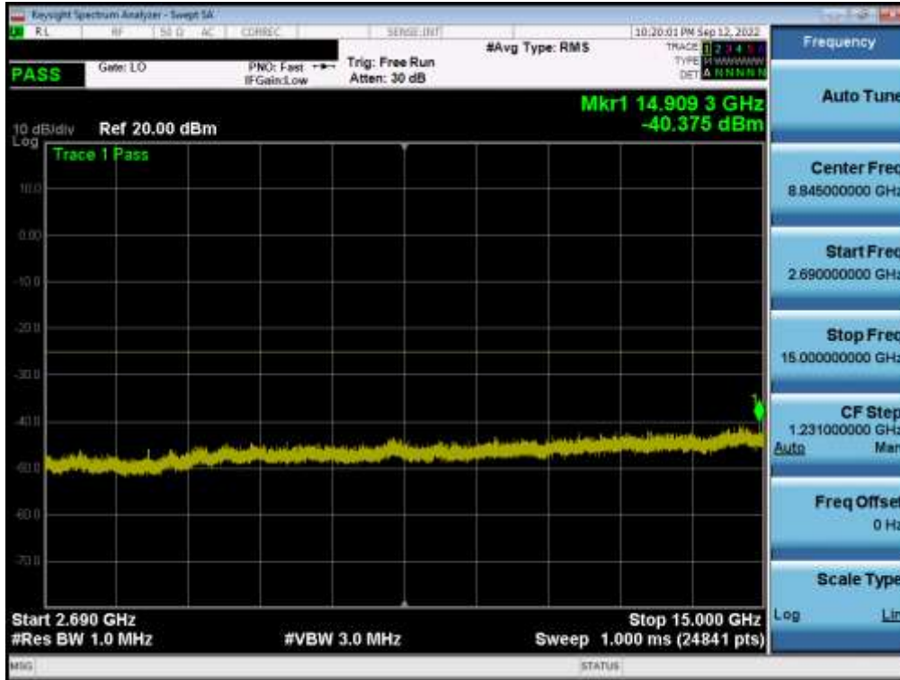
Plot 7-62. Conducted Spurious Plot (ULCA LTE B41(PC3) - 20MHz QPSK - RB Size 1, RB Offset 0 - Low Channel)
