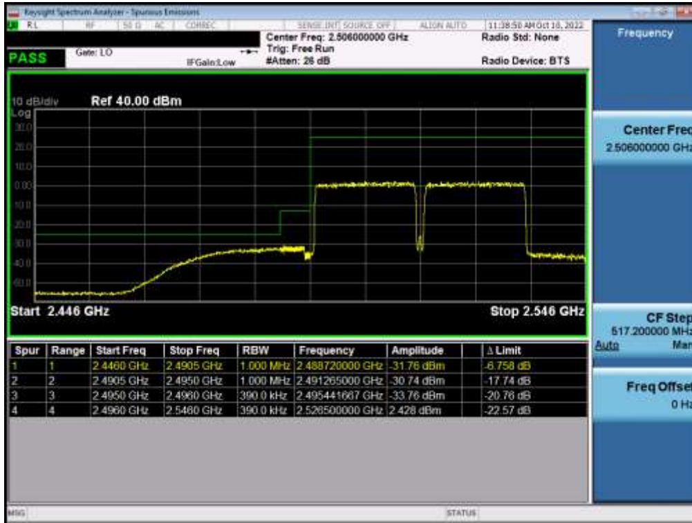
Plot 7-102. Lower ACP Plot (ULCA LTE B41(PC3) - 20MHz QPSK – Full RB)
