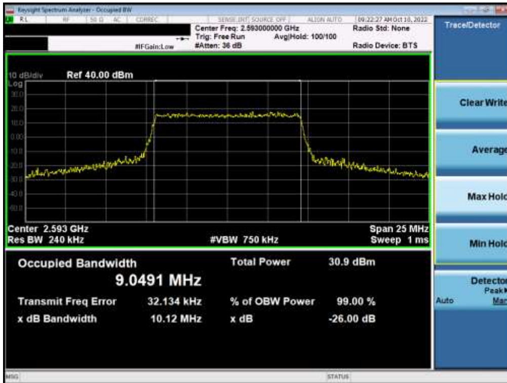
Plot 7-6. Occupied Bandwidth Plot (LTE Band 41(PC3) - 10MHz 16-QAM - Full RB)
