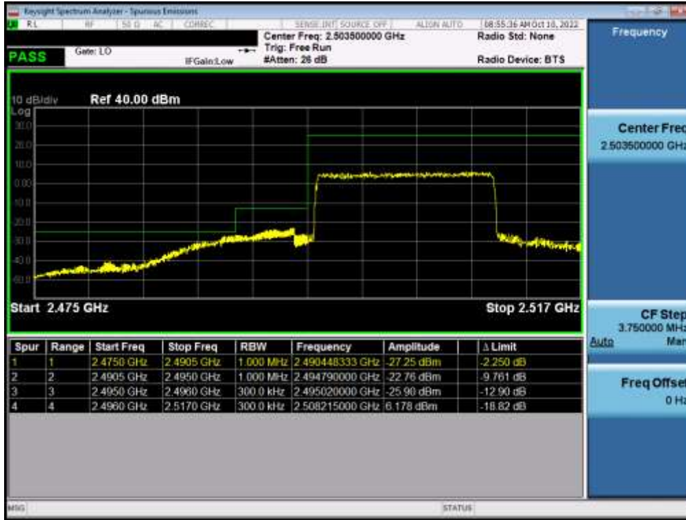
Plot 7-74. Lower ACP Plot (LTE Band 41(PC3) - 15MHz QPSK – Full RB - Ant B)
