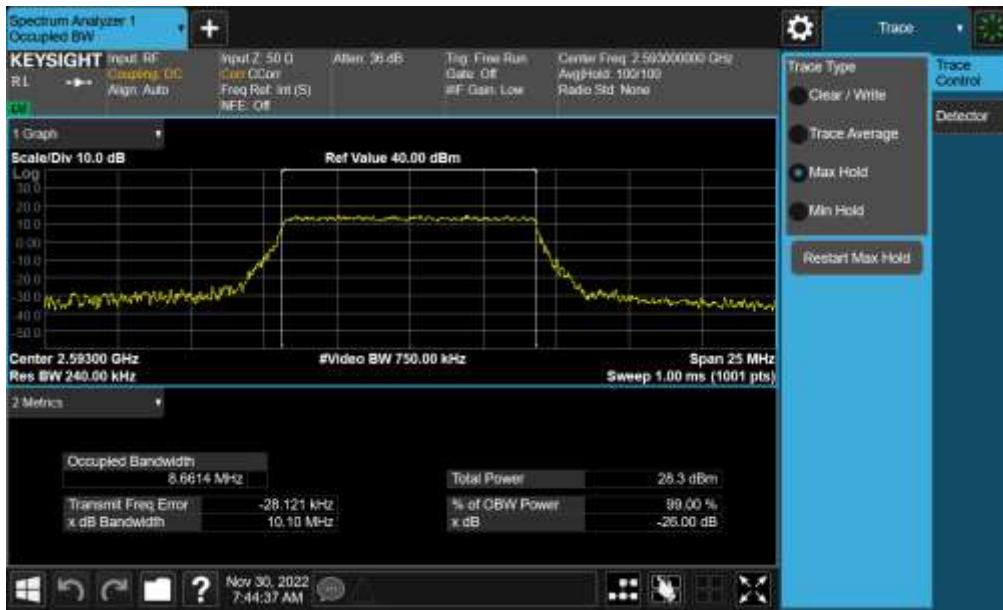
Plot 7-40. Occupied Bandwidth Plot (NR Band n41(PC3) - 10MHz QPSK - Full RB)
