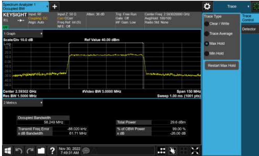
Plot 7-23. Occupied Bandwidth Plot (NR Band n41(PC3) - 60MHz 16-QAM - Full RB)
