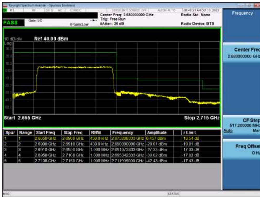
Plot 7-73. Upper ACP Plot (LTE Band 41(PC3) - 20MHz QPSK – Full RB - Ant B)
