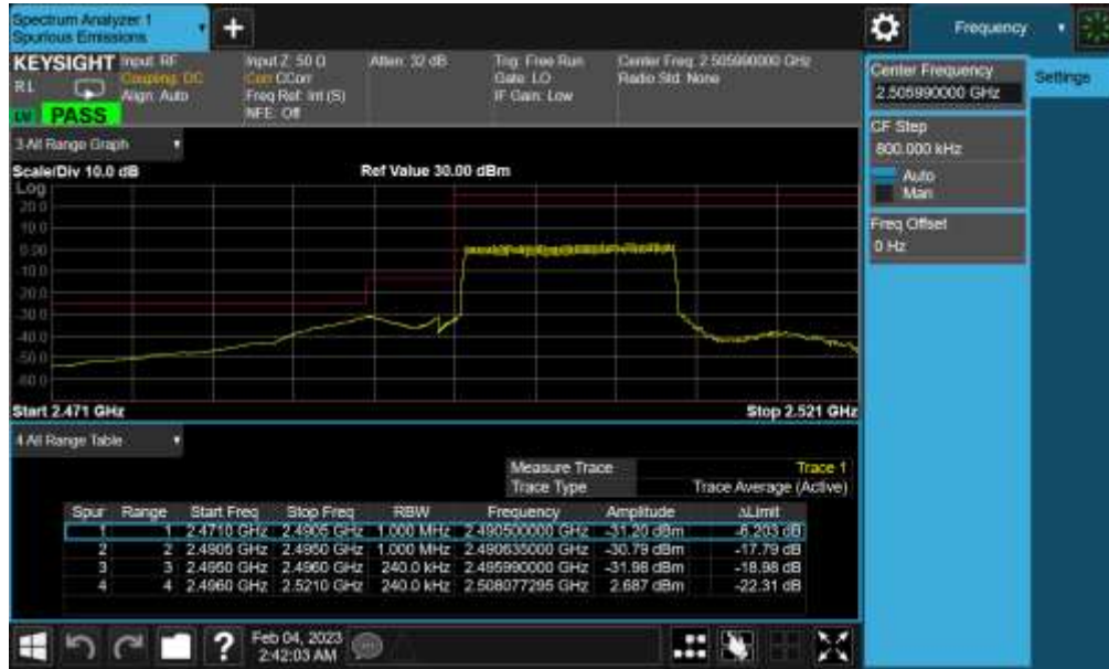
Plot 7-100. Lower ACP Plot (NR Band n41(PC3) - 10MHz CP-OFDM-QPSK – Full RB)
