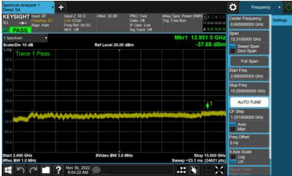
Plot 7-55. Conducted Spurious Plot (NR Band n41(PC3) - 100MHz QPSK - RB Size 1, RB Offset 0 - Mid Channel)
