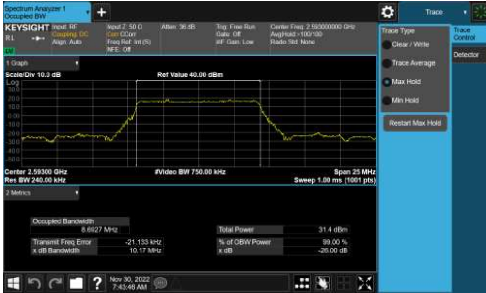
Plot 7-39. Occupied Bandwidth Plot (NR Band n41(PC3) - 10MHz \pi/2 BPSK - Full RB)
