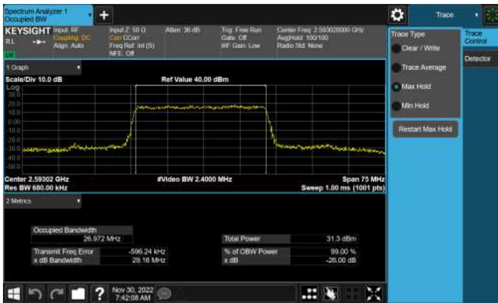
Plot 7-30. Occupied Bandwidth Plot (NR Band n41(PC3) - 30MHz \pi/2 BPSK - Full RB)
