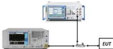
Figure 7-1. Test Instrument & Measurement Setup
