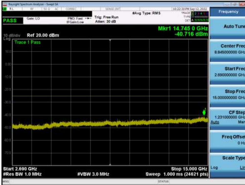
Plot 7-66. Conducted Spurious Plot (ULCA LTE B41(PC3) - 20MHz QPSK - RB Size 1, RB Offset 0 - Mid Channel - Ant B)
