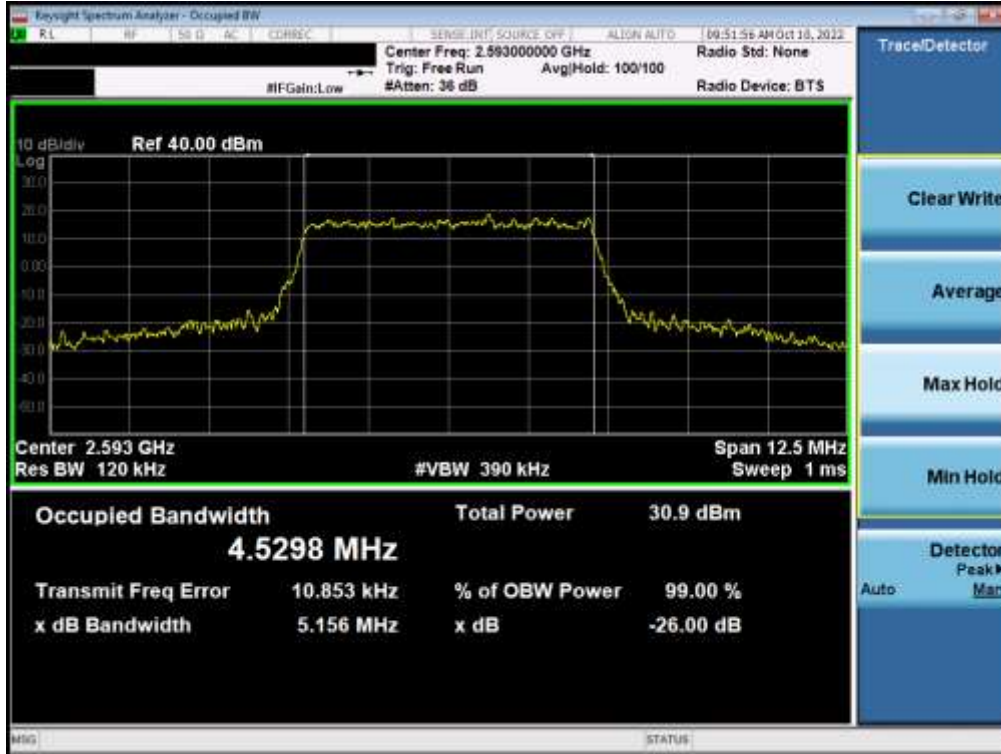
Plot 7-7. Occupied Bandwidth Plot (LTE Band 41(PC3) - 5MHz QPSK - Full RB)
