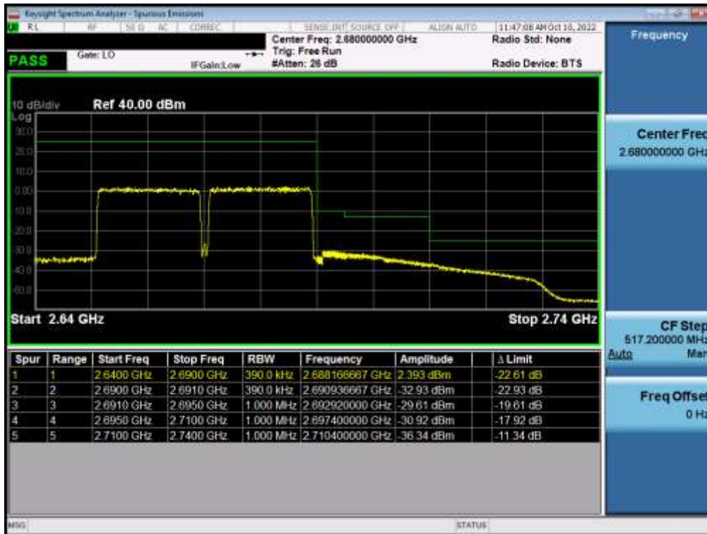
Plot 7-103. Upper ACP Plot (ULCA LTE B41(PC3) - 20MHz QPSK – Full RB)
