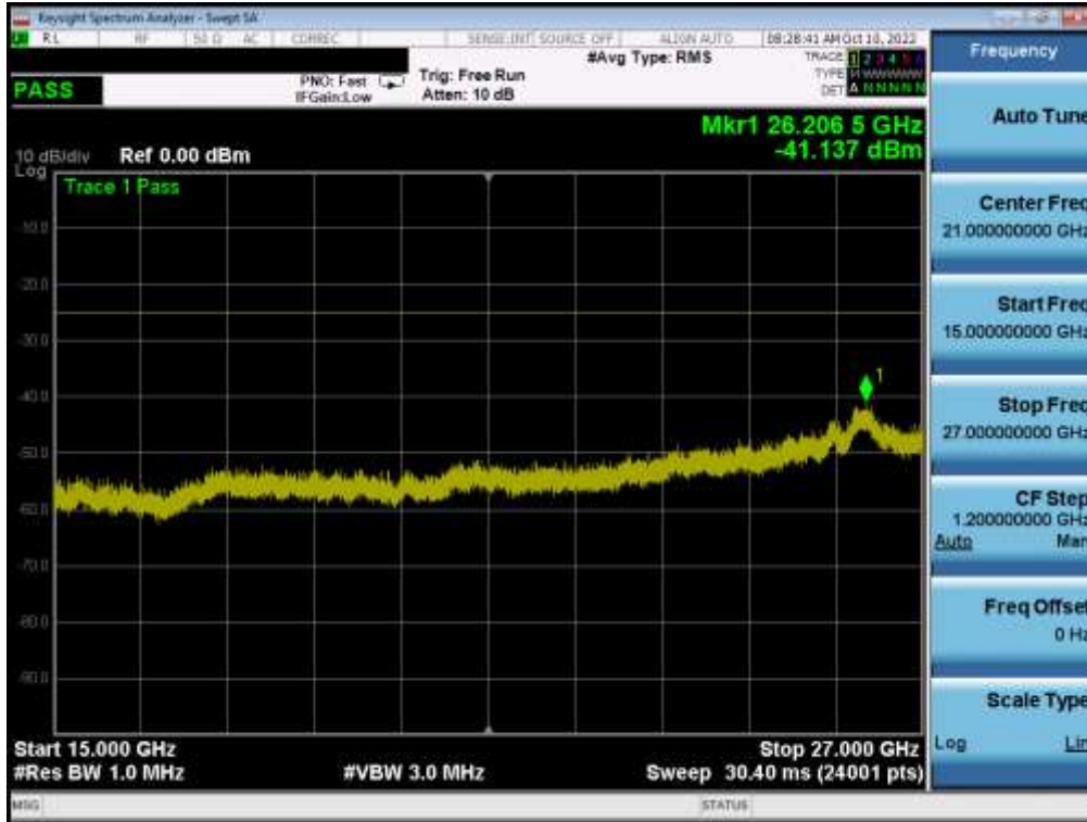
Plot 7-44. Conducted Spurious Plot (LTE Band 41(PC3) - 20MHz QPSK - RB Size 1, RB Offset 0 - Low Channel)
