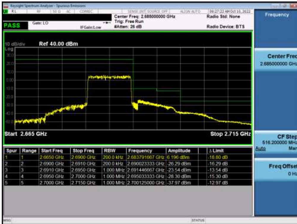
Plot 7-77. Upper ACP Plot (LTE Band 41(PC3) - 10MHz QPSK – Full RB - Ant B)
