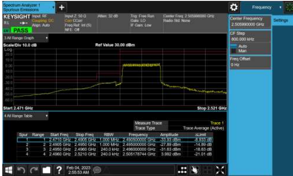
Plot 7-98. Lower ACP Plot (NR Band n41(PC3) - 15MHz DFTs-OFDM-QPSK – Full RB)
