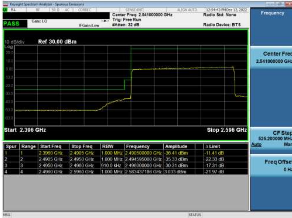
Plot 7-82. Lower ACP Plot (NR Band n41(PC3) - 90MHz CP-OFDM-QPSK – Full RB)
