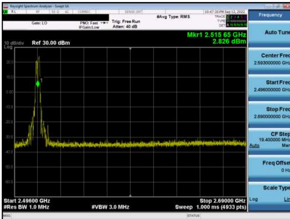
Plot 7-61. Conducted Spurious Plot (ULCA LTE B41(PC3) - 20MHz QPSK - RB Size 1, RB Offset 0 - Low Channel)
