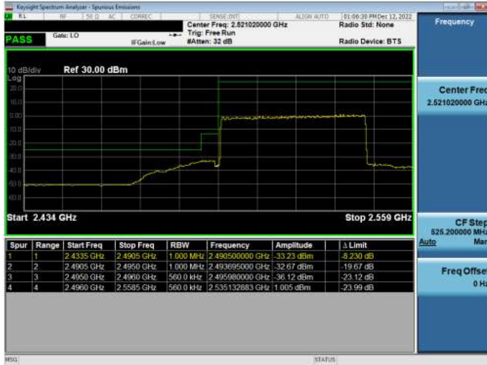
Plot 7-90. Lower ACP Plot (NR Band n41(PC3) - 50MHz CP-OFDM-QPSK – Full RB)
