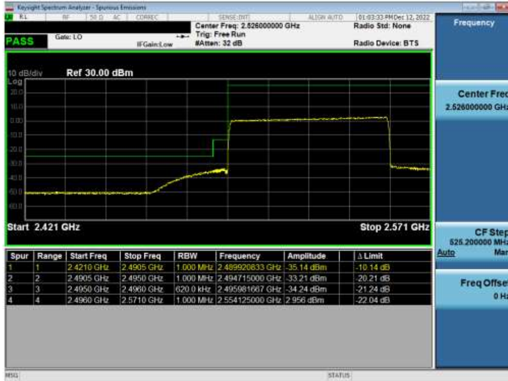
Plot 7-88. Lower ACP Plot (NR Band n41(PC3) - 60MHz CP-OFDM-QPSK – Full RB)
