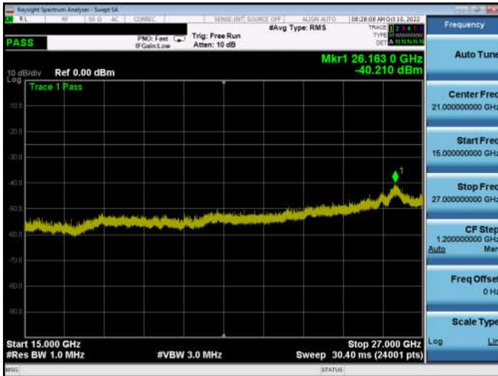
Plot 7-47. Conducted Spurious Plot (LTE Band 41(PC3) - 20MHz QPSK - RB Size 1, RB Offset 0 - Mid Channel)
