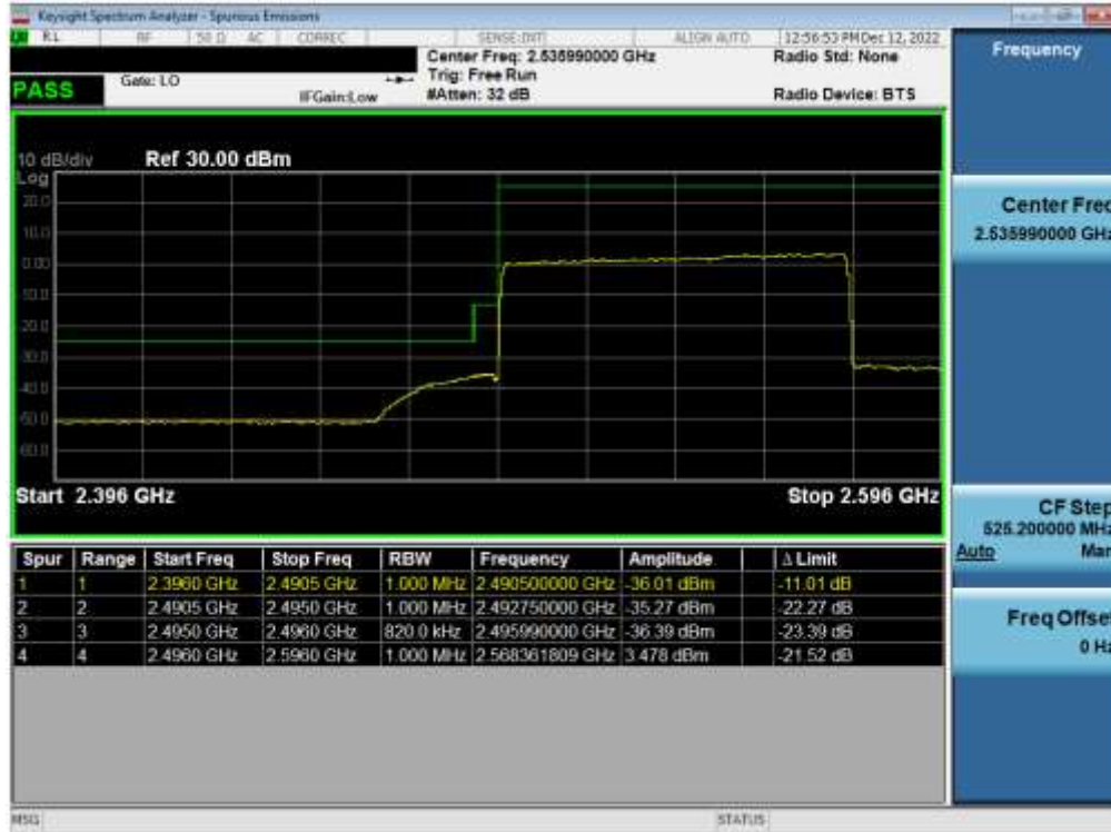
Plot 7-84. Lower ACP Plot (NR Band n41(PC3) - 80MHz CP-OFDM-QPSK – Full RB)
