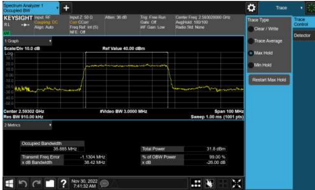
Plot 7-27. Occupied Bandwidth Plot (NR Band n41(PC3) - 40MHz \pi/2 BPSK - Full RB)
