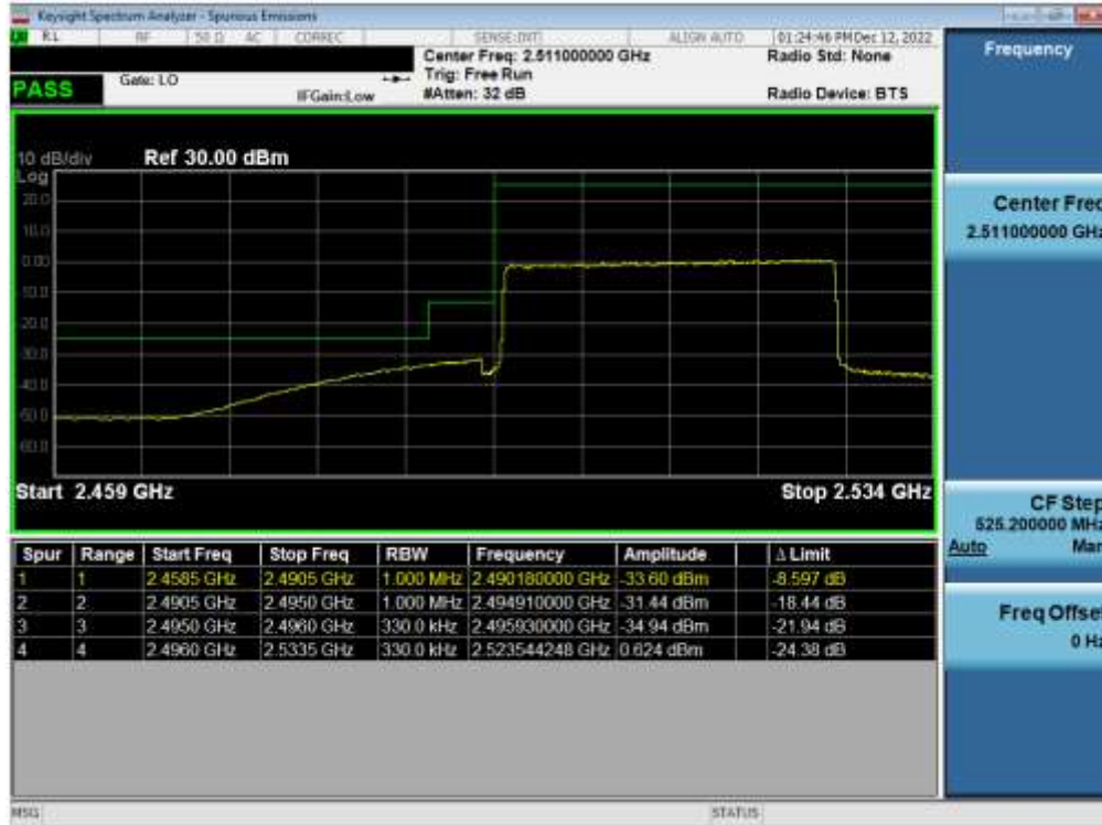
Plot 7-94. Lower ACP Plot (NR Band n41(PC3) - 30MHz CP-OFDM-QPSK – Full RB)
