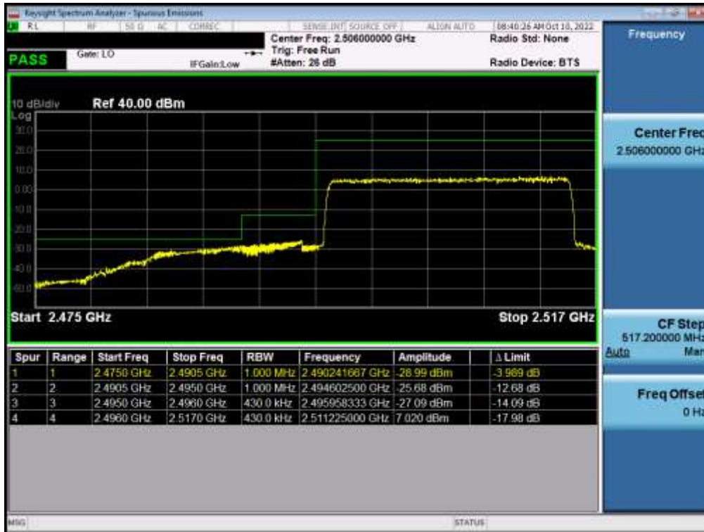
Plot 7-72. Lower ACP Plot (LTE Band 41(PC3) - 20MHz QPSK – Full RB - Ant B)
