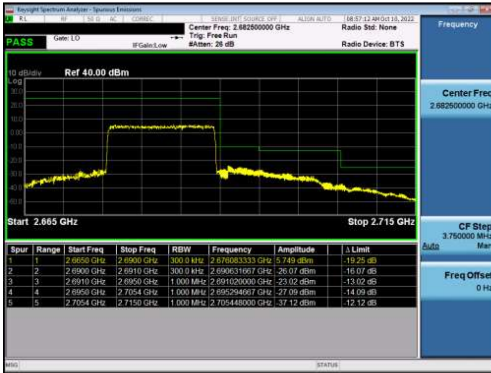
Plot 7-75. Upper ACP Plot (LTE Band 41(PC3) - 15MHz QPSK – Full RB - Ant B)
