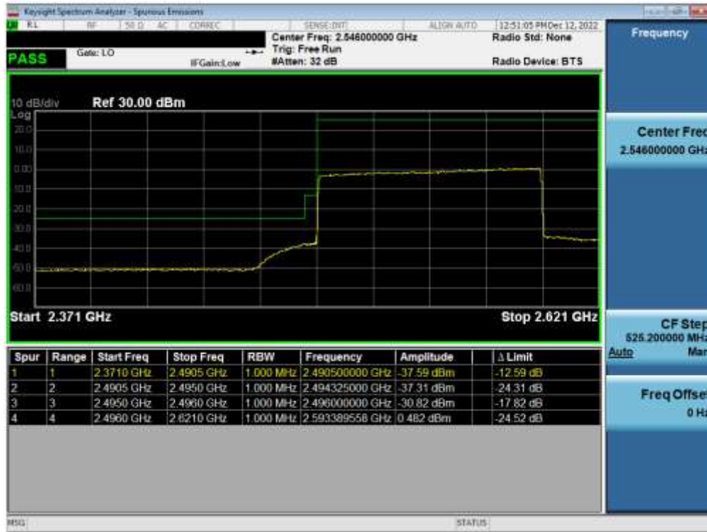
Plot 7-80. Lower ACP Plot (NR Band n41(PC3) - 100MHz CP-OFDM-QPSK – Full RB)
