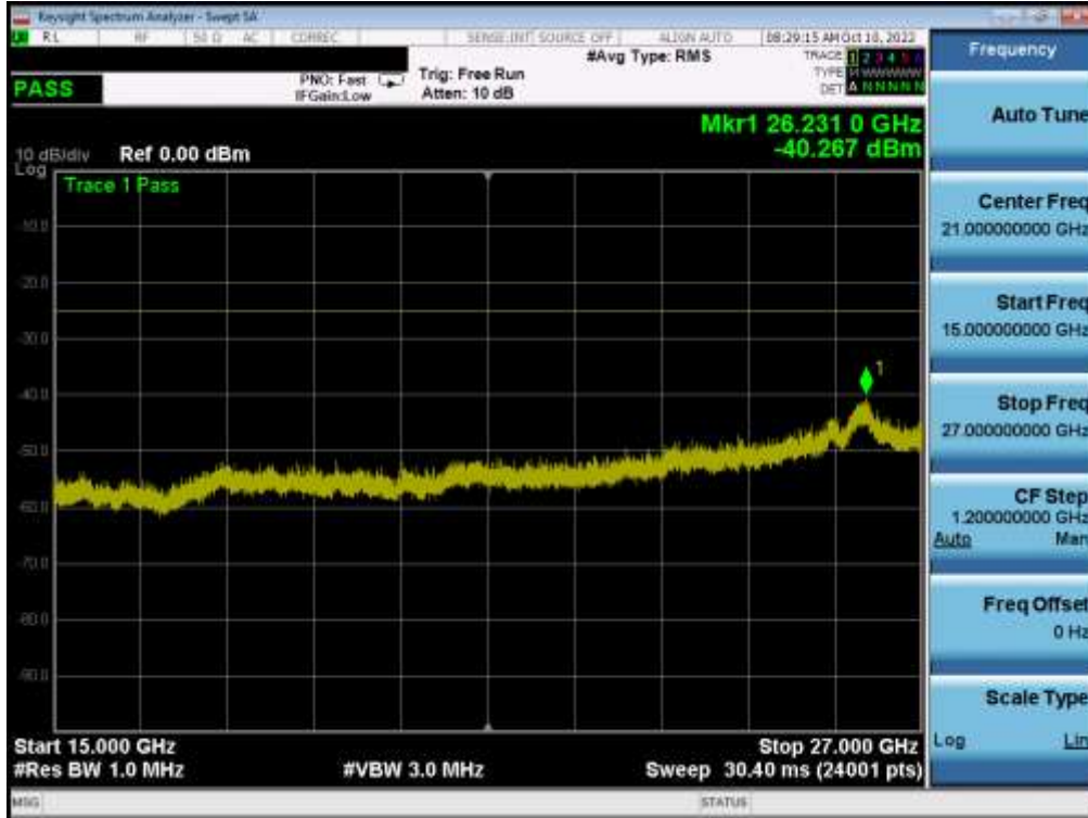
Plot 7-50. Conducted Spurious Plot (LTE Band 41(PC3) - 20MHz QPSK - RB Size 1, RB Offset 0 - High Channel)
