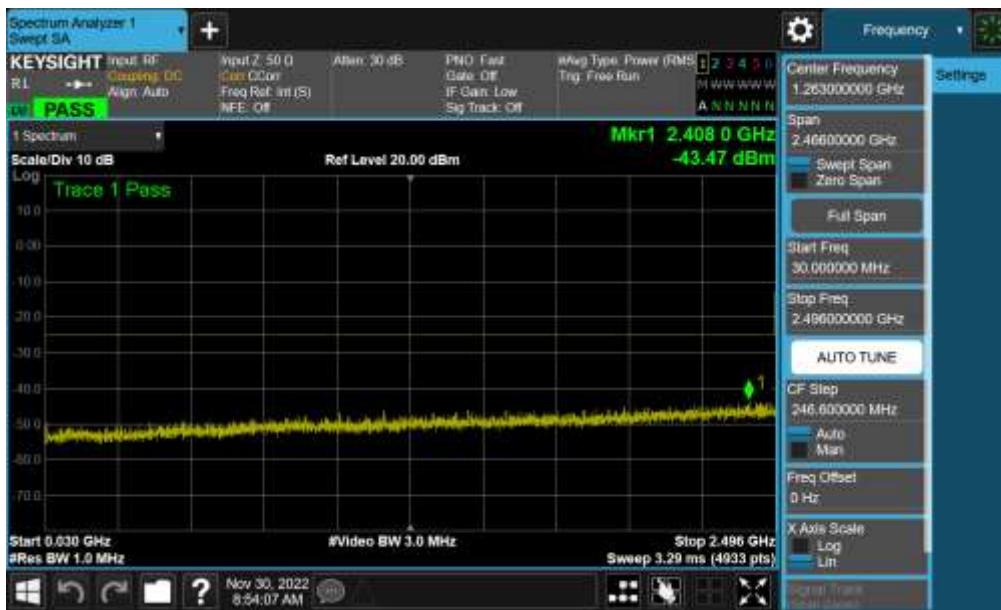
Plot 7-54. Conducted Spurious Plot (NR Band n41(PC3) - 100MHz QPSK - RB Size 1, RB Offset 0 - Mid Channel)
