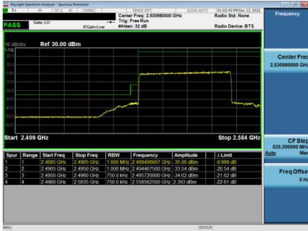
Plot 7-86. Lower ACP Plot (NR Band n41(PC3) - 70MHz CP-OFDM-QPSK – Full RB)
