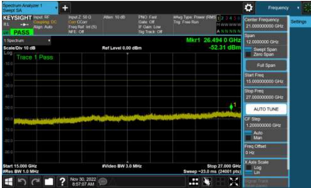
Plot 7-53. Conducted Spurious Plot (NR Band n41(PC3) - 100MHz QPSK - RB Size 1, RB Offset 0 - Low Channel)
