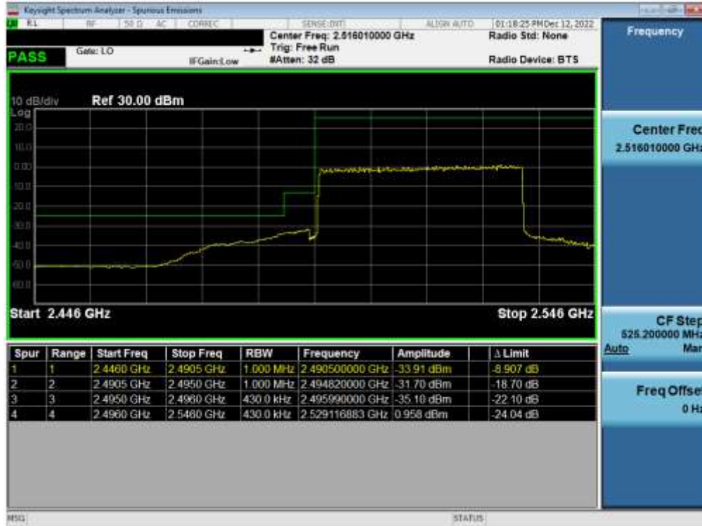
Plot 7-92. Lower ACP Plot (NR Band n41(PC3) - 40MHz CP-OFDM-QPSK – Full RB)
