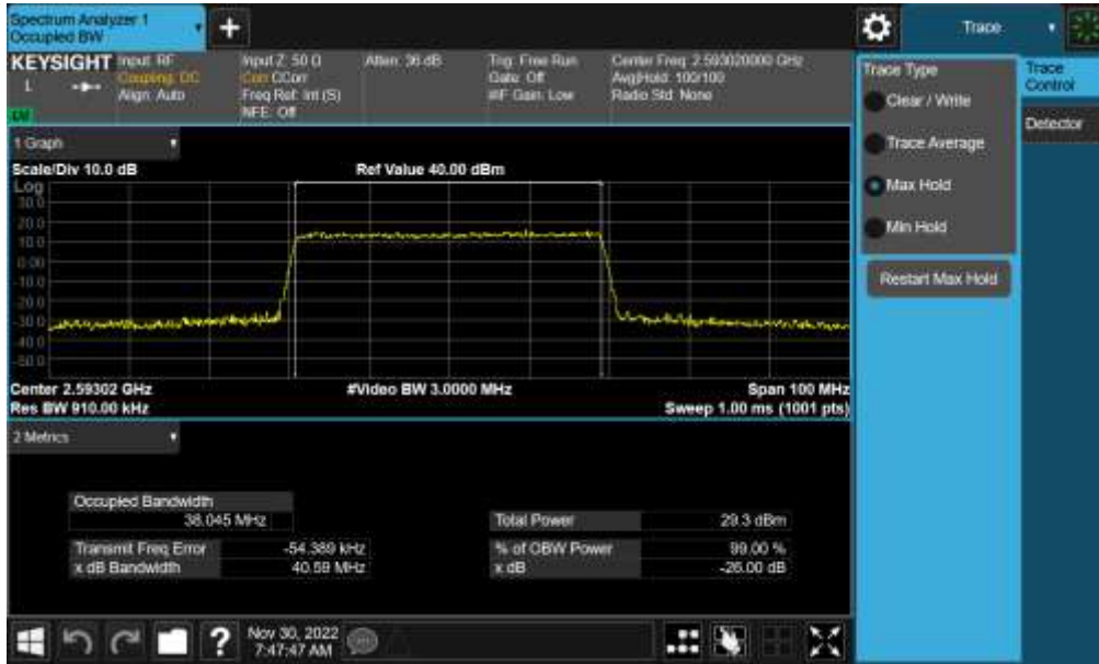
Plot 7-29. Occupied Bandwidth Plot (NR Band n41(PC3) - 40MHz 16-QAM - Full RB)
