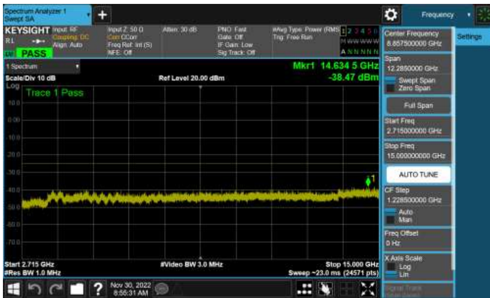
Plot 7-58. Conducted Spurious Plot (NR Band n41(PC3) - 100MHz QPSK - RB Size 1, RB Offset 0 - High Channel)
