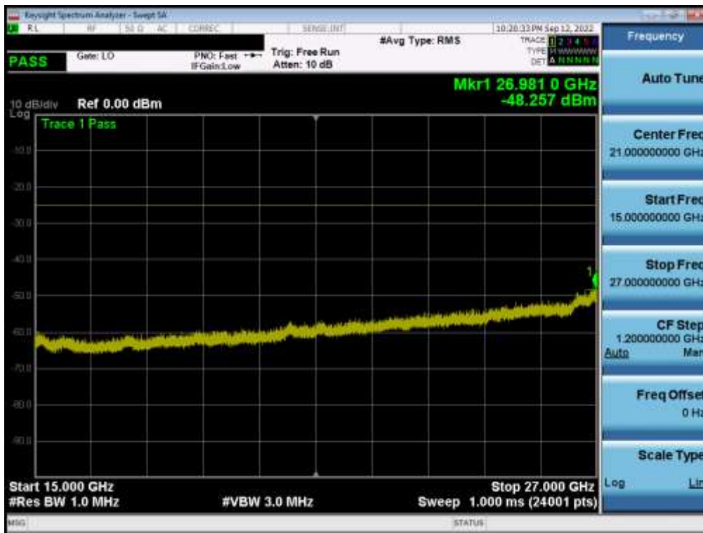
Plot 7-63. Conducted Spurious Plot (ULCA LTE B41(PC3) - 20MHz QPSK - RB Size 1, RB Offset 0 - Low Channel)
