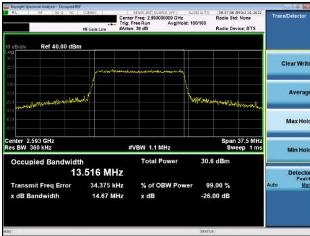
Plot 7-4. Occupied Bandwidth Plot (LTE Band 41(PC3) - 15MHz 16-QAM - Full RB)
