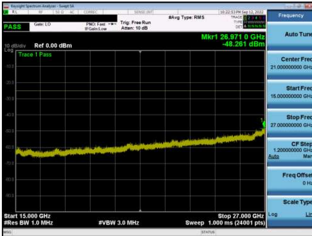
Plot 7-67. Conducted Spurious Plot (ULCA LTE B41(PC3) - 20MHz QPSK - RB Size 1, RB Offset 0 - Mid Channel)
